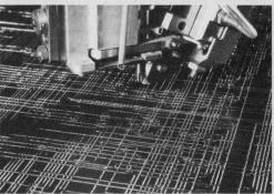
But cost is not the only reason for the superiority of Multiwire over wirewrapping. There are also design advantages. For example, Multiwire offers two-dimensional packaging density equal to wirewrapping. But with Multiwire panels, you reduce board-to-board spacing. And Multiwire weighs much less too. So it can contribute substantially toward improving the envelope or three-dimensional package of your product.
