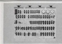
The TCU-100, a self-supporting timekeeper for a PDP-11, can give you the time as follows: month and day, hours and minutes, seconds. It can be initialized by simple commands from the computer and features rechargeable battery power for uninterrupted use when the computer is off, plus extensive interrupt capability. Price: \$495. For literature, write or call Digital Pathways, 4151 Middlefield Road, Palo Alto, CA 94306. (415) 493-5544.
