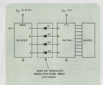
1. An inexpensive CMOS-TTL interface can be made of a diode array or of individual signal diodes. The diodes must be able to withstand a reverse voltage equal to  $V_{\rm ce}$  and to have a forward drop less than the TTL LOW level.
