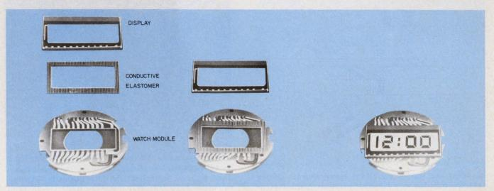
3. A tiny assembly such as a watch module can use the material to provide shock mounting and electrical connection.
