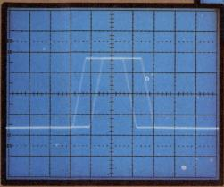
**Position intensified spots** at beginning and end of time interval.
