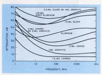
Shielding effectiveness of conductive coatings varies with material type and coating thickness. Typical attenuations of Acheson Colloids' formulation on a 0.125-in.-thick polycarbonate sheet are shown.
