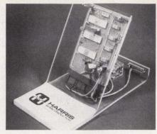
Just four circuits are needed to build a minimal operating system—the 6100, a ROM, a RAM and a PIE.
