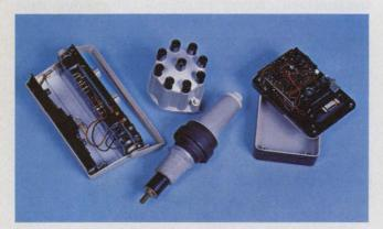
Conductive silver coatings, sprayed inside the plastic cases of a sensitive digital meter (left) and analog meter (right), protect meter circuits from EMI. Coatings on distributor cap (top center) and circuit-breaker bushing (bottom center) reduce radiated EMI.
