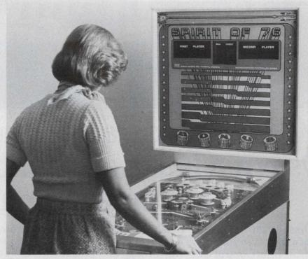
Microcomputer control of a pinball machine makes troubleshooting simple. The Mirco Games unit uses only 1/10 the power of regular machines.
