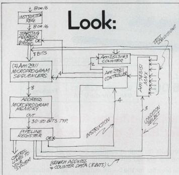
The Am2911 provides logic for sequential addressing, branching to any address, four levels of subroutining and looping. The Am29811 is used to control the Am2911, as well as a loop
