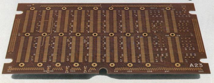
Two major systems — wirewrapping and multilayering — have been used for complex electronic interconnection in the last 15 years. Despite improvements and refinements, each still has inherent disadvantages. That's why Multiwire was created by Photocircuits. It overcomes the disadvantages of wirewrapping and multilayering.
