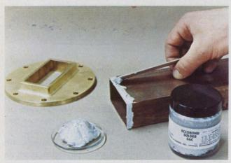
This waveguide and flange is assembled by using a twocomponent Emerson & Cuming conductive silver "epoxy solder." It forms a rigid connection.
