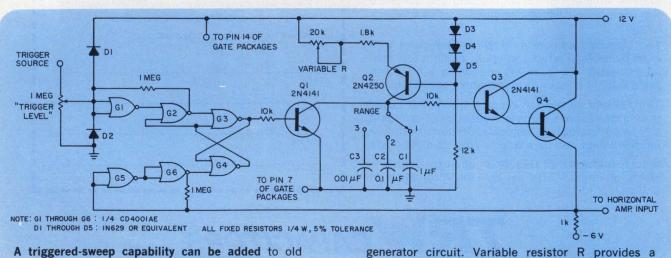
A triggered-sweep capability can be added to old recurring-sweep scopes with this simple trigger-
