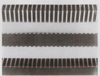
2. Alternate layers of conducting and nonconducting elastomers produce a material that connects PC board contacts to external components.
