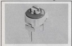
MINIATURE CERAMIC TRIMMER CAPACITORS 9371 series of ceramic trimmer capacitors are compact, economical and rugged. They are 50% smaller than other trimmers of this type yet provide high capacitance values. Available in 4 capacitance ranges, 1.5 to 4, 3.0 to 10, 3.5 to 18 and 5.0 to 25 pf with Q's > 300 at 10 MHz. They have an overall diameter of .225" with .215" above board height. JOHANSON MANUFACTURING CORPORATION, Rockaway Valley Road, Boonton, N.J. 07005 201-334-2676
