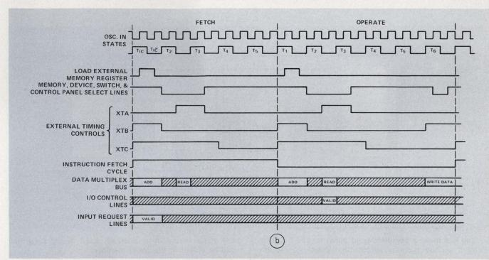
1. By using a shared address and data bus, the pin count of the 6100  $\mu\text{P}$  can be kept to 40 (a). Timing
