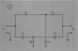
1. The notch filter (a) as it appears in application notes for op amps seems quite simple. The classical twin-tee notch filter (b) requires that the capacitors and resistors be matched for maximum notch attenuation.
