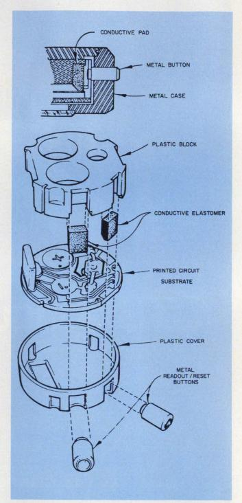
1. Conductive elastomers used as switch elements replace mechanical switches in a digital watch.
