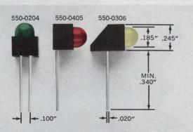
Mix 'em or match 'em. LED logic state fault indicators are available in red, yellow and green, in a variety of shapes, some with a built-in integral resistor. Can be driven from DTL and TTL logic. Designed for easy alignment on PC boards so that multiple functions can be displayed.
