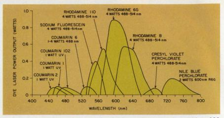
Various dyes can be used to tune the dye laser all the way from 400 to 800 nm. These are some of the typical dyes used. The performance data are for the Spectra-Physics Model 375 high-performance CW dye laser.
