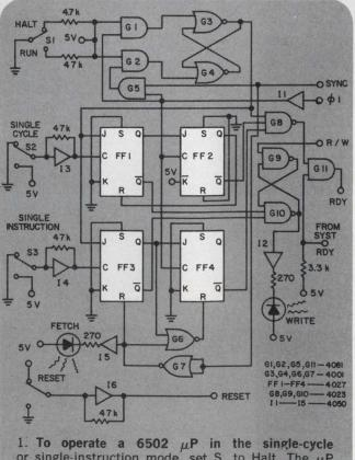
1. To operate a 6502  $\mu$ P in the single-cycle or single-instruction mode, set S<sub>1</sub> to Halt. The  $\mu$ P will then stop at the proper time to allow you to initiate either mode by momentarily pressing either S<sub>2</sub> or S<sub>3</sub>.
