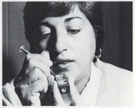
**Photodiode/preamplifier** weighs a scant 40 gms, yet provides high sensitivity. Its characteristics can be modified for specific applications.
