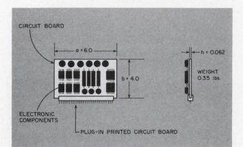
4. The plug-in printed circuit board used in the example is 0.062-in. thick and made of G-10 epoxy-fiberglass, a very common construction.
