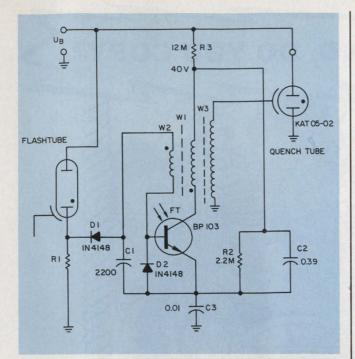
6. This computer-controlled photoflash circuit integrates the photocurrent with  $C_1$ . Only when the base-emitter junction is turned on does the oscillator start to trigger the quench tube.
