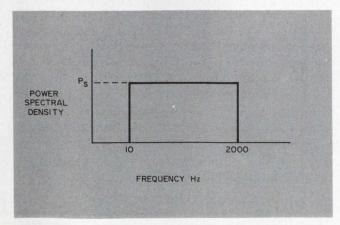
3. A white-noise power spectrum contains a uniform power spectral density over a given frequency range. It is a commonly specified environment for boards.
