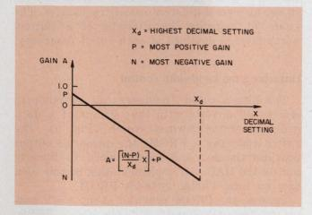
3. The cutoff frequency of the filter can be linearly related to decimal settings of a thumbwheel switch that controls the gain of the filter-system amplifiers. adjustment establishes both limit values. In Fig. 2, maximum gain, N, is set at -7 and P at approximately 0.65. The cutoff frequency range is greater than 20:1.
