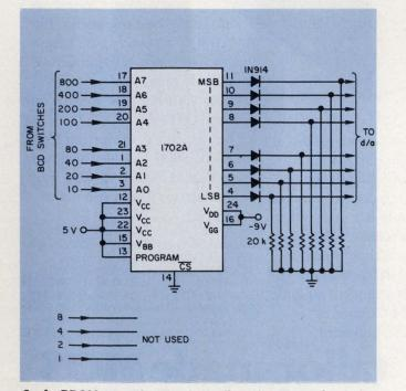
6. A PROM can be used to linearize control of the filter's cutoff frequency and allow the use of a thumb-wheel-switch to set the cutoff value.
