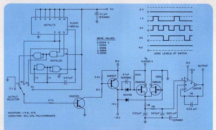
Accurate voltage division, is obtained by controlling the duty cycle of a digital signal applied to the FET switches. After averaging, the output is a precision voltage essentially independent of component drift.
