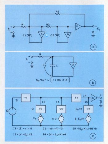
1. A two-pole Butterworth low-pass filter can be built from two capacitor-multiplier circuits in tandem (a), made up of two basic circuits (b) with an over-all feedback resistor,  $R_3$ . A generalized equivalent circuit (c) helps in deriving performance equations for the filter.
