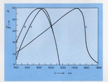
1. **Relative spectral response curves for photodiodes** compare the responses of normal silicon devices (a), silicon with enhanced response in the blue portion of the spectrum (b) and germanium photodiodes (c).
