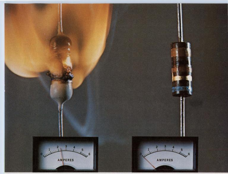
**The failure.** A 16 W overload causes this 1/2 W carbon film resistor to burst into flame. The initial failure mode is a short circuit, causing even more current to be drawn as shown on the meter.
