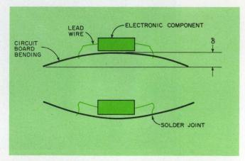
1. Circuit boards bend during vibration, with the most severe stresses on the lead wires of the components in the center of the board.
