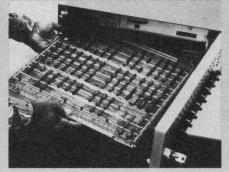
You can turn a Nova minicomputer into a parallel, multiprocessing system by plugging in some Micro-N microprogrammable processors. The Micro-N, developed by Educational Data Systems (17981 Sky Park Circle, Irvine, CA 92707. 714-556-4242), enhances the computing power of any Nova minicomputer by implementing user-defined, procedure-oriented macro-instructions.
