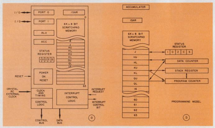
4. The CPU chip contains a 64  $\times$  8-bit RAM, two 8-bit I/O ports and internal clock (a). It also has a power-on reset function and 16 TTL-compatible I/O lines. All 64
