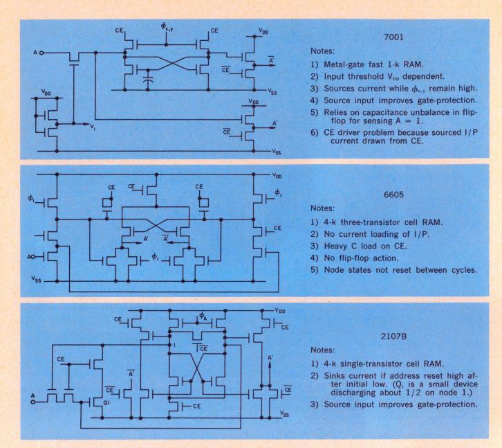
4. The input-buffer circuits of three high-performance MOS RAMs all show compromises in design caused by
