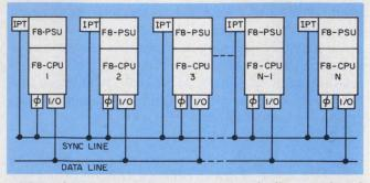
4. Data bus controllers can be dynamically reassigned so that if one device fails another may take over, still allowing the system to function.
