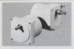
**Dual Speed Unidirectional Synchronous** Motor (Series 86000) offers advantages for instrument drives, especially strip chart recorders and telecopiers. Available torque to 35 oz-in. Choice of square or NEMA 2-11 gear box gives wide range of dual speed combinations. Fast start/stops eliminate need for clutching and prestarts. Available in 24, 120 or 240 VAC, 60 Hz, with CW or CCW rotation. Weight 30 oz. U/L listed. North American Philips Con-trols Corp. Cheshire, Conn. 06410 (203) 272-0301.
