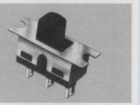
Model 1101 Slide Switch, subminiature SPDT in either Printed Circuit or Panel mount models. Electrical life: 40,000 actuations at full load. Contact rating: 6 amps with resistive load @ 120 VAC or 28 VDC; or 3 amps with resistive load @ 250 VAC. Free engineering sample on request. C&K Components, Inc., 103 Morse St., Watertown, MA 02172 Tel: (617) 926-0800 TWX: 710-327-0460 TELEX: 92 2546
