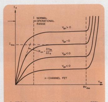
2. With its gate connected to its source, a FET's saturation drain-source current,  $I_{\rm dss}$ , can be used to limit current and protect a circuit against shorts.
