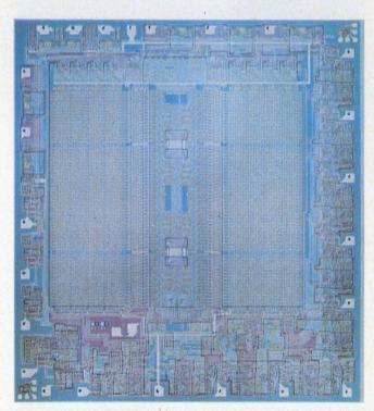
$C^{2}L$ , or closed CMOS logic, is used in the RCA CDP1832 512 × 8 memory for small size and high drive capability. Access speeds are between 200 and 400 ns.
