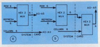
6. To accommodate all of the RAM pinouts you need slightly more address multiplexing on the board. Shown are circuits for (a) 18 and 22 or (b) 16 pins.
