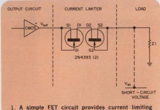
1. A simple FET circuit provides current limiting for easily damaged circuits.
