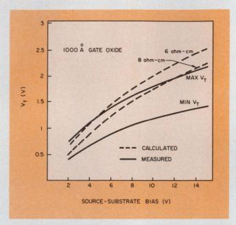
1. MOS-transistor threshold voltage,  $V_{\rm T}$ , varies with substrate resistivity and source-substrate bias.
