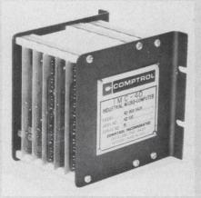
The IMC-40 industrial microcomputer can replace many larger machine and process-control systems. The  $\mu$ C consists of a 4040 CPU and can hold up to an 8-kilobyte control program. Since the I/O circuits use high-noiseimmunity logic, the IMC-40 is practically immune to industrial noise.
