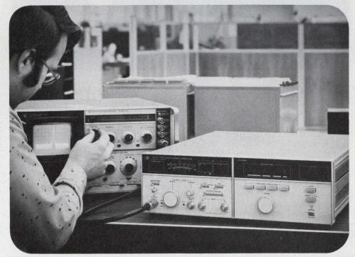
The new HP 8672A Synthesized Signal Generator with wide dynamic range and exceptional stability provides features important to both broadband testing or to highly stable receiver tests.
