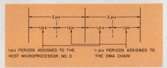
7. Memory time slices are allocated alternately to the host microprocessor and to the remaining processors.
