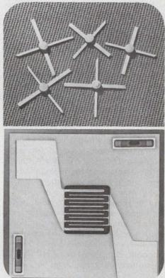
A new NPN bipolar transistor utilizing ion implantation techniques in its manufacture is provided with scratch protection over its active area.
