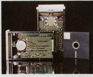
The 2230-line printer from Dataproducts has an unusual drum and hammer-bank design. This 300-lpm printer is ideal for minicomputer applications.
