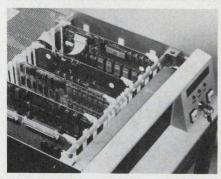
New modules for Motorola's EXORciser enhance its  $\mu$ P-debugging and test capabilities.
