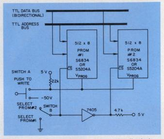
1. Different PROMs can be programmed collectively a key requirement for board programming. To write (program) data in or read them out, use switch B to select a PROM. For programming, apply address and data, and then depress switch A. For a read operation, simply apply an address; data will then appear on the bus.
