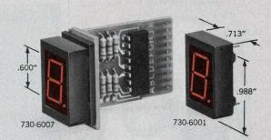
**730 SERIES** A new 0.600" LED character in super bright red, seven-segmented readout . . . low power . . . draws 10mA/segment or less . . . operates with standard IC power supply levels. Very high contrast ratio . . . visible from 40'. Available with or without on-board decoder/driver, plus or minus bar, and with bezel mounting. In 1000-lot quantities each LED **730-6007** . . . . **\$6.05**. **730-6001** . . . . **\$2.55**.
