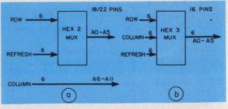
5. Systems may use boards designed for just one or two **RAM pinouts:** either (a) the 18 and 22 pin types or (b) the 16-pin version.
