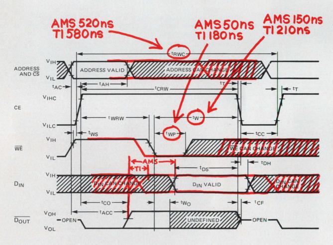
The excessively short system modify time for TI's 4060 stems from the fact that the  $\overline{\text{WE}}$  line must go low 60 ns earlier than our 7280. TI's Data In must be stable when  $\overline{\text{WE}}$  goes low, while ours only requires that Data In be stable 150 ns prior to CE going low, a clear advantage of 60 ns for the 7280, 80 ns for the 7270.
