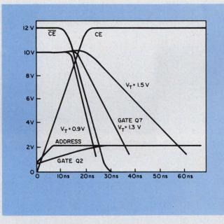
3. **RAM input-buffer delay** depends on the threshold voltage,  $V_{\rm T}$ , as shown in these simulated steering waveforms. Speeds can be increased, if unrealistic "TTL-compatibility" specifications are modified.
