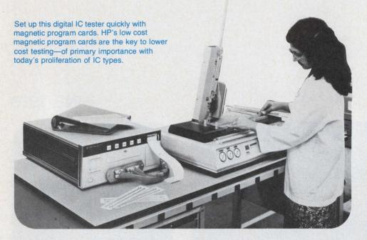
Insert an inexpensive magnetic programming card, and in five seconds this new multi-family Model 5045A digital IC tester is ready for dc parametric and functional testing of digital ICs. It's that simple—absolutely no other set-up or programming is needed. And it'll do some of your RAM and ROM testing too. Programming is so versatile that it can set-up a unique voltage and current level on each pin of the device under test within the limits of  $\pm 200$  mA and 0 to 15V or  $\pm 7.5V$  range.
