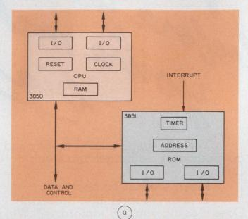
1. Two LSI chips comprise the minimum F8 system (a). One chip is the 3850 CPU, and the other is the 3851 program-storage unit. The latter performs all addressing functions, eliminating the need for an address bus and permitting the extra pins on both circuits to be used for I/O. The capabilities of the two-chip system can satisfy the bulk of control applications (b).
