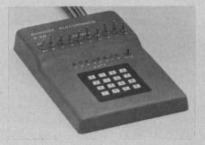
You can cut program development costs for  $\mu$ Ps by using a random-access memory that can be programmed by a remote keyboard. At least that's what Sunrise Electronics (228 N. El Molino, Pasadena, CA 91101. 213-793-7552) says about its series of KPRAM development tools.
