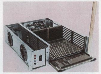
The first million-byte semiconductor memory to fit into a  $5 \cdot 1/2 \cdot in$ . high rack mount is produced by Control Data. It contains eight storage cards organized 64-k by 20, in 10-bit bytes to provide bits for error correction.
