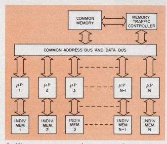
5. Microprocessors may have access to a common memory for general data, and an individual memory for program execution.
