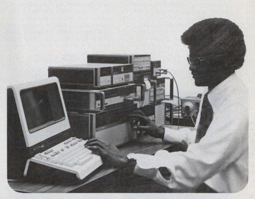
Now, system designers can connect HP-IB instruments, like the DVM, scanner, numeric display, thermal printer, timing generator, counter, and digital-analog converter shown above, to the powerful control, data processing, and storage capabilities of Hewlett-Packard Real-Time Minicomputers.
