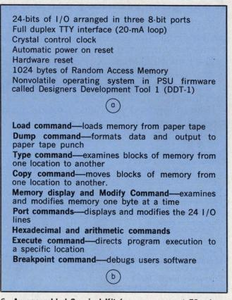
6. An assembled Survival Kit forms a compact F8 microcomputer with the features indicated (a). Application software can be written and executed by using commands stored in the PSU (b). The kit comes with a Fortran IV cross-assembler.
