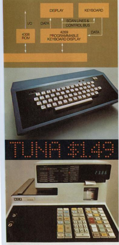
and system memory for display refresh since the necessary memory and control are built in. One 4269 can operate and refresh alphanumeric displays or indicator arrays with up to 32x4 digits, 16x8 characters or any configuration of 128 elements or lights, including a 20-character Burroughs Self-Scan\* Display.
