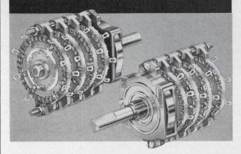
Reduce your design time with this 1½" diameter rotary switch. 8 to 36 positions, depending on detents selected (11 available, from 10° to 45°) allowing thousands of switching variations. Crisp, uniform ball and starwheel Unidex<sup>®</sup> detent. Double-wiping, self-cleaning, high-pressure contacts. Military types available.
