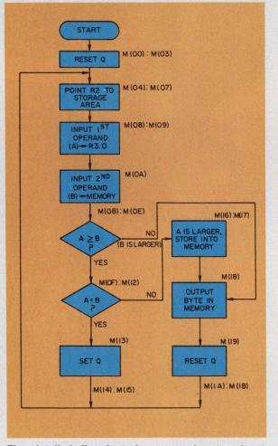
The detailed flowchart for processing two input bytes is used as the basis for writing the microprocessor program. ucts manager at Intel, Santa Clara, CA.
