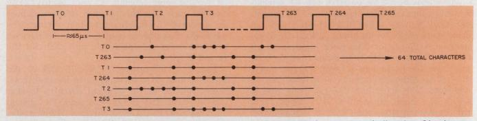
7. RAMs used as display buffers can access the points on a raster-scan display to automatically select 64 columns.
