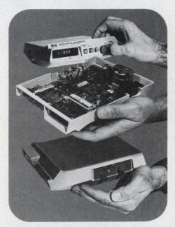
Compact new DMM with advanced circuitry and packaging resulting in high reliability. One circuit board contains all the electronics.
