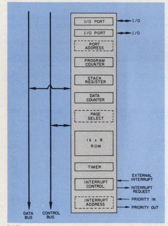
5. The 3851 program-storage unit, a mask-programmable IC, has memory-reference functions.
