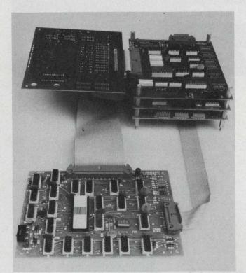
The MIKE-3 system of boards from Martin Research contains  $\mu$ P and clock, keyboard and display, debug, and memory—each on a separate plug-in board that connects with the others (3 boards plus 2 optional).
