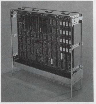
**Digital Equipment Corporation's LSI-11** is a 16-bit  $\mu$ C compatible with the firm's PDP-11 line of computers. I/O and additional memory cards are also available.
