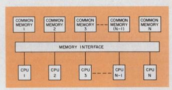
10. Systems that have individual subports of common memory allow fast operation, but require complex memory interface circuitry.
