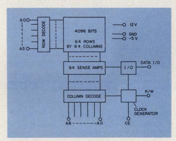
2. An 18-pin dynamic RAM has a single bidirectional data line. It has one fewer power pins than the 22-pin version and no chip-select pin.
