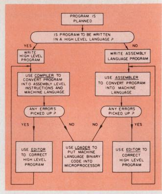
4. The binary code to be placed in a microcomputer's read-only memory can be prepared with the aid of a compiler or assembler, and with an editor and a loader. The compiler permits programming in a high-level language, which is simpler to use than an assembly language.
