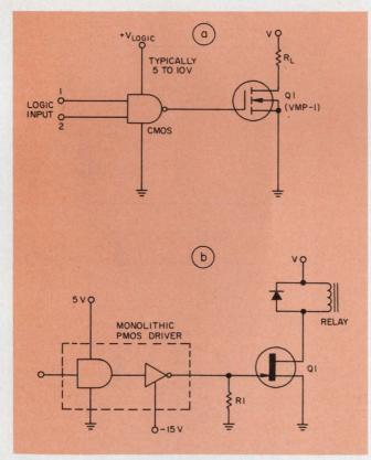
2. Enhancement-mode MOSFETs require no extra components to interface to CMOS logic circuits (a). N-channel JFETs, on the other hand, require an extra interface circuit to provide the negative gate bias (b).
