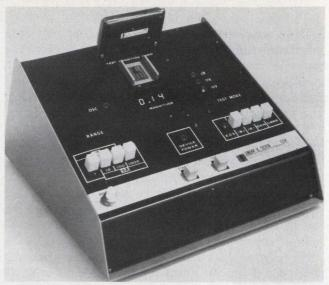
You can test six important op amp parameters with the ESI 1234:  $E_{\rm os}$ ,  $\pm I_{\rm B}$ , gain, CMRR and stability. Go/no-go testing is also possible.
