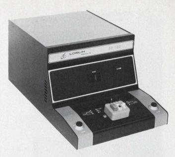
One advantage of computer control is that it allows multiple test stations. On Lorlin's SS100 station, you can test op amps, voltage regulators and interface ICs.
