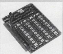
Two compact memory systems built with 4-k bit dynamic MOS RAMs offer direct compatibility with 8-bit  $\mu$ C systems.
