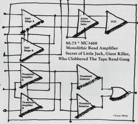
My EGC (Electronic Gain Controlled) amplifier provides differential outputs for the active differentiator and a single output is available for threshold function.
