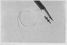
World's Smallest Displacement Transducer. Make precision, noncontacting displacement measurements at points never before possible. This new transducer, 0.080" OD, gives accuracy of  $<100~\mu$ in. in a range up to 0.020". Temperature stable. Repeatability and resolution is better than 10  $\mu$ in. Price \$485, including associated electronics. Kaman Sciences Corporation, P. O. Box 7463, Colorado Springs, CO 80933. (303) 599-1892.
