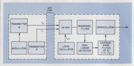
2. Communications systems with transmitters and receivers moving with respect to each other can use the Teich system to provide an output that cancels the Doppler shift. The analog-system shown has one carrier modulated.
