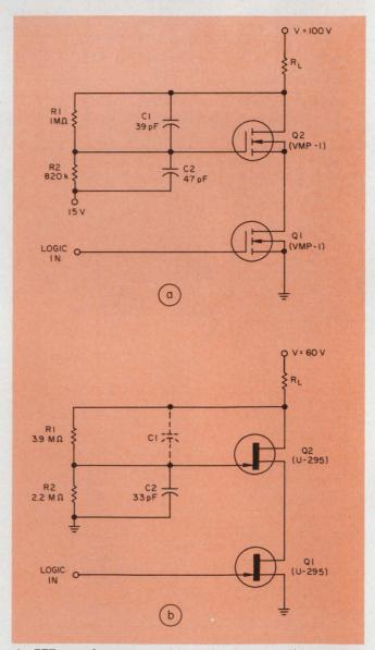
4. FETs can be connected in series for operation at higher voltages. Whether you use a MOSFET (a) or a JFET (b), the circuit to keep  $Q_2$  ON is similar. Power dissipation, though, is low since very little current is needed to keep  $Q_2$  ON.
