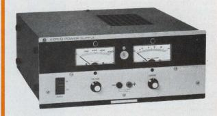
Control voltage with a 10-turn precision panel control (or program like the OPS). Another 10-turn panel control adjusts the output current. LED annunciators signal operation in either voltage mode or current modes. A built-in "uncommitted preamplifier" is available for scaling or summing programming inputs. Output is monitored on a pair of 2½" meters.
