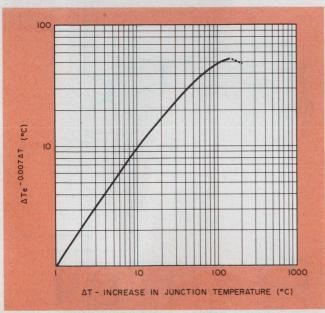
5. This plot of  $\Delta T$  e<sup>-0.007 $\Delta T$ </sup> versus  $\Delta T$  is useful when you have to find the rise in junction temperature and you know the power dissipation at ambient.
