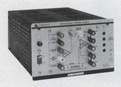
You may exercise control over the high voltage output with a 0–5V control signal, or use the built-in pre-amplifier to scale or sum your inputs operationally. The output follows input signals with a 100  $\mu$ sec programming time constant (OPS 500B). Current limit is both adjustable and electrically programmable.
