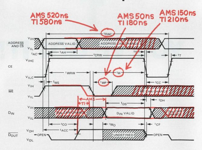
The excessively short system modify time for TI's 4060 stems from the fact that the  $\overline{WE}$  line must go  $\underline{low}$  60 ns earlier than our 7280. TI's Data In must be stable when  $\overline{WE}$  goes low, while ours only requires that Data In be stable 150 ns prior to CE going low, a clear advantage of 60 ns for the 7280, 80 ns for the 7270.
