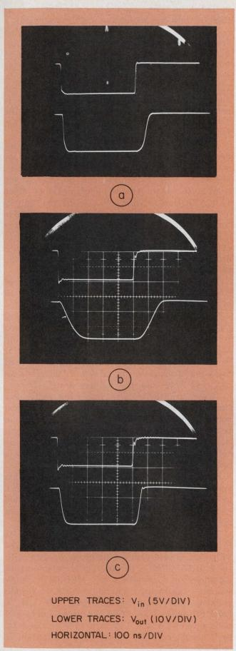
8. These scope photos show the actual performance of the circuits described in Fig. 7. The circuit of Fig. 7b cannot meet the 100-ns switching requirement of the design example because of high internal capacitance.
