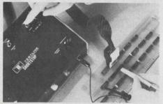
"Short-Stop" short-circuit locator uses near-field magnetic phenomena for fast, efficient PCB troubleshooting. LED readout positively locates short as probe passes over it. Easy to use; operators qualify in 15 minutes! \$495 in single units, lower in quantities. "Short-Stop II" (\$675 single unit) can also be used to exercise and control ICs and for on-board data bus diagnostics. Testling Instruments data bus diagnostics. Testline Instruments, 1625 White Drive, Titusville, Fl. 32780.
