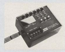
The unit can be plugged directly into any of the company's  $\mu$ P-card systems. The analyzer can be adapted to other 8080 systems by attaching the proper  $\mu$ P signals to its input circuits. The analyzer costs \$650. Delivery is 2 to 4 wks.
