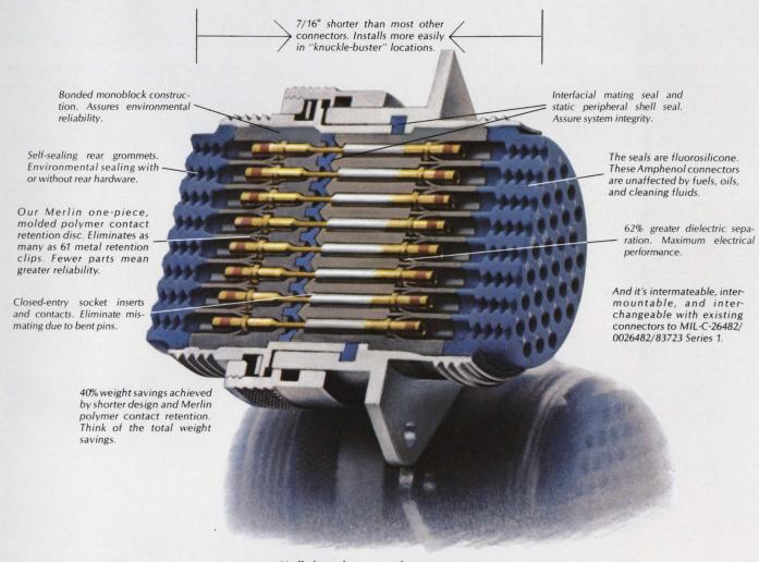
Merlin is a polymer retention system you can connect and forget. It's the guts of our 118 Series Connectors. They're competitively priced products, too. Ask for a quotation. Most sizes and styles are available, off-the-shelf, from your Amphenol Industrial Distributor. Or call or write: Wayne Zimmerman, Connector Division, Bunker Ramo Corporation, 2801 South 25th Avenue, Broadview, Illinois 60153. Phone: (312) 345-9000.
