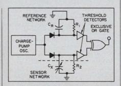
At the "zero" setting of the capacitor sensor, the RC constants and discharge times of both networks are equal, and no output appears. At the maximum sensor capacity the difference in the discharge times, and in the output-pulse width, are a maximum.
