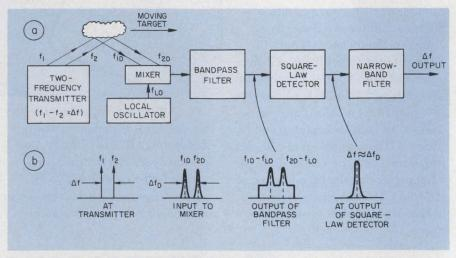
1. This three-frequency heterodyne system for radar provides an output of  $\Delta f$  that is not dependent on the Doppler shift of the transmitted signals. The power-spectral-density of transmit and return signals is shown (bottom).
