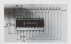
voltage levels, all the required circuitry is included in the UAA-180, thus eliminating the additional drive circuits usually required.
