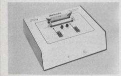
DIGITAL IC TESTER Fully automatic for DTL. TTL and CMOSno programming required—no switcheseasy to use for incoming inspection in the engineering lab., etc. Will quickly pay
