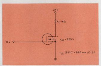
6. A typical ON condition for a MOSFET switch, starting at a room ambient of 25 C produces an initial  $V_{\rm DS}$  of 3.35 V. As the FET warms up, the  $V_{\rm DS}$  increases.
