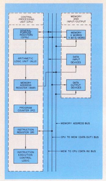
3. The internal structure of a  $\mu$ P—its architecture—resembles that of a conventional computer. Three busses are generally needed to provide communication among the  $\mu$ P, memory and I/O devices.
