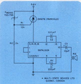
A two-tone fire-alarm warbler is turned on when a solid-state temperature sensor fires an SCR.
