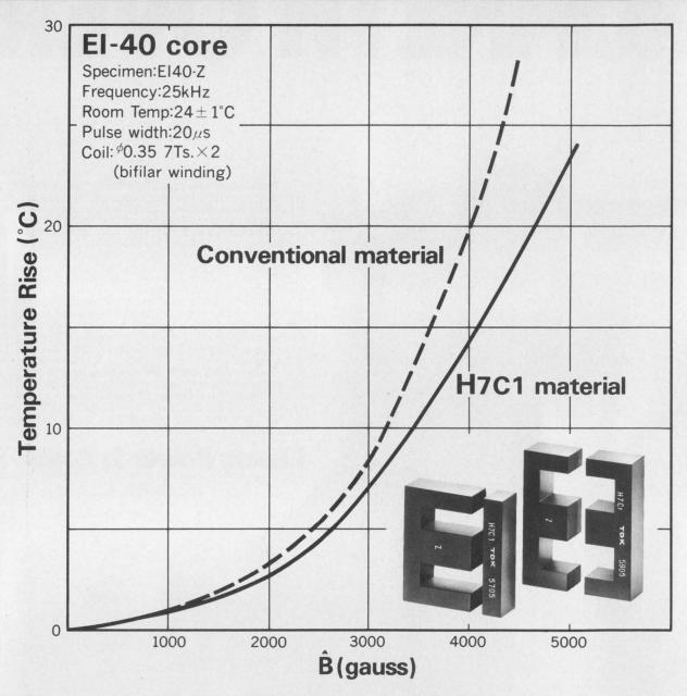
TDK has come up with a new high power ferrite core material. We list it as H7C1 and, as you can see from the graph, its temperature rise compared with conventional material puts it way out in front. TDK ferrite cores with H7C1 material bring compact, low heat generating power supplies as close as your drawing board.
