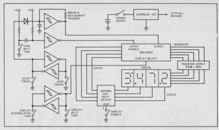
The Display Select debouncer/latch enables the contents of either the counter or the internal latch to the on-chip display drivers, which lets you read either accumulated time or split time (pulsing the Latch Enable line allows the taking of split time).
