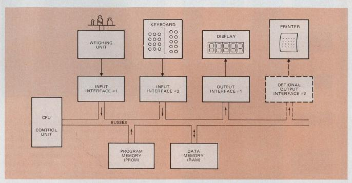
2. A simple microcomputer application—an automated scale—can be built with a single  $\mu P$  that communicates
