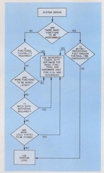
1. The choice between microprocessors and random logic depends on a series of tradeoffs that are illustrated in this flow diagram.
