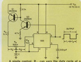
A single control,  $R_{\rm p}$ , can vary the duty cycle of a timer from 1 to 99% without affecting its period.
