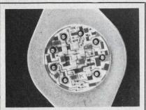
MSK MODEL 150. High Voltage—High Current Operation Amplifiers. 1 Amp Output Current. ±20 Volt Output. Full Mil Temperature Range. Short Circuit Protected. TO-3 Package. Designed specificially for Synchro Applications. 100 pc. price \$58.00 ea. M.S. KENNEDY CORP. Syracuse, N.Y. (315) 455-7077
