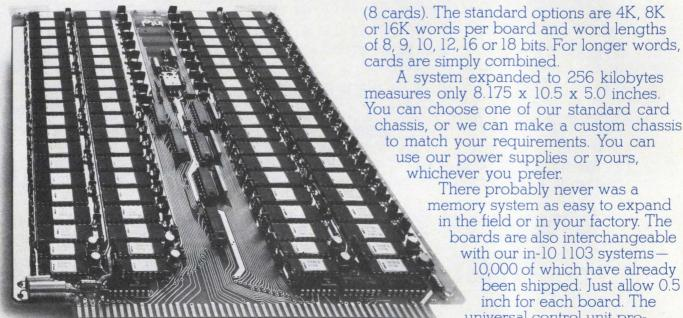
cards are simply combined. A system expanded to 256 kilobytes measures only 8.175 x 10.5 x 5.0 inches. You can choose one of our standard card chassis, or we can make a custom chassis to match your requirements. You can
