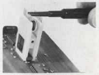
IC Test Clips: New Lower Prices. Eleven models of A P Test Clips provide full access to standard and LSI DIP leads . . . solve probe attachment problems . . . remove DIP's damagefree. Typical reduced prices: TC-14: \$5.25 TC-16: \$5.75. TC-24: \$13.85. Gold-plated contacts. Free catalog. A P Products Inc. Box 110-D, Painesville, OH 44077.
