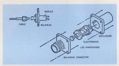
Fiber-optic connectors that use standard electrical connector shells are being used by the Navy to replace conventional wires with fiber optics.
