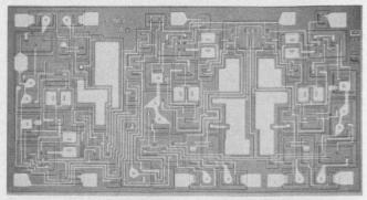
A new dual op amp designed for single-supply operation, Signetics' NE532, uses a Darlington input stage that can be driven slightly below ground (-0.3 V).
