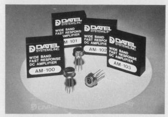
Wideband, fast settling FET op amps, by Datel, have bandwidths from 7 to 45 MHz and slewing rates from 60 V/ $\mu$ s to 400 V/ $\mu$ s. Settling times range from 300 ns to 2.5  $\mu$ s.
