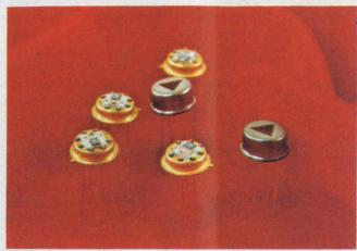
High accuracy op amps with FET inputs, the Analog Devices AD506, have a maximum offset of 0.1 mV,  $10\mu$ V/°C maximum drift and 5-pA maximum bias current.
