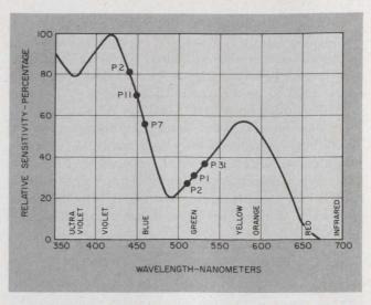
5. Relative sensitivity vs phosphor type for Polaroid 410 film. Note the difference in sensitivities for P11 at 450 nm and P31 at 530 nm.
