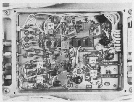
A 3  $\times$  4-in. module contains a complete quadriphase demodulator, including the "IQ" loop, which provides carrier reconstruction. The compact unit employs 1-GHz bipolar-logic ICs developed by Motorola.
