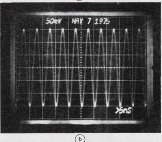
3. Film speed makes the difference in the production of clear photographs. With 3000 ASA film, a trace is just discernible (a). The same trace appears boldly when photographed with film of 10,000 ASA rating (b).
