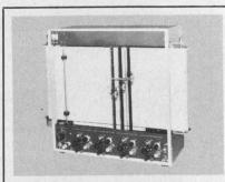
D-73BP Three pen X-Y<sub>1</sub>, Y<sub>2</sub>, Y<sub>3</sub> T Recorder features single X-axis common to 3 electrically independent Y axes. Use as a 3-channel recorder for accurate time correlation and greatly extended duration. Sensitivity: 2, 5, 10, 50, 100, 500mV, 1, 5, 10, 50 100V/full scale. Riken Denshi Co. Ltd. 5-5-2, Yutenji, Meguro-ku, Tokyo, Japan. tel (03) 711-6656.
