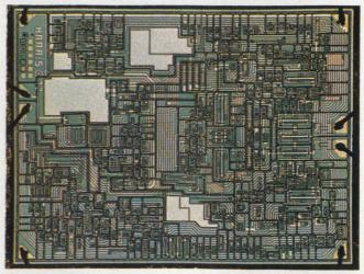
This monolithic chopper-stabilized amplifier, by Harris, has an offset voltage drift of only 0.2  $\mu$ V/°C. Open loop gain is 5  $\times$  10 $^{\rm s}$ , bandwidth is 3 MHz and slew rate is 2.5 V/ $\mu$ s.
