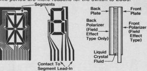
Flexibility of design permits LCDs to be scaled up or down to meet product needs. For example, Hamlin makes a display used in a ladies watch that measures only .450" x .575" (11.25 x 41.375 mm), but production facilities permitting, a display could be almost any size. Type of artwork used for creating the display design also provides an inexpensive way to customize with a logo, product illustration, etc.
