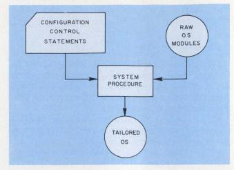
2. To start work with a supermini, the user must do a SYSGEN—in which selected operating system modules are joined to support the particular application.
