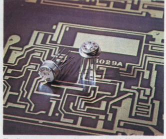
The first op amp to combine bipolar and CMOS on one chip, the RCA 3130, has a CMOS pair that is capable of swinging the output voltage to within 10 mV of either supply terminal.
