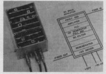
An experimental 50 Mb/s repeater developed by Bell Laboratories can be used to regenerate optical data.
