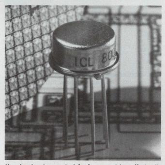
Very low input current of 1 pA max and low offset voltage of 2 mV max are features in this 8007 FET-input op amp by Intersil. Input impedance is 1012 ohms.
