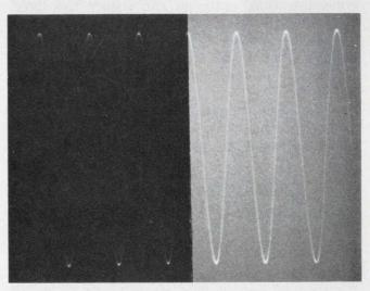
4. Two shots made under identical conditions show the effects of film fogging, that is, pre-exposure of the film. The left trace is hardly legible but appears clear and sharp after the film is fogged (right).
