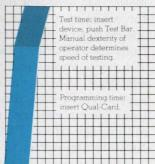
Test. The Qualifier 901 is ready for test and the device is inserted into the test head socket. The "Test Bar" is depressed and the device is tested in 60 to 200 milliseconds.
