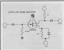
Ultra Low Noise Fet None quieter—  $2nV/\sqrt{Hz}$  at 1 kHz—our 2N6550 siliconN-Channel junction FET gives highest  $G_M$  available, improved  $A_V$ , high  $I_{DSS}$  within a 10-250mA range and low output impedance. "Data in short transistor catalog." Samples. Prices: 100-999, \$10. Teledyne Crystalonics, 147 Sherman St., Cambridge, MA 02140. (617) 491-1670
