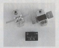
Over 500 W at 4.6 GHz in a p-i-n diode is tough to achieve. Motorola's wide gold lead is the key.
