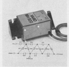
Photo shows typical tripler with focus tap
