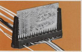
Models available for surface or through-thepanel mounting, with or without card guides and keys.
