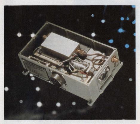
Temperature stabilization of this Micromega paramp system would normally require a 30-lb heat chamber. With thermal pads,  $\pm 1.8$  F stabilization is achieved in a 42 oz. package.
