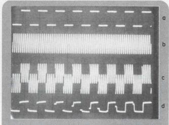
2. A 4-V $_{\rm pp}$ , 14-Hz square wave (a) is recovered from a superimposed 6.5-V $_{\rm pp}$ , 143-Hz sine-wave ripple signal, (b and c) with 40-dB suppression of the ripple and little deterioration of the square-wave rise time (d).
