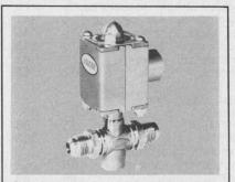
Cryogenic Solenoid Valves. New all stainless steel construction. Unique design provides high flow, long life and extreme reliability at temperatures down to -423°F. All joints heliarc welded. Metal to metal seating. Coil suitable for 50,000 hours of operation. Valcor Engineering Corp., 5382 Carnegie Ave., Kenilworth, N.J. 07033 (201) 245-1665.
