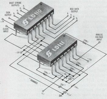
The unique conversion technique uses a single reference and a single full-scale adjustment to achieve a highly-accurate strobed 3½-digit output of up to 3100 counts plus sign. LD111 analog processor employs monolithic PMOS/bipolar construction and interfaces directly with the LD110 digital processor, which has a monolithic PMOS structure. For further information
