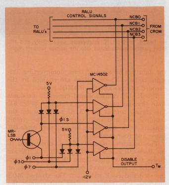
The control-signal generator produces pseudo microinstructions that will execute the required add and shift operations in the RALU.
