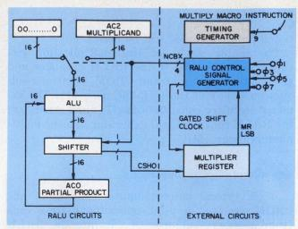
2. The complementary circuit provides alternative control signals, labeled NCBX, for the RALU. The technique can be used with the IMP-16C because it is a microprogrammable processor.
