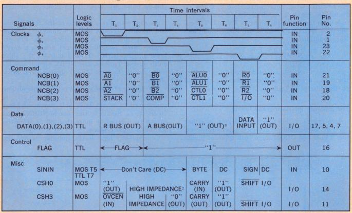
Note 1. A positive true logic convention is used for all signals—"1" = more positive voltage, "0" = more negative voltage. Signal names beginning with N are complementd signals.
