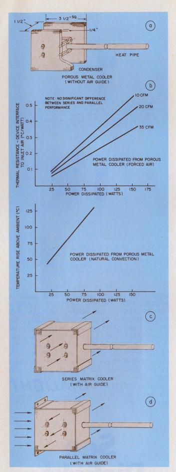
7. A high-performance condenser configuration for a heat pipe (a). There is no performance difference (b) between series (c) and parallel (d) air-flow patterns.
