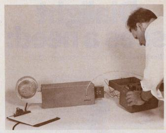
8. Test duct for transpiration coolers provides controlled, filtered air flow to allow measurement of component temperatures with a thermocouple. The blower housing contains a washable air filter.
