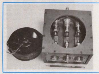
3. In this three-phase, full-wave power-rectifier assembly, six power diodes are mounted on panels that provide low thermal resistance to the cooling air. A half-wave unit would need only three diodes and a single panel.
