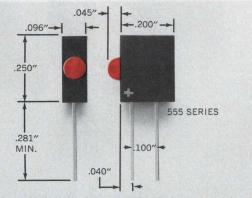
LED logic state fault indicators available in 14 models with voltage ratings from 1.7 to 14. Suitable for dense packaging on printed circuit boards—up to 10 units to the inch—IC compatible. With built-in series resistor. Polarity identified. Low power consumption.
