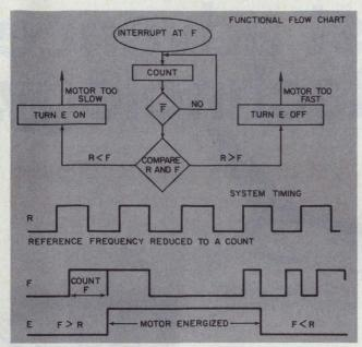
5. If the only concern is motor speed, an internally computed reference can be compared with the tachometer period. The operation resembles that of the PLL circuit in an out-of-lock condition.
