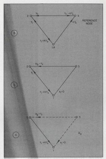
These transformations provide the graphic solutions. Node 3 is selected as the reference, and arrowheads directed to node 3 are removed. The single remaining branch and coefficients provide the circuit determinants.
