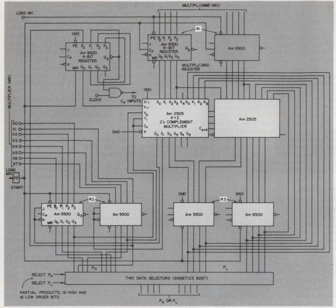
6. Two 4 × 2-bit IC multipliers sequentially add the 8-bit parallel multiplicand into the partial product regis-
