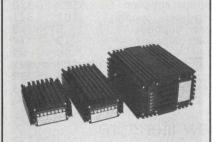
Logic and Linear DC Supplies available with single and multiple outputs ranging from 5V to 28V and currents to 25A. Line reg. is 0.05%, load reg. 0.1%. Features Internal OVP (STD on 5V), current fold-back, floating outputs. 220VAC input optional. 16 models in stock. Modular Power Inc., 4818 Ronson Ct. San Diego, CA 92111 (714) 279-1641
