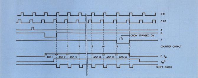
3. The 16-clock  $T_{\rm M}$  period is generated when the multiplication op code is detected. FF2 provides an inverted
