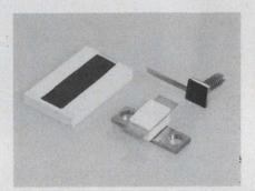
Conduction-cooled microwave resistors and terminations handle up to 100 W. These devices are from Pyrofilm on beryllia substrates.
