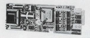
The SN Digital Interface Card accepts your data input on parallel lines, strobed for noise immunity, and stores the data in a buffer register. For isolation, the program is transferred across optical couplers so that your digital signal and the power supply it controls can be up to 1000V apart. The five types of SN Cards offer a choice of BCD or complementary binary programming.
