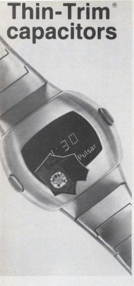
Tucked in the corner of this Pulsar Watch is a miniature capacitor which is used to trim the crystal. This Thin-Trim capacitor is one of our 9410 series, has an adjustment range of 7 to 45 pf., and is .200" x .200" x .050" thick. The Thin-Trim concept provides a variable device to replace fixed tuning techniques and cut-and-try methods of adjustment. Thin-Trim capacitors are available in a variety of lead configurations making them very easy to mount.
