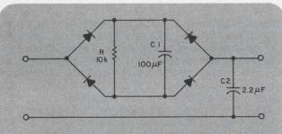
1. A low-pass filter for recovering signals from high levels of ripple voltages uses only seven low-cost components.
