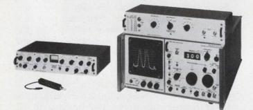
**Communications signal analysis** is the forte of this unit, the Nelson-Ross CSA-290. The 43-MHz analyzer can handle inputs to 400 MHz with a range extender.
