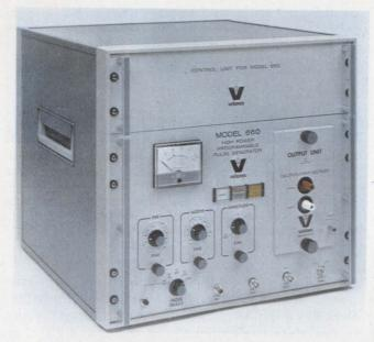
**High-power pulse generators deliver 31 kW** per pulse with amplitudes to 2500 V and 20-ns rise time. These units find use in EMI tests, magnetic component tests and laser pulsing. The Velonex Model 660 features BCD-programmable width, prf and amplitude.
