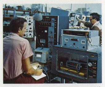
The DMM-42 from California Instruments is a  $4 \cdot 1/2$ digit programmable digital multimeter. It is BCD-programmable with a high degree of isolation between the unit's analog and digital sections.
