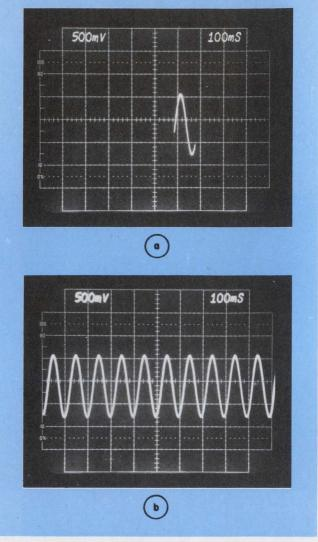
3. **Phosphors in nonstorage** CROs show only part of a slow trace (a). By contrast, a storage oscilloscope gives the complete picture (b).
