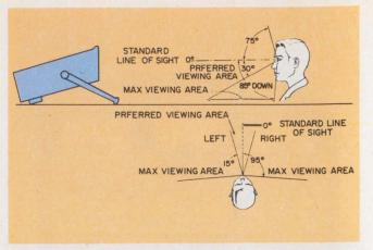
The ability to adjust the viewing angle of an instrument for comfortable use is of primary importance. Human engineering provides the preferred range of angles that most people can accommodate to.
