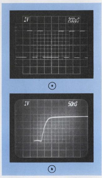
1. With storage, you can study nonrepetitive waveforms, such as digital words (a). With fast-transfer storage, rise times are easily measured (b).
