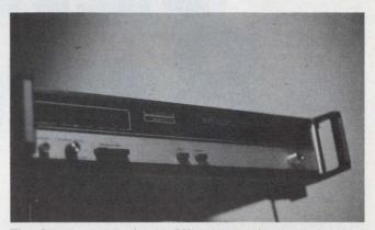
The latest automatic 18-GHz counter costs less than \$4000. Standard minimum sensitivities are -20 dBm at 12 GHz and -15 dBm at 18 GHz. The unit, from EIP (Santa Clara, CA) also has a 40-MHz, pk-pk, FM tolerance to 10-MHz modulation.
