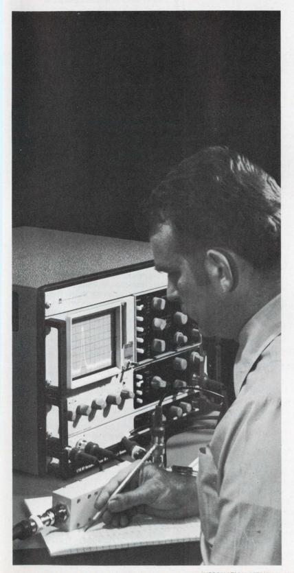
400 kHz to 500 MHz with 115-dB dynamic range and 0.005-dB resolution — these are not design goals of an idealized analyzer, they are performance facts of hundreds of instruments now in the field.
