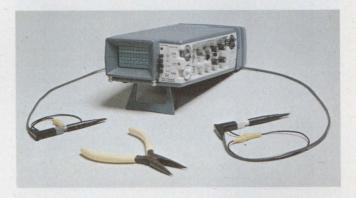
storage CRO gives the user a chance to inspect the signal visually and, in many cases, to make quantitative measurements of the signal's characteristics. Other people can be called in to give advice or inspect the waveform, and permanent photographic records can be made if necessary.
