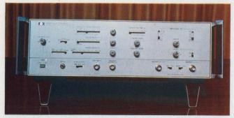
**Color these pulse generators flexible.** The HP Model 8082A (left) provides variable transition times down to 1 ns. The 250-MHz generator also provides adjustment of pulse delay, width and two output levels. Similar parameters are controllable either remotely or by thumbwheel switches on the Model 1501A from E-H.
