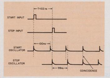
2. Two startable oscillators, one for START and one for STOP, give high-resolution, single-shot measurements.
