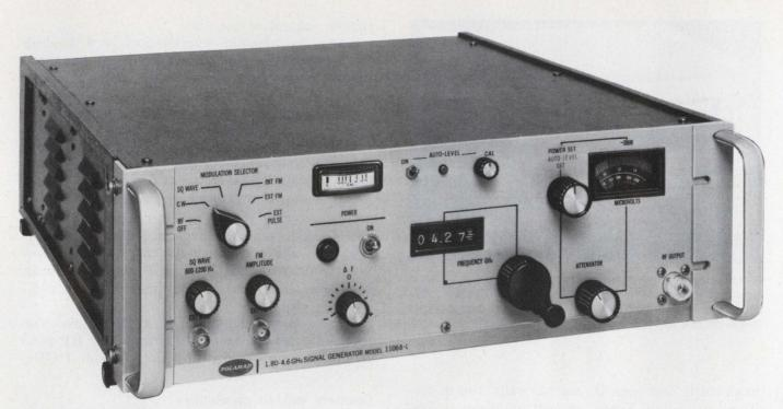
More than 10-dBm output and a calibrated range of +6 to -130 dBm can be obtained from the 1106B-L signal
