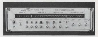
A simulator for radar range provides a target pulse at a precise time after a trigger pulse. The output pulse is controlled to simulate target velocity and range. Model PX 219 provides use times under 5  $\mu$ s for a 400- $\mu$ s target pulse. The PX 219 from Phenix Electronics can be programmed remotely.
