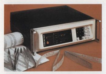
The only non-HP instruments that are ASCII-programmable and compatible with the proposed IEC interface standard are a series of waveform generators from Wavetek. This model, the 159, works to 3 MHz and can also be controlled by a keyboard on the front of the instrument.
