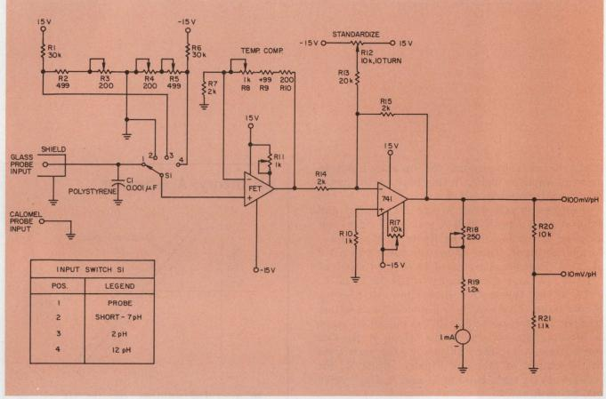
2. Just two op amp stages are needed to design an accurate pH meter. The first stage, a FET, provides high input impedance to prevent loading of the probe; while
