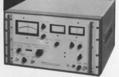
The PRD 915-B Attenuation Calibrator has long been in a class by itself. It measures up to 110 dB in a single step, and achieves an accuracy of ±0.03 dB/10 dB with only —80 dBm input power. It's *the* lab/production line instrument for attenuator calibration, extreme VSWR measurements, noise measurements, and sensitive detection in reflectometers, plasma diagnostics, etc.
