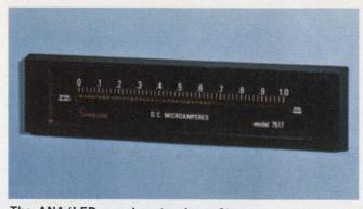
The ANA/LED panel meter from Simpson combines the advantages of both analog and digital meters. It has no moving parts but can show trends.
