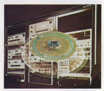
Macrodata's MD-500 is a large-scaTe, general-purpose LSI test system. It is controlled by an Interdata 70 minicomputer and contains primarily test instruments designed in-house at Macrodata.
