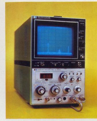
That analyzers are getting easier to use is demonstrated by Hewlett-Packard's 8558B. Just three controls are needed to make practically all measurements.
