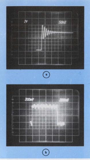
2. Single-shot, stored traces capture difficult signals such as switch bounce (a) and elusive amplifier ringing (b). Storage shows all details.
