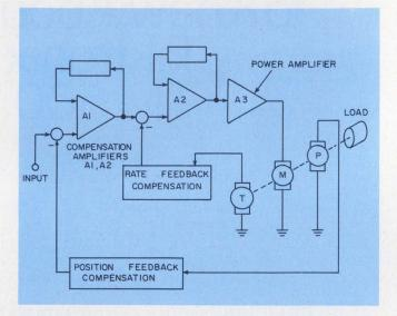
1. **Typical position servo** has two feedback loops: one to carry back the load position and the other to adjust the servo damping. When the main loop is broken at any point, one of the servo amplifiers usually saturates, which makes measurements impossible.
