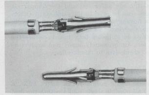
cover the full range of wire sizes. Number 24 to 16 AWG and .040" to .130" insulation diameter. They also feature serrated wire barrels to break up surface oxides and a stepped insulation barrel to keep the conductors in perfect alignment with the contacts.
