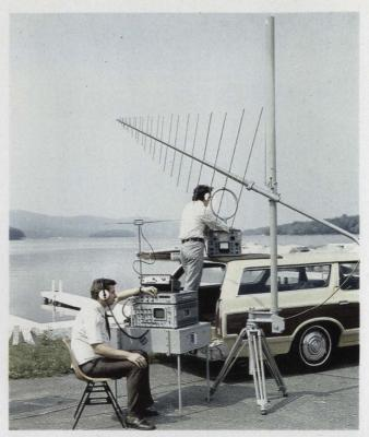
**Battery operation for field use** is another trend in spectrum analyzers. Though it can be used outdoors, Rohde & Schwarz's Analyskop gives laboratory performance.
