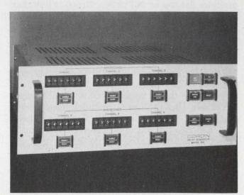
**Time-delay generators** provide delayed triggers calibrated to nanosecond increments. The Model 438 from Cordin (right) provides delay from 0 to 999.999  $\mu$ s with outputs to 40 V into 50  $\Omega$ . Model 7030 (left), part of Berkeley Nucleonics modular system, offers 1-ns increments to 100  $\mu$ s. These devices are often used in the operation of Image Converter Laser Diagnostic Cameras and flash X-ray analysis.
