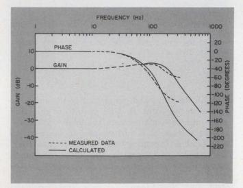
7. **Closed-loop response of the torque tester** also shows a close correlation between the experimental and theoretical data over most of the frequency range.
