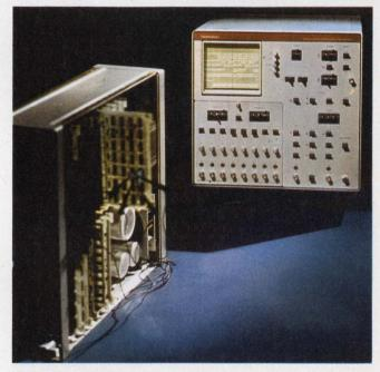
**High speed logic can be analyzed** with the 8200 logic analyzer from Biomation. It can accept 8 channels of data at a rate of 200 megabits/s.
