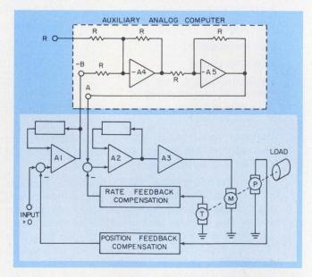
2. To measure open-loop (and closed-loop) response with the loop closed, a break is made at the summing junction between amplifiers  $A_1$  and  $A_2$ , and an auxiliary computing chain is inserted at the break. With zero reference signal, the servo-loop gain remains unchanged.
