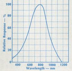
Standard Vactec phototransistors provide very high sensitivity and good blue response. Liberal design flexibility is also offered with trade-off for some characteristics, including: light current; response time; spectral sensitivity; and breakdown voltage. Selection of packages are TO-18, co-axial, pill, non-hermetic TO-18 size and special arrays on 50-mil or 25-mil centers.
