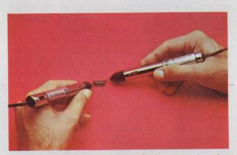
A hand-held pulser and logic probe locate stuck nodes quickly. The Model HL-583 stimulator (left) operates at 5 Hz or in a one-shot mode. The unit can supply up to 1 A for 1  $\mu$ s with CMOS or TTL amplitude levels and takes its power from the circuit under test. The resultant logic state is shown in the probe (Model LP-575). Both units are from Kurz-Kasch, Dayton, OH.
