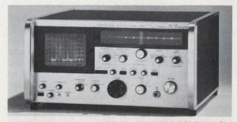
Analyzers from Texscan fall in the remarkably low price range of \$2500 to \$4500. The units use a unique marker system to identify frequencies to within 0.005%.
