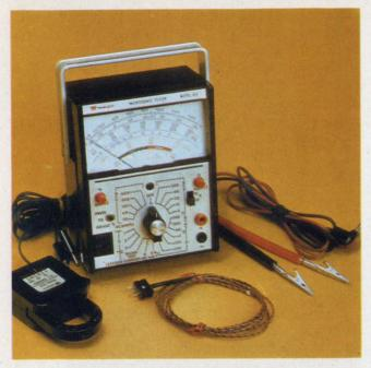
The Triplett Model 615 is a 20,000 ohms-per-volt multitester with a -50 to +1500 F thermocouple thermometer. Accuracy is  $\pm 3\%$  of full scale.
