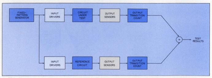
2. With the pattern-generator approach to testing, the ATE counts ONE-to-ZERO and ZERO-to-ONE transitions,
