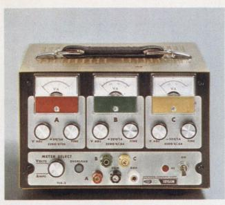
**Color coding** ties the power supplies and output terminals in Trygon's TL8-3 triple-output power supply.
