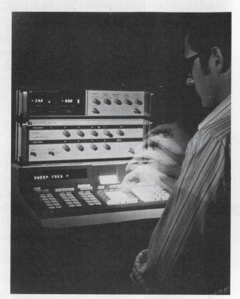
1. Systems using calculators can take data from a variety of instruments, process the data and output the results to an assortment of peripherals.
