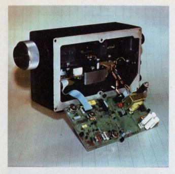
**Infrared thermometer** from E<sup>2</sup> Thermodot of Carpenteria, CA, measures temperature by optically sensing the intensity of radiant energy emitted by a warm surface.
