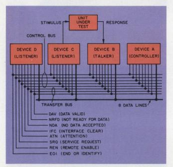
**Hewlett-Packard's Interface Bus** is being considered by the IEC for use as an international interface standard for automatic test systems. Up to 15 devices can be attached to the bus asynchronously with data rates of up to 1 Mbyte/s.
