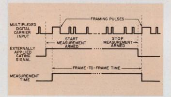
3. With external gating, measurements can be made despite the presence of data on the digital carrier input.
