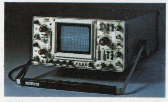
The fastest storage scope around is the 466 from Tektronix. It has a writing speed of 1350 cm/ $\mu$ s and a viewing time of from 15 s to 6 minutes.
