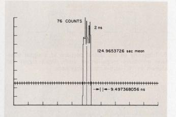
4. **Histogram of frame-to-frame jitter** obtained in real time, with use of a programmable calculator as the data-reduction element.
