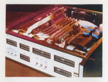
cycle are interdependent. And these tradeoffs become apparent at high speeds. The first tradeoff is usually amplitude for rise time and rep rate. For example, it's almost impossible to get 16-V pulses at rep rates above 50 MHz. But you can expect 5-V amplitudes with 20-ns rise times at rates from 100 to 250 MHz, and 2 V from 500 MHz to 1 GHz—all into 50  $\Omega$  loads.
