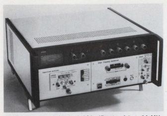
With a dynamic range of 120 dB, the Adret 11-MHz 6303 holds the title for this spec. With a substitution of plug-ins, the unit becomes a synthesizer.
