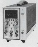
**Delay By Events Trigger** Select and display any data segment in a disc, drum, or tape memory. Examine serial data transfers. Study serial transmission. Jitter-free, delayed oscilloscope triggers for all of these appli-
