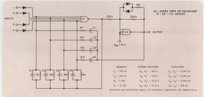
A sine-wave oscillator can be built with linearly biased CMOS gates and a Wien-bridge network.
