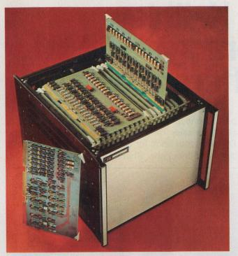
The E-H 1604 word generator generates simultaneous pulses for up to 48 pins (at rates to 20 MHz) and compares the measured output with expected levels stored in its own memory. Each pin can provide 512 bits. And all the parameters on this device are programmable.
