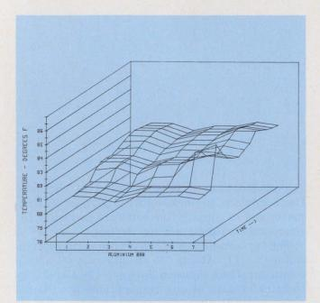
3. The temperature profile of an aluminum bar is displayed at the output of an HP data-acquisition system. The time scale represents 10 seconds between plots.
