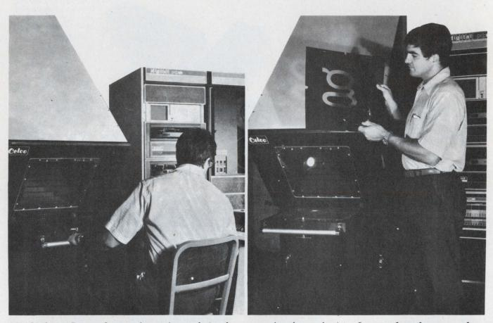
CELCO's Large-Format Scanner is a unique solution for automating the production of master fonts for a manufacturer of computer typesetting equipment. Scanning a 16-million point area, this system calibrates itself and reduces an artwork master 14 inches x 14 inches to a digital record in 16 seconds.
