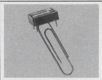
New low profile low cost TTL DIP Crystal Oscillator measures only 0.3" high x 0.49" w x 0.78" L; plugs into single IC socket; available at any fixed frequency from 4 MHz to 20 MHz, with frequency tolerance  $\pm.01\%$  from  $-25^{\circ}$ C to  $+75^{\circ}$ C; fanout 10 TTL. Supply 5 Vdc  $\pm5\%$ . Connor-Winfield Corp., West Chicago, III. 60185 (312) 231-5270. INFORMATION RETRIEVAL NUMBER 615
