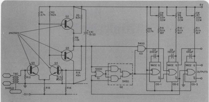
The timing of this slave clock circuit is controlled by RC time constants. The component values shown are for 1.5-MHz operation. Capacitor scaling can change the frequency range.
