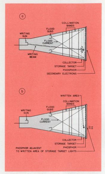
7. With variable persistence, the writing beam charges the target positively at the points of contact (a). Floodgun electrons pass through the written areas to light corresponding screen points (b).
