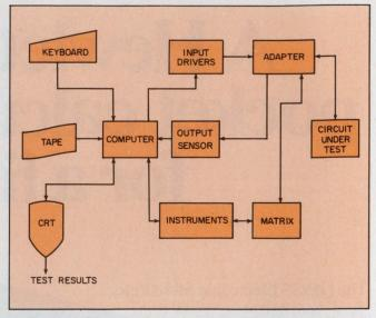
4. For functional testing, the most versatile—and most expensive—configuration uses diagnostic software.
