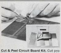
Cut & Peel Circuit Board Kit. Cut prototype boards or ground planes. Assortment of 7 includes one and two sided Cut & Peel Boards on .100" grid drilled and plain epoxy-glass, "X" and "X-Y" Board, a plug-in Cut & Peel GP Board with etched gold/ nickel edge connector, and a special knife. Kit #8964 is \$37.00. Circuit-Stik, Inc. Box 3396, Torr., CA 90510. INFORMATION RETRIEVAL NUMBER 601
