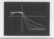
The 1090 offers numerical readout of any selected data point. Selection is made with an easily moved cursor. Wherever the vertical cursor intercepts the waveform the alphanumeric readout on the CRT displays time from trigger and voltage recorded at that point in time. Both values are calculated by the 1090 so that the CRT alphanumerics are in actual time and voltage. (You don't have to multiply a number times a switch setting.)
