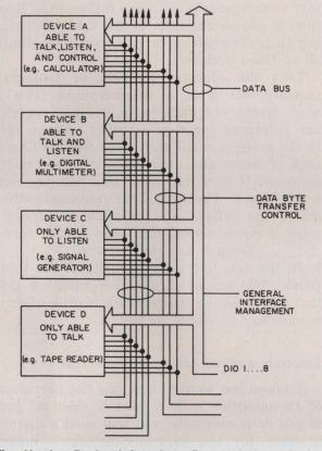
2. The Hewlett-Packard Interface Bus includes 16 signal lines to convey addresses, commands and data to the various interconnected devices.
