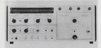
With a plug-in, the 7.9-to-18.5-GHz countermeasures band can be swept in the Model 610C Sweeper Series from Wiltron (Palo Alto, CA). Leveled output is 5 mW.
