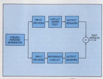
1. A fixed-program, comparator-type ATE compares the circuit under test with a reference circuit.
