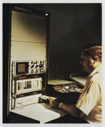
The first system to use the HP Interface Bus is the 3042A network analyzer from Hewlett-Packard. This system is a calculator-controlled frequency synthesizer and network analyzer for measuring amplitude and phase from 50 Hz to 13 MHz.
