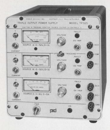
and without need to turn a switch. The patented circuit uses multiple-output unregulated supplies connected via a series of OR gates to a group of series-pass regulators—the regulator used is determined by the load requirement. Thus you have at your fingertips a power supply that retains the same efficiency at 10 V as it does at 60 V. And you don't sacrifice anything in doing this—regulation is a comfortable 0.01% +1 mV. And the cost is only \$229 for the four-in-one supply.
