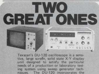
unit designed to satisfy the particular needs of a production or laboratory testing system using sweep generator techniques. The DU-120 incorporates the latest circuitry, including regulation of the high voltage source and a dual packaged FET input. The VS-60 sweep generator is a completely solid state, low distortion, wide sweep instrument covering the frequency range 5 MHz to 1000 MHz with many optional features available from stock.
