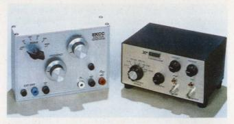
A two-chip monolithic waveform generator is incorporated in the prototype instrument by Exar, at right. A singlechip device is used in the other instrument, produced in kit form by Electronic Kits and Components.
