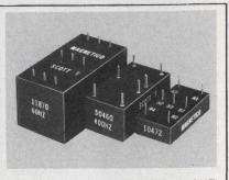
Scott T Transformer. 11870: 60HZ, 90v, L-L in. 1.1x2.1x1.1. 50460: 400HZ, 90v, L-L in. 7/8x1-5/8 x11/16. 50642: 400HZ, 11.8v, L-L in. 7/8x1-5/8-11/16. 10472: 400-HZ, 11.8v, L-L in. 3/4x1-1/2x3/8. All with 6v RMS sine & cosine output. MAGNETICO, INC., 182 Morris Ave, Holtsville, N.Y. 11742 516-654-1166.
