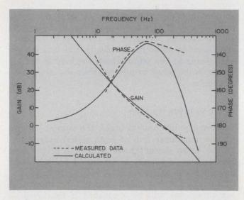
6. **Open-loop response of the bearing-torque tester:** Measured gain and phase agree closely with the calculated data for the frequencies of interest.
