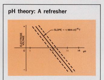
In a neutral solution—one that is neither acidic nor basic—the pH is 7.0 at 25 C. This decreases for acidic solutions and increases for basic solutions. Each unit change in pH number represents a tenfold change in hydrogen-ion activity,  $a_{\rm H}$ , which is related to the concentration of hydrogen ions in a solution—specifically pH  $= -\log a_{\rm H}$ .
