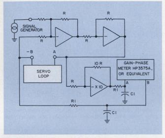
3. Two improvements make low-frequency measurements easier: noise blocking low-pass filters in series with the leads of the gain-phase meter, and a loop-gain booster amplifier that precedes the meter.
