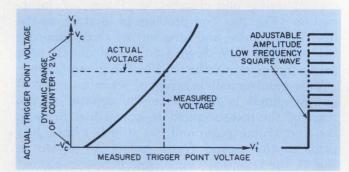
7. Determining settability error over the dynamic range of the counter input.
