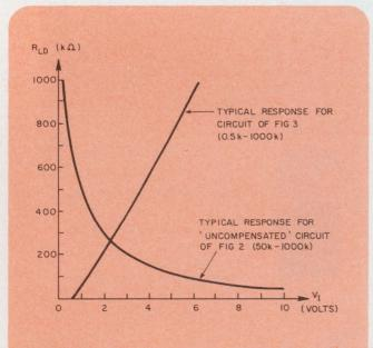
1. Light-dependent resistors are highly nonlinear, but a feedback circuit can linearize an LDR's response.
