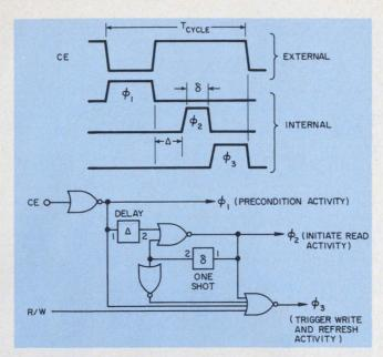
6. A timing generation scheme is needed for the operation sequence. Three sequential pulses— $\phi_1,\ \phi_2$  and  $\phi_3$ —are triggered by a single external clock (CE). The period of the CE signal defines the memory cycle. Delay  $\Delta = \phi_1 - \phi_2$  is required by the decoder circuit employed.
