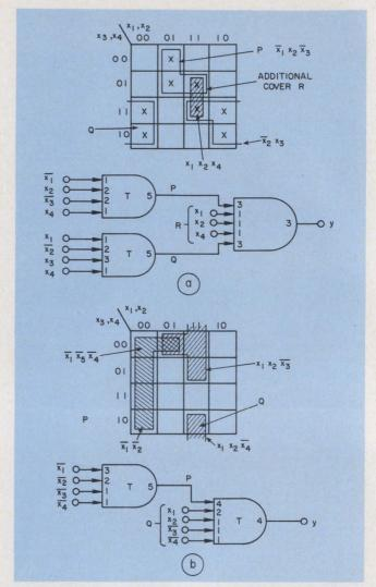
6. Standard map patterns help eliminate switching hazards in logic circuits.
