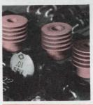
The Triac-Kooler is a low cost (only 17¢ each in quantity) heat dissipator that effectively levels excessive heat rise in triacs, affording greatly prolonged usefulness to the triac. A push-in rivet firmly assembles the Triac-Kooler to the base of the triac. The multiple finned area disperses the heat. The small size of the Triac-Kooler permits dense packaging. The attaching push-in rivet is supplied with each Triac-Kooler. Nothing else is næded. No tools, Send for your sample . . . try it.
