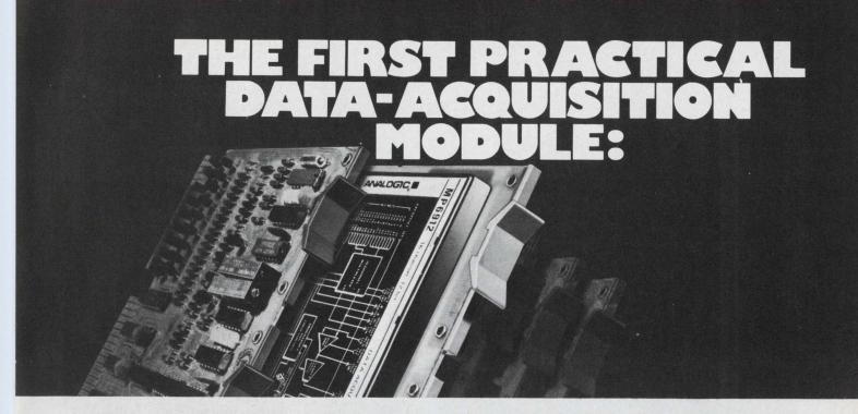
Complete 12-bit, 16-channel system fits 0.5" card spacing-anywhere. Better performance, at lower cost, than individual module combinations.
