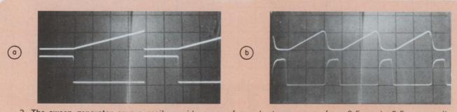
3. The sweep generator covers easily a wide range of speeds; traces range from 0.5 ms to 0.5  $\mu$ s per div
