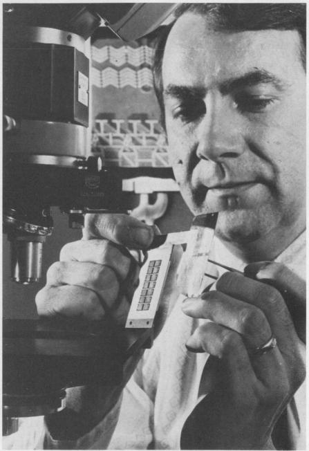
Magnetic bubble memory chips developed by Bell Laboratories have been fabricated into a 460,544 bit bubble memory module that has a data rate of 700,000 bits/sec and an average access time of 2.7 ms.
