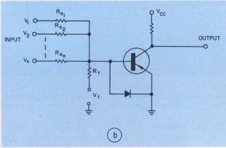
3. Though obsolete, the magnetic core type of threshold gate (a) is very versatile. It uses square-hysteresis-loop material in its core. A discrete-component threshold circuit (b) uses resistors to provide weighting for the input. It was designed originally for use in a computer to test threshold-logic theory and practice.
