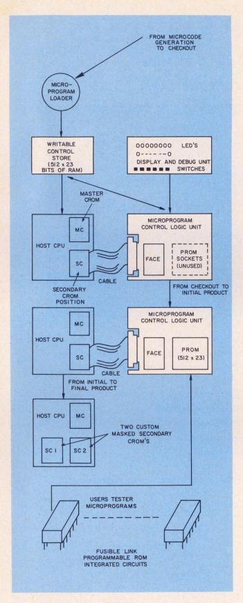
6. One development system for field microprogramming can be used in low-volume applications. The system employs a writable-control store, control-logic unit and display and debug unit. The FACE (field-alterable control element) chip in the control-logic unit constitutes the heart of the system. Functionally similar to a CROM, the FACE chip uses external memory for the microprogram store.
