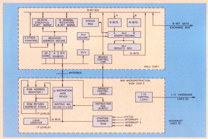
Another microprogrammable unit has been proposed by American Microsystems. Unlike the other units, this one employs an 8-bit slice, rather than 4 bits, and the control chip uses a ROM instead of a PLA.
