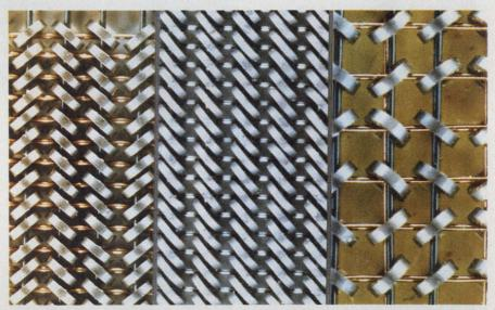
Obsolete core spacing used until 1970 (right) yielded 1678 cores per sq. in.; higher-density spacing introduced in 1970 gave 5276 cores per sq. in. (left). In 1973 density was upped to 6469 (middle).
