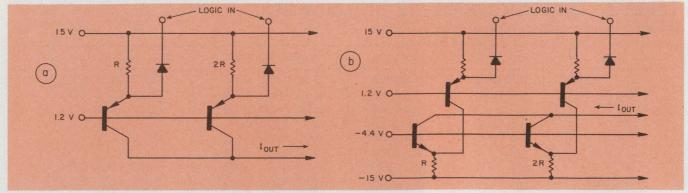
1. Weighted current-source configurations for straight binary (a) and complementary binary (b) coding gener-
