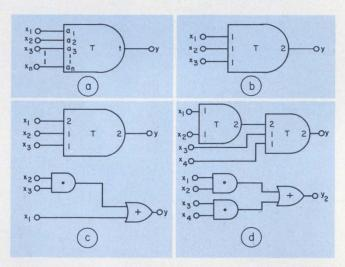
2. A generalized threshold gate can be symbolically represented (a). The three-input gate (b) performs majority logic, since it provides an output when any two out of the three inputs are ONEs. More complex gates (c and d) perform the functions depicted by the Boolean equivalent circuits shown directly under each T gate.
