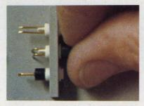
Easiest to use too. Just insert into 0.191" hole & press into position. Front panel relamping is also a cinch. No tools needed. Just remove snap-on cap. Remove lamp. Insert new one. Replace cap. Takes seconds.
