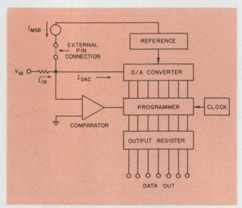
3. Most a/d converters for bipolar operation are offset by a current equal to the value of the MSB. The half-scale then becomes 100 . . . 0.
