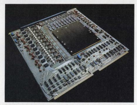
This 8-k core memory board is used in Data General's new Eclipse series of computers. It provides for correction of single-bit errors with five extra bits in the memory word and a modified Hamming code.
