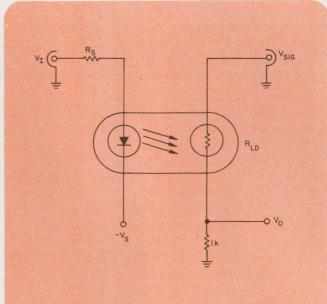
2. An uncompensated LDR circuit has a nonlinear response. The resistance of the unit, when  $V_1=0$ , can be determined by  $-V_s$ .
