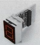
730 SERIES Your choice . . . a red or green LED readout with large 0.625" characters . . . low power, operates with standard IC power supply levels. Comes in plus-minus module. Display uses standard or high brightness LEDs for maximum light output arranged in a seven-segment format. Available with or without onboard decoder/driver. Unique lens design generates bright, highly legible characters.
