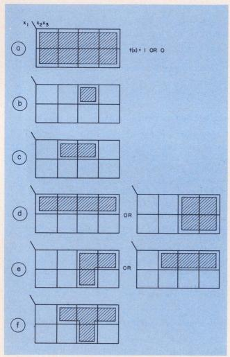
3. Each Karnaugh pattern defines a specific threshold-gate configuration for the n≤3 Chow parameters.
