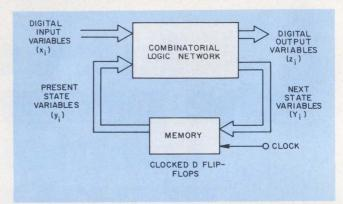
1. Sequential machines generate outputs that depend on the current state and input. Delay elements or clocked flip-flops constitute the memory.
