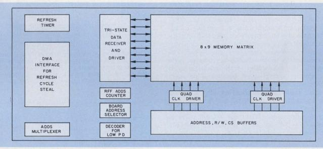
2. A 32-k-word × 9-bit memory board (photo) uses interchangeable 4-k RAMs from AMI and Motorola Semiconductor. The single board directly replaces four boards using 1-k dynamic (1103-type) RAMs. It is also a quar-
