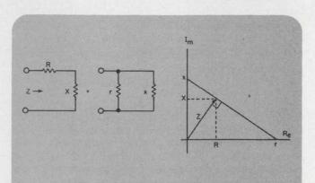
In the graphic or algebraic transformations the driving-point impedances for the series and parallel configurations are equal to each other.
