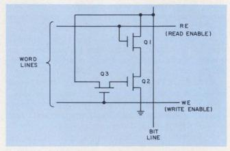
5. This three-transistor-per-bit cell forms the basis of the 6605 4-k RAM. On the chip, the present cell measures 3.4 mil<sup>2</sup> with a new cell design of 2.5 mil<sup>2</sup> expected to appear on the market in the near future.
