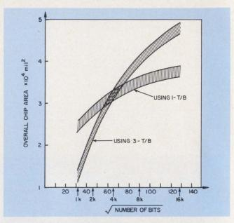
3. A smaller over-all chip size is generally a feature of RAMs using one-transistor-per-bit cells, compared with those using three transistors. But the opposite is true when storage densities begin to exceed 4 k, because of the requirements of internal peripheral circuitry.
