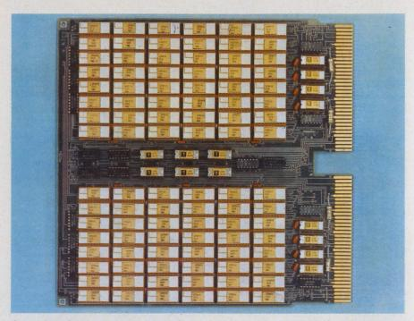
A semiconductor memory array board used in Honeywell's Series 64 main memory consists of 16,000 12-bit words of dynamic MOS RAM storage. Each of the chips contains 2048 bits of memory.
