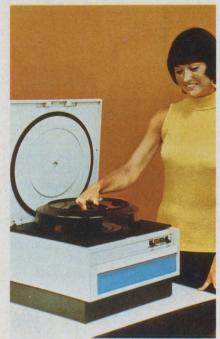
Calcomp's Trident disc drives provide from 25 to 80 Mbytes of storage, with bit densities running from 4040 to 6060 bpi and track densities of from 185 to 370 tpi.
