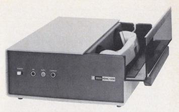
The acoustic coupler gives quick access to a line. Data rates up to 1200 baud are possible with the ADAC 1200 from Anderson Jacobson.
