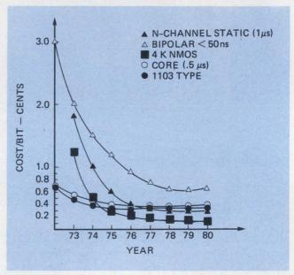
1. The low cost per bit of today's 4-k dynamic NMOS RAMs is expected to drop even further in the years ahead. Access times are also expected to drop.
