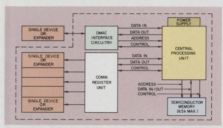
A unique architectural feature for minicomputers, a communication register unit, is provided for TI's 960B in process-control or manufacturing-control operations. This register is used instead of an I/O unit to permit bit-by-bit input and output in serial form.
