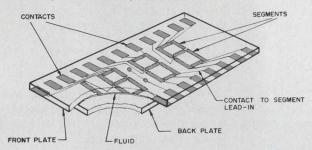
How they work. When the liquid is not electrically excited, its long cigar-shaped molecules are parallel to one another in a position perpendicular to the plates. The liquid appears transparent. When an electric current is applied, ion activity of the molecules leads to turbulence causing the liquid to scatter incident light. Depending on the type of nematic liquid used, either a dynamic scattering or field effect display results.
