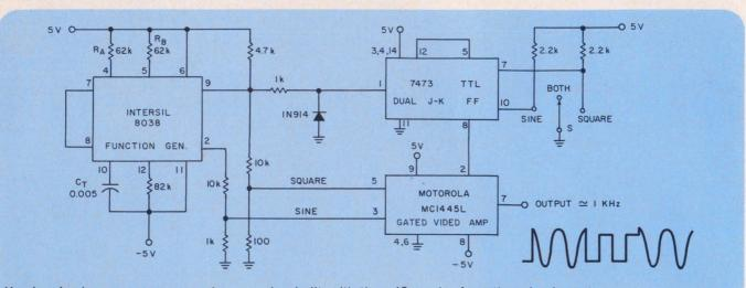
Handy sine/square-wave generator can be built with three ICs and a few other simple parts.
