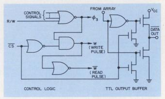
4. Operation modes are determined by the chip-select (CS) signal and the read-write (R/W) control signals in the 6605. Information readout is nondestructive and refresh of the entire memory occurs by a cycling of each of the 32 addresses every  $2 \, \text{ms}$ .
