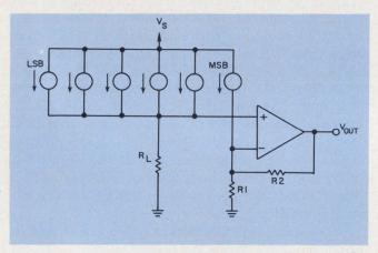
4. For two's complement coding in a d/a, the MSB current-source must go to the opposite terminal from the other weighted sources to avoid output glitches.
