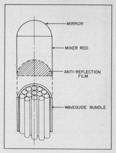
Low-loss star coupler for optical fibers permits two-way data communication on all fiber bundles.
