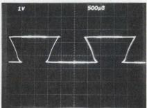
ing edge) of 500  $\mu$ s, a hesitation (trailing edge) of 500  $\mu$ s and a flare (wide top or bottom) of 2 ms.
