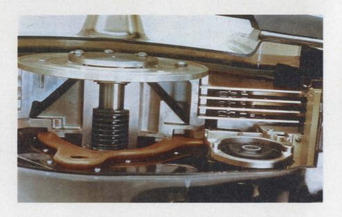
Incorporating the head-positioning system and the recording medium in the same module makes the IBM 3340 disc drive unique. Data density on the Winchester is 5636 bpi, and average access time is 25 ms.
