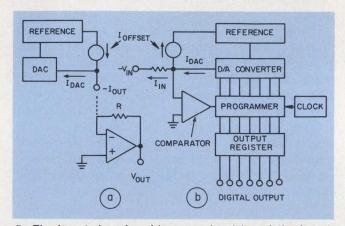
5. The inverted-analog d/a converter (a) and the inverted-analog a/d converter (b) have negative-going analog output and input values, respectively.
