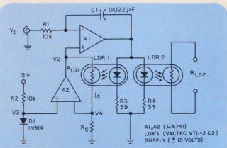
3. A reference light-dependent resistor, LDR $_1$ , in a feedback circuit, linearizes the response of LDR $_2$  to the input voltage  $V_1$ .
