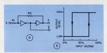
3. Two inverters and two resistors form a Schmitt trigger (a). The hysteresis loop (b) has distinct switching points at the 50% limits.
