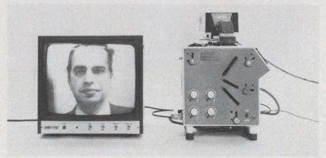
Rapid photo composition of a suspect's picture in a TV monitor is possible with the GBC Video Identification System.
