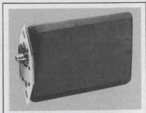
"VLF to HF ACTIVE AIRBORNE ANTENNA provides highly efficient reception for Omega, Loran C and Communication applications. Operating frequency is 10 KHz to 30 MHz with a 50 ohm constant output impedance." BAYSHORE SYSTEMS, Springfield, Va.
