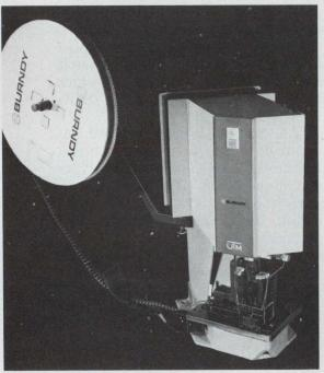
machines feature easy-to-set dial adjustments for wire size and insulation size.
