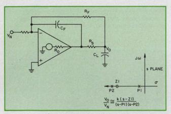
2. The addition of  $C_{\rm F},~R_{\rm S}$  and  $R_{\rm F}$  decouples the load and introduces a zero in the transfer function.
