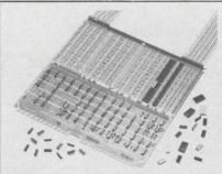
NOVA/DCC-116 general purpose interface board provides: multiple device selection, 4 I/O registers, DMA zero word count detect, 105 socket positions for 14, 16, 24 & 40 PIN IC's. Basic board (all features of data general 4040 plus multiple device select) \$350. MDB Systems, Inc., 981 N. Main St., Orange, CA. (714) 639-7238.
