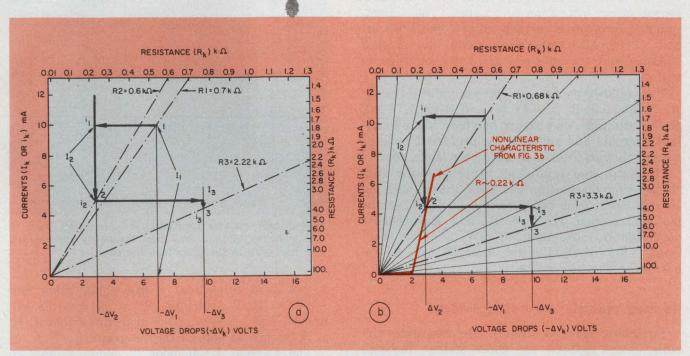
2. Both linear (a) and nonlinear (b) resistors can be handled with the graphical method.
