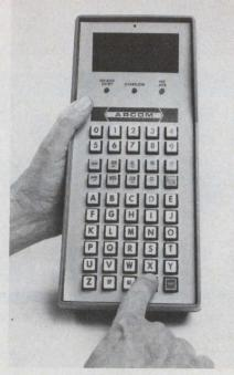
The smallest mobile terminal available is the MCT-16 from Atlantic Research. The unit features a full alphanumeric keyboard plus 10 special-function keys.
