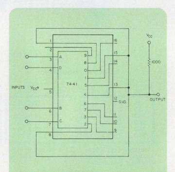
Four-input EXCLUSIVE-NOR gate logic is provided via inputs A, B, C, D. For a three-input gate, tie the D input LOW, unless you want to use the D input as an inhibit. With D as an inhibit, the decimal-eight output must be omitted from the output.
