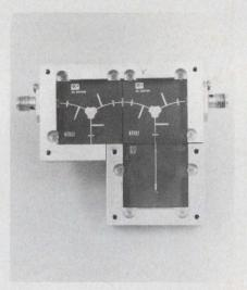
Wideband 200 to 400-MHz power amplifier modules from Collins Radio use beryllia substrates. Some newer modules are built on aluminum carrier plates.
