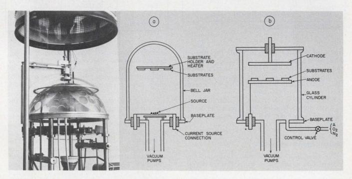
2. Either a planetary evaporation chamber (photo and a) or a sputtering system (b) are used to deposit thin-film
