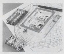
A 9.2 to 9.8 GHz parametric amplifier from AIL is fabricated on a YIG substrate. The pump oscillator is not shown in the photo.
