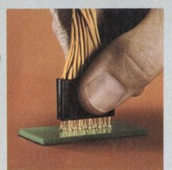
The Locking Clip Connector mates with .025² posts on a true grid. Receptacle contacts are tinover-nickel plated by a unique process which makes them approach the performance of gold. The connector is available in 4-, 10- and 20-position configurations and will accept #26 to #30 AWG wire. Contacts can be terminated by high-speed, automated machines for uniform reliability at low applied cost.
