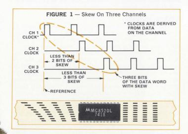
trated in Figure 1 which shows three channel clocks which are derived from the data on the respective channels. The skew is caused because the magnetic tape is not precisely parallel to the recording or read heads, either due to mechanical tolerances, or due to the fact that a tape may be written on one transport and read on another with a different alignment between tape and read head.
