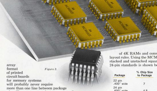
pins. Since some manufacturers presently run two leads between 100 mil center pins, one lead between 75 mil center pins should present little problem for conventional double sided boards. This approach gives a 4:1 density improvement over the industry standard 22-pin (.4 inch wide) dual in-line package and a 6:1 improvement over the 24-pin (.6 inch wide) package. Used with present 4K RAMs, the technique allows expansion into the next generation of larger (8K and 16K) NMOS dynamic RAMs.
