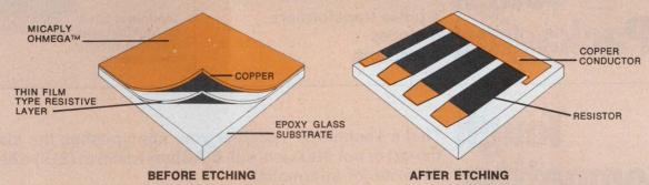
Micaply Ohmega<sup>TM</sup> can reduce costs and eliminate the need for discrete resistors. And it's available immediately.
