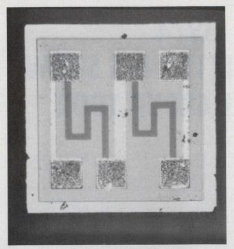
5. A center-tapped film resistor maintains a stable ratio over wide temperature ranges for a long time.
