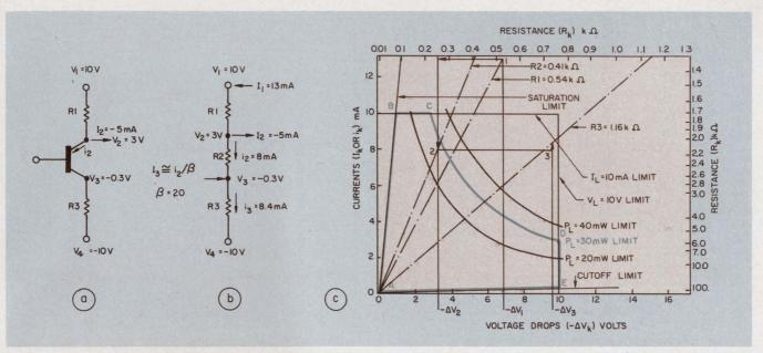
4. Voltage, current, resistance and power limits can be outlined on the voltage-divider graph as a guide.
