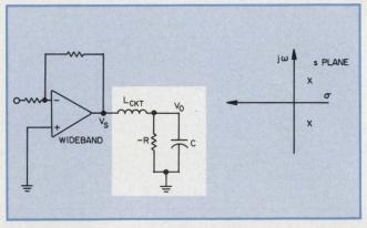
5. Active loads that exhibit negative resistances can also degrade an op amp's output.
