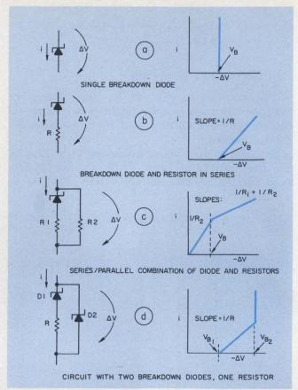
3. **Nonlinear resistor configurations** are often used in voltage-divider circuits and they are easily represented and dealt with in the graphical approach.
