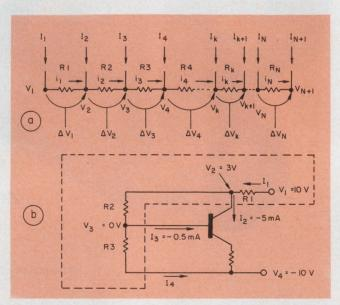
1. The generalized voltage divider circuit (a) and a three resistor divider as used for transistor biasing (b) follow the convention that currents,  $I_k$ , that flow into the divider are positive and voltage drops,  $\Delta V_k$ , across the resistors are negative.
