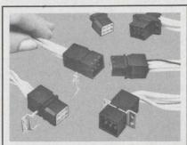
CAPITRON subminiature LGH highvoltage connectors. They're lightweight—a mated pair is less than 14 gr. And compact—requires less than .6 sq. in. of mounting surface. Operates up to 5 KVDC at 70,000 feet. And within a temperature range of -55°C to +125°C. AMP Incorporated, Capitron Division, Harrisburg, Pa. 17105. (717) 564-0100.
