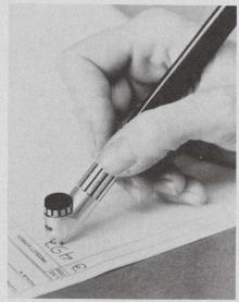
Computerized pen automatically translates hand-printed data into ASCII-coded data. The pen is designed to replace keyboard entry devices now used.
