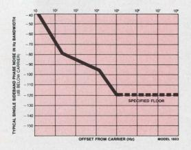
How do conventional synthesizers achieve microwave frequencies? By using multipliers. But that multiplies noise too. Systron-Donner's idea: eliminate multipliers, use **octave band** signal sources instead. Result: a family of frequency synthesizers with the highest spectral purity obtainable today. Industry response: enthusiastic. Request our new application note entitled "The Microwave Frequency Synthesizer: An Improved Standard for Microwave Research, Testing, and Applications."
