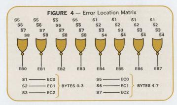
for example, if bit 5 was lost in storage, syndromes 1, 3, 5, 6 and 7 would go high. The pattern was further chosen so that the different columns of X's in the H matrix are different from each other in at least two rows. Therefore, a double error will not appear as a single, or no, error but will show up as an even number of syndromes high.
