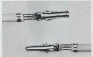
cover the full range of wire sizes. Number 24 to 16 AWG and .040" to .130" insulation diameter. They also feature serrated wire barrels to break up surface oxides and a stepped insulation barrel to keep the conductors in perfect alignment with the contacts.
