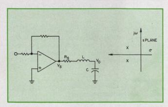
4. A small resistor,  $R_{\rm s},$  shifts the poles to the left of the  $j\omega\textsubscript{-}axis.$
