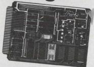
Our 4-bit microprocessor system can replace a rack full of your TTL chips. You'll save design time and production costs. No big redesign jobs for options or changes because the logic is stored in reprogrammable ROMs. Our programmed logic systems are available now, off the shelf.
