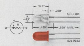
Available in red or clear LED packages with or without a built-in current limiting resistor. Red LED is also made without resistor. Suitable for circuit status indication, alpha-numeric displays and visual indicators. Features long wire-wrappable leads. IC compatible with solid state reliability. High luminous intensity, low power consumption, low cost.
