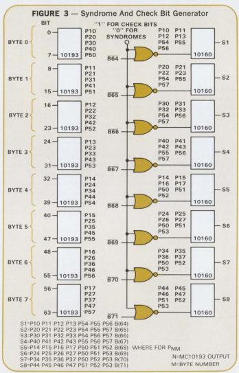
would be generated and compared with the old check bits. The comparison forms eight syndrome bits ( $S_1$  through  $S_8$ ) which can be decoded to show the type and location of any error. The syndrome bits are physically generated by the odd parity of data bits *and* old check bits in the appropriate column.
