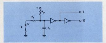
2. Two inverters, a capacitor and two resistors form an integrator that can minimize switch bounce.
