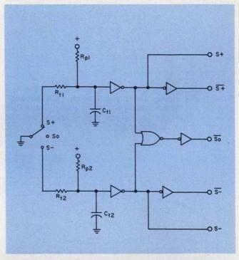
4. A three-position switch-bounce eliminator can be built with a few inverters and a NOR gate. This circuit can be expanded to cover a wide number of switch types.
