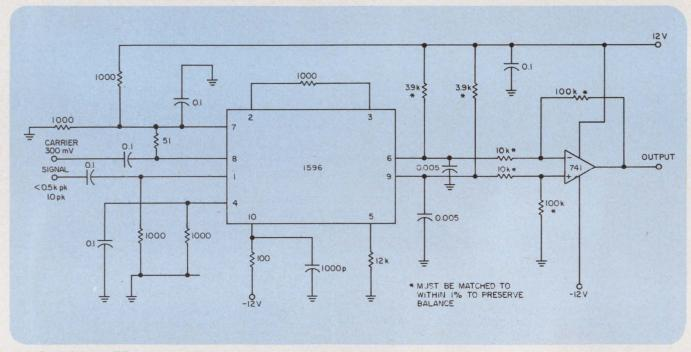
A differential amplifier can couple a balanced output from a doubly balanced mixer.
