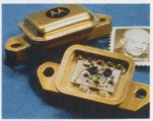
A wide-band, low-noise cable television amplifier, the Motorola MHW 526, produces 16 dB of gain from 40 to 300 MHz. Input and output impedance is 75  $\Omega$ .
