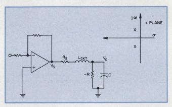
6. However, oscillations can be damped by the addition of resistor  $\ensuremath{\mathsf{R}}_s.$
