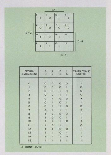
3. You must convert the truth table to a modified Karnaugh map. The numbers in each box represent the decimal equivalent of the minterm (1 = full weight, 0 = no weight). The horizontal and vertical lines indicate the columns (rows) for which the associated variable is ONE. The 1,0 and d entries are the same as stated in the truth table below the map.
