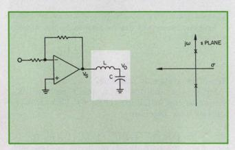
3. Reactive loads produce undamped oscillations.
