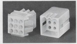
mis-mating. Low profile mounting ears make Hylok® fast and easy to install, and resilient take-up springs hold the housing securely over a wide range of panel thicknesses. Hylok® housings are available in 2,3,4,6,9,12 and 15 positions to cover virtually every application.
