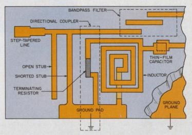
The basic current element in most MICs is the microstrip transmission line. A conductive strip is fabricated on one side of a flat dielectric substrate and a ground plane on the back side. Most of the rf energy is propagated along the line in the TEM mode, and the electric field is confined to the dielectric directly below the strip conductor.
