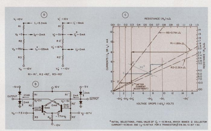
5. To design a divider for a two-state circuit, such as a flip-flop, can be a tedious trial-and-error job. However,
