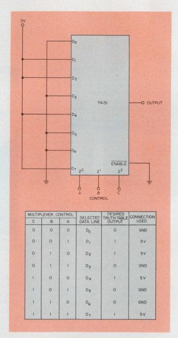
1. A digital multiplexer can generate arbitrary logic functions. In this case, the output is the odd-parity function of variables A, B and C. The inputs  $D_0$  to  $D_7$  are wired HIGH or LOW to correspond to the truth table. This simple technique lets you handle a number of variables equal to the number of control inputs of the multiplexer (in this case, the 74151).
