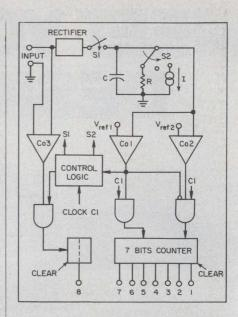
rapidly. After the opening of switch  $S_1$ , switch  $S_2$  closes in synchronism with the clock pulse. Each clock pulse increments the counter (initially reset to 0) by 16, as long as the decaying capacitor voltage is greater than the reference voltage of 32 V. When the capacitor voltage drops below 32 V, the comparator Co 1 changes state, which prevents further counting by 16.
