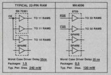
Fewer signal lines and signal drivers required. Compared with 22-pin packages, the MK4096 requires six less address lines to be driven throughout the memory matrix. In addition to making PC layout easier, this means fewer address drivers are required.
