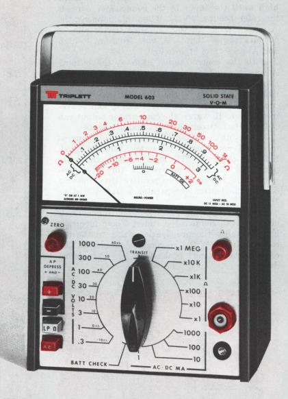
Model 603 also has a unique, Patented Auto-Polarity circuit: push a button, measure either plus or minus voltages without switching leads. Make very fast voltage checks where polarity is known or doesn't matter.
