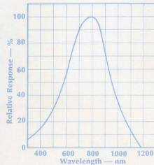
Standard Vactec phototransistors provide very high sensitivity and good blue response. Liberal design flexibility is also offered with trade-off for some characteristics, including: light current; response time; spectral sensitivity; and breakdown voltage. Selection of packages are TO-18, co-axial, pill, non-hermetic TO-18 size and special arrays on 50-mil or 25-mil centers.
