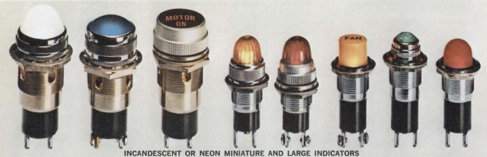
Designed to accommodate either incandescent (2-250V) or neon (105-250V) lamps for panel mounting in 11/16" or 1" clearance holes. Units meet or exceed MIL-L-3661 requirements; all are listed in Underwriter's Recognized Components Index. Wide selection of lens shapes, colors,
