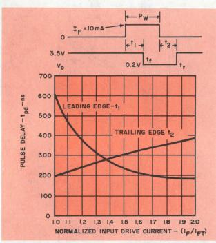
5. The opto-isolator's output delay can be different for the output signal's leading and trailing edges.
