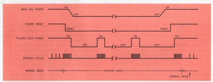
2. Control of the transition between the memory's standby and normal operating modes is via a power-reset signal furnished by the main system supply. During the standby mode, refresh cycles are performed in bursts;
