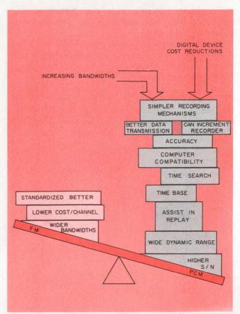
3. **PCM** has more to offer than FM recording when frequencies are low, as this comparison shows.
