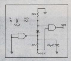
across the diode is about 6 pF. With a bias current of 8 mA, the predicted diode switching time is 0.35 ns. With a 0.5-ns-duration pulse, the circuit operates satisfactorily down to 0.5 V, at which point the switching becomes erratic. The addition of inductance between the diode and the gate input can improve the switching speed by removal of the shunt-capacitance effect of the logic gate.
