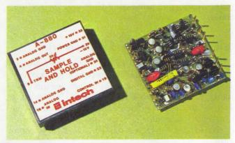
The A-880 sample-and-hold circuit, by Intech, provides a sample acquisition time of  $1.4-\mu s$  and a voltage droop of only 1 mV/ms.
