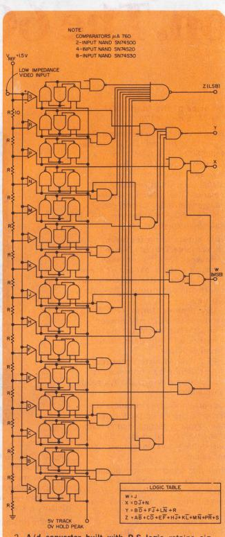
2. A/d converter built with R-S logic retains signal peaks when the control line is ZERO. The R-S logic remembers the high states that occur. The circuit follows the input when the control line is ONE.
