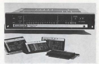
The Analogic 5800 data-conversion system can combine both a/d and d/a converters, sample-and-hold circuits and multiplexers to handle up to 64 channels of data.
