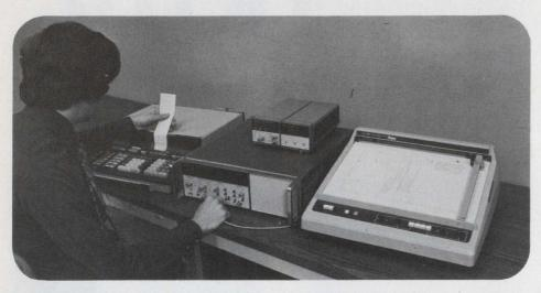
The HP 5345A counter's unmatched capabilities in time interval measurements and automatic systems operation pay off in applications such as the time interval jitter measuring system shown above.
