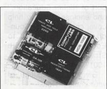
The new Computer Labs RDA Series D/A's eliminate harmonic distortion and produce clean "glitchless" pictures for reconstructed TV or other video signals. Input word rate for all models is 15 MHz with accuracies to  $\pm 0.05\%$ . Min. settling time to either 8-bit or 10-bit accuracies. Computer Labs, 1109 S. Chapman St., Greensboro, N.C. 27403.
