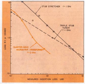
1. A quarter-wave microstrip transformer offers less insertion loss than other approaches when an impedance of 3  $\Omega$  or less is matched to 50  $\Omega$ .
