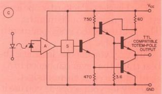
1. Opto-isolator logic couplers (a) can have an open-collector, current-sinking output (b) or a TTL-compatible, totem-pole output (c).
