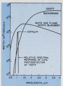
The narrow spectral response of cadmium telluride at 0.975  $\mu$ m makes it suitable for detecting flames against a hot, broad-band infrared background radiation.
