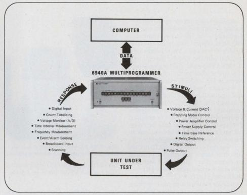
Multiprogrammer mainframes and plug-in cards let you design and build low-cost automatic test systems more efficiently.
