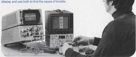
Twelve-bit parallel pattern recognition capability enables the 1601L logic state analyzer to trigger on a particular logic pattern. The unique trigger signal, available as a front panel output, is an extremely powerful tool in digital circuit analysis. By applying this trigger signal to an oscilloscope, the scope's display is positioned in the same "time window" as the digital event.
