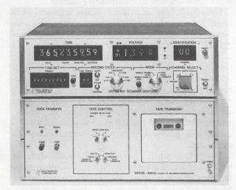
A multichannel data-acquisition system is formed when the Datos 306 cassette recorder-player and Datos 901 scanner-digitizer are combined. The equipment is from Data Graphics Corp.
