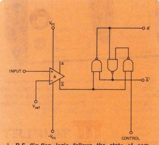
1. R-S flip-flop logic follows the state of comparator A if the control line is ONE. The logic circuit will latch on the high state of A when the control line is ZERO.
