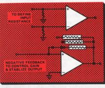
Victoreen MINI-MOX resistors are used widely to modify op-amp characteristics to: 1. Stabilize output and eliminate oscillation. 2. Define gain so measurements can be quantified. 3. Restrict bandwidth to the region of specific interest.
