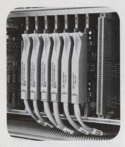
Each multiplexer input circuit provides high common mode rejection from transients and noise. Drift is eliminated by an offset sampling amplifier which further improves accuracy.
