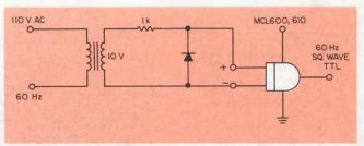
7. Conversion of sine waves to square waves makes use of the opto-isolator's Schmitt-trigger circuit.
