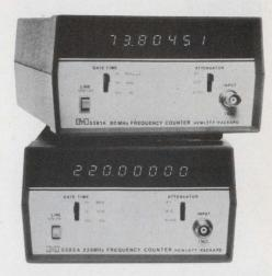
These new counters have 25 mV sensitivity, LED displays, measure ratio as well as frequency, and weigh just 4.75 lbs. (2.2 kg).
