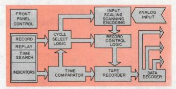
5. Control and operating sections of a recorder work together to acquire and scale data for analysis.
