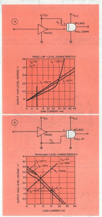
3. The input current to the opto-isolator can be derived from a TTL element and controlled by a resistor,  $R_{\rm L}$ , in either a pull-down or pull-up configuration.
