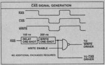
Address multiplexing is accomplished easily. Multiplexing of addresses is common to all memory systems using dynamic RAMs due to the refreshing requirement. 22-pin 4K RAMs require a 6-bit refresh address as does the MK4096. The only additional requirement with the MK4096 is that the address be multiplexed in two 6-bit bytes, accomplished with a multiplexer that is 3-wide instead of 2-wide and a multiplexer control that is 2-bits wide instead of 1-bit wide.
