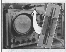
A typical application involves microwave device research. A gallium arsenide sample is firmly supported by the SERVOMETER bellows spring contact without undue compressive loads which would shatter this delicate material.
