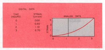
1. A typical strain-vs-time measurement can be represented either by a computer's numerical output or a plot of the analog data on a graph.
