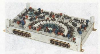
Radial arrangement of components in the Computer Labs Model 7110 a/d converter keeps propagation delays constant between all the converter signal paths. This unit converts 10 bits at 10 MHz.
