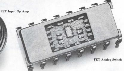
All standard Siliconix FET chips are equivalent to their JEDEC or house-numbered parents on all testable parameters. We have hundreds of JEDEC and house-numbered parts in our product line. To specify a JEDEC-equivalent chip simply add the suffix "CHP," as in 2N4416 (JEDEC registration) = 2N4416CHP (chip form). When
