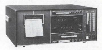
Time, channel number and parameter value are displayed on the front panel of the Digitec Model 1266 data logger. It has a built-in system clock and manual switches to control the scan rate and the scan mode.
