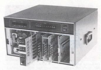
The modularized construction of the Monitor Labs Model-9400 data-acquisition system can be seen in this front view. CMOS circuitry keeps the power dissipation low.
