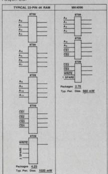
Only standard TTL required for chip select decode logic. Using MOSTEK's MK4096, two-level decode logic for
