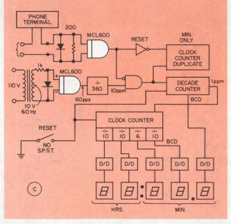
8. The isolation of the optocoupler is needed in phoneline circuits to detect the off-hook condition (a), the ringing signal (b) or to build a phone timekeeper (c).
