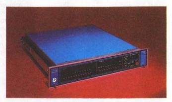
Plug-in circuit cards (left) are used in the Datel-256 data-acquisition system to perform all signal-conversion and sampling functions. This system can be expanded up to 256 channels due to its structure. Some of the front-panel options are shown above, including channel-select and manual controls.
