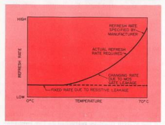
4. To further decrease battery drain, the refresh cycles are spaced in accordance with the memory temperature. Charge leakage decreases with temperature, but most manufacturers only guarantee the value at 70 C; so be sure to choose a conservative model.
