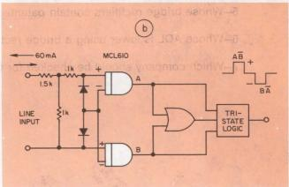
11. Opto-isolator circuits can function as polar transmitter relays (a) and polar receiver relays (b).
