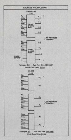
Result? The MK4096 scores highest in density, lowest in power dissipation and requires no additional packages in the memory controller.
