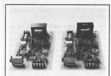
AC-line data transceiver modules wire directly to 120V AC, transmit & receive FM data via carrier-current signals on power line. Can be used with  $45\Omega$  speaker for high-quality voice communication or in telemetry applications. Stock to 4 wks., \$109/pr (1-100). Electronics Research Group, Arlington, Mass. (617) 646-9760.
