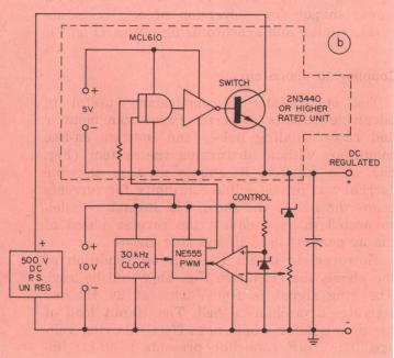
opto-isolator can provide. The isolator can couple a high-voltage level to a low-level control circuit.
