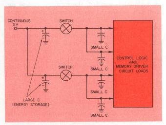
3. The switched power is subdivided near the loads to avoid voltage drops from the high peak currents drawn by bypass capacitors (with TTL logic) and MOS input capacitance. Simple transistor switches suffice for control of the dc power.
