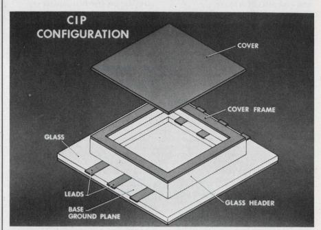
Circuit connections to the Bendix microwave IC packages are made by means of striplines. No coax connectors are used. The Controlled Impedance Package is mounted on a special mother board prepared for this system.
