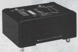
Model 9744 can be ranged to accept AC input from 100mV through 700V. It converts the input to a 1-volt DC output signal for the full-scale RMS value of the AC signal. Will also scale AC current input from 1uA to 1mA. Operates on either 115V or 230V,50-60 Hz line.
