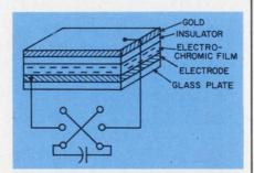
The electrochromic display is a solid-state passive display. When the lower electrode is negative, the electrochromic film turns deep blue. Reversing the polarity makes it clear again.
