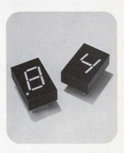
Standard 0.3 in. (0.66 cm) dual-in-line package permits easy mounting on PC boards or in standard IC sockets.
