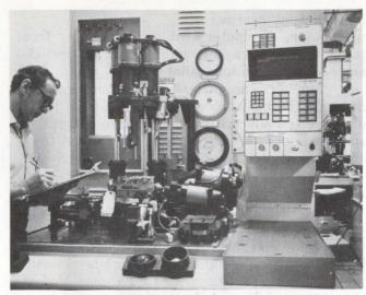
A carburetor test stand, made by General Automation, controlled by a computer-based data-acquisition system, not only tests the units but also keeps track of all the test data.
