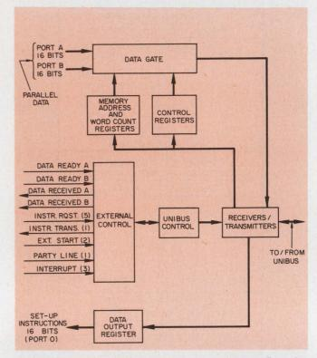
8. The computer buffer interfaces the bus with the telemetry devices and acts as the controller for the telemetry equipment. The control and memory registers establish the alternating memory buffers for entering the data blocks. Use of the buffer also ensures that the continuous telemetry data do not lock the CPU out of the computer bus. This block diagram is a simplified schematic of the EMR 2763 buffered data channel, which interfaces with the PDP-11 computers.
