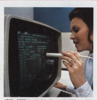
IBM's 3270 terminal is the most widely used intelligent terminal in the field. It is intended for data-entry systems with up to 32 terminals in a cluster to an IBM host computer.
