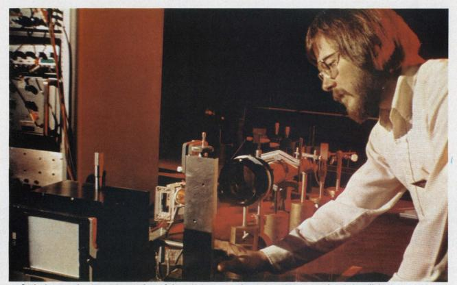
**Optical memories** like this one from Sperry Univac are being designed to store up to  $10^{\circ}$  bits of in-
