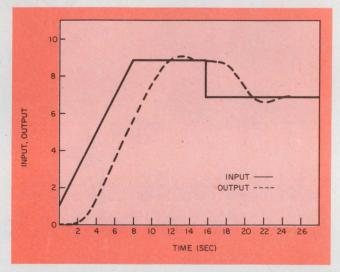
1. **Exact responses of linear systems** to commonly used waveforms are computed in segments and combined. The forcing function, in this example, is inputted as a sequence of unit-step, positive-ramp, negative-ramp and negative-step waveforms.
