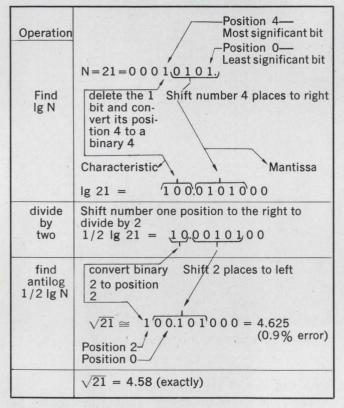
the characteristic to the mantissa, the least-significant bit of the characteristic,  $A_0$ , is wired into the most-significant bit of the mantissa (see Table 4), which becomes  $I_0$  of the 8243-B. Note that  $A_0$  is kept in its inverted form to correspond to the other inverted bits of the logarithm.
