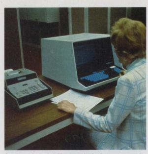
Sanders 810 intelligent terminal has a 12-in. cathode-ray tube with 1920 characters. It can support up to eight "dumb" terminals with its processor, and it sells for \$6900.
