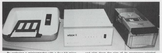
By replacing a minicomputer with a four-bit microprocessor, Data Type Corp. was able to cut costs
