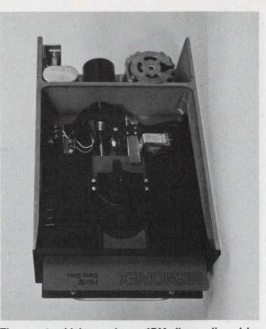
The most widely used non-IBM floppy-disc drive is the Memorex 651. More than 3000 of these are in the field. The drive uses a disc with a thicker coating, for longer life.
