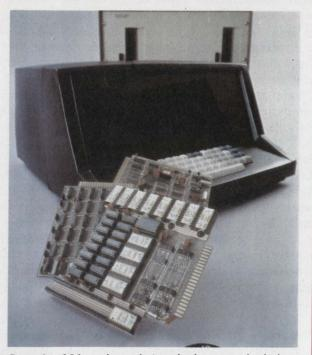
**Dasyn's 101 universal terminal** uses single-bus architecture and an Intel 8008 CPU to provide considerable flexibility. A variety of memory boards and I/O interface boards and peripheral controller boards can be plugged into the bus.
