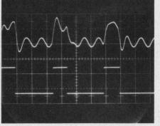
Upper trace: distorted, noisy input. Lower trace: pulse generator output (Pulse Amplifier Mode).
