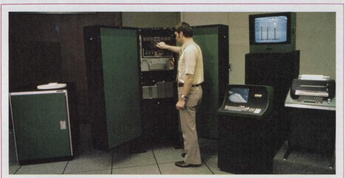
A Western Electric plant in Massachusetts uses a DEC PDP-8 minicomputer to monitor and control several coil-winding stations. The stations are
