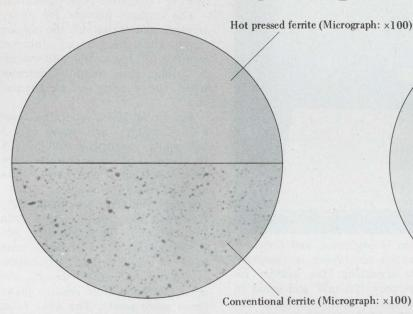
TDK is now producing manganese-zinc ferrite combinations with optimum performance characteristics for computer application. The crystalline powder of these ferrite materials is ground to uniform granular size, hot pressed and sintered into molded head pieces of high density. TDK's Mn-Zn hot pressed ferrite head pieces are free of voids, smooth in finish and have excellent contact wear resistance.
