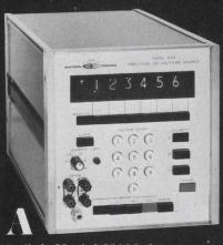
**6-digit Model M106 A.** Accuracy  $\pm 0.002\%$ . Range  $\pm 1$  microvolt to  $\pm 1,000$  VDC in 4 ranges. Solid-state voltage selections and digital display. Isolated remote BCD programming optional. A proven, versatile performer for bench, production or computer-controlled test systems . . . with a low basic price of \$2,375.
