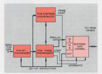
4. A typical PCM data path uses three pieces of equipment. The bit synchronizer extracts coherent serial PCM data and timing signals. The frame synchronizer identifies the data channels and provides parallel outputs. The subframe unit provides the frame count. Once started, the PCM path continually loads data into the computer via the buffer channel in a DMA mode.
