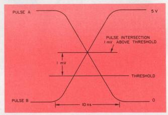
1. Problems can arise in a gate when the leading edge of an incoming pulse intersects the trailing edge of the second incoming pulse at a point near the threshold of the gate.
