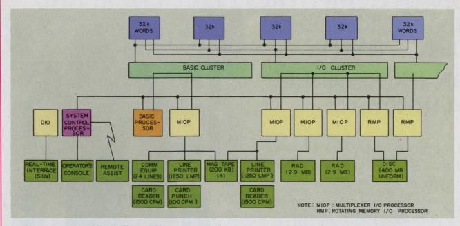
A very modern midi, the Xerox 560, makes use of an hierarchical architecture. Input-output and arithmetic processors have distinct functions but
