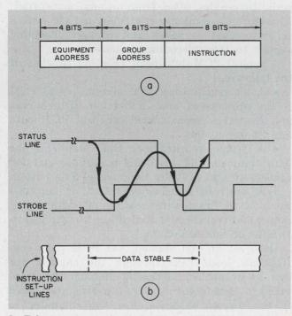
3. **Telemetry control words** (a) specify device address, type of instruction and the value associated with the instruction. For an FM path, the group address could signify center frequency deviation and the last eight bits the value. The status and strobe lines (b) control the transfer of information.
