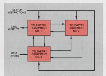
2. **Telemetry systems often have** multiple devices that require computer setup. However, a single output channel is typical.
