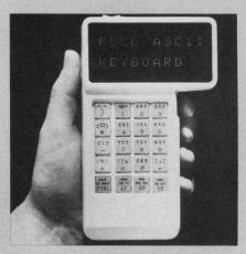
they appear as one or two-line displays. A display line consists of 10 5  $\times$  7 LED dot-matrix characters. When a line is filled, the display scrolls automatically. A 1000-character scrolling memory is built into the unit. And by operating one switch, the user can move forward or backward in this memory, to recover any part of a message that has been sent or received.
