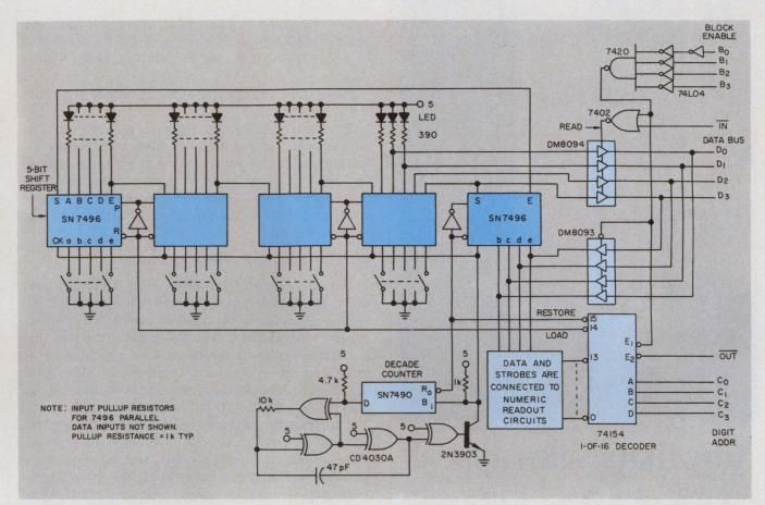
5. The functions of the switch circuitry include the sensing of switch closures in an addressable format.
