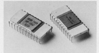
we've crammed all of the following: seven general-purpose registers, a status flag register, an arithmetic logic unit, an I/O multiplexer, and a 16-word LIFO stack that improves speed and performance while conserving main memory. The RALU number is IMP-00H/520D.
