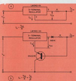
1. Resistive output divider allows adjustment of three-terminal regulator output (a) at the expense of variations due to changes in  $I_q$ . Addition of the transistor (b) reduces this sensitivity by a factor of  $\beta$ .
