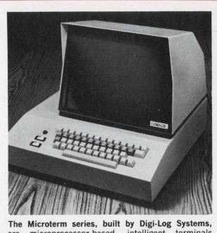
are microprocessor-based, intelligent terminals that can be customized to a user's specs.
