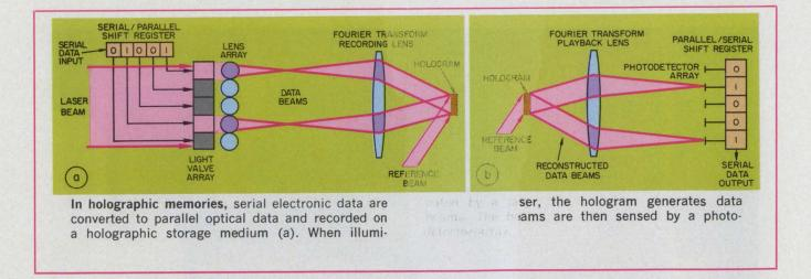
ally believed that the bit-by-bit memory will be widely available first. However, the holographic memory appears to be the goal of most developers of optical memories, because it offers higher speed and redundancy of data.
