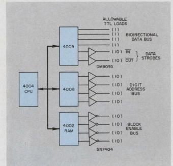
4. I/O operations and interfaces constitute much of the design effort. The I/O bus connections and loading are shown for a 4-bit microcomputer system, expanded for more than the basic 16-digit addresses.
