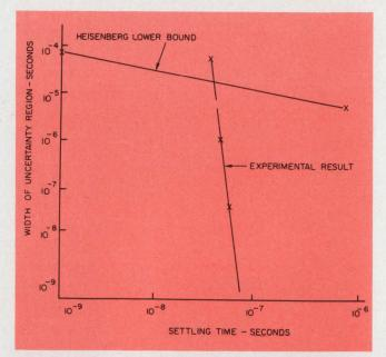
4. Experimental results of the "uncertainty" test are compared with the values predicted by Heisenberg's uncertainty principle. Discrepancies may be caused by thermal noise.
