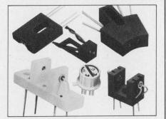
SENSOR AND EMITTER ASSEMBLIES Reflective sensor and optical switch assemblies, utilizing phototransistors or photodarlingtons, are available in several configurations. From a mirror reflection, the phototransistor version generates a 600 microamp signal with 30 milliamps of current on the LED. The photodarlington unit will generate a typical signal of 8 milliamps. These devices are designed for optimum performance at distances ranging from 0.075 to 0.5 inch and are TTL compatible.
