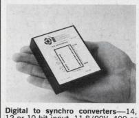
12 or 10 bit input, 11.8/90V, 400 or 60Hz transformer isolated output, accuracy  $\pm 4$ ,  $\pm 15$  or  $\pm 30$  min. Driving 1VA, 2VA (2.6" x 3.1" x 82"H module) or 5 VA loads ( $4\frac{1}{2}$ " x 9<sup>1</sup>/<sub>4</sub>" pc card). Price from \$350 in qty. Computer Conversions Corp., East Northport, N.Y. 11731. (516) 261-3300.
