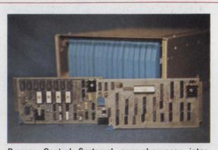
Process Control Systems' general-purpose interface, the Series 2000 (background), uses the Intel 8080 as the heart of a micro-CPU module.
