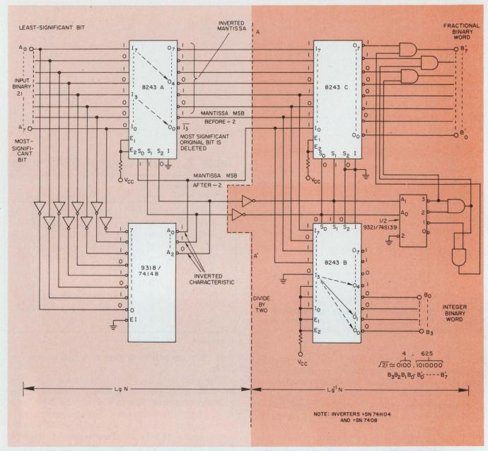
2. A combinatorial 8-bit square rooter needs only a log\_ circuit, a wired divide-by-2 and an antilog\_ circuit.
