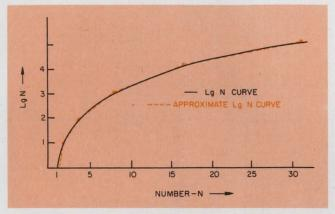
1. A plot of logarithms is closely approximated by straight-line segments between whole powers of 2, which are the logs<sub>2</sub> of the binary-number sequence.
