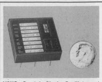
VCXO Crystal Clock Oscillator at freqs. from .00005 Hz to 50 MHz freq. tol.  $\pm$ .0005% 0°C to  $\pm$ 50°C, control voltage range  $\pm$ 4V to -4V changing freq. 20 ppm/V, linearity  $\pm$ 2%, 1.75" sq. x 0.5", Supply 5Vdc  $\pm$ 1%, Sq. wave 2.4V into 200Ω at Vdd = 5V, stock to 5 weeks; Connor-Winfield Corp., W. Chicago, III. 60185. 312-231-5270
