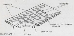
When the liquid is not electrically excited, its long, cigar-shaped molecules are parallel to one another in a position perpendicular to the plates. Thus, the liquid appears transparent. Applying an electric current creates ion activity which leads to turbulence and causes the liquid to scatter incident light. The visual effect is that of a frosted glass. LCD's can be made completely transmissive for back-lighting, reflective for ambient light or semi-reflective for dual mode operation.
