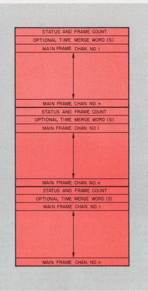
5. A typical data block in memory starts at location x and consists of y words. The status block permits the computation of the subframe or channel at which sampling began. The buffer signals the computer via an interrupt when a block is completed and begins a new block in an alternate buffer area. PAM/PDM data are handled in much the same way that PCM are. Once set up, the path continuously sends data into memory.
