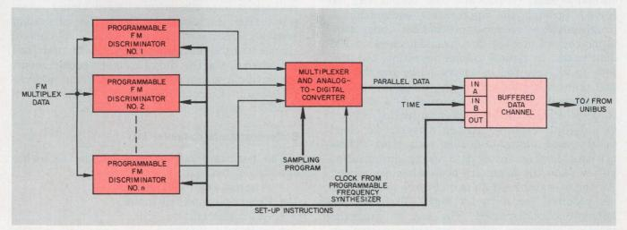
6. FM analog data must be digitized before being inputted to the buffer. The multiplexer controlled by the computer via the channel selects the appropriate sampling plan in accordance with the data rates. vention during data acquisition.
