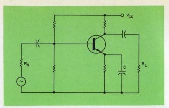
4. By simplifying the design equations for the decoupling capacitor, you can use a calculator to get the answer.
