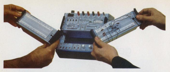
Removable sockets are provided by Adam I, by E&L Instruments, so one engineer can use the system's power
