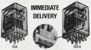
The new RAX relay is an adaptation of the popular RA Type and includes plastic barriers between the movable arms, thereby enabling opposite polarity voltages to be applied to the unit without fear of arc-over.
