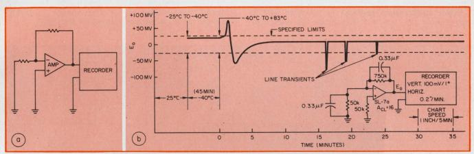
1. Simplified test setup to monitor the magnitude and settling time of the warmup drift of a differential op
