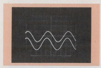
3. Phase shift of the class-D amplifier varies according to input frequency. The top sinusoid (signal at B<sub>3</sub>) lags the input  $(A_1)$  by 19°.
