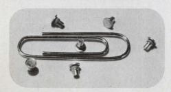
These developmental diodes have operating voltages from 100 to 143V, with operating current from 50 to 900 mA, depending upon frequency and power output.
