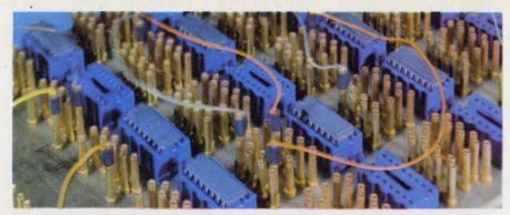
For breadboarding small quantities of ICs, this panel from Augat is handy, because interconnections are made with standard wire jumpers.
