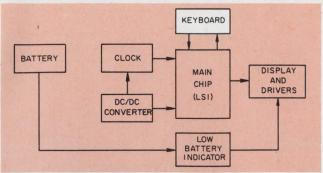
The basic calculator can be divided into many different functional sections that together do the computations and display the result.
