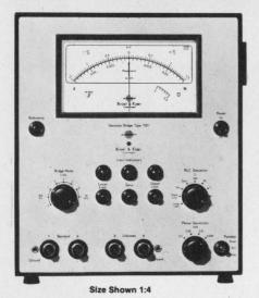
B & K's 1519 and 1521 Deviation Test Bridges are direct-reading instruments for fast, accurate determination of the percentage deviation of impedance and phase angle difference of capacitors, inductors, and resistors. No need for expensive standards; use your acceptable component as reference.
