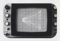
A non-triggered modulation trapezoid display of a 1 GHz carrier modulated with a 12 MHz sinewaye.
