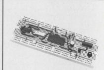
A P Super-Strip. Universal bread-boarding with 840 solderless, plugin tie points, incorporates eight distribution buses. Specifically designed for LSI packages and components with lead diameters up to .032". Accommodates up to eight 14 pin DIPs. No special patch cords required. A P Products Inc., Box 110, Painesville, Ohio 44077.
