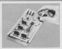
Free sample shows how you can assemble your prototype circuits in minutes even your card cage bread board. Mini-mounts, a series of etched patterns which adhere to your ground plane, mount all electronic components for prototype circuits from dc to GHz. Christiansen Radio, Inc., 1950 San Remo, Laguna Beach, Ca 92651. (714) 497-1506. INFORMATION RETRIEVAL NUMBER 182
