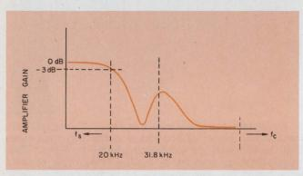
4. Frequency response of the amplifier attenuates and boosts input f<sub>s</sub> at two points. The -3 dB point shown corresponds to amplifier bandwidth. The second peak in the curve, which has a center frequency of 31.8 kHz, corresponds to the resonant frequency of the demodulator components.
