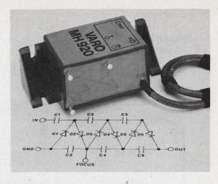
High-voltage multipliers are available for CRT display systems, electrostatic power supplies, TV receivers, and other high-voltage applications.
