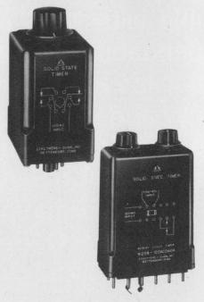
Time delay is precise, compact, and cheap with this new S-D plug-in family of hybrid relays. Choose from "on" delay, "off" delay, repeat cycle, and monitor timers, all designed specifically for industrial environments. All have transientprotected solid state timing circuits that remain accurate over wide variations of voltage and temperature. Timing is adjustable from 0.1-10, 0.6-60, or 1.8-180 seconds. DPDT relay contacts handle 10 amp loads with complete input/output isolation at minimum cost.
