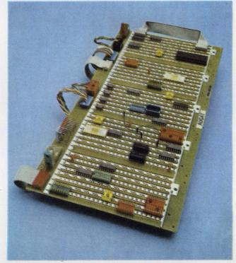
Breadboard hardware, by Augat, is designed to accept either ICs or sockets into which ICs can be plugged. Interconnections are made with wrapped wire.
