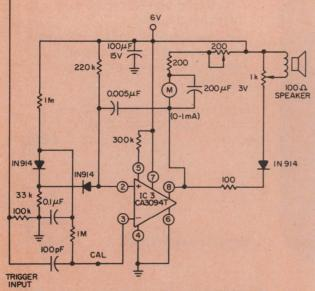
A single 6.75-V mercury battery runs this micropower Geiger counter. Full-scale meter deflection is 5000 counts/min and the entire circuit draws less than 2 mA in the absence of ionizing radiation.
