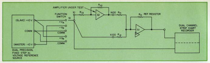
Initial step-transient response is measured with a fairly simple rig. The test determines the effects of
