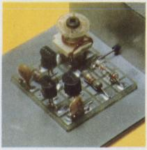
Tuned circuit can be mounted in less than four minutes on a GP-7 Mini-Mount, Christiansen Radio says. It's one of 14 patterns used in the company's no-hole, no-drilling, dc-to-GHz breadboard systems.
