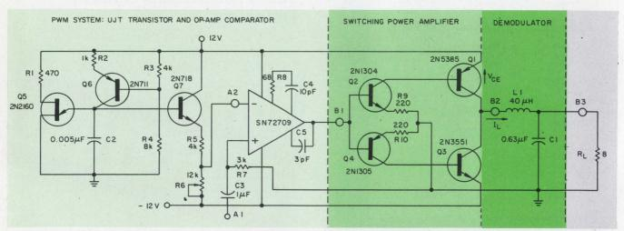
1. The circuit uses a combination of analog and digital techniques, so efficiency of the switching power amplifier approaches the theoretical 100% limit. The value of
