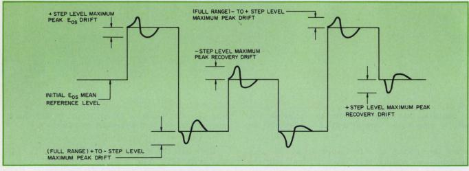
3. Various step input levels are selected by trial and error to pin down the maximum step-transient criteria.
