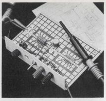
Instant Breadboard, by Instant Instruments, Glen Cove, N.Y., allows the engineer to assemble a circuit without inserting components. The circuit is soldered to pre-etched patterns of large, lift-resistant copper.
