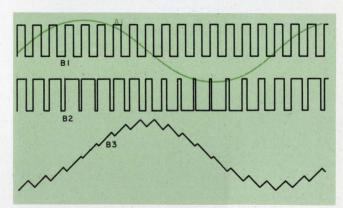
2. Waveforms at various points in Fig. 1. The sinusoidal input signal (point  $A_1$ ) provides a modulation frequency  $f_{\rm s}$  at the comparator's noninverting terminal. Without the input signal,  $f_{\rm c}$  consists of a 50% duty cycle square wave (point  $B_2$ ). The presence of  $f_{\rm s}$  modulates  $f_{\rm c}$ , and varies the duty cycle. The signal at  $B_3$  consists of an amplified pulse-width-modulated carrier, integrated in a low-pass LC filter.
