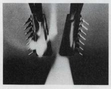
ICs, MOS, CMOS, and other devices made with flame resistant silicone molding compounds provide in many applications the reliability of hermetics at about ½ the cost.
