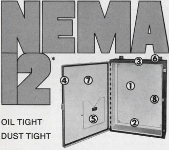
1. Heavy gauge steel rigid construction. 2. All seams continuously welded. 3. Rolled lip for strength, also helps keep dirt and liquid out when door is open. 4. Neoprene door gasket with oil resistant adhesive and steel retaining strips. 5. Removable print pocket. 6. External mounting feet. 7. All sizes, full stock: wall and floor mounted, one to five door. 8. Models available in stainless steel and aluminum. For detailed specifications, write for new catalogue.
