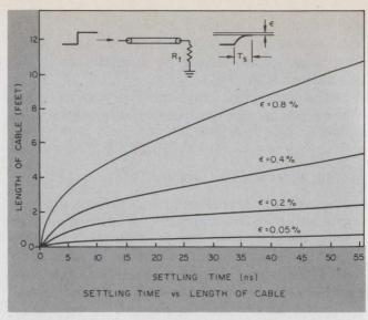
7. Settling times of RG58/U coaxial cable for a step input and for various error bands expressed as a percentage of step amplitude. Miniature cable takes longer to settle, while larger, low-loss cable takes somewhat less time than RG58/U.
