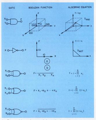
3. Recognition of potential static hazards requires ternary algebra with permissible levels of 0, 1 and r, where 0 < r < 1. Logic functions, such as these basic types, can be approximated by simple polynomial equations (a). The polynomials have values in the closed interval (0,1) and represent ternary functions. The equations are easily combined by ordinary algebra to represent multi-input gates (b).
