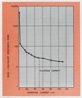
3. The equivalent base-1 resistance can be approximated by a constant—the resistance corresponding to an average current value. The constant gives the resistance for the discharge period of the circuit capacitor.
