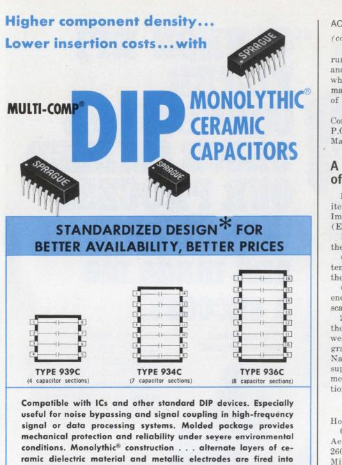
\* Other circuit configurations (including internally-paralleled capacitor sections, commoned capacitor leads, and various ratings within single package) are available on special order.
