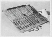
NOVA/DCC-116 General purpose interface board provides multiple device selection, 4 I/O registers, DMA zero word count detect, 105 socket positions for 14, 16, 24 and 40 PIN ICS. Basic board (all features of data general 4040 plus multiple device select) \$350.00. MDB Systems, Inc., 981 N. Main, Orange, CA 92667. (714) 639-7238.
