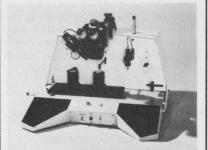
SA202 "EPOBONDER" Epoxy Die Bonder—can be used with LSI's, MOS's, diodes, transistors, chip ca-pacitors and resistors. Picks up, locates, places and bonds chips quickly and accurately. Ultra-reliable operation. Laurier Associates, Inc., Littleton, Mass. 01460 (617) 486-8100
