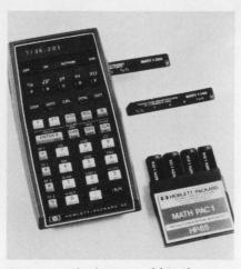
the new calculator enables the user to write and store on magnetic cards a program containing up to 100 steps or several programs totaling 100 steps. When the recorded program is no longer needed, the magnetic card can be erased on the same machine and reused to record another program. Accidental erasures can be prevented through clipping of a corner of the magnetic card.
