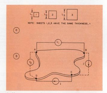
1. Measurement of  $R_{\Box}$  depends on the fact that the resistance between the edges of a square sheet is independent of size (a). Thus  $R_{\Box}$  can be determined from just two voltage measurements (b).
