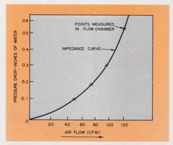
2. Pressure drop across an air-cooled electronic assembly varies exponentially with increasing air flow. The most practical way to obtain such an impedance curve is to measure the data with a test chamber as in Fig. 3.
