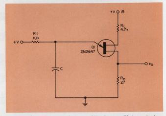
1. A unijunction-transistor relaxation-oscillator design involves trial and error when you use a conventional approach to obtain the capacitance.
