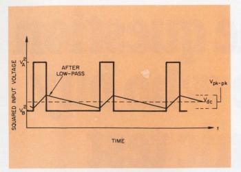
7. If you square the pulse train of Fig. 6 and then low-pass filter it, you can get a triangular waveform.
