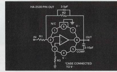
summations, high speed integrators, wave form generators, coaxial line drivers, and fast D/A outputs. For details see your Harris distributor or representative.
