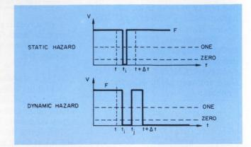
1. Two common logic hazards that can occur with input signal changes. Glitches result from static hazards; contact-bounce waveforms result from dynamic hazards.
