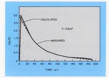
4. Close agreement results between measured output voltages and those calculated from the improved formula for pulse width.
