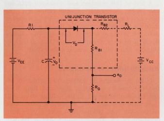
2. The equivalent relaxation-oscillator circuit reveals UJT parameters— $V_{\rm D}$  and  $R_{\rm B1}$ . These parameters can be used to simplify the oscillator circuit design.
