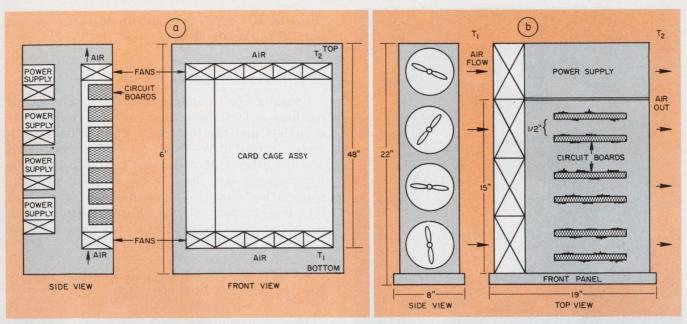
5. Multiple fan systems have advantages. A series fan configuration (a), with one set at the input port and the other at the output, provide double the pressure capability that a single set would. And the parallel arrange-
