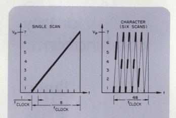
1. Series of six vertical scans provides the raster for character generation. Blank portions of the character are formed by deflection of the CRT spot off the scope face.
