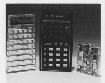
The HP-35, the first pocket electronic slide rule to be introduced, contains five ICs.
