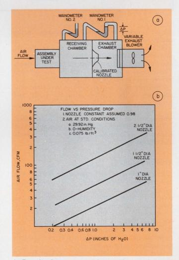
3. Two chambers connected by a calibrated nozzle (a) provide a measure of the air-flow rate. A calibration chart (b) converts the pressure difference read on manometer 1 into air flow. Manometer 2, which is open to the atmosphere at one end, indicates the pressure drop that the cooling fan needs to generate to force the given air-flow rate through the assembly.
