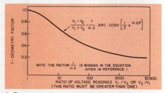
2. To account for current distributions in irregularly shaped conductors, a geometry factor, f, is plotted as a function of the ratio of the voltage readings.
