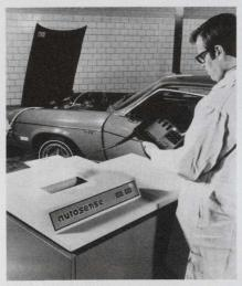
Autosense system employs sensors attached to engine and other parts of the car to measure vehicle operating performance. Computer is housed in console. Hand-held unit controls and monitors the test system.
