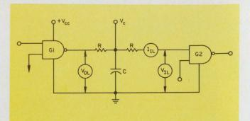
5. When  $G_1$  goes low, the important circuit parameters are  $V_{\rm OL}$ ,  $I_{\rm IL}$  and  $V_{\rm IL}$ .
