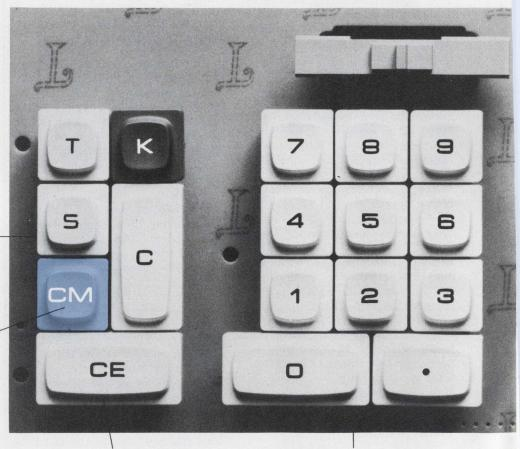
Keyswitch materials and a high length-over-diameter ratio provide the smooth, quality feel necessary for professional users. Fully assembled on a circuit board to reduce your assembly costs.
