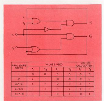
5. Analysis of sequential networks for potential glitches uses a variation of Eichelberger's theorems. The secondary variables are analyzed for their sequence of values. The sequence 0-r-0 for  $y_1'$  denotes a potential static hazard.
