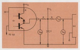
4. Equivalent circuit of gate with the output of  $G_1$  in the HIGH condition.
