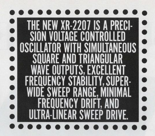
By providing 30 ppm/°C frequency stability, 3000:1 sweep range, and 0.15% /V frequency drift in the XR-2207, Exar produced a precision VCO that can easily do those tough FSK, FM generation jobs. With a minimum of external circuitry, you can use the XR-2207 in applications such as two-channel FSK generation for modems, as the VCO portion of phaselocked loop systems, and voltage to frequency conversion that formerly required crystal controlled oscillators.
