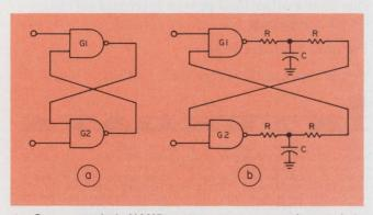
1. Cross-coupled NAND gates are commonly used to form the flip-flop in memories and registers (a). A simple RC T-network connected between gates can prevent the network from changing states when a nuclear transient burst occurs (b).
