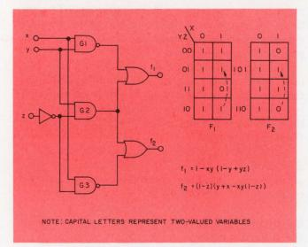
4. A combinatorial network can produce glitches for a specified input transition if the ternary function also has values between 0 and 1. The algebraic equation represents the ternary function. Outputs  $f_1$  and  $f_2$  can have glitches for the transition XYZ = 110 to XYZ = 101. Both equations equal  $1-r+r^2-r^3$  since y and z are indeterminate (equal to r) for this transition. The Karnaugh maps show a function hazard for  $f_1$  and both function and logic hazards for  $f_2$ .
