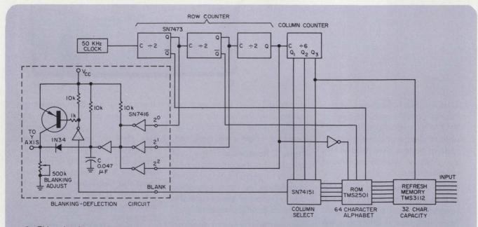
2. This circuit generates the vertical scans and blanking to form the alphanumeric characters. Auxiliary devices store the 64-character alphabet (ROM). The over-all system displays a full alphanumeric line when connected to the vertical input of a scope.
