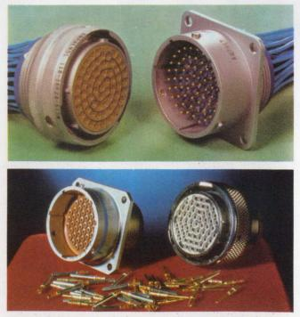
Both Amphenol's Merlin I and Bendix's Pygmy (bottom) lines feature dielectric retention discs. The discs eliminate the need for individual metal clips. This results in lighter and shorter connectors. Also, both lines employ a rear-release method for contact insertion and extraction and crimp-type terminations.
