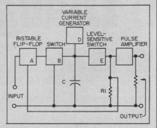
**Pulse-delay circuit** aids stroboscopic observation of parts.
