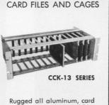
height adjustable card files supplied assembled ready for connectors which mount on 4-way adjustable struts. The cages are designed for and the cases with width ranges of 1.0" to 2.73"; 2.73" to  $41/_2$ "; 6.2" to 7.98"; and lengths up to 9.6". Plastic or metal guides available. Continuous extruded aluminum plate style has 106-0.075" wide continuous grooves on 0.150" centers for cards allowing maximum flexibility.
