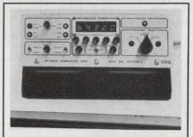
The Pulsecom Model 461-6 Automatic Message Numbering Device electronically inserts station identification and message numbers. This device saves operator time, and prevents mistakes. The 461-6 operates at 45-1200 Baud with most terminals. PULSECOM, 5714 Columbia Pike, Falls Church, Va. 22014. 703-820-0652.
