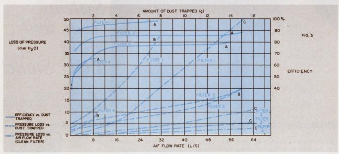
Filter efficiency remains nearly constant until accumulated trapped dust causes it to suddenly increase—a signal that the filter should be cleaned or replaced. While
