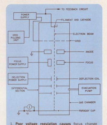
and beam deflection in pulsed operation of an
