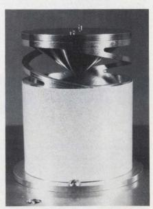
**Optical antenna** for a laser remote control system, a "parabocone," receives energy throughout 360 degrees.
