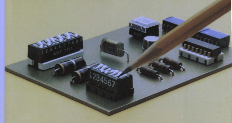
Down to the size of a DIP header—with our miniature Dual In-Line Switch. Because you can use it to program IC's right on the board without remote wiring, it cuts packaging costs, too.
