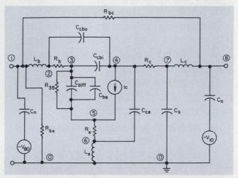
1. An rf-transistor equivalent circuit can be used for large-signal analysis or a precise determination of narrowband performance. Components  $R_{\rm be},\ R_{\rm be}$  and  $C_{\rm n}$  permit the handling of a wide variety of applications.
