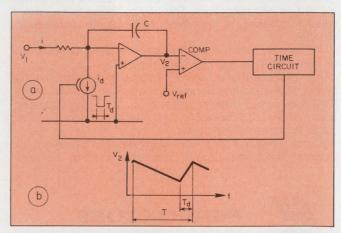
2. Best linearity is obtained by discharging C through a constant-current generator (a). Improved output occurs during  $T_{\rm d}$  (b).
