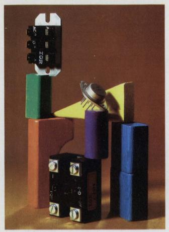
Power modules that contain several thyristors and diodes in various circuit configurations are available from International Rectifier.
