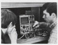
This simple to use, dual trace, 10 MHz D54 gives you low-cost, dependable performance in a wide variety of applications. Like all Telequipment scopes, it is light weight, easy to carry and is backed by Tektronix' warranty and reputation for quality. Students shown are testing amplifier circuit by measuring the gain between input and output signals.
