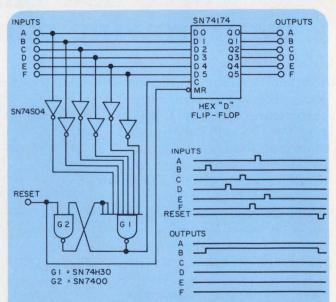
Hex flip-flop provides a logical output of the first pulse received. Once  $\mathbf{G}_1$  and  $\mathbf{G}_2$  latch, the pulse on the input line is transferred to the output of the flip-flop, and further output transitions are inhibited. A momentary ZERO on the reset line clears the flip-flop and arms the circuit for the next set of inputs.
