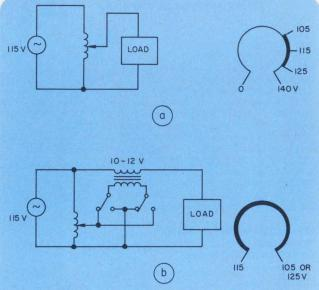
Autotransformer technique for setting load voltage (a) often requires expensive transformers and gives poor voltage resolution. The improved technique (b) gives better resolution at lower cost.
