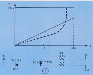
modifies the VI characteristic to ensure full output with current-sink loads.
