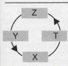
Operational stack has 4 registers . . . for automatic storage and retrieval of intermediate solutions. The stack design permits review of stored data at any time.
