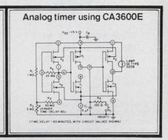
Meet the linear IC with the advantages of COS/MOS. The new RCA CA3600E Transistor Array... three pairs of complementary enhancement-type MOS (p-channel/ n-channel) transistors on a single chip.
