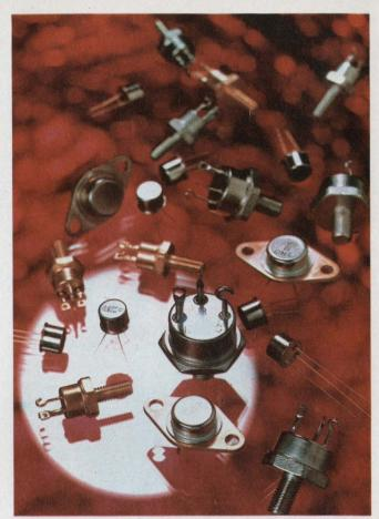
Silicon power transistors from Unitrode come in a variety of current ratings ranging from 0.5 A to 20 A.
