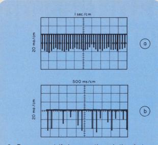
3. Beam current that passes through the electrongun aperture is approximately the same for each pulse (a) with use of the feedback circuit. Without the feedback circuit, the current pulses are nonuniform (b), an indication of beam wander.
