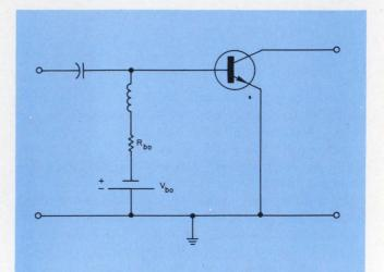
2. The internal resistance of a real voltage source must be considered, along with the voltage, to determine Class AB amplifier performance.
