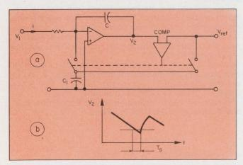
1. Linearity is improved in feedback-type  $\mathbf{v}/\mathbf{f}$  converter (a) by discharging feedback capacitor through  $C_1$  at the right moment during the cycle (b).
