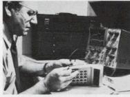
If you don't require delayed sweep but need dual trace at 25 MHz, here's another economical, quality scope—the D66. Trouble-shooting consumer digital products such as mini-calculators is made easier by using dual trace. Also a "SUM" mode with normal-invert capability makes it possible to look at small signals in the presence of common mode noise—such as power supply hum.
