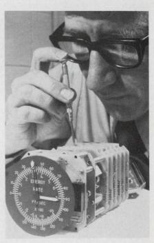
Adjustments are being made to Honeywell energy meter by Nelson Zagalsky, program manager of instrument development.
