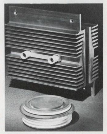
Disc packages, like the one used for Power Semiconductors' 6000-A diode, permit double-sided cooling.
