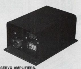
Choose from 1.4 watt output amplifiers to the new 2200 watt unit above. Only 10" long and weighing just 7 lbs., the XA-2200 is a highly-efficient solid-state amplifier that furnishes output required by 1 HP motors.
