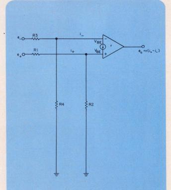
Effect of input  ${f V}_{\rm BE}$  on current-mode amplifiers can be eliminated if  ${\bf R}_4$  and  ${\bf R}_2$  are added to the circuit, provided  ${\bf R}_4={\bf R}_1$  and  ${\bf R}_2={\bf R}_3$ . The amplifier output equals a constant times the difference in input currents, as usual.
