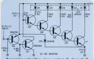
Successive saturation of transistors  $Q_1$  through  $Q_5$  give the LED display a bargraph appearance. Feedback through  $CR_1$  helps linearize the apparent deflection as a function of input voltage.
