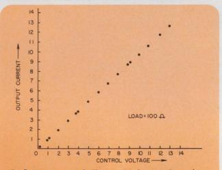
2. **Output current is linear** with input voltage from 0 to 10 V. The circuit shown provides a scale factor of 0.96 mA/V.
