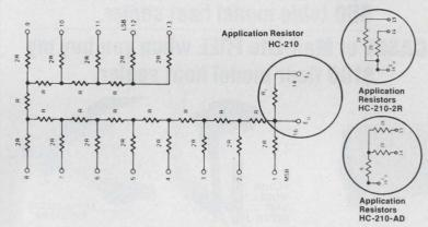
HC-1000 SERIES . . . 12 BIT LADDER NETWORK WITH STANDARD RESISTANCE VALUES OF 5K, 10K, and 25K. IN 16 LEAD DIP OR FLATPACK, HERMETIC OR NON- HERMETIC . . . OR 100 x 150 MIL CHIP. AS LITTLE AS \$23.20(1-99)
