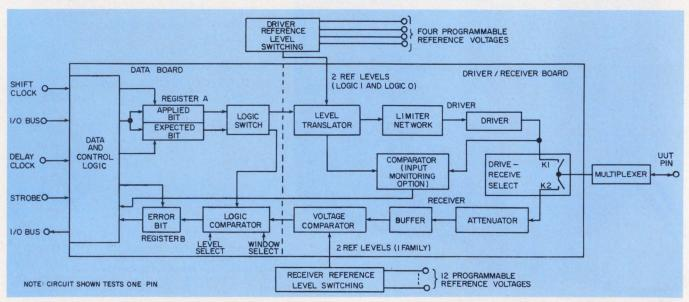
**Driver receiver module** handles a variety of logic levels. Each module can, on command, supply stimuli
