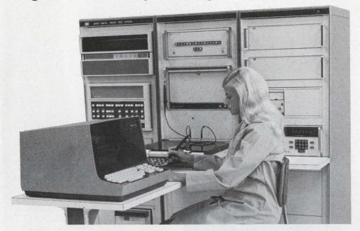
You don't need reference units because the 9560 system uses stored test patterns (truth tables). You can test at rates up to 22,000 patterns/second.
