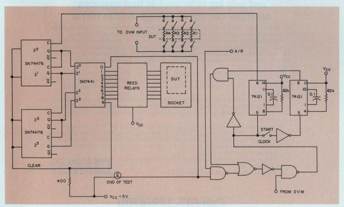
3. Details of counter, decoder-driver and clock: Seven decoder outputs energize double-pole reed relays that
