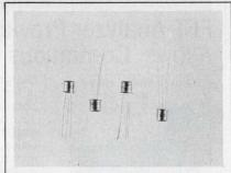
The 2N5650, 2N5651 and 2N5652 are low noise transistors specified for operation at VHF, UHF and low microwave frequencies. These NEC transistors are packaged in the popular T0-72 package and feature 500 MHz noise figures of 1.5, 2.0 and 2.5 dB. California Eastern Laboratories, Inc., One Edwards Court, Burlingame, California. (415) 342-7744.
