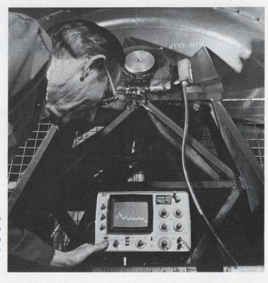
It's portable (only 35 lbs/16 kg.) and operates on batteries or line power, so you can take the new 3580A spectrum analyzer anywhere. This unique low-frequency spectrum analyzer has digital storage, CRT display, 80 dB dynamic range, "adaptive" sweep, and -150 dB sensitivity.
