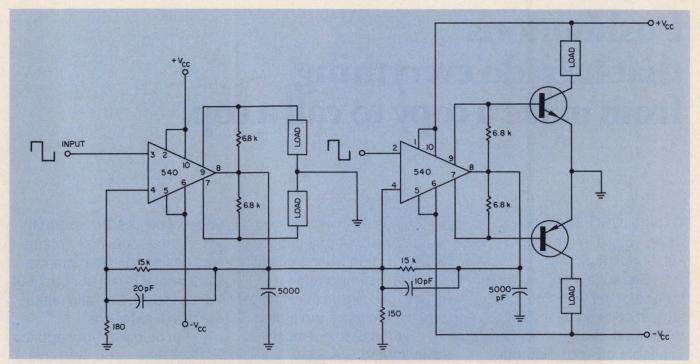
7. Relays, solenoids and small motors can be driven by the power driver, as shown.
