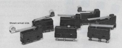
For example: A line of SUBMINIATURE switches designed to give you unlimited performance in a limited space. Features like: five basic ACTUATOR STYLES— pin, integral flexible leaf, leaf/roller, integral rigid lever, lever/roller— four TERMINAL STYLES—ELECTRICAL RATINGS from 1 ma 1.5 VDC up to 10 amp 250 VAC and 2.4 amp 28 VDC lampload—allow you to select the exact small switch to do your big job.
