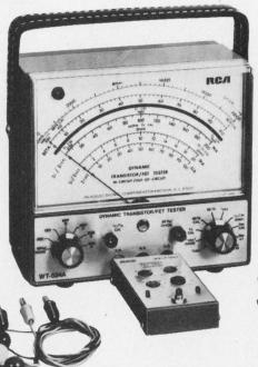
RCA introduces the WT-524A, a new "one for all" tester for solid-state devices. With it, you can measure AC beta – up to 5,000 – of any bipolar transistor, and Gm – up to 100,000  $\mu$ mhos – of any field-effect transistor (FET). And you'll do it with an accuracy of  $\pm 3\%!$  It also checks diodes, SCR's and triacs – and can do the job in-circuit or out
