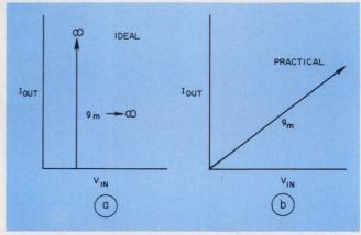
1. An ideal transconductance amplifier (a) has an infinite  $g_{\rm m}$  and, consequently, current. In practice, however, the current-vs-voltage curve is a linear function, with  $g_{\rm m}$  being the curve's slope (b).
