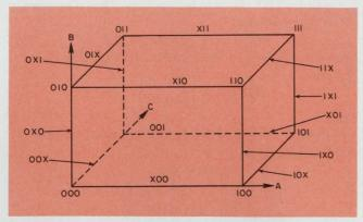
1. The universal cube for a three-variable Boolean function has 6 planes (2-cubes) and 12 edges (1-cube). In this topographical interpretation, vertices represent minterms; X's signify absence of a literal; and 1 denotes the variable and O, its complement. The literals in the are A, B, and C—in that order.
