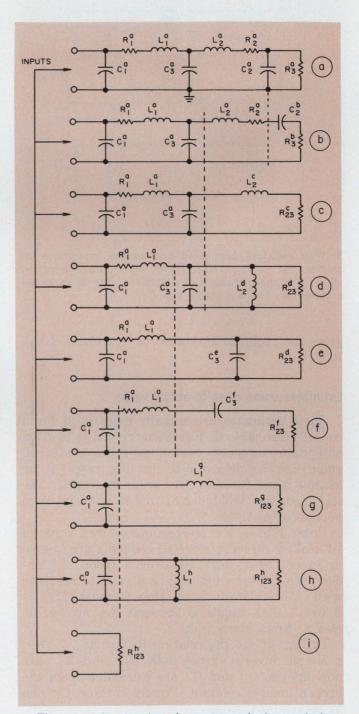
4. The general network reduces to a single, equivalent component by use of the relationships in the circular chart. For maximum power transfer, design the image input impedance— $R_{123}$ h—to equal the source impedance.
