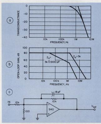
3. Constant transconductance over a wide frequency range is obtained when the load is resistive (a). Openloop voltage gain falls off faster when the load is capacitive (b). One way to compensate a power driver is to insert a lead network into the feedback loop (c).
