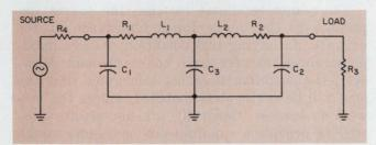
3. A general RLC network covers a variety of transfer functions often encountered. These include circuits for large-signal rf amplifiers.
