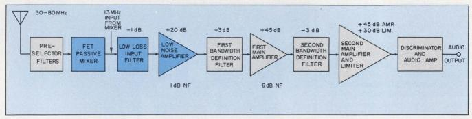
High-level rejection of nearby, strong adjacent channel signals was provided in the receiver, above, by use of new design techniques. The rf input stage was eliminated and only the passive mixer stage, preceded by preselective filters was used for the front end. The system selectivity was due to the first crystal filter.
