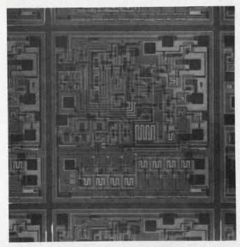
Waveform generators are fast shrinking in size but growing in performance. The example shown is the Intersil 8038—a monolithic multiple waveform generator.
