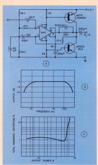
6. Power amplifier for a car radio (a) has a wide range of flat output vs frequency (at 0 dB, output is 1-V rms into  $5-\Omega$ ), as shown in b. The total harmonic distortion is relatively low over the range of useful power output (c).
