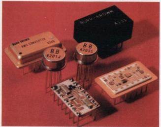
Burr-Brown makes these rms converter modules that contain thermally coupled transistor pairs that accurately perform rms calculations without regard to waveshape.
