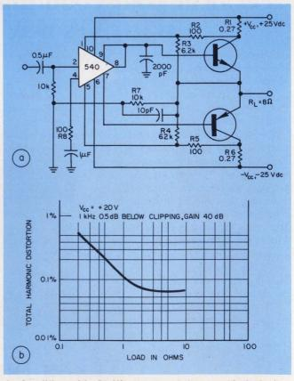
2. Amplifier with 35-W output (a) has a relatively low total harmonic distortion (b).
