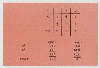
3. **Row intersection** determines the minterms common to  $c^i$  and  $c^j$ . The appearance of  $\phi$ , when the columns are compared according to the table, gives a vacuous response (case 2).
