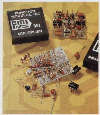
Construction of this multiplier from Function Modules. Inc., typifies the usual packaging approach for modules. Combined on one potted printed circuit board are resistors, capacitors, transistors and "discrete" ICs.
