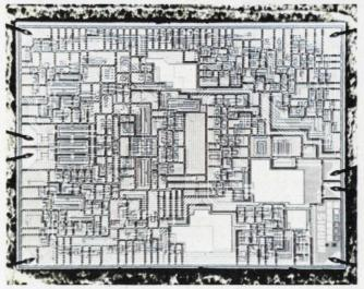
By combining bipolar and MOS technologies. Harris Semiconductor has developed the first truly monolithic chopper-stabilized op amp with differential inputs.
