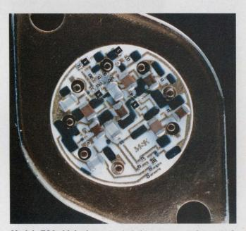
**Model 780 high-slew-rate** hybrid op amp, from M.S. Kennedy, offers a 2000 V/ $\mu$ s slew rate with an output drive of 80 mA. It also has a 120-MHz bandwidth and is spec'd over the Mil temp range of -55 to +125 C.
