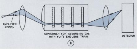
Wide-angle laser receivers with low noise and high sensitivity are seen as feasible with arrangements like those shown above. The absorbing element in both systems allows the signal to pass, yet blocks the noise.
