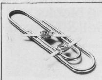
Thin-Trim variable capacitors vide a reliable means of adjusting capacitance without abrasive trimming or interchange of fixed capacitors. Series 9401 has high Q's and a range of capacitance values from 0.2-0.6 pf to 3.0-12.0 pf and 250 WVDC working voltage. Johanson Manufacturing Corporation, Boonton, New Jersey (201) 334-2676.
