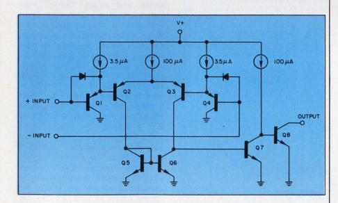
Unlike most comparators, the LM 139 can operate from a single power supply and still have an input common mode voltage range that includes ground. It is compatible with all forms of logic and has a power dissipation ranging from 570 mW to 900 mW, depending on the package.
