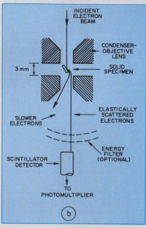
Conventional electron microscopes (a) use a long focal-length lens while IBM's new technique (b) allows the use of shorter lenses for higher resolution.
