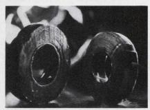
Appliance malfunction and even fire hazards can be minimized with Sylgard® 170 elastomer. For example, television manufacturers are using it on high voltage flyback transformers as shown above (left).
