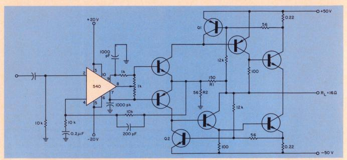
5. 75-W, 95-V-swing power amplifier uses two stages.
