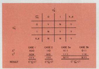
2. **Boolean product c' subsumes** (is a subset of) c<sup>1</sup> if it contains nothing but a subset of minterms of c<sup>1</sup>. An all-Y result, based on a column-by-column comparison according to the table, is needed to affirm that c' subsumes c<sup>1</sup>.
