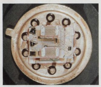
Halex's Model HX610 hybrid wideband amplifier delivers gain at frequencies beyond 100 MHz. When connected to a  $100-\Omega$  load the maximum output voltage at 100 MHz is 1.2 V pk-pk.
