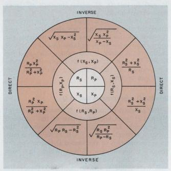
2. All possible conversions are tabulated in a circular chart. The formulas in the outer ring provide the RLC equivalents for series-to-parallel and parallel-to-series conversions.
