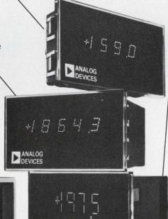
A high-performance 3½ digit DPM for systems applications. The kind of performance you need for complex system interfacing and data processing. Incandescent display. True differential instrumentation amplifier input. Full scale range of 0 to ±199.9mV. 0.05% ±1 digit accuracy. Automatic zero and polarity. Normal mode rejection of 40dB at 60Hz or 50Hz. Common mode rejection of 80dB at ±2.5V. Fully-latched DTL/TTL compatible BCD outputs and control interface signals. \$99 in 100's. AD2003.
