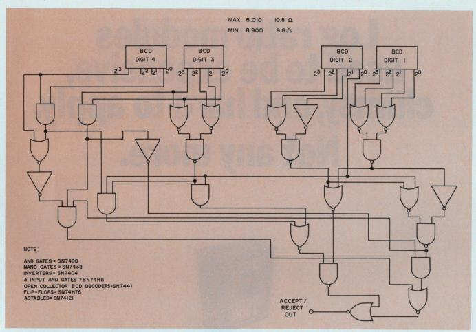
2. DVM data outputs are decoded for the device limits by NOR-NAND gates. Readings outside the limits are
