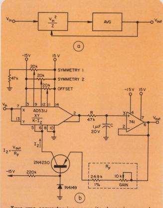
True rms converter increases its dynamic range by simultaneously squaring and square-rooting in the  $V_{\rm in}^2/Z$  block (a). The actual circuit (b) requires only four trim adjustments and 13 components.
