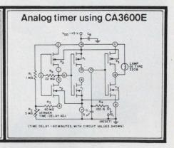
Meet the linear IC with the advantages of COS/MOS. The new RCA CA3600E Transistor Array... three pairs of complementary enhancement-type MOS (p-channel/n-channel) transistors on a single chip.
