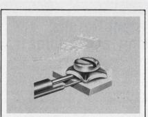
Sems Termi-Lox Saves Assembly Time. X-rib design permits better fastening with various variety wire sizes. Stripped wires are inserted straight in without wrapping. Shape holds wire, of same or different size, without binding, jamming and shearing. Sems Div. Camcar Screw & Mfg., 1818 Christina, Rockford, III. 61108. 815-226-2400.
