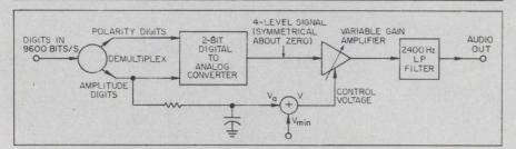
**Two-bit adaptive pulse-code modulation coder** (above) produces an output of 9600 b/s. At the receiving end the digits are demultiplexed by the two-bit decoder shown below.
