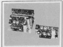
50 sub modular, D.C. power supply models for "In House" and custom designs, upto 30V, upto 75A. Unique "building block" design exclusive built-in rectifier, filter, regulator, protective functions. Transformers, heat sinks, wiring harness and chassis available. Send for catalog. Powertec, Inc., 9168 DeSoto Ave., Chatsworth, Ca. 91311. (213) 882-0004.
