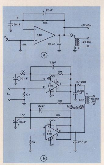
8. Single-ended (a) or balanced line driver (b) can be built with the power driver, simply and inexpensively.
