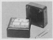
New low-cost compact modular os-cillator Model UC utilizes piezoelectric ceramic resonator for frequency control. Frequency range 12 Hz through 400 kHz, accuracy to .05%, output TTL or CMOS compatible. 1% tuning option available. Fork Standards, Inc., 217 Main St., West Chicago, III. 60185. (312) 231-3511.
