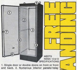
rack angles available. 3. Heavy gauge steel. 4. All seams continuously welded. 5. Lifting eyes for easy handling. 6. Neoprene door gasket with oil resistant adhesive and steel retaining strips. 7. 3-point latching mechanism, oil tight key locking handle. 8. Heavy gauge continuous hinges. For detailed specifications on over thirty different sizes, write for latest bulletins.
