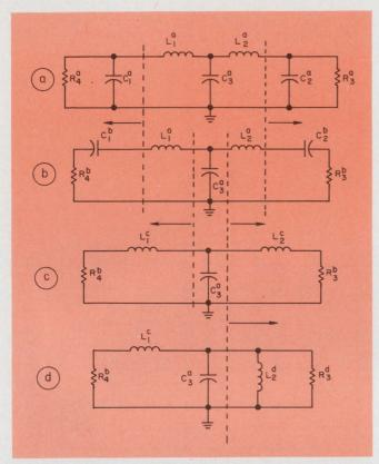
5. With resistors eliminated and source impedance included, the iteration begins with an arbitrary selection of  $L_2$ . The approximation of a lossless case is generally a close one for reasonable coil Qs.
