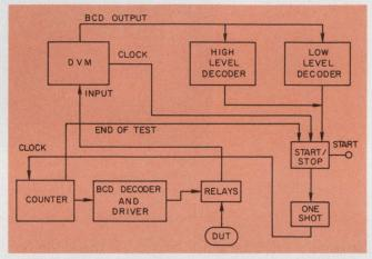
1. **Test-system block diagram** shows functional relationship between circuit elements. For N devices, N drivers are required; for n limits, n decoders are needed.
