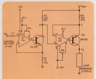
1. Variable-current generator operates by successively transferring input-voltage variations to the emitters of  $Q_1$  and  $Q_2.$  Control of emitter current instead of base current minimizes errors caused by changes in  $h_{\rm FE}$  and  $V_{\rm BE}.$
