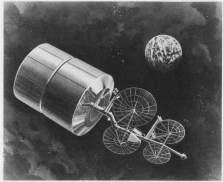
Intelsat IV-A, which is expected to be launched in mid-1975 to a station over the Atlantic, will handle 8600 circuits and output 500 W of power. The satellite will weigh 1700 pounds and has been designed with a seven-year life expectancy by Hughes Aircraft Co.
