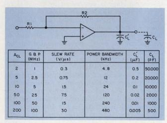
4. A capacitor across the output frequency-compensates a power driver. The required capacitor value depends on the closed-loop gain,  $A_{\rm CL}$ , as shown in the table.
