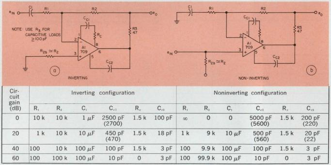
Parenthesized values are nearest 10% components. Values of  $C_1$  chosen to give  $15.9\,$  Hz lower corner frequency
