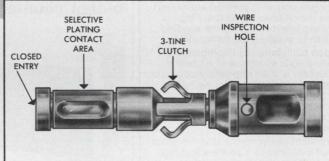
Crimp removable socket contact with wrap around spring provides positive contact between socket and pin. 3-tine clutch assures extra reliability in socket contact insertions and removal.
