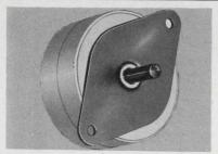
Permanent Magnet Synchronous Motor. Low cost motor provides torque to 10 in-lbs at 300 RPM rotor. Features electric reversability, instant start/stop, permanent lubrication, quiet operation, and compact size—2·1/4" dia. x 1·1/8" long. For computer peripherals, control devices, chart drives, and similar applications. ECM Motor Co., 1301 E. Tower Rd., Schaumburg, III. 60172.
