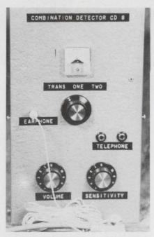
**Debugging device** is an untuned rf receiver that picks up signals between 1.75 and 900 MHz. When the receiver squeals, it has picked up a hidden, active transmitter.
