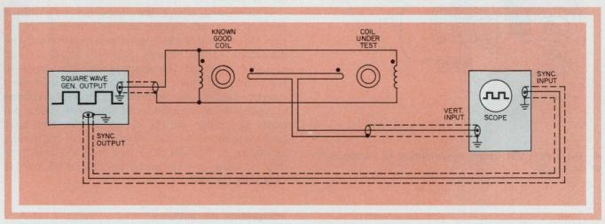
2. Coils are tested with a very simple circuit, a scope and a square-wave generator.
