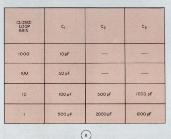
3. Typical amplifier frequency characteristics as a function of compensation used. Reductions in compensating capacitor values increase the GBP. The reduction in compensating capacitance applies to the use of higher noise gain.
