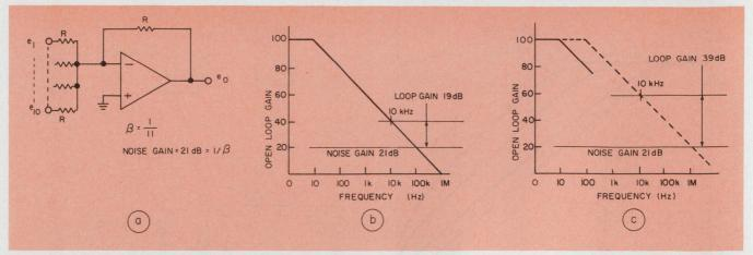
6. Noise gain of a unity gain mixer (a) limits the available loop gain (b). However, decreasing the compensating capacitance increases the available amplifier GBP
