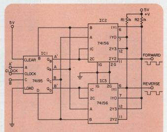
3. Pulse trains appear at the output of IC<sub>2</sub> or IC<sub>3</sub>, in the quadrature decoder, depending on whether the transducer motion is in the forward or reverse direction. The number of pulses generated is proportional to the transducer displacement. The clock rate should be set for at least eight times the pulse frequency of the input.
