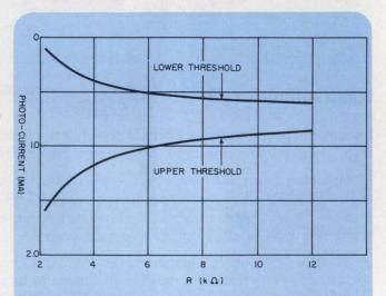
2. Select the operating thresholds from these curves. The saturation voltage of the phototransistor must be less than 0.4 V at the upper threshold current.
