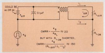
1. The CMCT "rejects" an unwanted common-mode pulse, eg, but passes the desired dc differential current.
