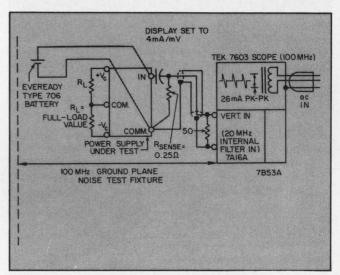
3. A converter's input current spikes, known as reflected input ripple current, are measured at the input terminals by sampling current with a nonreactive resistor.
