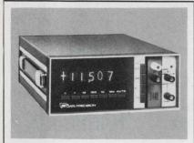
Auto-ranging 4-1/2 digit DMM, \$675. Model 2440 measures  $100~\mu$  V to 1000~VDC (accuracy  $\pm 0.007\%$  of reading  $\pm 1$  l.s.d.);  $100~\mu$  V to 500~VAC; 2-wire & 4-wire resistance; DC/DC & AC/DC ratio. Includes autorange, auto-zero, remote range & trigger, & isolated BCD output. Data Precision Corp., Wakefield, MA 01880. (617) 246-1600
