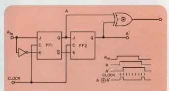
2. The EXCLUSIVE-OR of signals A and A' determines the transition points of the transducer signal  $A_{\rm IN}.$
