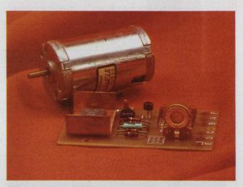
This speed-regulated dc automotive stereo tape-deck motor made by Barber-Colman keeps wow and flutter to 0.1%. And the speed can easily be adjusted over the range of 400 to 4800 rpm with regulation held to 1%. The motor can deliver 1.5 oz-in. at 3000 rpm.
