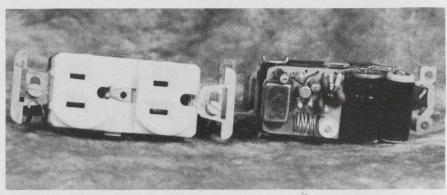
The bug in the plug pulls juice from the wall plug it's slipped into, and it will transmit indefinitely all room conversations to a receiver 800 feet away. The unit can still be used as an electric plug while transmitting.
