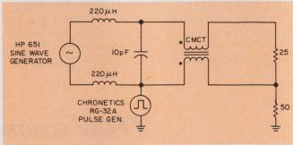
2. 10-MHz differential signal is unattenuated, but the common-mode pulse is rejected.
