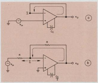
4. Both circuits provide unity operating gain. But the loop gain of the inverter (b) is half that of the voltage follower (a) because of the presence of the divider in the feedback path. The 50% reduction in loop gain with the inverter permits use of smaller compensating capacitors.
