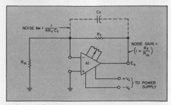
1. Op amp powered by dc-dc converter passes negligible converter switching spikes because of narrow bandwidth and slow response.
