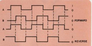
1. Forward or reverse movements of an incremental encoder cause waveform B either to lag or lead waveform A.
