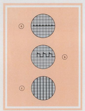
5. **Typical test patterns** on the scope show the results if two identical coils are tested (a). If two coils differ by a small number of turns, a square-wave pattern results (b). If the two coils are connected wrong or wound in opposite directions, a vertical grid appears (c).
