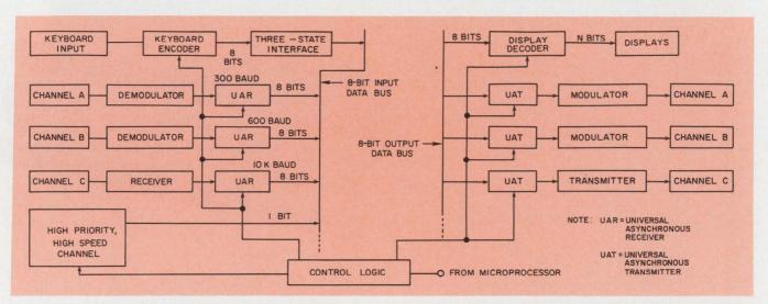
1. The determining factors in the interface design are word length, speed and priority. Transmission of dif-
