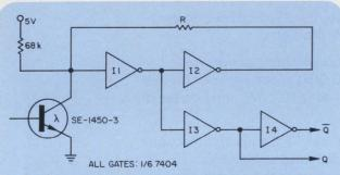
1. Optical Schmitt trigger operates with upper and lower threshold currents determined by resistor R. The controlled hysteresis prevents noise triggering during the time the beam is broken.
