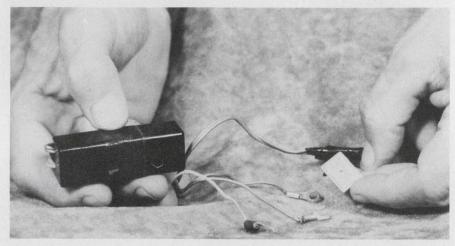
Three-wire bug can be placed in a telephone base and transmit both room and telephone conversations up to 800 feet under good conditions. It measures  $2 \cdot 1/2$  by 1/2 by 1/2 inches and can be installed in five minutes.
