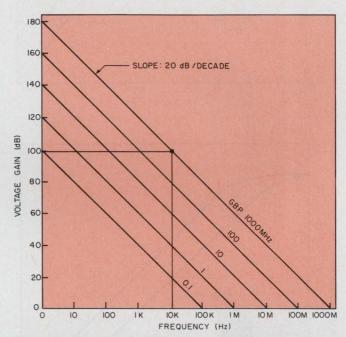
2. Nomogram for estimating required gain-bandwidth product (GBP). Select the highest operating frequency and draw a line equal to the operating gain plus the desired loop gain, both expressed in dB. The intersection of this line with one of the constant GBP curves yields the required amplifier GBP.
