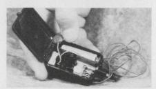
Small, wearable FM transmitter measures 1-1/4 by 2 by 1/2 inches. It operates on 0.5-W power for 1/4 mile. The battery lasts seven days. It's built by Gene Levette.
