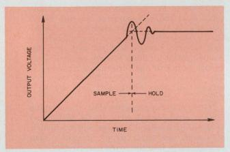
3. By extrapolating the two straight-line segments to meet each other, you can find the effective time at which the hold period starts.
