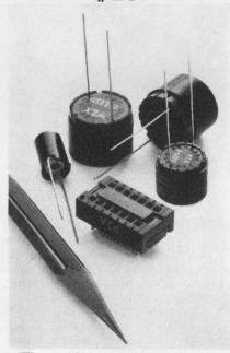
These self-regulating solidstate component temperature stabilizers provide a low cost means of controlling the environment of a wide variety of transistors, diodes, and ICs. Application of these component ovens permits the use of less expensive semiconductor devices by improving their thermal characteristics as much as 30:1. See how much less you get for your money. Less Bulk. Typically 1/10th the size of conventional ovens.
