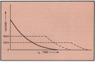
3. Controlled-avalanche rectifiers can keep transients between acceptable limits. Such transients can occur when power to an inductor is suddenly switched off, and can damage conventional rectifiers.
