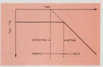
4. If you use a different scope input, the effective point of hold initiation can be found by extrapolating back to the zero point.
