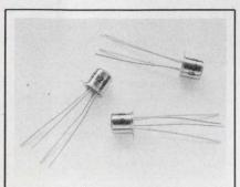
Low noise IF transistors. Type NC-921 and NC 920 have maximum 70 MHz noise figures of 1.2 dB and 1.5 dB respectively when measured in an untuned, broadband amplifier. The NC921 noise figure is typically 1 dB in a tuned amplifier. TO-72 package. California Eastern Laboratories, Inc. One Edwards Court, Burlingame, California. (415) 342-7744.
