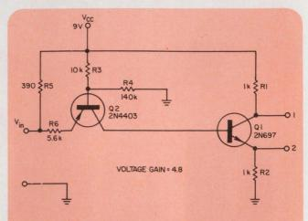
Current source  $\mathbf{Q}_2$  isolates the emitter circuit of phase inverter  $\mathbf{Q}_1$  from the effects of input signal loading. The impedances seen at terminals 1 and 2 are approximately those of their respective load resistors,  $\mathbf{R}_1$  and  $\mathbf{R}_2$ .
