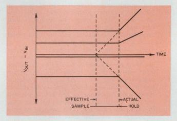
5. The effective start time for hold is not affected by the slope of the input ramp—for a first-order analysis.
