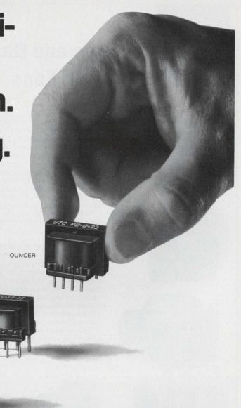
TRW/UTC can help you open up some refreshing solutions to your printed circuit board audio transformer problems. Our Ouncer, Subouncer and Subsubouncer lines, the quality standards for years, are now available with plug-in terminals for labor- and cost-saving board mounting. Leads are designed for wave soldering.
