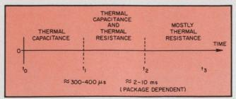
4. Transient duration determines whether the energy must be absorbed by the thermal capacitance of the junction  $(t_0 > t > t_1)$  or by the thermal resistance of the rectifier and its package  $(t > t_2)$ .
