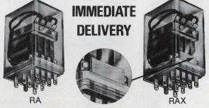
The new RAX relay is an adaptation of the popular RA Type and includes plastic barriers between the movable arms, thereby enabling opposite polarity voltages to be applied to the unit without fear of arc-over.
