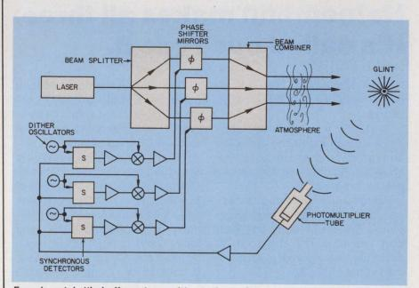
**Experimental "ladar" system** with a three-element array incorporates the Coherent Optical Adaptive Technique to maintain its effective beamwidth. This system has operated over a 100-meter turbulent airpath.
