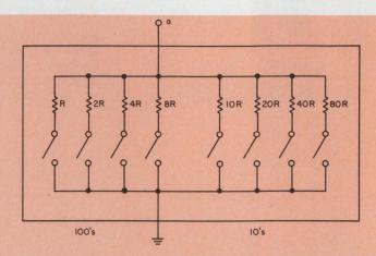
2. Use of binary or BCD-weighted admittances for network N allows the circuit of Fig. 1 to act as a multiplying DAC.
