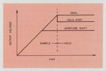
2. Dynamic errors caused by the hold step and the aperture shift are hard to distinguish.
