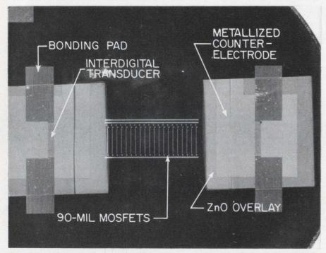
**Experimental surface-wave correlator** is produced by use of piezoelectric zinc-oxide overlay transducers to generate the surface wave in nonpiezoelectric silicon, in which a MOSFET array has been diffused. The MOSFETs detect the surface-wave energy with a detection loss of about 65 dB.
