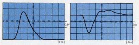
When pulsed laser light strikes the surface of a molybdenum thin film (left), a voltage pulse arises in the plane of the film. When the laser strikes the bottom side of the film through a transparent substrate (right), voltage polarity is reversed.
