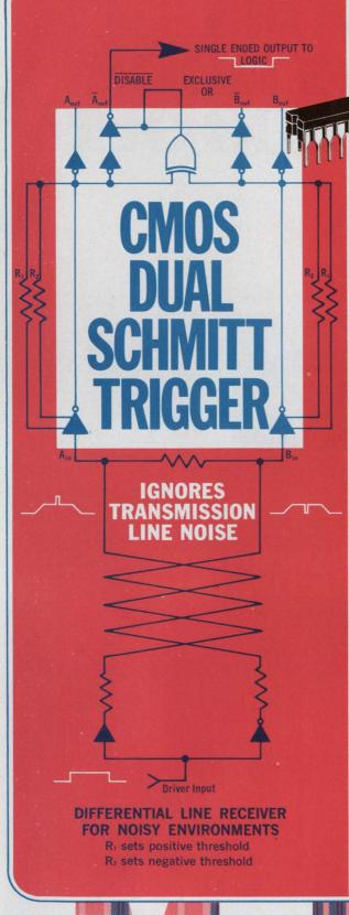
Try any other Schmitt Trigger in this type of application, and short pulses of common mode noise cause false triggering.
