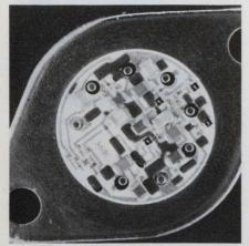
M. S. Kennedy, Pickard Dr., Syracuse, N.Y. 13211. (315) 455-7077. \$125 (1-9), \$112.50 (10-24); stock. The model 850 eight-pin TO-3 hybrid FET amplifier is designed for radar system applications. It has a 1000 V/ $\mu$ s slew rate, a fullpower output to 12 MHz, a unity gain bandwidth of 100 MHz and an output current of 100 mA at ±10 V.
