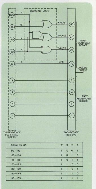
**Two-decade DAC** provides 60% overrange capability, because all possible states of its mostsignificant digit are used. The encoding logic maps the BCD data, as shown.
