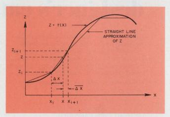
2. Interpolation is a useful technique for providing a limited number of additional decimal places of accuracy between stored values of a function.
