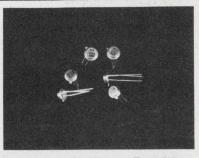
Microwave Oscillator Transistors. NEC types V926 and V020 are in popular TO-46 package, and use gold metallization. The V926 is rated at 400 mV output power at 1.7 GHz and the V020 is rated at 300 mW output power at 2 GHz. California Eastern Laboratories, One Edwards Court, Burlingame, 94010. (415) 342-7744. California, **INFORMATION RETRIEVAL NUMBER 195**
