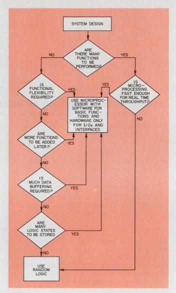
3. Choose between microprocessors or random logic. A flow diagram can be used to analyze the tradeoffs.
