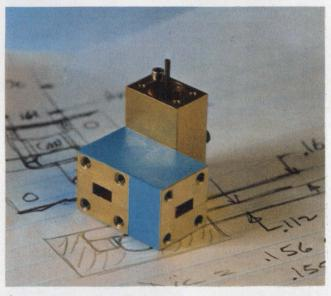
GaAs transferred-electron amplifier from Varian operates at 35 GHz and delivers more than 110 mW with less than 20 mW drive (Session 20).
