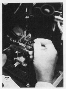
In a special clean room at Fort Monmouth a technician bonds leads to two transducers on a surface-wave dispersive delay line. The device might be used in a radar to determine range resolution.
