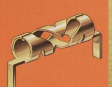
Dual chevron-shaped springs provide positive contact and grip between receptacle and pin, and minimize overall length and diameter of mated contacts. built-in misalignment allowance compensates for wide mounting tolerances. Gold over nickel plating on beryllium copper contacts provides maximum performance reliability in the most critical environments.
