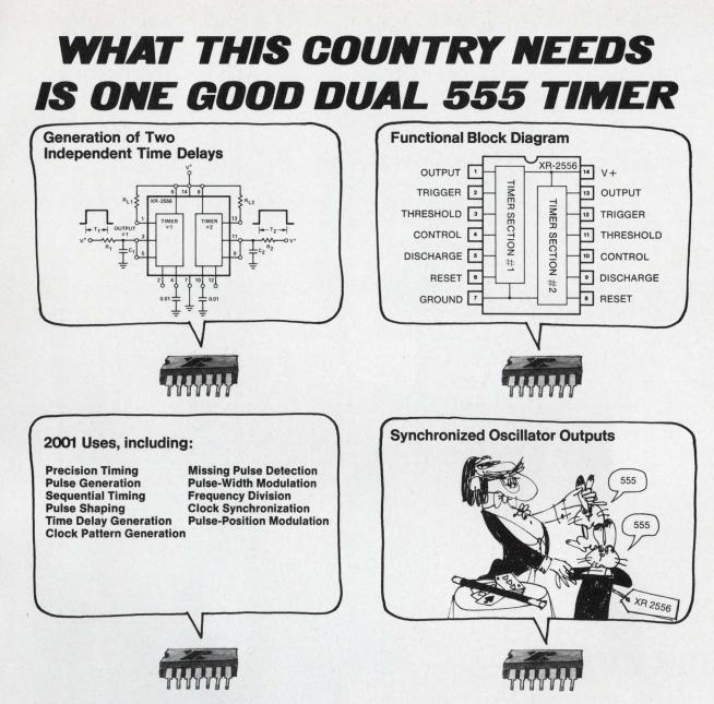
The XR-2556 is a monolithic dual timer IC. It contains two independent 555-type timers on a single chip which exhibit matching and tracking characteristics far superior to those obtainable from two separate timer packages.
