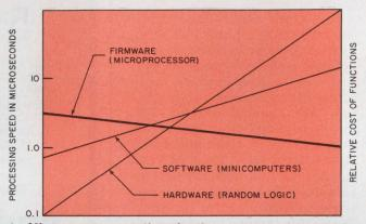
1. Microprocessors offer the lowest cost, but at the lowest speed, with system control provided by firmware. For the highest speed, but at the highest cost, random logic is the way to go. Minicomputers fall between the two approaches in this speed-cost tradeoff.
