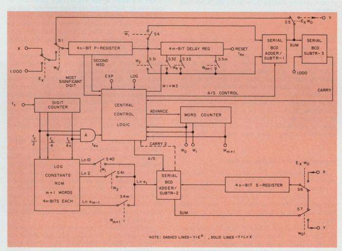
4. With only a short table of iterative constants stored in a ROM, both the logarithm and exponential functions
