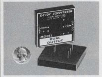
DC/DC converter power supply. 4.5 watts of isolated, regulated  $\pm 15$ VDC,  $\pm 150$ mA from a 5, 12, 24, 28 or 48 VDC Input. Low noise, multiple transformer shielding and 6 sided case shield. No derating required; -25°C to 71°C. Ultra-miniature 2" x 2" x 0.375" module. \$79 (1 - 9). Stevens-Arnold Inc., South Boston, Mass. (617) 268-1170.
