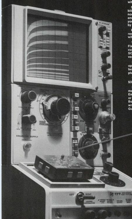
... like letting you view changes in characteristics while you vary operating conditions. As pictured here, the zero temperature coefficient of a junction F.E.T. is easily found by observing the curve that changes least with changing temperature.
