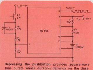
tone bursts whose duration depends on the duration for which the voltage at pin 4 exceeds a threshold. Components  $R_1$ ,  $R_2$  and  $C_1$  cause the astable action of the timer IC.
