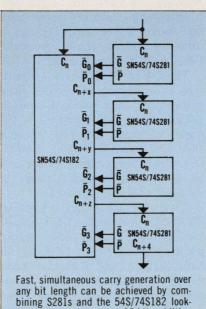
two binary numbers (see above) and can be used in multiples of 4 bits to construct whatever system size desired. It can improve performance, lower costs and reduce board space in "intelligent" terminals, machine/process controllers, minicomputers, and specialized and medium-size main-frame computers.
