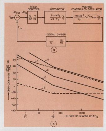
6. In PLL stability analysis, the PLL can be represented by its open-loop block diagram (a). The corresponding Bode-plot is shown in by. The open-loop gain,  $F_{out}/F_{in}$ , varies as a function of the rate of change of  $F_{in}$  in radians per second.
