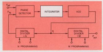
1. Functioning of a phase-locked loop can be best understood from its simplified block diagram.
