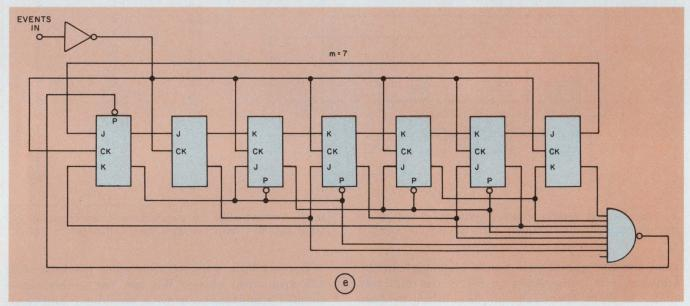
2. Self-correction is added to a residue counter in two ways: by the configuration of its connections and by the
