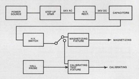
The magnetizing power unit in a typical system charges in as little as 30 seconds and delivers calibration pulses up to 20,000 watt-seconds.
