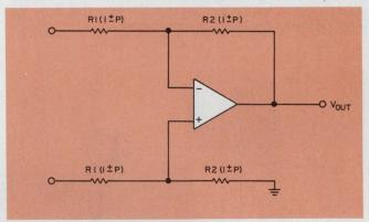
3. Adjusting the resistor ratios to increase gain is extremely difficult when trying to keep the CMRR high.
