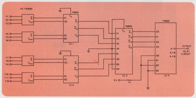
Circuit detects when five out of 12 inputs are true, by examining the binary sum at the output of ICa.
