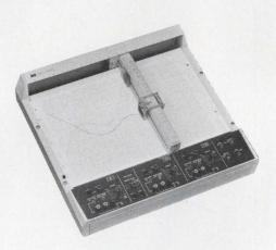
You can plot two signals at once with HP's 7046 high-speed two-pen x-y recorder. Acceleration of the y axis is > 2,500 in/sec<sup>2</sup> (6.3 meters/sec<sup>2</sup>); and on each x axis, 1,500 in/sec<sup>2</sup> (3.9 meters/sec<sup>2</sup>). The y axis pens go from 0 to 30 in/sec (76 cm/sec) in less than 15 milliseconds. Even at these fast speeds, accuracy is ±0.2% of full scale and overshoot is < 1% of full scale.
