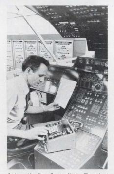
Automatically Controlled Electrical System is being tested in a mockup of the space-shuttle cockpit. The new system moves the power switching location from the cockpit to remote electrical load centers.
