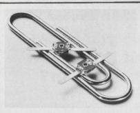
Thin-Trim variable capacitors provide a reliable means of adjusting capacitance without abrasive trimming or interchange of fixed capacitors. Series 9401 has high Q's and a range of capacitance values from 0.2-0.6 pf to 3.0-12.0 pf and 250 WVDC working voltage. Johanson Manufacturing Corporation, Boonton, New Jersey (201) 334-2676
