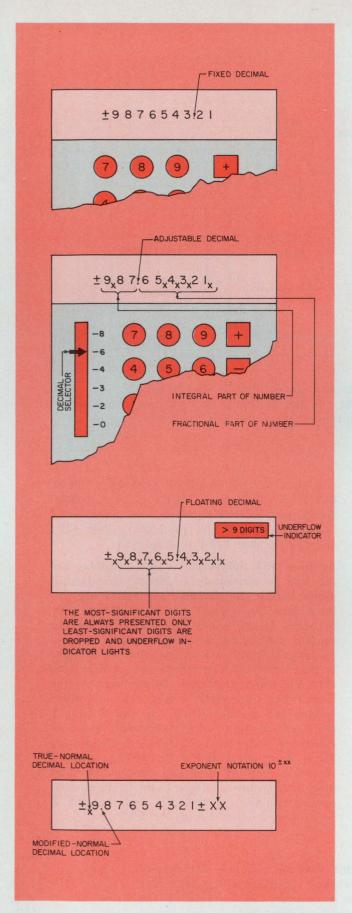
Calculator displays use a variety of methods for handling the decimal point. They vary from the simplest fixed-point system used in accounting machines to the most advanced floating-point and exponential notation methods for scientific calculations.
