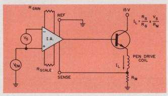
6. A typical general-purpose instrumentation amplifier can be used in chart recorders to cancel out commonmode voltage.
