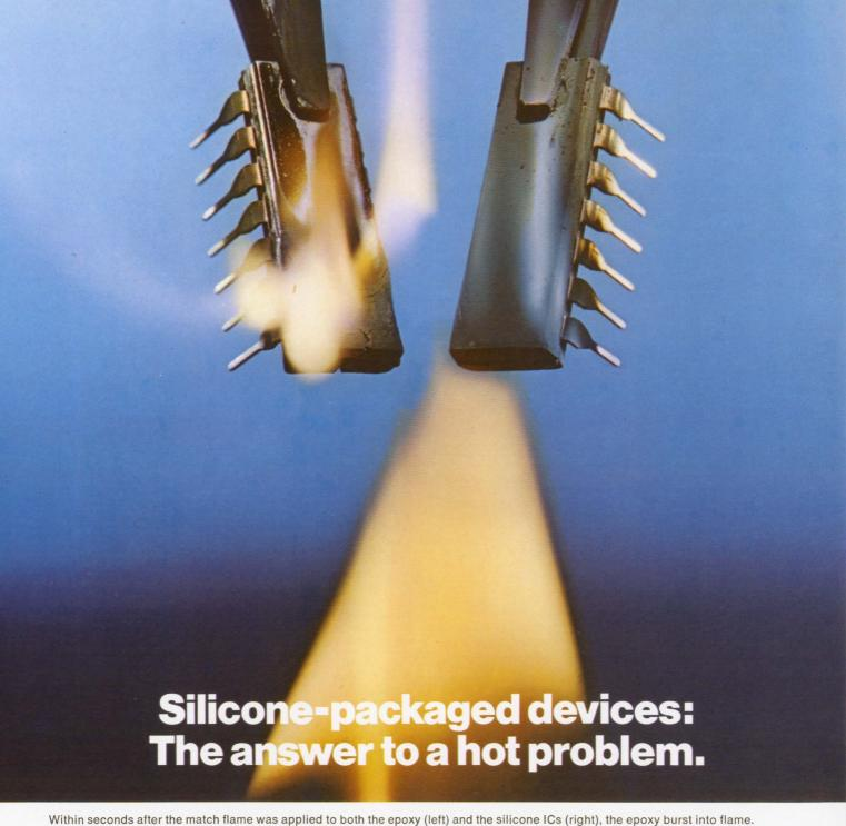
The hot issue in electronics today is flame retardancy. While epoxies and other plastics support combustion, silicone-packaged devices are virtually nonflammable. So, they don't need flame-retardant additives that alter the electrical and mechanical properties of epoxies and other materials.
