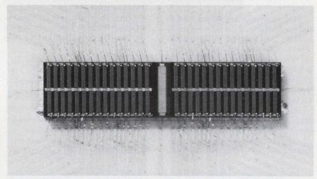
15-bit quadraphase progammable correlator from Motorola is integrated on a wafer of silicon. MOS transistors detect the outputs at the taps. A zinc oxide film is used for the delay line.
