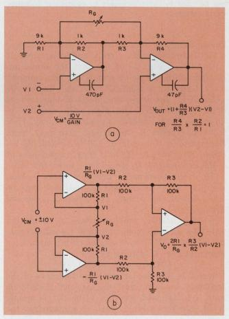
4. Easier gain adjustments are possible with a dual opamp circuit (a) and a triple op-amp circuit (b), but at the expense of higher noise, drift, instability and cost.
