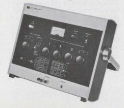
quality factors to 5% accuracy. The measuring frequency is 1 kHz; other frequencies (50 Hz to 10 kHz) can be obtained with an external oscillator. Results appear on a four-digit display.
