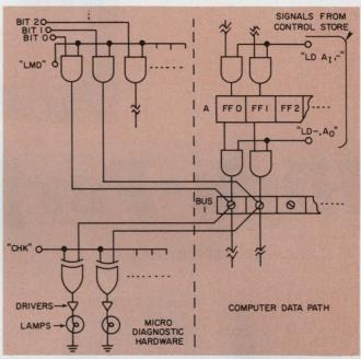
3. Microdiagnostic hardware permits direct examination of a register by intercepting and displaying the signals on the bus that serves the register. Signals from the control store load the requisite test patterns. The Exclusive-OR gates compare the actual pattern with the theoretical.
