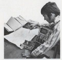
The 1710A scope is fast enough to test ECL, as shown here.
