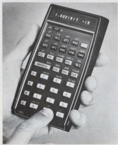
rarely found even on large machines: n factorial, percentage and % difference, mean and standard deviation,  $x^2$  and 10, and polar-rectangular coordinate conversions. It's easily the most powerful scientific calculator of this size or price.
