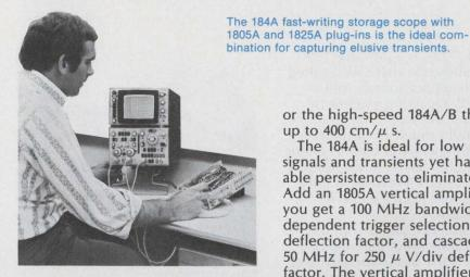
or the high-speed 184A/B that writes up to 400 cm/ $\mu$  s. The 184A is ideal for low rep rate
