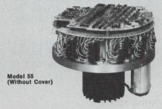
DATUM Series 55 Drum Memories provide 262K 16-bit word capacity with 72,000 bits per track on 64 tracks. Access time averages 16.6 milliseconds.
