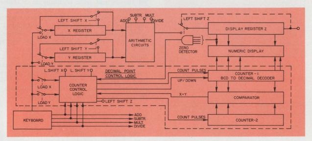
A floating-point calculator automatically keeps track of the decimal with the help of the decimal-point key on the keyboard. The routines performed by the circuit are different for each of the four arithmetic operations, thus:
