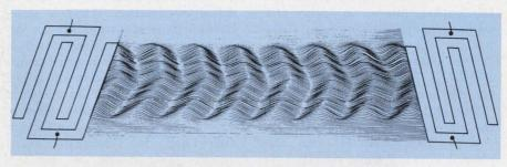
Basic interdigital electrode patterns for excitation and detection of surface acoustic waves on a piezoelectric substrate. The surface-wave pattern shown was derived from voltage-probe measurements at the Lincoln Laboratory.
