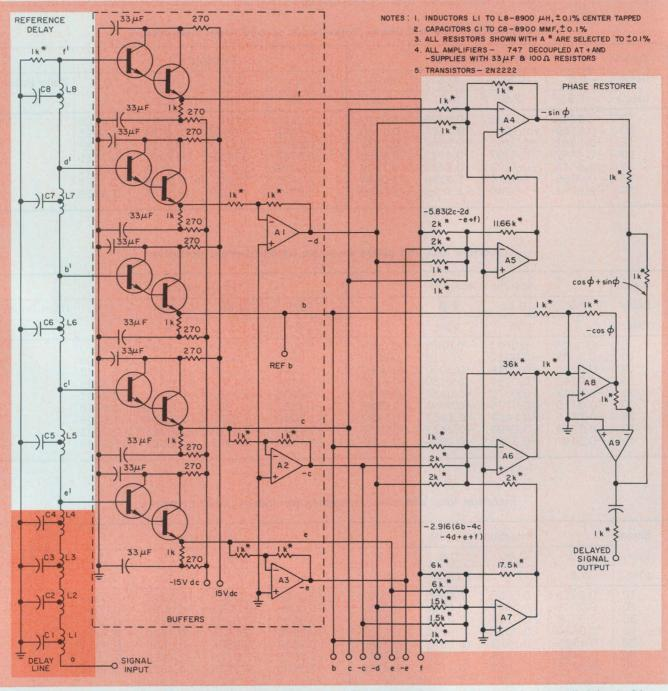
4. Practical fifth-order network maintains the output phase to within -2 to +3 degrees of the input signal.
