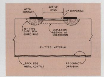
2. The graded guard-ring structure is used for silicon and germanium APDs. Junction-edge breakdown is eliminated by the guard-ring concentration and curvature.
