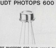
UDT PHOTOPS 600 high speed detector/amplifier combination has response to 10 megahertz with sensitivity to 5 x 10-12 watts. All PHO-TOPS utilize latest FET circuitry and are available to Icm<sup>2</sup> active area. PHOTOPS may be used as replacements for photomultipliers. United Detector Technology, Inc., 1732 21st Street, Santa Monica, CA. **INFORMATION RETRIEVAL NUMBER 185**
