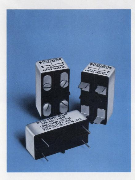
The new 601-1400 series features LED optical isolation and synchronous/zero voltage switching to virtually eliminate RFI for any resistive or reactive load, up to 10 amps steady state. 1000% surge current capability assures maximum reliability without derating for the toughest loads — lamps, solenoids, motors, transformers, etc. High dv/dt rating assures maximum output transient immunity. The sensitive control input is TTL compatible, accepting drives from 3 to 32 VDC.
