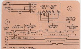
With a shift register connected for sync separation (a), the vertical sync pulse appears shortly after the start of the vertical interval (b). ONEs entering pin 1 and clocked toward  $Q_{\rm D}$  reach  $Q_{\rm B}$  during the long serrated pulse interval. ZEROs from pin 5 are clocked toward  $Q_{\rm A}$  when the composite sync signal is high.
