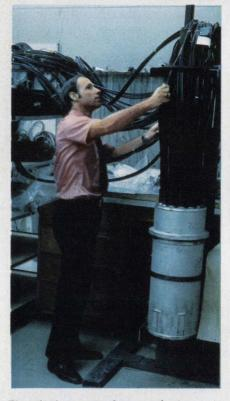
**Electrical penetration conductors** at Gulf take data from sensors inside a reactor's core through the containment wall to a display.
