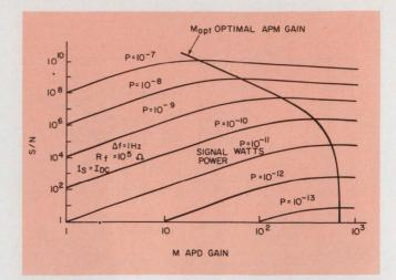
6. The variation of S/N vs APD gain at different light power levels for the TIXL 56 at  $\lambda = 632.8$  nm. Since M is a highly nonlinear function of bias voltage, these curves are altered from the curve in Fig. 1.
