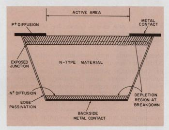
3. The exposed junction structure is used in silicon APDs. Here breakdown problems are eliminated by removal of the curved portion of the pn-junction.
