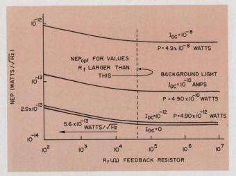
7. Feedback resistance vs NEP variation for different background light levels. In general, the value of R<sub>f</sub> doesn't depend on the background light. The NEP improves with larger R<sub>t</sub> values up to a value of 5  $\times$  10<sup>4</sup>  $\Omega$ .
