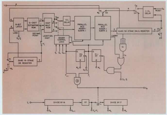
4. Table look-up methods and a bit-parallel configuration provide an order-of-magnitude increase in speed in this
