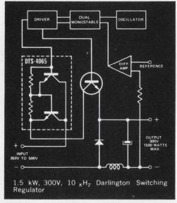
in circuit design where dc drive conditions may have created awkward problems when using SCR's.
