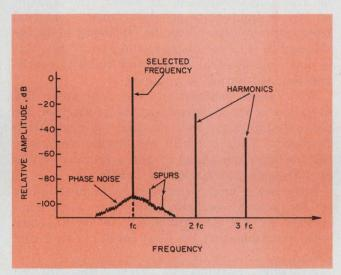
1. A synthesizer's output contains unwanted components in addition to the carrier. The unwanted signals can be separated into harmonics and spurious components, with phase noise often dominating close to the carrier.
