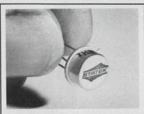
Crystal oscillators in TO-5s or flat paks. Standard versions 10 kHz to 250 kHz (low as one cycle per month available). TTL, DTL, RTL and CMOS compatible. They're rugged, accurate & highly resistant to shock & vibra-tion. Write or call for literature. STATEK CORP., 1233 Alvarez Ave., Orange, Calif. 92668, (714) 639-7810.
