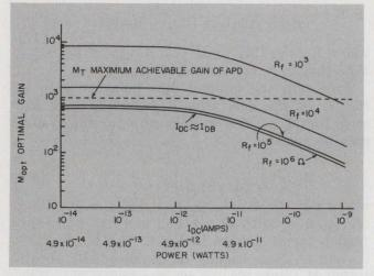
8. Optimal system gain exceeds the maximum achievable gain for certain values of feedback resistance. Above  $M_{\rm T}$ , the APD becomes excessively noisy.
