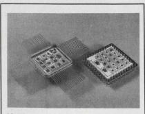
Multi-chip "MSI" custom arrays, built to complete MIL-STD-883 specs. are available in 9-12 weeks ARO. Complex digital circuits using TTL, MECL, CMOS, or PMOS logic are packaged in planar or plug-in flatpacks as shown—up to 25 devices in a 1.25" sq. and 20 devices in a 1.0" sq. J. W. M. Corp., 4901 Stenton Av., Phila., Pa. 19144.
