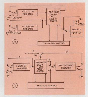
1. The general organization of a single-precision divider (a) can be converted to a double-precision divider (b) if the functions of the dividend register, DR, are combined with the Q register to form a DN/Q double-length register to hold both quotient and dividend.
