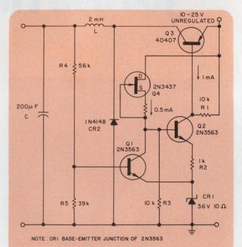
Switching regulator uses low-hysteresis Schmitt trigger ( $Q_1$  and  $Q_2$ ) to drive switch  $Q_3$ . Switching action occurs when the voltage across divider  $R_4$  and  $R_5$  goes above or below the trigger point.
