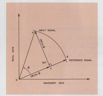
2. **Orthogonal phasors** derived from the delayed reference signals serve to reconstruct the input signal. One of the phasors is parallel to the phasor representing the signal input to the reference network.
