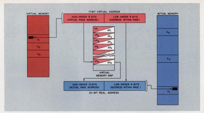
Xerox's virtual-memory system maps virtual program addresses into as many available real memory slots as possible. Tight packing of main memory minimizes the amount of program swapping and enhances multimode operations like time-sharing, data-base inquiry and real-time control.
