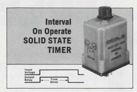
Timing period begins when input voltage is applied and internal control relay age is applied and internal control relay energizes. Control relay de-energizes at the end of time delay period. Time delay resets when input voltage is removed. If the input voltage is removed before timing period is completed, control relay de-energizes and time delay resets.
