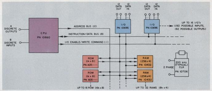
Rockwell Microelectronics' parallel-processing system uses the 10660 central processor, which has a basic instruction cycle of only 5  $\mu$ s and a 50-instruction set repertoire. Data can be handled internally at four times the rate of the external clock; the processor divides the
