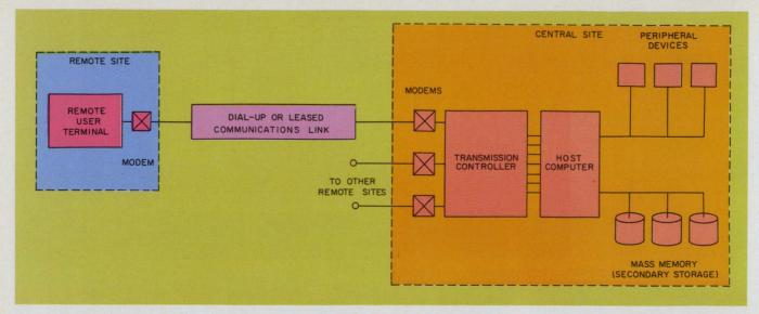
The modem is a basic interface device at both ends of a data link between a central computer and a remote
