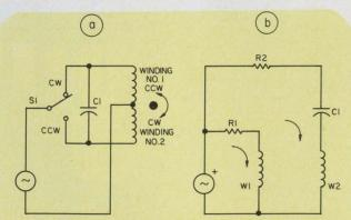
1. A bidirectional ac motor (a) has a capacitor,  $C_1$ , which creates a phase difference between the currents in the two windings, as shown in the equivalent circuit (b). Conventional dc braking won't work with this type of motor.
