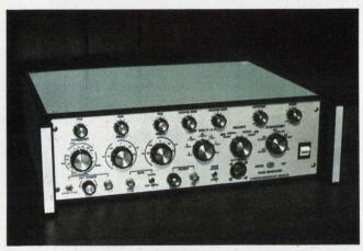
E-H Research Laboratories' Model 137 features a rep rate of 100 MHz, variable rise and fall ramps from 0.5 ns/V to 40  $\mu$ s/V and variable baseline offset to  $\pm 5$  V. Delay and width are also variable.
