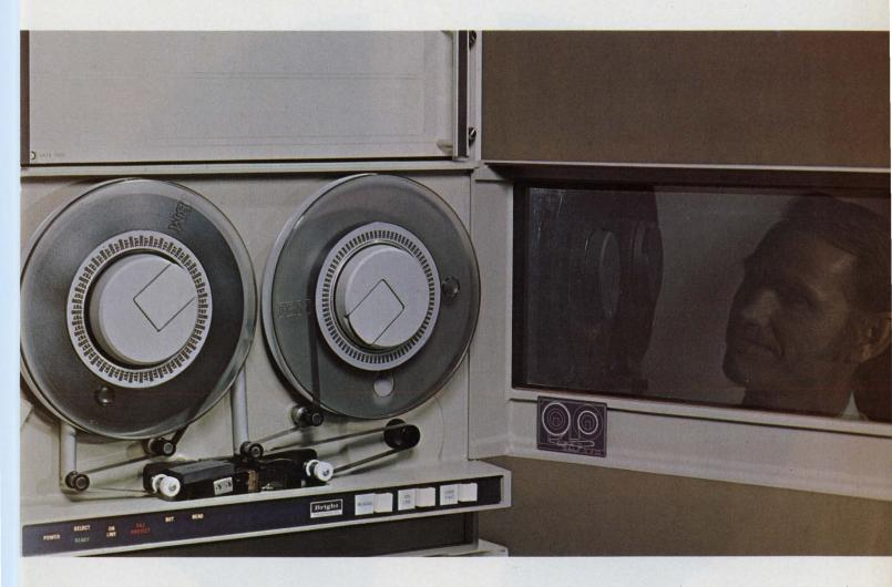
Look closer. The cover frame is cast of solid aluminum. So is the deck panel.
