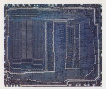
American Micro-systems' proposed 7200 system consists of a three-chip central processor, including this micro-control chip. Another chip provides registers and an ALU, and the third—a microinstruction chip—contains the microprogram in a 512-word-by-24-bit ROM. All three ICs are ion-implanted, p-channel devices.
