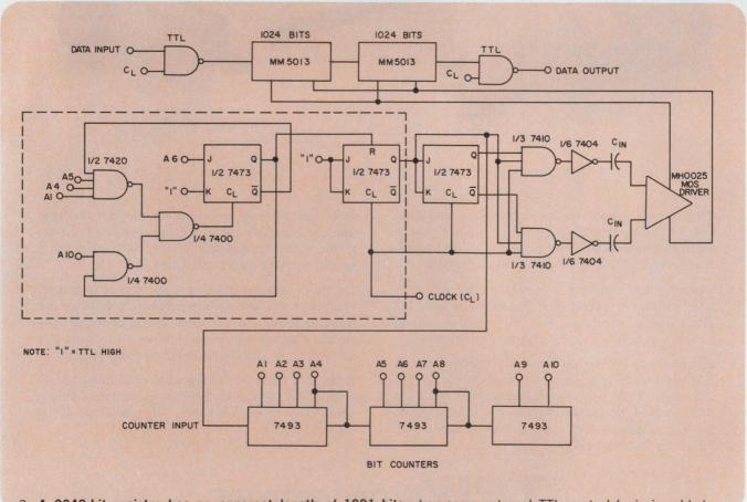
2. A 2048-bit register has an apparent length of 1991 bits when some external TTL control logic is added.
