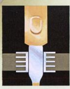
Solder band is pulled into through-hole with just enough force to retain it during reflow.
