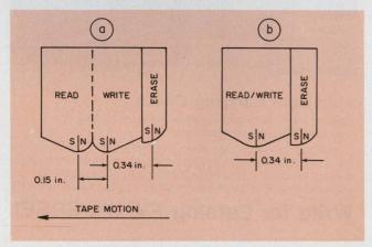
2. Turning off write and erase currents on a dual gap head (a) must be done immediately after the last character is written because of an additional distance that the tape must travel to reach the read gap. Slower turnoff can be tolerated in a single-gap head (b).
