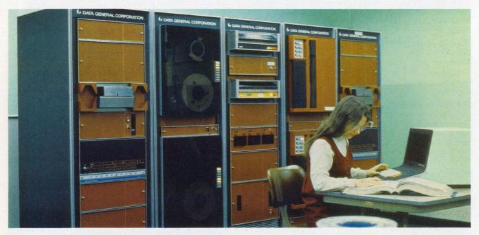
A variety of peripheral equipment is used in this dualprocessor system from Data General. Included in the system are two Nova 1200 computers, three on-line disc
