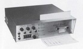
Helena Laboratories is using an Intel micro computer in an instrument that measures the protein content of blood, printing a separate quantitative reading for each of several different proteins.
