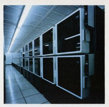
Ampex's terabit memory system has a capacity of 3  $\times$  10  $^{12}$  bits and an access time of 10 s.
