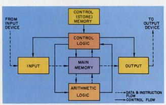
2. The microprogrammed computer uses an additional control memory in which the program elements are stored. These elements carry out the instructions.
