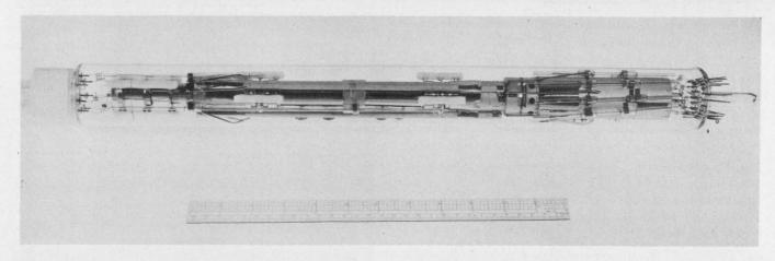
The storage tube used in Micro-Bit's beam-addressable storage system can store a million bits of data. Data
