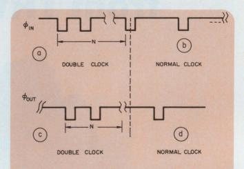
1. Doubling the input clock rate allows artificial shortening of shift registers. The input clock is doubled for N periods (a) and then returns to the normal frequency (b). The output clock (c and d) follows the same patterns.
