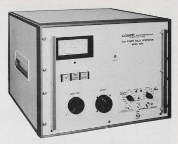
A peak of 24 kW is obtainable from the 605P, Cober Electronics' high-power pulse generator. Minimum width of the 11-A, 2.2-kV pulse is 50 ns.
