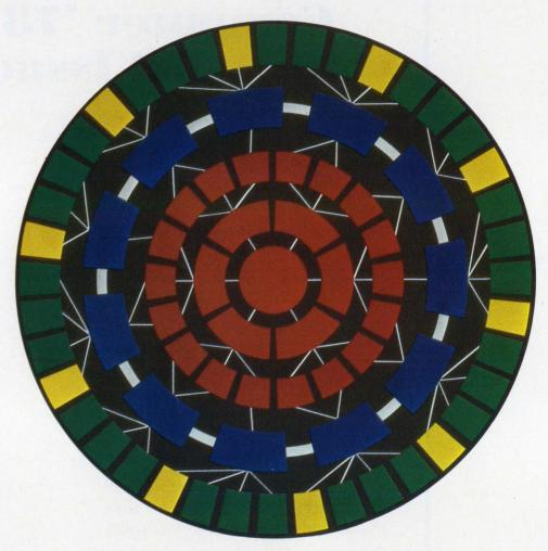
Symbolic concept of General Electric's Mark III Information Services Network. Outer ring of blocks represents low-speed remote concentrators. Blue colored blocks represent high-speed data concentrators. The third ring depicts preprocessor computers. Next ring performs batch processing. The central circle features "future massive storage devices."
