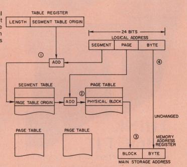
megabytes of virtual storage into the smaller domain of real storage. Mapping maintenance is done by the software portion of the package—the control program.
