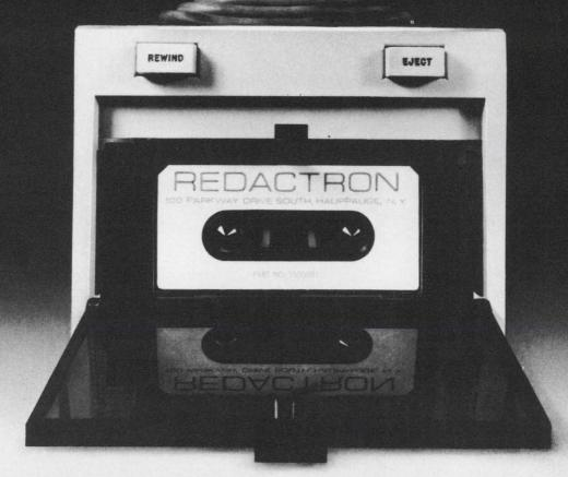
Our Cassette Transport has no pinch roller, capstan or servo system to clean, maintain or cause problems. We've shifted the burden of tape speed regulation from mechanics to electronics ... and you get added reliability at a lot less cost.
