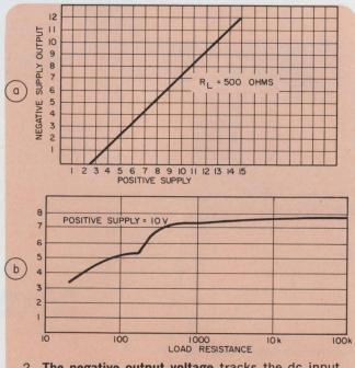
2. The negative output voltage tracks the dc input voltage linearly (a), but its magnitude is about 3 V lower. Application of a 500- $\Omega$  load (b) causes a 10% change from the no-load value.
