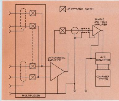
2. A multiplexer can rapidly scan many thermocouples and reference-junction temperatures at rates far greater than a junction can significantly change its temperature to allow accuracies within the thermistor's capability. Low-level signals obtained from thermocouples and thermistors require careful attention to the details of proper grounding and shielding of the scanning and measuring equipment, especially in electrically noisy environments.
