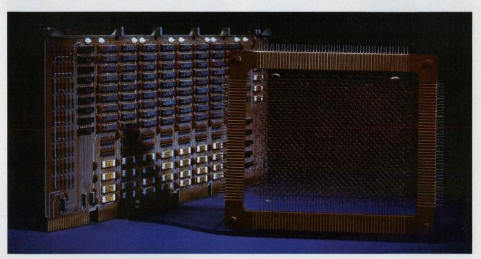
MOS semiconductor memory card (left), made by Digital Equipment, can store about 10 times more data than the Honeywell core plane (right). In addition to the increase in
