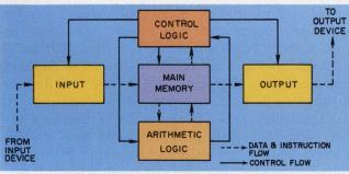
1. The architecture of the basic single processor is derived from the configuration of its five elements: the input, the output, control, memory and arithmetic unit.
