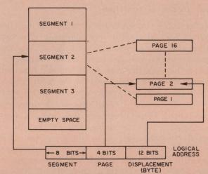
1. Virtual memory is divided into pages and segments. Logical addresses specify a location in virtual memory by segment, then by page number and, finally, by displacement within the page.
