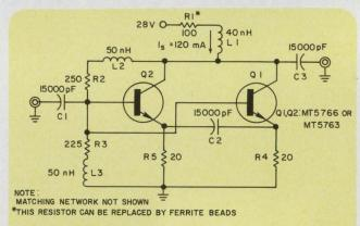
Replacing the 100- $\Omega$  resistor with ferrite toroids in this amplifier increases the efficiency. The circuit provides 6-dB power gain from 50 to 500 MHz.
