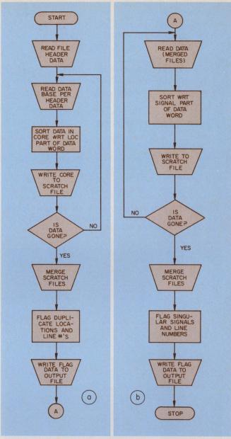
3. Sorting by node location permits detection of multiple assignments to a single terminal (a), whereas a sort by signal name reveals unwired terminals (b). Subfiles are sorted and merged to form the central data base.
