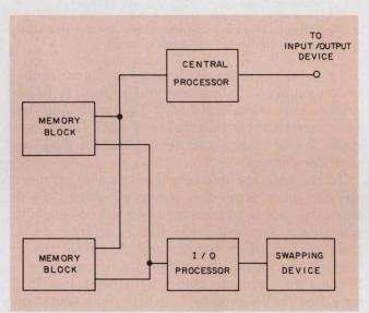
Independent overlapped operation is a characteristic of an asynchronous system design. It greatly improves efficiency and processing power by having the CPU execute a program in one memory block while programs are exchanged with the other block.
