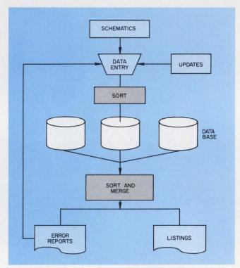
1. Entries based on the wiring schematics are sorted and placed in a central data base. Sort and merge operations array the data in requisite report order.
