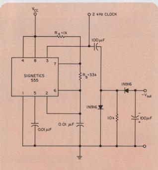
1. Transformerless dc-dc converter derives a negative supply voltage from a positive. As a bonus, the circuit also generates a clock signal.
