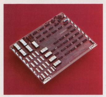
National Semiconductor offers a 16-bit microprocessor on a card, the IMP-16C. Included on the card: clock system, I/O bus drivers, 256 words of RAM and provision for 512 words of ROM or pROM. The card has one control ROM that stores the microprogram and provides the logic for four 4-bit register-and-arithmetic-logic units.
