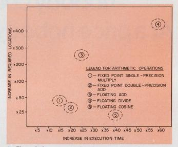
1. The relative computational power of a typical largescale computer and a 12-bit mini with a minimum hardware-instruction set. The required number of instructions and the execution time of the large computer are taken as unity and other data are normalized.
