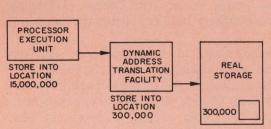
2. Real-storage addresses required by the processor execution unit are derived from the program's logical, or virtual, addresses through the DAT translator.
