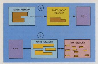
3. A main computer memory may appear to be faster or larger than it really is. A fast semiconductor cache memory between the main memory and the CPU (a) gives the main memory the apparent speed of the cache memory. Keeping track of data and swapping it into and out of the main memory onto an auxiliary memory (b) makes the main memory look substantially larger than it is.
