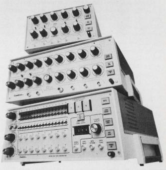
A range of generators are offered by Comaltest. From top, are the 610, a 2-phase unit; the 601, a 4-phase unit; and the 801, a 16-channel data generator.
