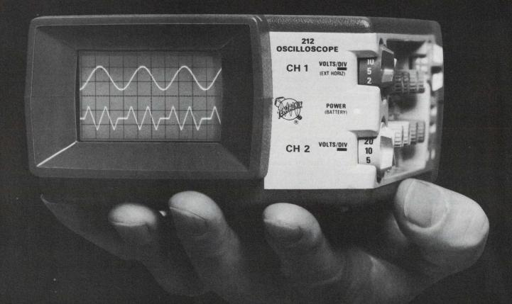
With the 212. A completely new DUAL-TRACE, 500-kHz, 3 x 5½ x 9-inch scope that weighs only 3.4 pounds and costs just \$725. The high-impact plastic case withstands severe environments — double-insulated construction protects you while floating the scope to make high-voltage measurements.
