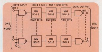
3. Use of the double clocking technique reduces the package count of an equivalent register from 24 to 16. It also saves the cost of ordering a custom-masked MM5019 register.
