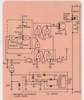
Initiation of load power occurs at a precise point on the ac waveform after depression of  $S_1$ . The controllable-pulsewidth of  $MM_1$  ( $R_1$ ,  $C_{1A}$ ,  $C_{1B}$ ) determines the moment  $FF_2$  is latched and the triac gated on.
