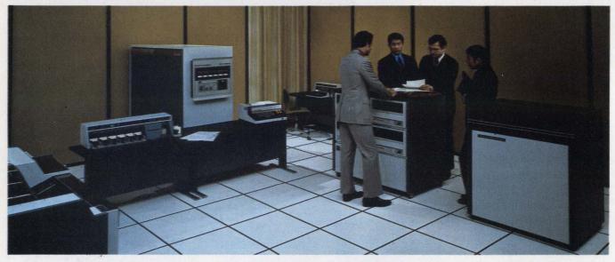
Variable micrologic alters the run-time environment according to the language processed in the Burroughs B1700 series. The system runs Cobol, Fortran, Basic
