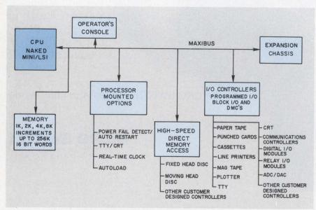
**Double-bus structure** allows different types and speeds of memory to be used together without any special software. The bus allows direct addressing of up to 248 I/O devices. The 162 element instruction set is implemented by internal microprogramming.
