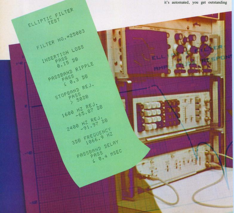
data repeatability along with the dramatic speedup in testing rate. Use it to fully test such time-takers as active filters, crystals or op amps. You can do them in seconds or minutes instead of the usual hours or days.
