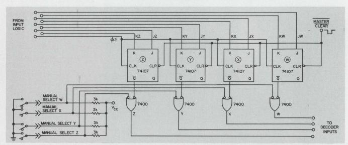
9. The Sequence-Events flip-flops derive their inputs directly from the Input-Logic circuit's outputs. Note the extra features for checkout of these flip-flops. To use
