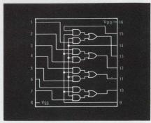
Pin for pin compatible with CD-4019A. 100-999 units
