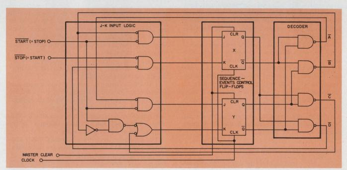
3. Three basic circuits—the J-K Input logic, the Sequencer-Event logic and the Decoder—implement the
