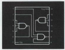
Pin for pin compatible with CD-4023A. 100-999 units
