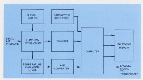
Output of vibrating transducer in new altimeter is digitized by feeding it to a counter. From the counter the signals are fed into an LSI computer that solves a pressure-temperature equation for altitude.
