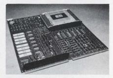
15-by-16-inch printed-circuit board contains an entire minicomputer, including 4-k, 16-bit words of core memory. The large packages on the left side of the board contain the central processing unit and microprogram control on silicon-gate MOS/LSI circuits.
