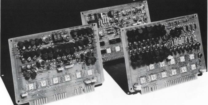
Kearfott can solve your synchro-to-digital and digital-to-synchro conversion problems with three production model solid state converters. All three meet MIL-E-5400.\*
