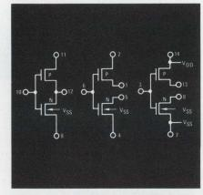
Pin for pin compatible with CD-4007A. 100-999 units
