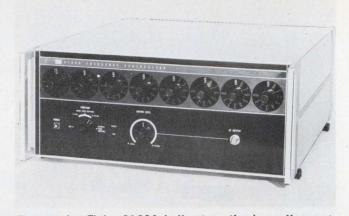
The popular Fluke 6160A indirect synthesizer offers output to 160 MHz, BCD programming with 0.5-ms switching time, and a signal-to-phase-noise ratio of 62 dB.
