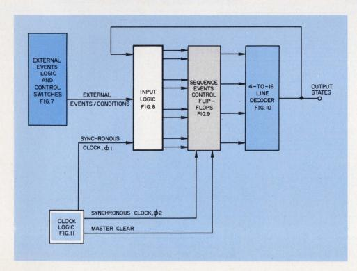
6. The a/d controller block diagram has two circuits not needed in the simple example of Fig. 3—the external-events logic and a two-phase clock.
