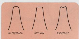
2. Typical filter output response with various amounts of feedback. The range of magnitudes plotted represents 40 dB, and the fractional 3-dB bandwidth is about 2.5%.
