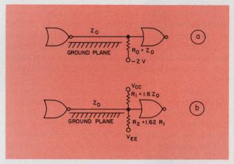
2. Terminations can eliminate reflections. The possible termination techniques include resistor  $R_o \approx Z_o$  connected to a termination voltage (a) or the use of an equivalent resistor network (b).
