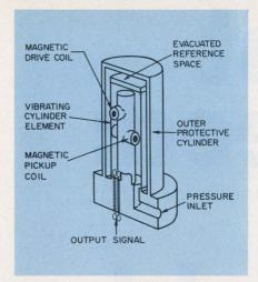
Key to the new all-electronic altimeter is Hamilton Standard's digital pressure transducer. The pressuresensing element is a cylinder that is driven magnetically to vibrate at its natural frequency of about 4 kHz. As the static air pressure increases, internal forces increase the stiffness of the sensing element, increasing the frequency in proportion to the change in pressure.
