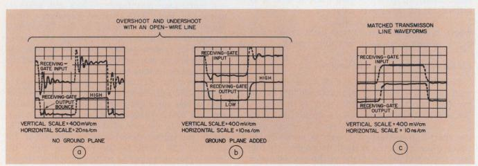
3. Waveforms show reduced ringing when a ground plane is used (a and b). Further improvements are ob-
