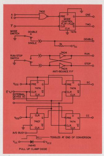
7. External events such as the external device signal clock (SC) and the a/d Busy signal, must be temporarily stored and then strobed synchronously into the sequencer by clock  $\phi 1.$  The four external-events store flip-flops are cleared when state C occurs. The external EOC signal goes directly to the input logic circuits from the computer, since it always occurs and stabilizes before it is needed by the sequencer.
