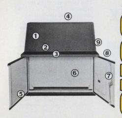
1. 24", 36", 48", or 60" width. 2. Hinged sloping control panel. 3. Optional writing desk. 4. Instrument panel top available. 5. Neoprene gaskets for complete oil tightness. 6. Accessory subpanel. 7. Three-point latches and key-locking handles. 8. Doors on both front and back. 9. All seams continuously welded. 10. NEMA-12 construction. 11. Many modifications available. Write for Bulletin C-14.
