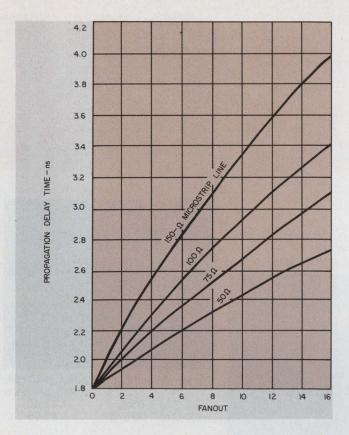
4. Low-impedance lines also result in reduced delay times, or higher speeds. Curves show the propagation time for a 12-inch lump-loaded microstrip line as a function of fanout.
