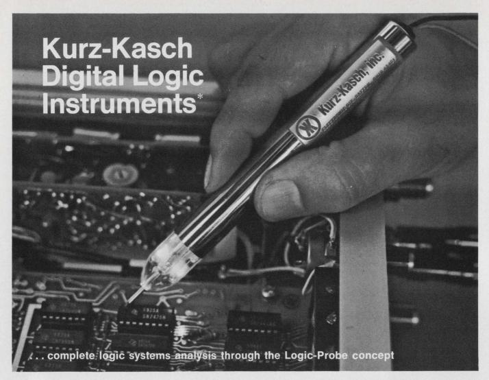
Rugged, all solid-state, Kurz-Kasch logic probes are designed for fast, accurate testing of logic levels in all types of integrated circuit systems. A simple readout system indicates "true", "zero", or "pulse" readings precisely through color-coded visual electronic readouts in the probe tip. Absence of logic levels is indicated by all readouts remaining OFF.
