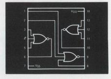
Pin for pin compatible with CD-4025A.
