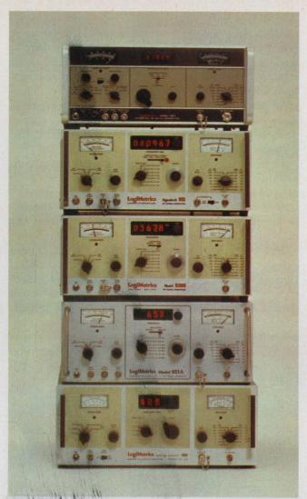
Logimetrics sig gen line ranges from the 750A, a 520-MHz unit with five-digit readout, to the 921A, an 80-MHz unit with a three-digit display.
