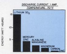
Energy from one lithium D cell at a 1-A discharge is equivalent to four mercury zinc cells, five alkaline manganese, seven magnesium and 30 carbon zinc cells.
