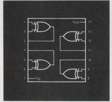
Pin for pin compatible with CD-4030A.
