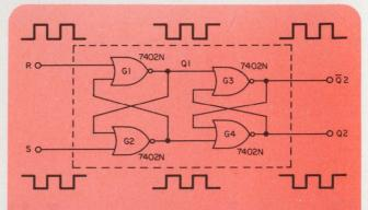
1. Circuit with two cascaded, set/reset flip-flops rejects common-mode spikes of either polarity. Each flip-flop separately rejects negative-going spikes but inverts positive spikes.
