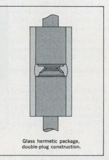
Designated 1N4001 through 1N4006, the 1-amp devices offer a reverse voltage range of 50 to 800V. Repetitive peak forward current (10 cycles, 75°C or below) is 10 amps. Peak surge current is 30 amps. Static reverse current is 10 microamps at 25°C and 50 microamps at 100°C.
