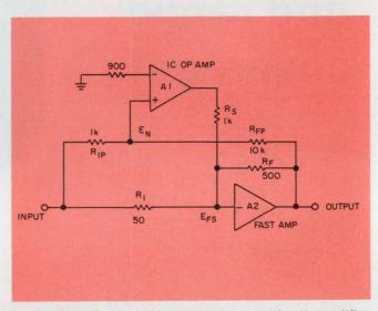
1. Junction  $E_{\rm FS}$  is held at zero by the "fast" amplifier for the first 100 to 200 ns. Then the IC op amp begins to make the final corrections with its high open loop gain.
