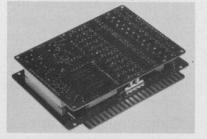
GOOD SPEED AND STABILITY. ADC700 Series. 6.5 Microseconds for 12 bits, 3.5 Microseconds for 8 bits. Up to 0.025% full range accuracy and ±10 ppm/°C stability. Voltage switching attains high conversion speed without sacrificing accuracy. Series includes six repairable models. Many options, modifications for special applications. If it's stability, accuracy, speed, or all-around quality performance you need in Data Conversion, contact Phoenix Data *now*!
