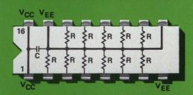
SERIES 898-42 -5.2 VOLT TERMI-NATORS contain twelve resistors for pull-down to the -5.2 volt bus. Each unit contains a 0.01  $\mu$ F decoupling capacitor to bypass the -5.2 volt bus. Price (1,000-4,999) \$1.25
