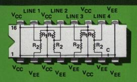
SERIES 898-43 THEVENIN EQUIVA-LENT TERMINATORS contain four Thevenin equivalent terminator sections. Each terminator section consists of two resistors connected as a divider from the ground bus to the -5.2 volt bus providing a Thevenin equivalent voltage of -2.0 volts. Each unit contains a 0.01  $\mu$ F decoupling capacitor to bypass the -5.2 volt bus. Series 898-43 units are available with Thevenin equivalent impedances of 50, 75, and 100 ohms.
