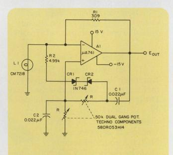
**Waveform purity at low frequencies** for a Wien bridge oscillator is enhanced by diode limiting. Lamp L<sub>1</sub> stabilizes the loop gain at higher frequencies while the limiting action of  $R_2$ ,  $CR_1$  and  $CR_2$  prevents clipping at low frequencies.
