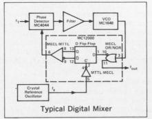
means to generate frequencies up to 250 MHz without the use of tuned circuits. The output frequency can be either a single fixed frequency or a series of programmable frequencies.
