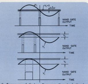
2. Sequence of timing diagrams (top to bottom) shows the NAND gate output voltage as  $V_r$  is progressively raised from zero (top frame) to the height  $V_i$  of the sine wave input.
