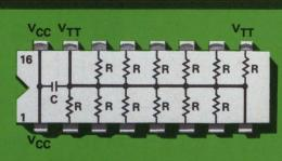
SERIES 898-41 - 2.0 VOLT TERMINA-SERIES 35-41 – 2.0 VOLT TERMINA-TORS contain eleven resistors for ECL line termination to a –2.0 volt bus. Each unit includes a 0.01  $\mu$ F decoupling capaci-tor to bypass the –2.0 volt bus. Standard R values of 50, 75, and 100 ohms are avail-able and are designated 898-41-R50, 898-41-R75, and 898-41-R100. Price (1,000-4,999) \$1.25
