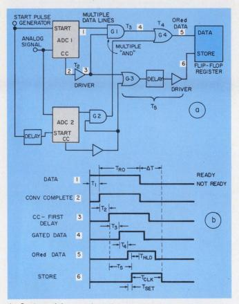
4. System delays rather than actual hardware are emphasized (a). The CC signal (b) gates the a/d output data and generates the Store signal. Data to the register are delayed by arrival of the CC signal at gates  $G_1$ , while the generation of the Store signal is delayed by the driver and composite delays  $T_5$ . Other circuit requirements include the register setup time ( $T_{\rm SET}$ ), data hold time during clocking ( $T_{\rm HLD}$ ) and a minimum clock signal duration at the store input.
