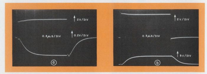
5. With improper adjustment of  $R_N$ , the amplifier output (top trace) shows a slight droop (a) or overshoot (b).
