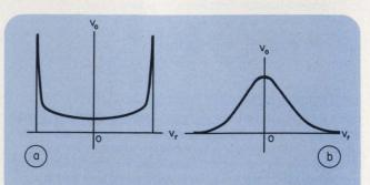
3. Sample outputs from a sine wave input (a) and amplified resistors noise (b) as a function of  $V_r$ , show excellent agreement with the corrsponding theoretical probability density functions.
