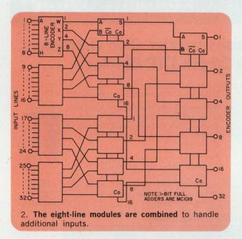
For a greater number of input lines, multiple groups of eight-line encoders can be combined, as shown in Fig. 2.
