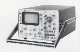
All 1700B scopes have a new color-coded front panel for easier operation.
