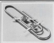
Thin-Trim® variable capacitors are designed to replace fixed tuning techniques. Applications include crystal oscillators, CATV amplfiers, communication and test equipment. Series 9410 has high Q's with five capacitance ranges from 1.0 - 4.5 pf to 10.0 - 50.0 pf. Johanson Manufacturing Corporation, Boonton, N. J. (201) 223-2676
