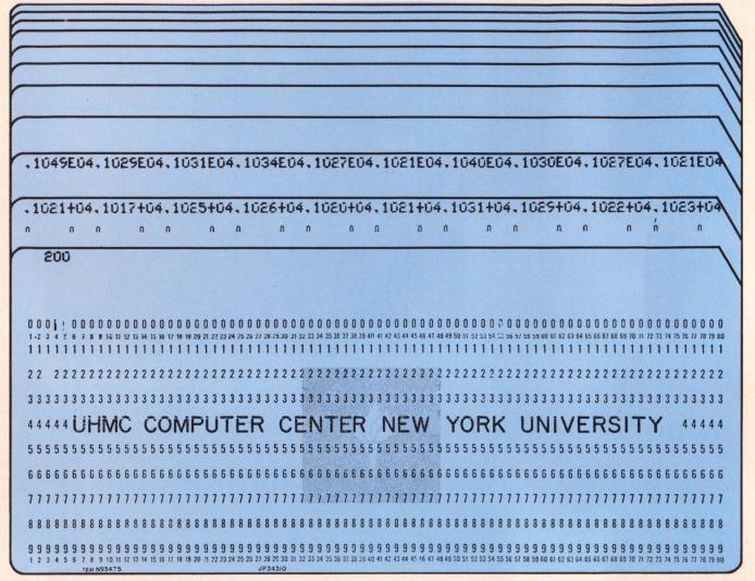
Each data card contains 10 measurement values in E8.4 format. The first card contains the number of measured values in I5 format. This sample deck shows the values punched for the first 10 measurements.
