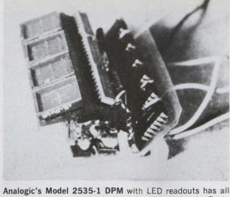
Analogic's Model 2535-1 DPM with LED readouts has all of its circuitry on a single flexible printed circuit. Packaging is thus greatly facilitated.
