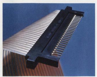
Laminated flat-conductor cable from AMP, Inc., comes preterminated for easy installation.
