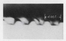
2. The steps in forming a thin-film optical waveguide (above) lead to a guiding structure that has center-to-center spacing of 4100 Å (below).
