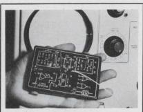
COS/MOS Pulse Generator—Features Squarewaves 1Hz-1MHz/Pulsewidths |<sub>µ</sub> - .1 sec./"D" FF with S & R/Non-Capacitive Differentiator/Level Detector/"De-bounced" Push button. Q & Q outputs and complementary inputs available all functions. 3 - 15V circuit supply. Ideal as bench and built-in test equip. \$125. American Laser Systems. (805) 687-1212
