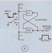
1. Clock-pulse counts up to 512 can be obtained with this circuit (a). Larger pulse counts can be obtained by adding more SN-74191s. A simple circuit (b) eliminates switch-contact bounce.
