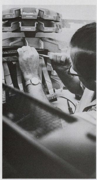
Advantages of flat flexible cable are apparent in this complex interconnection task—the wiring of an IBM computer mainframe.
