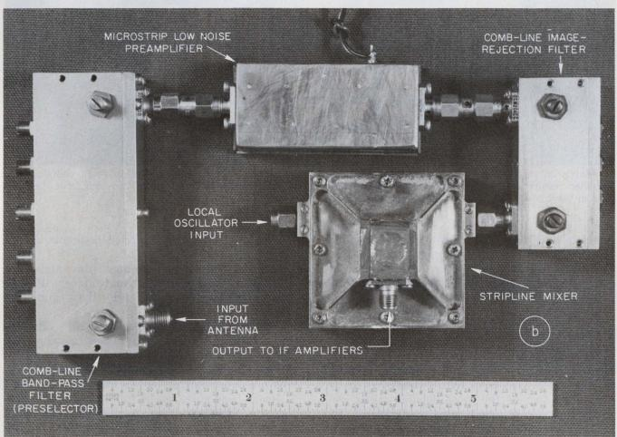
high performance transistors and carefully chosen input-output matching and interstage coupling circuits. The resulting microwave amplifiers can yield high gain, excellent stability, and low dc power consumption.
