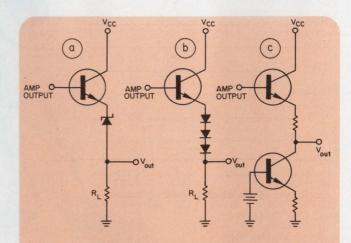
2. Circuits a and b remove the common-mode output but are temperature-sensitive. Circuit c degrades the frequency response.
