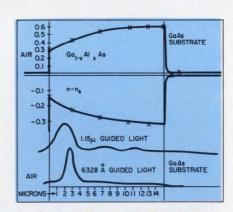
1. **Gradient guide** offers simpler fabrication alternative for thin-film semi-conductor waveguides. Near-infrared waves are guided in this structure.
