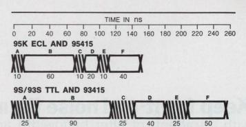
A – ADDRESS COUNTER B – MEMORY READ ACCESS TIME C – REGISTER D – 16-BIT ADD E – REGISTER F – MEMORY WRITE TIME
