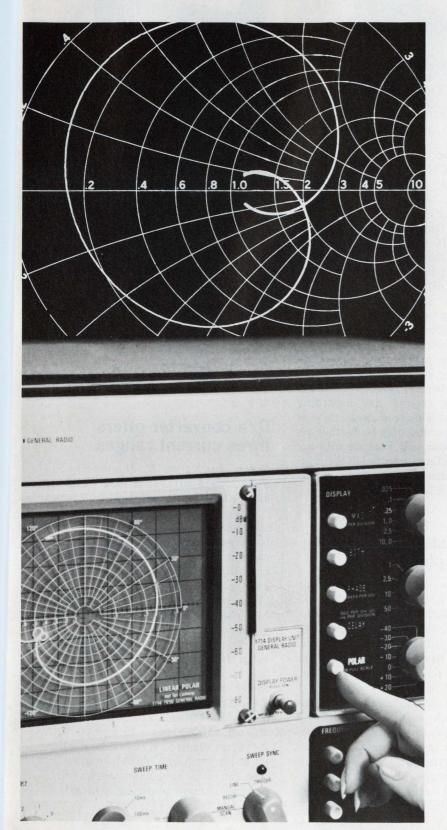
WHEN you need concise measurement data on antennas or rf cables, you'll see the value of polar (Smith-chart) displays of impedance versus frequency.
