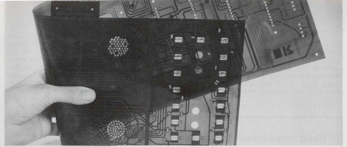
Rogers Corp.'s multilayer two-sided flexible PC combines the complexity of a rigid multilayer with the flexibility of an etched flat flexible cable. The resulting
