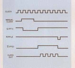
2. Four clock pulses are obtained from the programmable clock of Fig. 1a by presetting it to 4 with the toggle switches. The continuous clock can be derived either from the system clock or from an external source.
