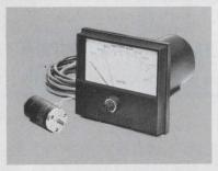
Control Meter Relay Speed Indicating System for use in process & control machinery. Adjustable singled dbl set pt systems, accuracy ±2% full scale, repeatability 0.5%, speed ranges 10rpm to 12,000rpm. Dbl set pts adjust to 0° ea other. Servo-Tek Products Company, 1086 Goffle Road, Hawthorne, NJ 07506 (201) 427-3100.
