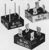
**B-50 Series**—DC rating: 10A @ 75°C case. Forward surge rating: 300A @ rated load. Ratings from 50 to 600 PRV per leg. Epoxy case construction.
