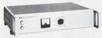
The 5087A is the first distribution amplifier to accept single 5 MHz input and distribute 0.1, 5 and 10 MHz outputs.
