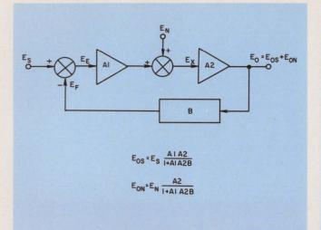
4. **Noise in the forward path** will be attenuated by preceding gain. But noise at the input cannot be reduced by closing the loop around an amplifier.
