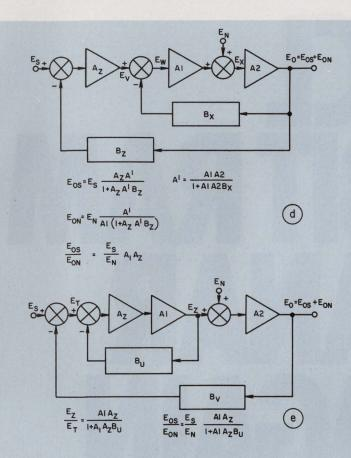
5. Signal-to-noise ratio is improved by preamp gain factor (5b and 5c). Multiple loops allow higher preamp gain than a single closed loop.
