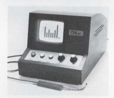
Probes of a Computer Synektics Micro-Sum monitor connect to the circuits of system being measured. CRT shows computer element activity.
