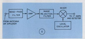
1. The basic microwave receiver front-end (a) can be designed simply and easily to limit noise figures with a tradeoff of filter bandwidth and loss between the preselector and image-rejection filters. The final design (b) uses coaxial filters built with comb-line structures.
