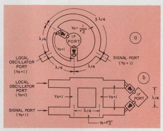
3. The most popular microwave mixers are the 180° (rat-race) hybrid coupler (a) and the 90° (branch-line) hybrid coupler (b). The design described uses the ratrace hybrid with beam-lead, hot-carrier, diodes as the mixing elements. The coupler selected provides wider bandwidths, better isolation and lower VSWR.
