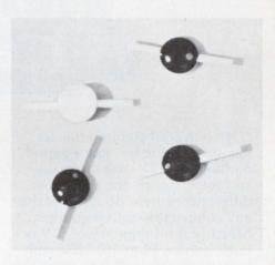
These low-noise stripline diodes are only 0.1 inch (2.5 mm) in diameter.
