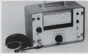
• High sensitivity, wide range .001 to 10,000 fc. • Accuracy 5% full scale, linearity 3%. . AC or battery operation. . Recorder output (1 v. to 1 ma. output). • Probes available with cosine correction and increased sensitivity to .0002 fc. . Use a densitometer, reflectometer, edge sensor, counter.
