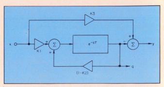
8. Digitally including the scaling factors,  $K_1$ ,  $K_2$  and  $K_3$  converts the differentiator to a digital high-pass filter.
