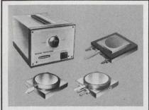
Wafer probes/controllers. Accurate measurement of electrical parameters of ICs thru 811-2000-01 bipolar controller with automatic temperature regulation. Gold plated vacuum chuck, 0 to +50°C range. 0.1°C accuracy. Other stages available. CAMBION. 445 Concord, Cambridge, Mass. (617)-491-5400).
