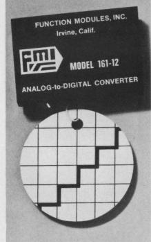
And you can put in 0 to -10V, or  $\pm 5V$ , or  $\pm 10$ . You can change the coding by changing pin connections ... straight binary, offset binary, and 2's complement are all there. Serial output comes for free.
