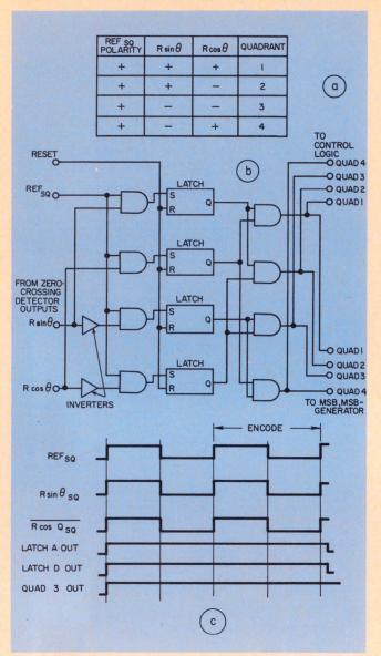
5. Instead of conventional demodulators, quadrant selection is essentially digital, in accordance with the truth table (a) and its implementation (b). The operation is detailed in "c."
