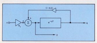
4. By digitally including the scaling factor, the integrator becomes a digital low-pass filter.
