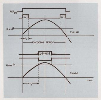
2. To eliminate pulsewidth jitter at large angles, both outputs of the Scott-T transformer (R  $\times$  sin  $\theta$  and R  $\times$  cos  $\theta$ ) are used. The R  $\times$  sin  $\theta$  is used for angles of less than 45°, and R  $\times$  cos  $\theta$  is used for angles of more than 45°.
