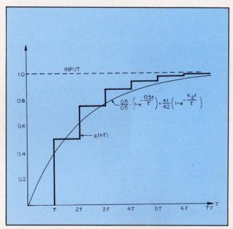
5. A good comparison is obtained between the unit-step input response of a low-pass filter and the approximation derived from the S-domain calculation.
