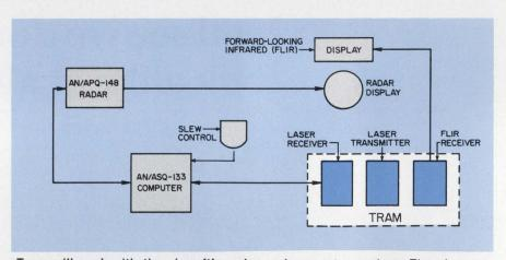
Tram will work with the aircraft's radar and computer system. The slew control realigns the infrared detector when the target drifts off center.
