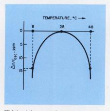
Wristwatch crystal operating temperature limits are typically established between 8 C and 48 C, with the normal wrist temperature (zero-error point) at 28 C.
