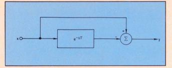
A digital differentiator is formed by using a subtractor with a shift register.
