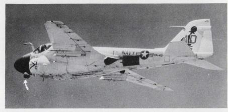
A small bulge had to be built into the A-6E attack plane to accommodate the new infrared-laser sensor system called Tram.
