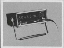
Low-cost 60MHz Frequency Counter. With five digits (overflow to 8 digits) the Tucker 60 is a 1 KHz to 60 MHz Counter with resolution to 1 Hz. Aging Rate is 1 part in 10-6/week. \$299.00 from stock. Tucker Electronics Company, P. O. Box 1050, Garland, Texas. (214) 348-8800.
