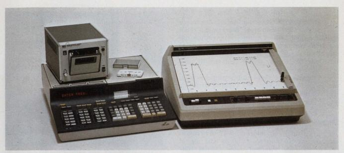
3. Programmable calculators that use a bus architecture are easy to interface with almost all the peripherals
