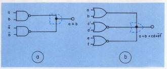
1. The wired-AND is formed by connecting the outputs of individual gates (a). The implied-OR is similarly obtained (b).
