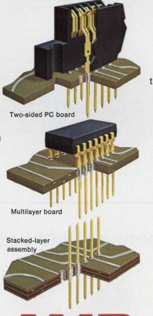
bridging, peaks, icicles, board delamination or damaged plated through-holes. After reflow, post and contact ends are clean and ready for point-to-point wiring. And can be replaced without damage to the board.
