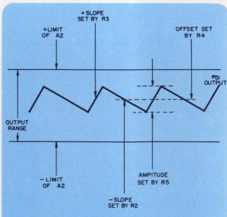
2. Triangular-wave output has positive and negative slopes, which may be varied independently of amplitude by potentiometers  $R_3$  and  $R_2$ .
