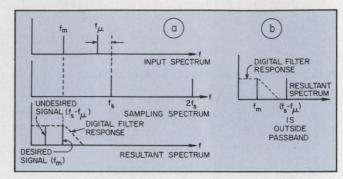
12. Aliasing of undesired signals into the passband is a serious problem in digital filters. Raising the sampling frequency helps reduce this problem.
