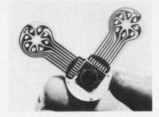
The silicon element—used in differential pressure and direct pressure transmitters—is sealed in a silicon fluid through which the fluid pressure is transmitted.
