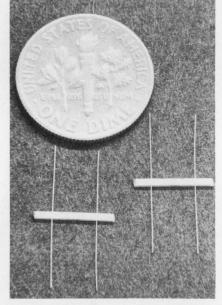
These tiny bars of quartz are the 32.786 kHz frequency standards that drive the Bulova Accuquartz watch. The leads shown are shortened and attached to a sealed can assembly.
