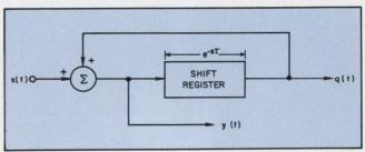
2. A digital integrator is formed by combining a shift register with an adding circuit.
