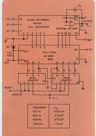
Capacitor  $C_{\rm F}$  smooths the output waveform of the MN 410 d/a converter in this ac reference circuit. Optimum values for the capacitor are indicated in the table.
