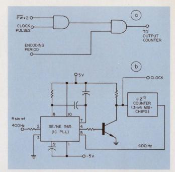
8. Pulsewidths are converted into digital data by a single AND gate (a) that puts out the clock pulses during the pulsewidth ( $\overline{PW} \times 2$ ). The second AND gate stops the output pulses to the output counter at the end of an encoding period. To eliminate the effects of the drift in the reference signal (synchro excitation voltage, R  $\times$  sin t), the clock is slaved to the reference (b).
