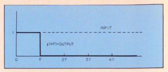
7. The response of the circuit in Fig. 6 to a step input shows that it behaves as a differentiator.
