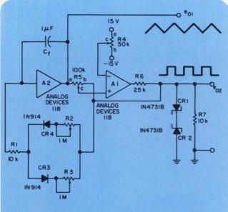
1. Integrator  $A_2$  generates a triangular wave from the square-wave output of comparator  $A_1$ . Resistor  $R_3$  controls amplitude, but has no effect on slope.
