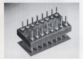
8. A dual-in-line adaptor plug for discrete components extends the versatility of Wire-Wrap techniques.
