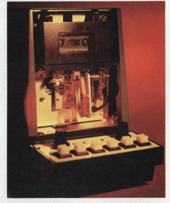
Bell & Howell's model 410 digital cassette decorder pulls tape out of the cassette in order to wrap it around a large capstan. This allows much more precise tape control than is possible with the small capstans that many other manufacturers use.
