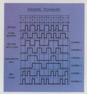
**Five of the more popular** data encoding techniques are illustrated in the table. Phase encoding is the method accepted by the new ANSI-ECMA standard.
