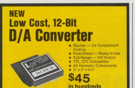
Now at a remarkably low OEM price . . . The DAC372-12 is a fine performance, general purpose 12-bit D/A converter featuring 30PPM/°C temperature coefficient, 0-70°C operation, and 5 $\mu$ Sec settling. The unit incorporates thin film precision resistors and is complete and ready to use. Price for 1-9 — \$75.
