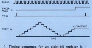
lustrated by the waveform for the output at point A.
