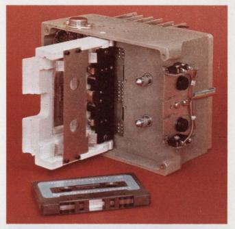
**High speed and high density** are characteristics of the Peripheral Dynamics 4200 Digital Cassette Tape Recorder. It is a reel-to-reel drive with servo-controlled tape speed and tension. It records on 4 tracks in order to store up to 8 million bits on a standard cassette.
