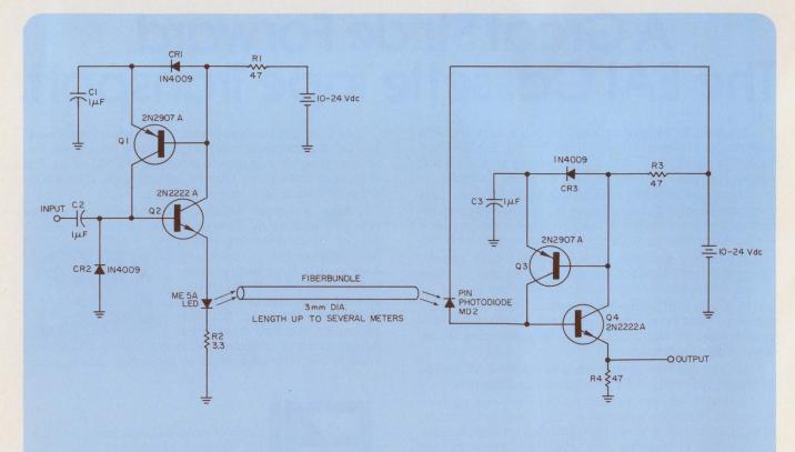
**Transmitter and detector operate** without standby power. Complementary switches  $Q_1 + Q_2$  and  $Q_3 + Q_3$
