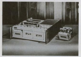
**Remex RCP drives can be packaged** with up to 3 drives to a case or can be bought as a transport for a single cassette. Remex stresses cassette interchangeability between systems and between decks in the same system. The drive is of the dual capstan variety.
