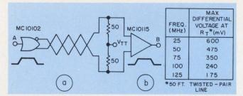
5. Pulldown resistors can also terminate a twisted-pair line (a), providing full output levels to the receiver. Attenuation data for 50 feet of twisted-pair line and 50  $\Omega$  pull downs (b) show higher differential voltages.
