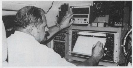
**Grumman Ecosystems' manager of systems technology,** R. W. Pate, searches for mineral deposits in Peru with Texas Instruments' AN/ASQ-81 magnetometer. In another aircraft the same area is mapped by sidelooking radar.
