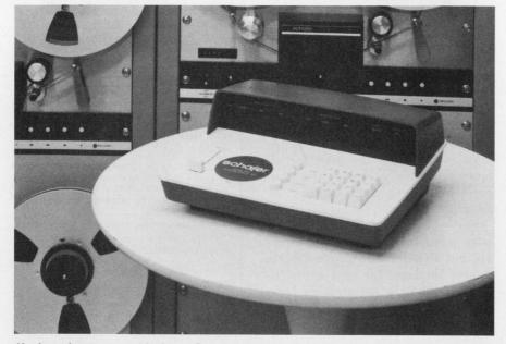
**Keyboard memory unit** from Schafer Electronics uses an MOS random access memory to store the operating program instead of magnetic tape. The unit holds an entire day's scheduling and can be loaded directly from the keyboard or from a prerecorded cassette.
