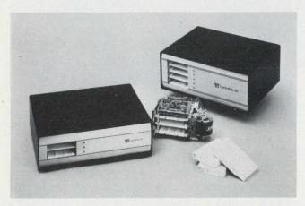
**Tri-Data produces several digital cartridge recorders.** The drives handle either two or four cartridges at a time. The 1/4-inch tape is contained within the cartridge as an endless loop. Tri-Data's drives all output data in parallel format of either 8, 12 or 16 bits.
