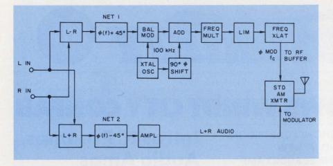
**AM stereo system** developed by Kahn Research uses sum and difference signals to transmit stereo information. Stereo signals are transmitted via upper and lower sidebands of the AM signal.
