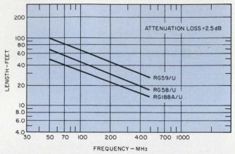
1. Maximum coaxial line lengths for a constant 2.5-dB attenuation loss depend on the operating frequency. This plot of three common cable types assumes that the lines have matched terminations.
