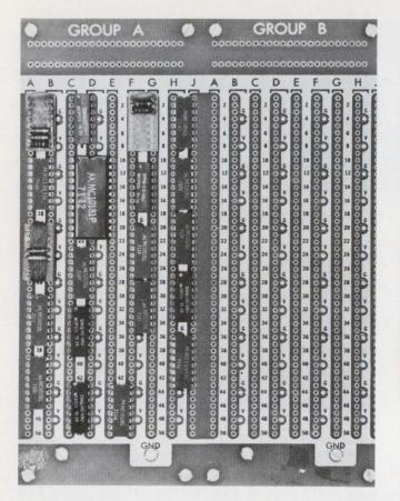
9. This  $4 \times 4$ -bit multiplier prototype shows Wire-Wrap with MECL 10,000 logic. Signals are taken on and off the board with commercially available conventional multi-
