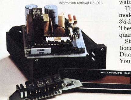
2. Only one circuit board. It carries both A/D and digital circuitry.
