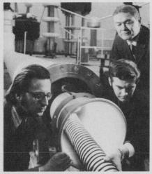
**Cryogenically cooled** (-320 F) aluminum power cable withstood 435,000 V at GE's R&D Center.
