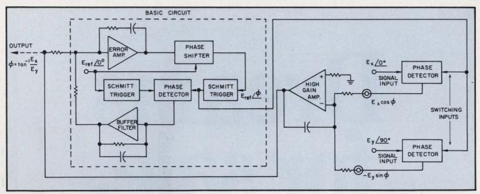
5. An all-electronic resolver is an interesting application for the wide-range phase shifter. Outputs from the two extra phase detectors,  $\text{Excos}\phi$  and  $\text{Eysin}\phi$ , are dc analogs of the resolved  $\sin/\cos$  components of the ac
