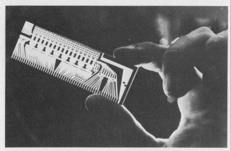
Laser machining technique forms circuit patterns directly onto insulative substrate. Process eliminates the need for clean room conditions.
