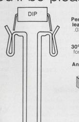
Permits extremely short lead-length - as short as .035" below device for full contact!
