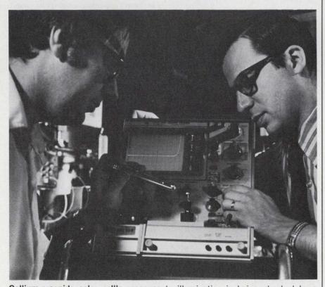
Gallium-arsenide solar cell's response to illumination is being checked by a flashlight by IBM engineers Jerry Woodall (left) and Harold Hovel. The oscilloscope reading shows the cell's very low resistance.
