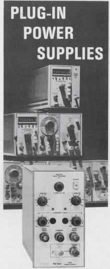
These high density, easy to operate supplies are designed for today's devices. Ideal for circuit investigation, device testing and educational applications. The PS 503 is a dual power supply with precisely regulated, shortproof outputs variable independently or at a constant ratio. All plug-ins have a +20 V floating supply and +5 V ground referenced supply.
