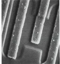
RCA's scanning electron microscope at 1000 X magnification shows excellent conformity of conductors over wafer contours, assuring continuity and reliability of metal interconnects. This is a dramatic example of process refinements achieved under the RCA high-reliability program which are automatically applied to commercial products.
