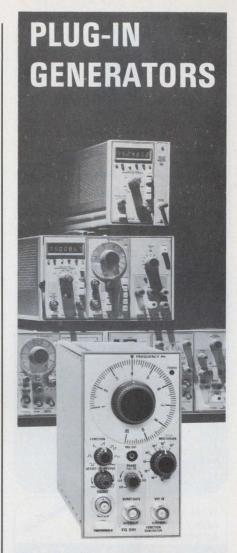
The FG 501 is a .001 Hz to 1 MHz function generator with sine, square, triangle, pulse, and ramp outputs. Harmonic distortion is low. VCF input has 1000:1 range. Gate/burst input has phasing variable from  $-90^{\circ}$  to  $+90^{\circ}$ .
