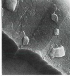
6000 X magnification shows excellent metal coverage over an oxide step.
