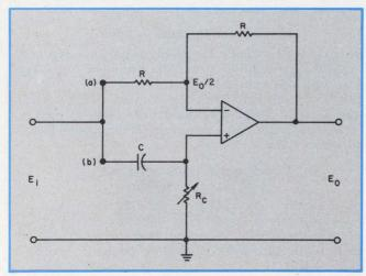
1. This basic op amp shifter provides a constant voltage output,  $E_{\rm o}$ . The output phase leads the input by an amount controlled by resistor  $R_{\rm o}$ .
