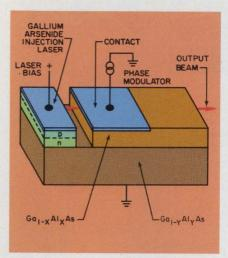
5. Schematic view of a thin-film gallium-aluminum-arsenide waveguide structure incorporating an injection laser and a phase modulator.
