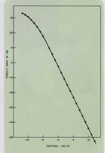
2. The control characteristic is nonlinear at high gain because of the noise and cutoff characteristics of transistors Q4 and Q5.
