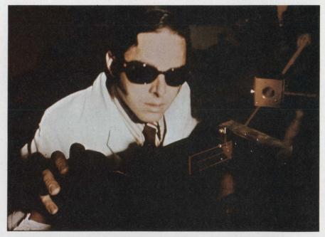
A laser beam is being injected into an experimental optical waveguide by J. E. Goell of Bell Laboratories. The waveguide, made by a masking and etching process similar to that used for ICs, is a deposited glass film.
