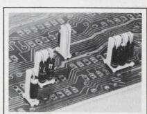
Verti-Mount Insulators permit vertical mounting of DO-7, DO-34, and DO-35 diodes and 1/8-, 1/4-, and 1/2-watt resistors on printed circuit boards. Verti-Mounts increase packaging density by 200%. Robison Electronics, Inc., 2134 W. Rosecrans Avenue, Gardena, Calif. 90249. Phone: (213) 321-0080.
