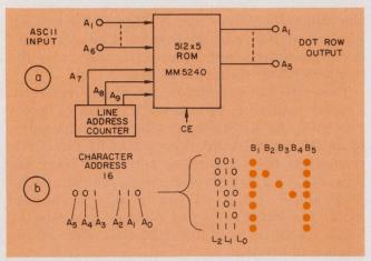
5. A raster-scan circuit for the generation of ASCII characters (a). The output provides the dot-row information for a typical  $5 \times 7$  character (b). This technique is often used for TV monitor tubes. A total of  $8 \times 5 \times 64$  bits are stored in the ROM.
