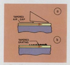
3. The efficiency of coupling optical energy from the waveguides is increased by the use of tapered air gaps (a) and tapered gratings (b).
