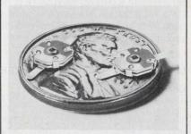
Thin-Trim capacitors are designed to replace fixed tuning techniques. Applications include crystal oscillators, CATV amplifiers, communication and test equipment. Series 9410 has high Q's with capacitance ranges of 1.0 - 4.5 pf and 10.0 - 50.0 pf. Johanson Manufacturing Corporation, Boonton, N. J. (201) 334-2676
