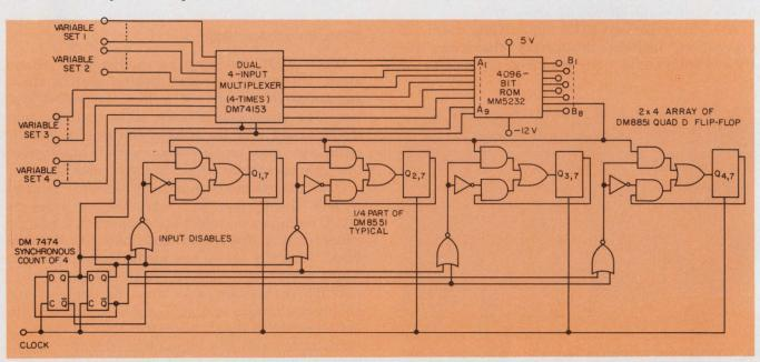
7. Any ROM can be used for random-control sequencing or random-logic synthesis. In this application a multi-
