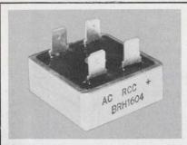
RCC BRH1600 serles 16 amp./65° C. single phase silicon bridge rectifiers. Available voltage types of 50 to 800 volts peak with single cycle surge current ratings of 125 amps. peak. 1-99 quant. \$3.30 to \$6.60 dep. on voltage type. Rectifier Components Corp., Freeport, N.Y. 516-868-0470.
