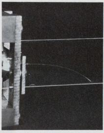
Curved optical waveguide of sputtered glass, from Bell Laboratories, is 20  $\mu$ m wide and about 0.3  $\mu$ m thick.
