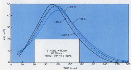
Relaxed timing requirements of Ampex TIN core is evident from these curves of core response as a function of time in switching from a ZERO state to a ONE state. Each curve shows the core response at a different temperature. The strobe window is the timing slot that the designer can use if the memory must work over the full specified temperature range. The curves are taken at a constant drive level of 475 mA.
