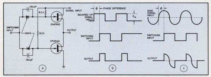
3. This typical phase detector circuit provides a pulsed output. Its average value is directly proportional to the phase difference of the inputs when a squared-up signal input is applied, as in 3(b). The phase-detector output
