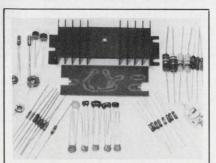
**Broad Band**—No Tuning Power amplifier in kit form. Frequency range 500 kHz to 100 MHz with 25 watts of cw power. It accepts inputs of AM, SSB, pulse and other complex modulation. The unit withstands a +15-dB overdrive including and open-circuit loads. Larkton Scientific, P.O. Box 302 Monroeville, Pa. Phone: (412) 731-6829.
