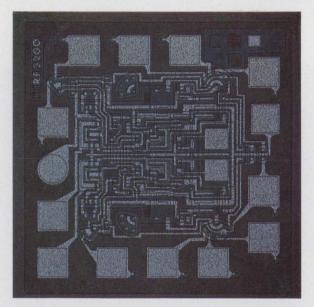
An AND-input J-K flip-flop is offered in the RAY III series from Raytheon Semiconductor. Termed the RF3200, it has a listed speed of 10 ns.
