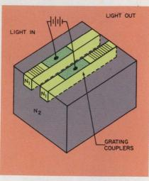
6. A basic gallium-arsenide structure for electrically varying the coupling between two waveguides. Power is thus transferred between them.
