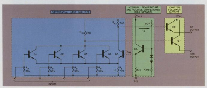
1. The basic circuit in the MECL 10,000 series is this gate. The  ${\sf OR/NOR}$  outputs provide simultaneous com-
