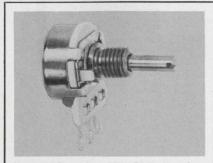
New CTS series 205  $\frac{5}{8}$ " dia. Cermide® thick-film variable resistor. Excellent environmental char.; and immediate design versatility. 1 w power @ 70°C;  $50\Omega$ -5meg- $\Omega$  resistance;  $\pm 20\%$  tol.; dust shield; many mounting styles and shaft types. Only 82¢ in quantity. Power switch available. CTS Keene, Inc., Paso Robles, Calif. 93446. (805 238-0350.
