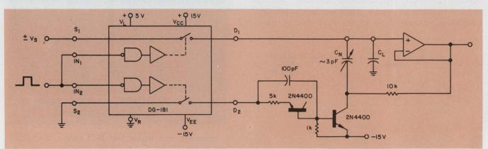
7. This neutralization circuit is almost perfect over a  $\pm 15\text{-V}$  signal range. It uses a dual driver and the DG181
