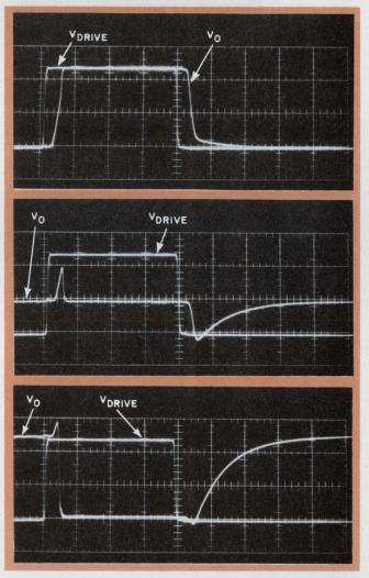
5. Transients in a typical fast JFET switch, the GD187. Here  $R_{\rm L}=10~k\Omega,~C_{\rm L}=30~pF$  and the scales are 2 V/div and 500 ns/div. From top to bottom,  $V_{\rm A}=+5.0,$  and -5~V.
