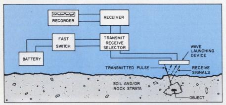
Electromagnetic Subsurface Profiling system uses a fast switch to produce nanosecond, time-limited pulses, which are transmitted and received by a specially designed antenna.
