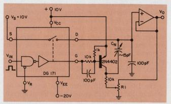
10. The single-switch PMOS DG171 is easily neutralized because the driver output is available at a terminal pin. A pnp transistor provides charge transfer to the neutralizing capacitor  $C_{\rm N}$ .
