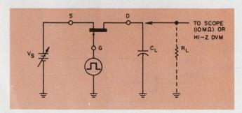
4. Basic circuit for measuring transients by the charge-transfer method.
