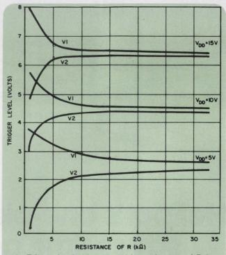
2. Trigger levels plotted against resistance of R for three values of dc supply voltage  $V_{\rm DD}.\ V1$  is the ON trigger, V2 is the OFF.
