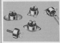
Precision snap-action thermostats from Elmwood, widely specified for quick, reliable response; proven industrial and military performance record. Environ. expos. –85° to 550° F; narrow or wide diff.; rated to 15 amps. Prototypes from stock. Wide choice of brackets, terminals. Elmwood Sensors, Inc. (401) 781-6500. TWX 710-381-6413.
