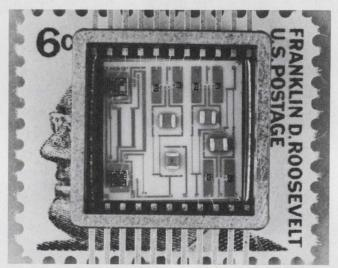
This dual muliplier/divider (5/8 by 5/8 flatpack) is used by General Electric's AICS department on several aerospace programs for precision analog computation.
