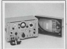
HP 623B RF test set. Completely reconditioned and guaranteed. A complete test package for communications station equipment. Choice of 3 klystrons in 5925-7750 MHz range. Send for free catalog listing thousands of instruments. \$1395.00. Tucker Electronics Company, P. O. Box 435, Edison, New Jersey. (201) 225-2900.
