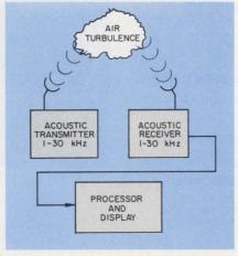
Acoustic radar for detecting aircraft wake turbulence.
