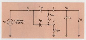
1. Gate-pulse edges form switching transients as they are coupled to the load through FET capacitances.
