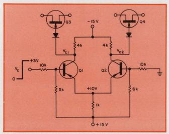
3. **JFETs could be used** as analog switches, but due to the large pinch off voltages (P-channel), they cannot be driven directly from the comparator outputs. Hence complex and costly drivers would need to be provided.
