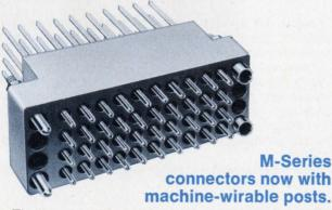
The latest addition to our M-Series connectors gives you real production economy. They have posts for automatic machine wiring . . . four sizes: .022" x .036"; .031" x .062"; .025" square; .045" square.
