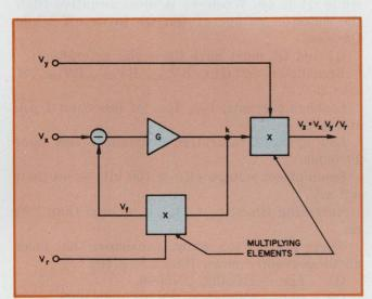
1. Every servo multiplier employs two elements to multiply two signals  $V_{\rm x}$  and  $V_{\rm y}$ . The element in the feedback loop normalizes the product with respect to  $V_{\rm r}$ .
