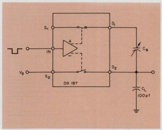
6. This basic neutralization circuit has the advantage of simplicity, but it offers complete neutralization at only one value of signal voltage.
