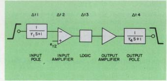
How circuit components contribute to propagation delay. The input-pole contribution depends on inputwaveform transition times.
