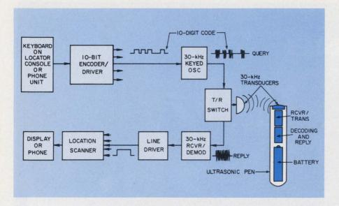
In the Trackatron finder system, entering a person's code in a seeker keyboard sends out a building-wide ultrasonic query. The person's transponder replies with a 30-kHz burst that identifies his whereabouts.
