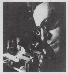
A new gas laser developed by Bell Telephone Laboratories is only two inches long.
