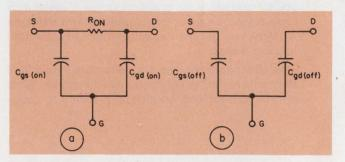
The ON (a) and OFF (b) equivalent circuits of a JFET are useful in the noise analysis.
