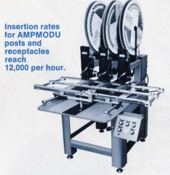
AMPMODU\*, our post-receptacle interconnection system, now offers you even higher production capabilities than ever before. It's the ideal technique for modular-designed consumer or industrial electronics.
