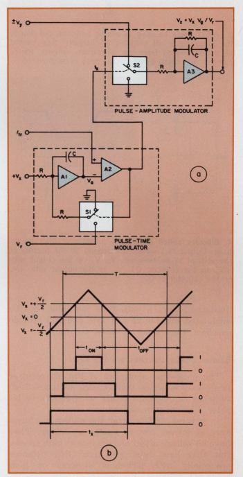
2. Using analog switches as multiplying elements (a), we can build a very accurate pulse-time multiplier. The pulse-width signal,  $t_{\rm x}$ , is a linear function of one multiplication variable,  $V_{\rm x}$ , and of the voltage reference  $V_{\rm r}$ .
