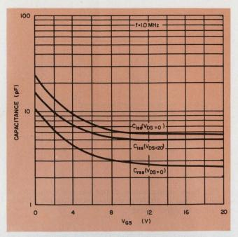
3. Capacitance vs gate-to-source voltage for 2N4091, 4391 and 4856 JFETs.  $C_{\rm rss}$  is the gate-to-source capacitance;  $C_{\rm iss}$  is the sum of gate-to-source and gate-to-drain capacitances.
