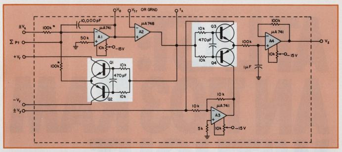
5. This precision four-quadrant multiplier/divider can be built discrete or hybrid (in a single flat pack). It requires
