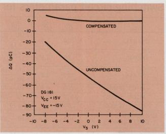
8. Compensation with the circuit in Fig. 7 drastically reduces the change in transferred charge with signal level for the DG181, a  $30-\Omega$  JFET switch.
