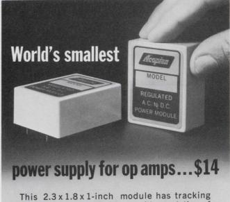
outputs of  $\pm 15$  V @ 25 ma with regulation of ±0.1% and ripple of 1 mv. It costs \$14.00 in 1,000 lots and only \$24.00 for one. Requisition Model D15-03. (For  $\pm$  12 V @ 25 ma, order Model D12-03.) Three-day shipment guaranteed.
