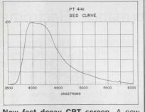
New fast decay CRT screen. A new long life phosphor screen is available with a decay time of 80 nanoseconds and with an efficiency substantially higher than standard P-16. Available in a wide variety of CRTs for scanners and readers. Thomas Electronics, Inc., 100 Riverview Drive, Wayne, N. J. Phone: (201) 696-5200.
