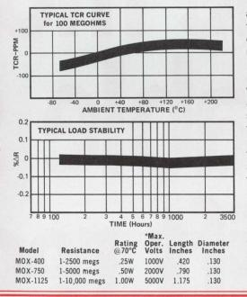
full-rated voltage; in addition, typical quantech noise at 20 megohms is less than 0.5 microvolt/volt.
