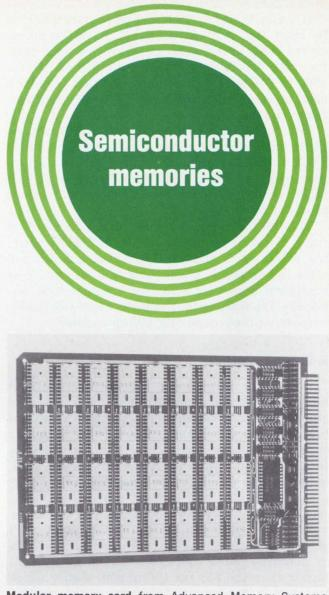
**Modular memory card** from Advanced Memory Systems uses 1024 X 1-bit MOS RAM chips with 350-ns access to provide 4096 eight-bit words.
