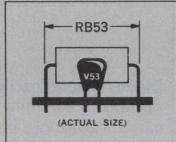
Size comparison between V-53 and RB-53 type wirewound. Vishay V-53 requires only 1/8 the space needed by the RB-53.
