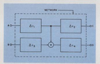
3. A logic interlock also fixes the required time relationships. With the logic connection, both inputs must be present before there is any output. To optimize the system with this method it is required that  $(\Delta t_4)_{\min} \ge (\Delta t_2)_{\max}$  and  $(\Delta t_1 + \Delta t_4)_{\max}$  be minimized.
