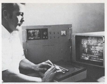
**Encoded time and frequency measurements can be sent via television broadcasts** to industry and homes without affecting normal transmissions, says the National Bureau of Standards, which is developing the system.
