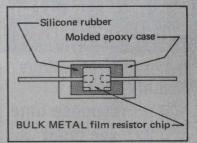
Section of Vishav Model M-53 Molded Resistor for direct RB-53 replacement.
