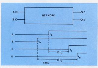
1. Obtaining  $t_d \ge t_c$  while minimizing time delays at the output is the objective in guaranteeing signal timing relationships. The required timing relationships are defined for output signals C and D, which are responses to inputs A and B, respectively.
