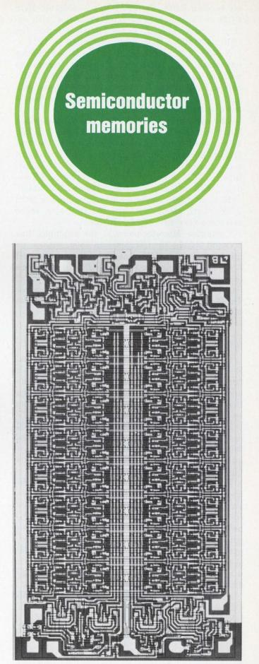
Schottky-clamped Am3101, a 64 X 1-bit bipolar RAM from Advanced Micro Devices, offers 30-ns access.
