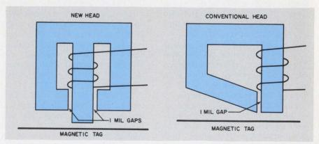
**Double-gap magnetic recording head** gives an accurate recording with up to 45° angular displacement or tilt from the data line. Present recording heads work only with about 15° of angular displacement and about 10° of tilt.
