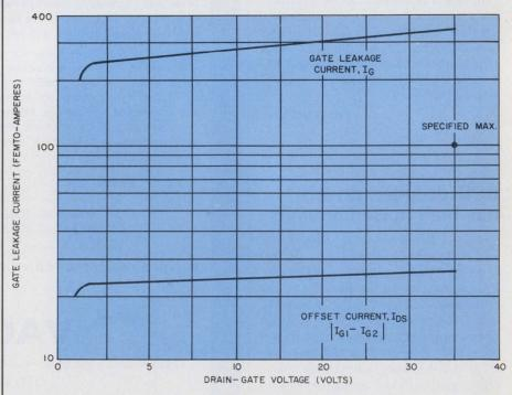
A new family of monolithic JFET duals features devices with ulta-low leakage and offset currents down in the femto-amperes region. These new JFETs can handle drain-gate voltages as high as 35 V with no input current degradation. Drain current for the above curves was set at 100  $\mu$ A.
