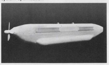
Garrett AiResearch enclosures are also cooling the pod mounted ALQ-76 and ALQ-99 electronic countermeasures systems. The enclosure in the ALQ-99 pod (shown above) for the EA-6B utilizes surface heat exchangers as the ultimate heat sink.
