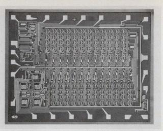
The fastest static shift register, Ragen's 64-bit MS612, can operate at 25 MHz. It uses complementary MOS transistors to slash standby current to 1 microampere.
