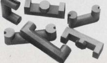
Tektronix, Inc. selected 24B for their "U" and "E" cores. This proven material has seen years of service in flybacks for television. Ideal for power applications, it can be operated at higher frequencies than laminated steel. It is cool running, due to low losses under power conditions and controlled power permeability. Tooling is available for a wide range of "U", "E" and "I" configurations.
