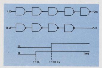
4. A simple example requiring a guaranteed timing relation of  $t_d \ge t_c$ , the basic network consists of NAND gates. Gate delays are 10 ns to 20 ns; delay lines have  $\pm 10\%$  tolerances. The minimum delay to be added to D, neglecting tolerances, is 80 ns.
