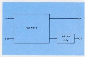
2. Introducing a delay in one path is the easiest way to obtain the  $t_d{\cong}t_e$  criteria. The delay can be determined by assuming a worst-case delay, tuning one path or tuning both paths. The last option provides the least delay to signal D.
