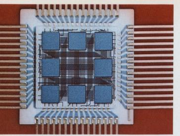
Gold-beam-lead chips on a ceramic substrate form a 2048 X 1-bit static MOS RAM from Texas Instruments.
