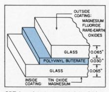
**CRT faceplate** is a sandwich of bluegreen polyvinyl buterate between two pieces of coated glass.
