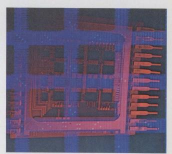
**Close-up (red) and closer-up** (blue) photos, superimposed, of CM2400 module from Computer Microtechnology, show 16 256  $\times$  1-bit MOS storage chips in the center, five bipolar sense amplifiers and decoders around the periphery of this TTL-compatible 4096  $\times$ 1-bit, 2048  $\times$  2-bit or 1024  $\times$  4-bit static RAM. Combination of MOS and bipolar chips, all using aluminum beam leads, provides high speed with low dissipation.
