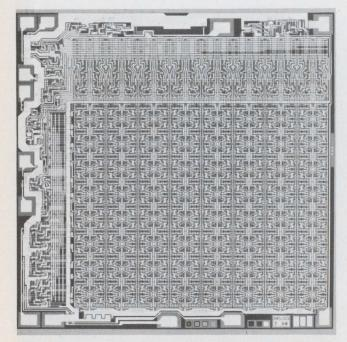
**One of the first 256 X 1-bit bipolar RAMs,** Intersil's 5503, fits on a 120 X 120-fil chip.
