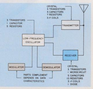
4. Station design is uncomplicated and inexpensive. The design details will vary with the system designer, but the parts complement should be approximately as indicated in this typical-system example.
