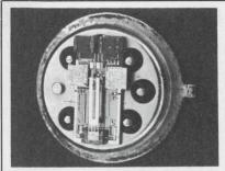
Ultra-miniature crystal oscillator and filter products are available from 10-100KHz in T0-5's or flatpacks, with as low as 10 micro amps consumption and O's of 2-40K. Products include timers from seconds to months, telemetry systems, clocks, signal processing filters, etc. Statek Corp., 1200 Alvarez Ave., Orange, CA 92668. 714-639-7810.
