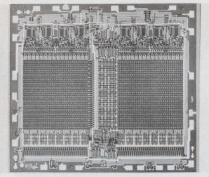
The first erasable field-programmable ROM, Intel's 1601 on a 147 X 161-mil chip, can be erased by exposure to ultraviolet light, then reprogrammed.
