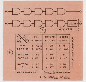
6. The hybrid technique of method 3 results in the optimum connection shown (a). A table giving all possible connections (b) lists each in terms of the criteria of method 3. The delay  $\Delta t_5$  is a variable used to solve the inequality  $[\Delta t_4 + \Delta t_5]_{min} \cong (\Delta t_2)_{max}$ . The optimum connection has least over-all time delay.
