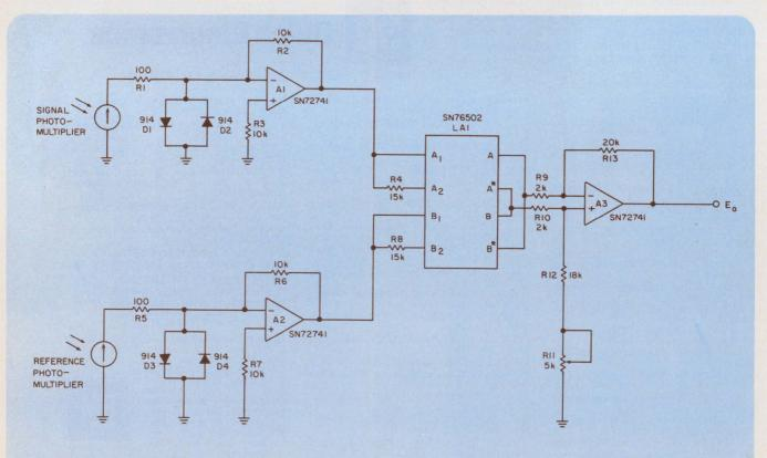
A low-cost, wideband (40 MHz) log amp (LAI) enables the circuit to achieve a faster and more accurate response than the usual design employing the nonlinear characteristics of diodes or transistors. The output voltage is proportional to  $\log A - \log B$ . Resistor R11 zero sets op amp A3.
