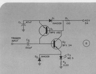
An avalanche transistor is replaced by a transistor switch in this light-pulse generator circuit (a). A
