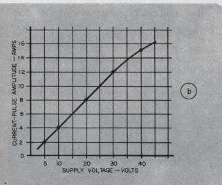
graph (b) relates the LED current amplitude to the supply voltage. Points plotted are measured data.
