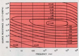
1. Noise figure is a constant for a given contour. Note that the NF is a single-valued function of source resistance and frequency, although there are two values of  $R_{\rm s}$  for each combination of frequency and NF.
