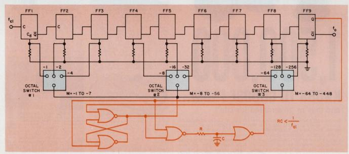
2. An RTL ripple counter with nine stages is similar in operation to the TTL circuit of Fig. 1. By selectively connecting the gate pulse to the  $C_{\rm d}$  inputs through three
