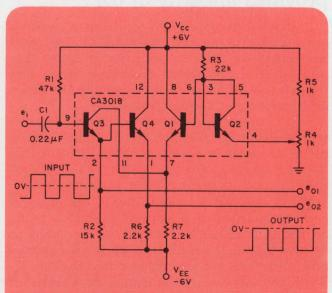
Monolithic quad transistor array with a minimal number of external components yields a low-temperature-coefficient dc restorer with adjustable clamping level and emitter-follower output.
