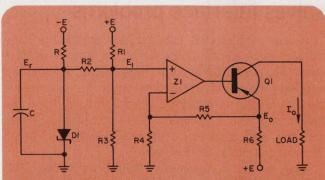
A very accurate, stable constant-current supply makes use of op amp  $Z_1$ . Neither the zener diode,  $D_1$  nor the amplifier carries any load current. The output transistor,  $Q_1$ , which supplies the load, has its  $V_{\rm be}$  within the feedback loop to minimize the effect of this parameter on performance.
