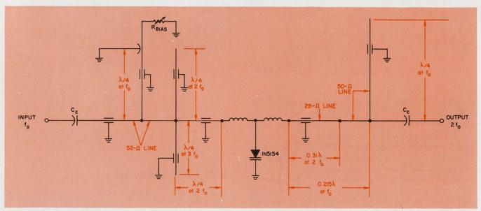
4. The bias is introduced before the input filter to avoid the formation of a low-frequency idler. Note that this com-
