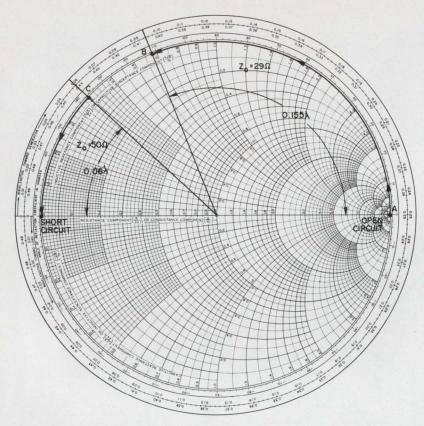
3. Rotating an open circuit, Point A, by 0.155 $\lambda$  converts it to j20  $\Omega$ , Point B, on a 29- $\Omega$  line. On a 50- $\Omega$  line, j20  $\Omega$  is at Point C so that only 0.06 $\lambda$  of additional rotation is needed to transform the open into a short.
