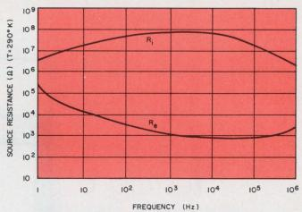
2. A plot of R<sub>e</sub> and R<sub>i</sub> is roughly equivalent to a 3-dB noise-figure contour in the region where the curves are widely separated. This particular amplifier has a minimum noise figure of 0.03 dB at 10 kHz.
