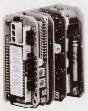
**Plug-in display t**ogether with plug-in PC boards (left) simplify servicing in the new 3-1/2 digit LED DPM (right).
