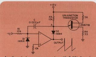
A voltage-to-frequency converter with 0.4% linearity can also operate as a sawtooth generator. This uncomplicated inexpensive circuit provides good temperature stability, too.
