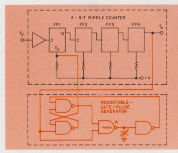
1. The division ratio of a four-bit ripple counter will increase to more than 1/16 if a variable width inhibit pulse (controlled by RC) is applied.
