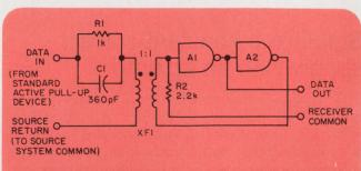
An interface circuit, acting as a line-driver/receiver, can cut parts cost to under \$5 per information line. Dual-in-line quad transformers and integrated-circuit hex inverters are used.
