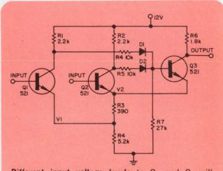
**Different input voltage levels** to  $Q_1$  and  $Q_2$  will trigger this circuit. The circuit can be used to match diodes. Connecting the bases of  $Q_1$  and  $Q_2$  produces a Schmitt trigger with low hysteresis.
