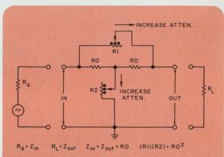
2. The attenuation of the constant-impedance bridged-T network depends on the values of  $R_1$  and  $R_2$ . The exact attenuation for given settings can be computed in advance by the program of Fig. 1.
