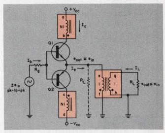
3. The generalized split-load output stage has an  $N_1$ :1 turns ratio between the collector windings and the output windings. In the analysis in the text it is assumed that  $\beta$  is high enough to consider  $I_e = I_c$ .
