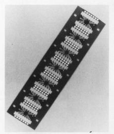
Silicon IC chips are attached to lead frames that are part of a plastic film strip in GE's new miniMod package. The chips are then encapsulated in a protective epoxy.
