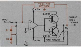
1. The emitter followers boost the op-amp power to about 0.5 W. With the dashed line connected and the colored components omitted, the circuit is a linear amplifier. The reverse case yields an oscillator-driver.
