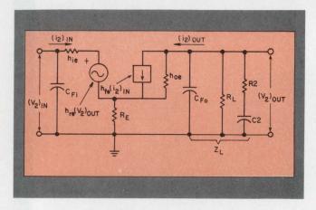
5. With the second stage described by its mid-frequency equivalent ac model (hybrid configuration), the input and output capacitance  $C_{\rm Fi}$  and  $C_{\rm Fo}$  are defined by the Miller Effect.
