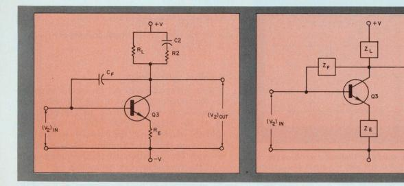
4. The device's second stage is redrawn (a) for analytical simplicity. Internal as well as compensation (external) feedback elements are recognized. The second
