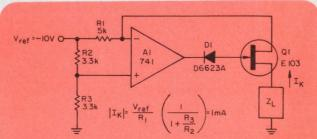
Precisely controlled load current flows only through the FET,  $Q_1$ . To reverse current flow,  $V_{\rm ref}$  should be positive,  $Q_1$  should be a p-channel FET and  $D_1$  should be reversed.
