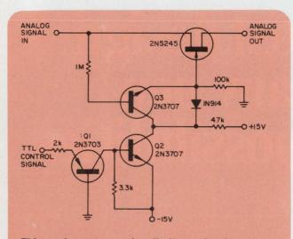
This analog gate can handle large signals because emitter follower  $Q_{\rm 3}$  allows the FET's gate to follow the analog signal input, keeping the channel resistance low over a wide voltage range.
