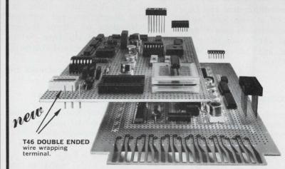
Precision punched .042" holes spaced .1" x .1" available in sheets of various sizes up to  $8\frac{1}{2}$ " wide by 35" long,  $\frac{1}{16}$ " thick Epoxy Glass, Epoxy Paper, Phenolic.
