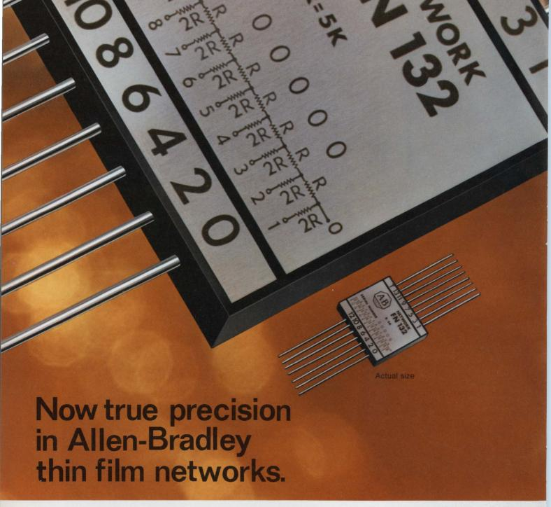
Resistance networks for A/D and D/A conversion, digital volt meters and numerical control systems demand extreme precision. Allen-Bradley can deliver. Precision that starts with a patented chromium-cobalt resistive material vacuum deposited on a substrate made to Allen-Bradley specifications. Precision based on exclusive computer drawn grids. Precision backed by extensive design and testing facilities. Precision on a continuing basis assured by Allen-Bradley's 14 solid years of experience.
