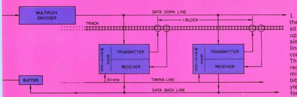
1. Speed commands on the Bay Area Rapid Transit system will be sent to up to 30 wayside boxes simultaneously on a single line with this multiplexed communication system. The comparison of data received with data transmitted in the fail-safe, bit-by-bit comparator yields vehicle location information as well.
