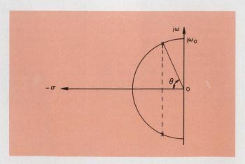
1. The poles of the filter can be arbitrarily placed anywhere in the s-plane in order to achieve the desired value of damping. The angle  $\Theta$  is given as  $\cos^{-1}\zeta$ , where  $\zeta$  is determined by the relative values of the passive components chosen for the particular active filter.
