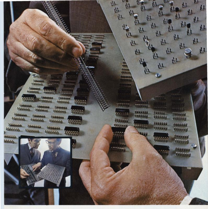
HERE'S A NEW AND BETTER WAY: To make printed circuit board connections. Reliably. At low, low cost. They're Molex Soldercon® terminals. Integrated circuit and transistor terminals. Offering the convenience of plugin I.C.'s and transistors without the cost of insulators. They fit directly on the board. And there is equipment available to do the job automatically. Fast! Soldercon terminals save time. Money. Speed installation. Make
