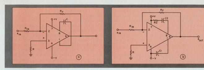
1. The recommended compensation specified by the manufacturer employs a single capacitor that introduces a simple 20-dB roll-off at low frequency and stabilizes the device against temperature variations and parts re-
