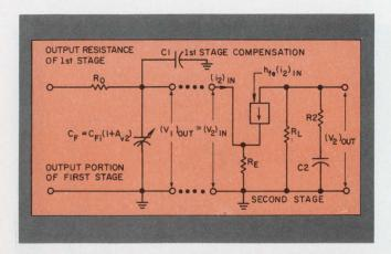
6. Valid ac model of combined first and second stages of the device, with  $C_{\rm F_0}=0$  and with the effect of h-parameters reduced for analytical simplicity. Note that  $C_{\rm F_1}$  is a function of the second-stage gain,  $A_{\rm V2}$ , the impedance of which decreases with an increase in frequency; this variation in  $C_{\rm F_1}$  is compensated by  $C_{\rm 1}$  connected in parallel.
