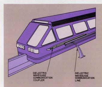
3. Bandwidths of up to 500 MHz are possible with a dielectric waveguide communications link. A length of waveguide on the vehicle couples energy from the line. The waveguide consists of a semicylindrical rod of polyethylene, bonded to a metal shield.
