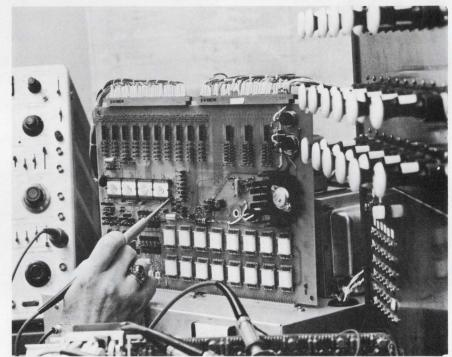
Entire North American Rockwell organ stop-selection system is contained on a single printed circuit board. The system contains four MOS/LSI arrays and 550 discrete components.
