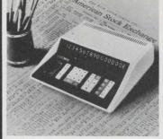
Sharp MAXI II. With 2 memory banks. Full 16 digit capacity. Pre-set decimal. Memory light. Function light. Round-off capability. Chain calculation. Automatic squaring. 8½ lbs. Sharp CS-362.
