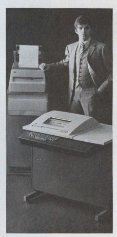
Inktronic® data terminals: A unique electronic, solid state terminal. Prints up to 1200 wpm. Forms characters through electrostatic deflection (no typebox). ASCII compatible.
