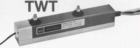
The WJ-3604 is a medium-power low-noise traveling-wave tube designed for use in airborne and shipboard applications. It is particularly suitable for applications where gain variation and noise figure are important (the tube provides fine structure gain variation of  $\pm 0.75$  dB across  $K_u\text{-band}).$
