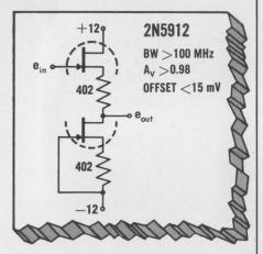
Half the device acts as a current generator for the source follower. Since the FETs are matched to less than 15 mV,  $V_{GS1} = I_DR_1 = I_DR_2 = V_{GS2}$  and near zero offset is achieved.
