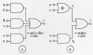
2. The normal Karnaugh map synthesis of the table of Fig. 1a results in the circuit "a." The exclusive-OR implementation reduces this to the circuit in "b."
