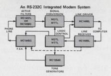
Frequency-Shift Keyer . . . The MC1445G is a dual-input, logic-controlled video switch that can connect either of two tone generators to an output line. It also has a low-impedance emitter-follower output stage.
