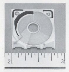
The substrate supporting the new variable network. The variable capacitors are the upper segments, while the fixed are on the bottom.
