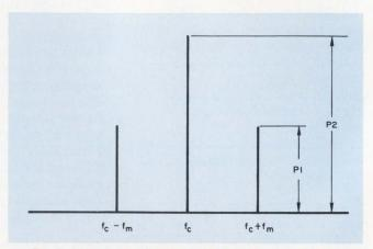
3. Bandwidth data stares at you from the face of a spectrum analyzer display. This frequency-domain measurement is probably the easiest to perform as long as the sidebands are clearly separated from the carrier.
