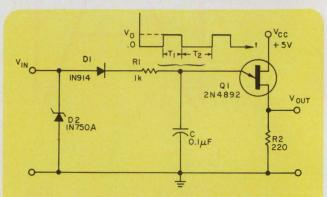
UJT counter uses zener diode to equalize input pulses. Capacitor C must be selected to allow complete discharge during pulse spacing period  $T_2$ . Component values are for a divide-by-7 counter.
