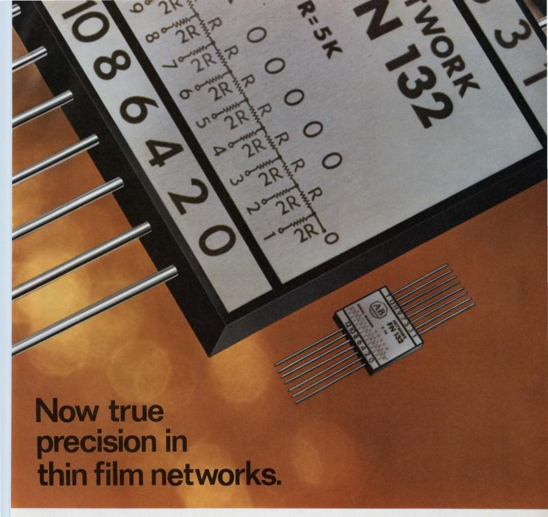
Resistance networks for A/D and D/A conversion, digital volt meters and numerical control systems demand extreme precision. Allen-Bradley can deliver. Precision that starts with a patented chromiumcobalt resistive material vacuum deposited on a substrate made to Allen-Bradley specifications. Precision based on exclusive computer drawn grids. Precision backed by extensive design and testing facilities. Precision on a continuing basis assured by Allen-Bradley's 14 solid years of experience.
