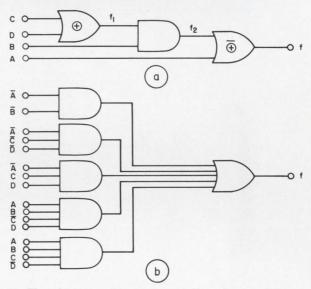
5. **The decomposition map** of Fig. 4d results in the circuit "a." The same logic derived with conventional methods gives the circuit of "b."
