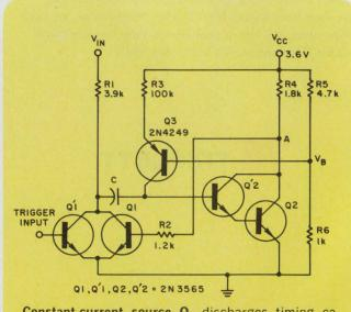
Constant-current source  $\mathbf{Q}_{\rm s}$  discharges timing capacitor C in this monostable. Over the full input range (V<sub>in</sub> = 0.2 to 25 V) linearily is  $\pm 1\%$ .
