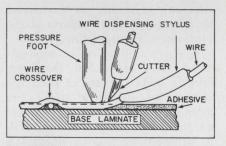
The Multiwire technique uses a numerically controlled machine to spit out insulated wire onto a circuit board.
