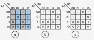
3. Three possible four-variable maps can be drawn for a given logic function. The AB-CD map of "a" is chosen for additional study because it has two sets of matching columns.
