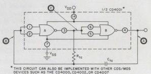
FIG.I. ASTABLE MULTIVIBRATOR CIRCUIT DIAGRAM
