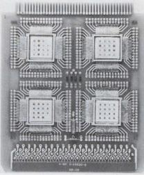
Circuit designers and suppliers hassled over the relative advantages of wire vs multilayer printed-circuit connections at the IEEE Eastern Electronics Packaging Conference. But amid the unresolved arguments, two new techniques were described that combine the features of multilayer with the fast turn-around and flexibility of wire interconnects.
