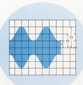
1. **Dynamic range information** is given explicitly in the time domain. Oscilloscope or power-meter measurements are particularly valuable at low-modulation rates when carrier and sidebands are very close together.
