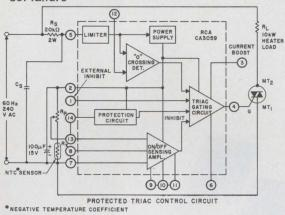
In the heater application shown here, the protection circuit removes power from the load if the sensor shorts or opens. To utilize the protection circuit, connect terminal 13 to terminal 14, as shown, and then:
