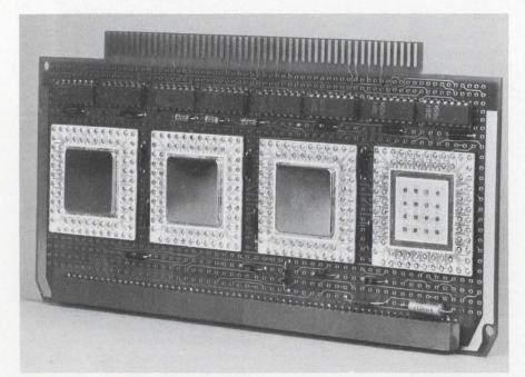
**QTA—Quick Turnaround—a three-tier system** developed by Loral Electronics. Each tier of printed circuits, substrates and chips is topologically structured—that is, multilayered—in itself.
