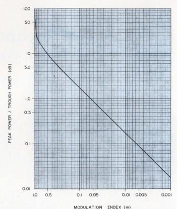
2. When a power meter is used to make time-domain measurements, this plot of peak-to-trough power ratio vs modulation index is a convenient tool. The power ratio is measured in decibels.
