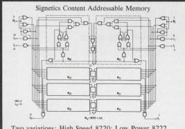
Two variations: High Speed 8220; Low Power 8222. Both monolithic arrays incorporate necessary addressing logic and eight identical memory cells organized as four words, each being two bits long. They offer associate, write-in only and read-out only function capability. Complexity: approximately one-hundred gates. Package: 16-pin.
