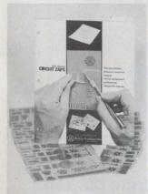
PRE-ETCHED, PRESSURE-SENSITIVE C O P P E R COMPONENT PATTERNS FOR INSTANT PC BOARDS. Circuit Zaps® are 1 ounce copper circuit components patterns, pads, and conductor paths, precision-etched on 5 mil (.005") glass epoxy base material, backed by a special pressure-sensitive adhesive. Circuit Zaps® completely eliminate the artwork, photography, photoprinting, touch up, etching, stripping, and other time-consuming steps in PC board development. Circuit Zaps® provide maximum flexibility.
