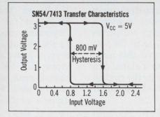
Unmatched stability Each gate has different input threshold levels for positive and negative going signals. Hysteresis-the difference between the
