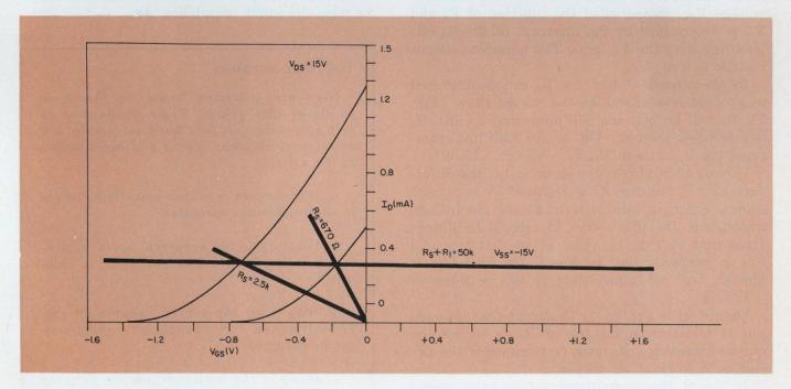
7.  $\textbf{R}_{s}$  can be trimmed to provide zero offset at some point between 670 ohms and 2.5 k $_{\Omega}$  (Fig. 1g). The source load line intercepts the V\_{GS} axis at V\_{SS} = V\_{GG} =
