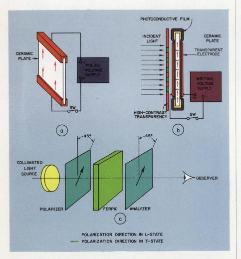
An experimental ferrolectric picture device ("ferpic") is shown in construction and operation: (a) poling the ceramic plate, (b) storing the image, and (c) observing the recorded image.
