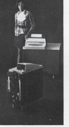
model 37 series: One of the most versatile heavy-duty terminal lines going. Generates all 128 characters of ASCII. Operates at 150 wpm. Prints in upper and lower case.
