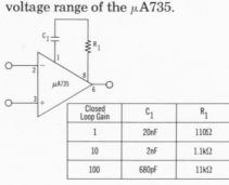
Most engineers like to eliminate those large, expensive, hard-to-find capacitors that hog space and dollars. Here's a nifty little application which will avoid large capacitors in low frequency, active filter design. And with very low supply current drain!
