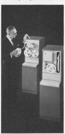
*Telespeed*<sup>TM</sup> *equipment:* A line of high-speed tape-to-tape terminals capable of sending and receiving at speeds of 750, 1050 (shown above), or 1200 words per minute.
