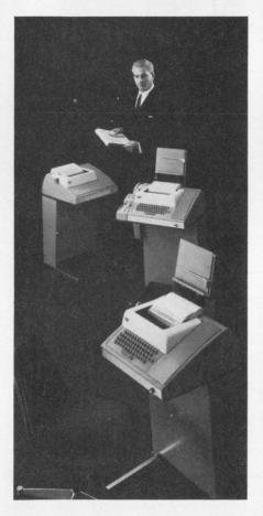
model 33 series: An extremely economical 100 wpm terminal line. Has 4-row keyboard, uses 8-level ASCII code. The most widely used terminal in time-sharing systems today.
