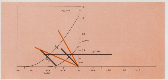
8. If  $R_{\rm s}$  isn't trimmed so that the load line passes through the origin, a voltage will appear at the gate
