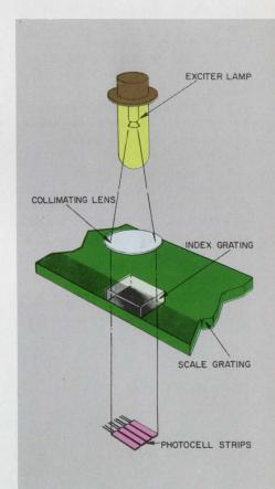
**Moire** fringe systems convert small linear motion into greatly magnified optical signals. This system can detect 0.0001-inch imperfections. In the Longannet scheme, 33 outstations—most of them underground—are connected by two-wire telephone circuits to the computer. Pat Wimbush, sales manager at Ferranti in Dalkeith, Scotland, suggests that the computer system could also handle manpower deployment, timekeeping, wage preparation, materials consumption, stock control and geological prediction.
