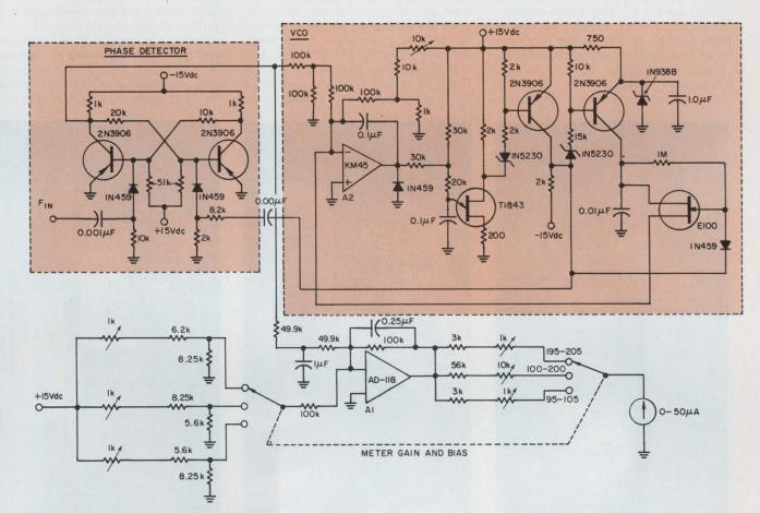
3. VCOs are calibrated with this discriminator circuit which operates from 95 to 205 Hz. Full-scale meter de-
