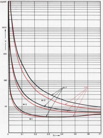
there exists a time beyond which the redundant amplifier configuration is less reliable than a single op amp. Values of M, of course, must be discrete.
