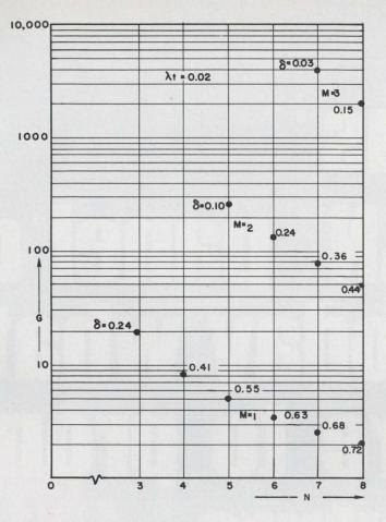
The reliability G of the RAMP for a given mission life decreases as the normalized RAMP output range increases for a given number of failures M.
