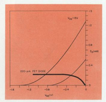
4. FET  $Q_2$  doesn't behave like an ideal current source when its  $V_{\rm DS}$  gets very small (Fig. 1d). Therefore,  $Q_1$  should have a significantly larger  $V_{\rm P}$  than  $Q_2$  does.
