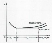
The characteristic failure-rate curve for electrical and mechanical systems has three distinct regions corresponding to the burn-in or debugging, normal operating, and fatigue or wearout periods.
