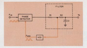
1. The basic loop configuration of the discriminator uses a VCO to provide feedback to the phase detector.
