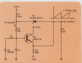
**Operation down to dc** is possible with this linear sweep generator because the zener diode replaces conventional design using a capacitor.
