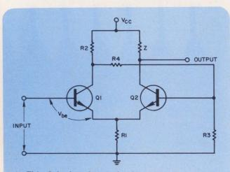
1. This Schmitt trigger circuit can be fully specified by means of the program in Fig. 2.
