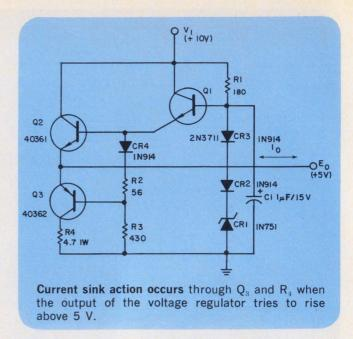
current through  $R_4$ . For the circuit values shown, the output voltage is 5 V, and the supply can sink up to 100 mA of current.
