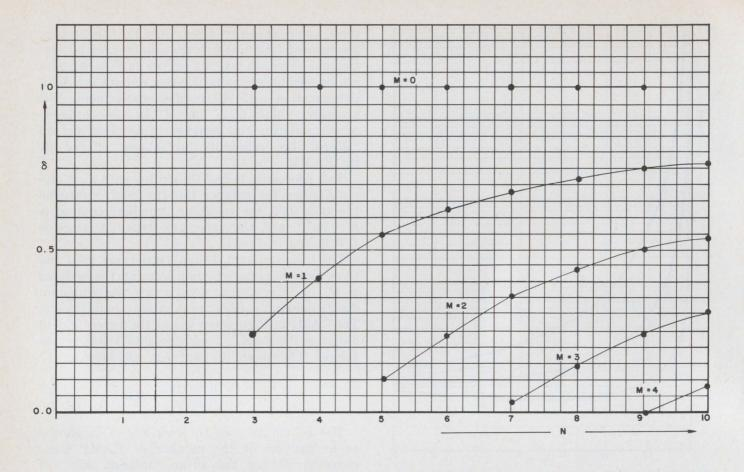
4. The normalized dynamic output range  $\delta$  of the fiveop amp RAMP decreases as the number of failures M increases, each point on the plot representing a possible
