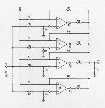
1. The single-input RAMP operates with all op-amp inputs tied together and supplied from a single source. It compensates only for internal op-amp or interconnection failures. The range and accuracy of compensation depend on the number of op amps used.
