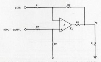
2. The basic element of the redundant amplifier (RAMP) is common operational amplifier.
