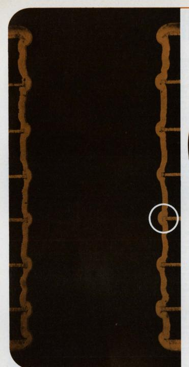
Left: Cross-section (enlarged 70 diameters) of plated hole through typical 8-plane Collins etch-back circuit board.
