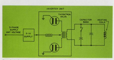
**Two deuterium thyratron tubes** have replaced SCRs in new induction heating furnace. Heating is produced by eddy currents set up in magnetic material. Capacitor bank forces commutation of the dc.
