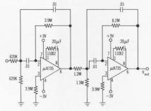
This circuit has a center frequency at 10 Hz, 12 dB rolloff with -3 dB points at 6.5 Hz and 14 Hz. The  $\mu$ A735 lets you use small capacitor values and large resistors for frequency shaping at a few Hz, due to the  $\mu$ A735's low input offset current.
