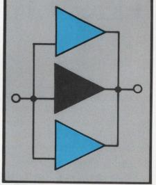
When good op-amp reliability is not enough—when you need ultrahigh reliability—special summing circuits can be the answer. A redundant amplifier (RAMP) connection of several op amps can continue to operate satisfactorily, even after one or more of the amplifiers fails.
