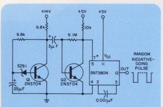
**Random negative pulses** from the monostable multivibrator are triggered from a combination noise generator/amplitude discriminator.
