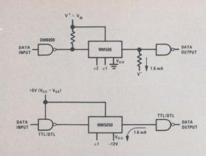
This form of interface can even be used to improve the operating frequency of MOS devices. When the MOS shift register is driving TTL, the total signal swing from a logic "0" to a logic "1" is reduced, hence the delay time is minimized. A long serial delay line, consisting of 1 MHz operating frequency shift registers, can be made to operate at 2.0 MHz by this method.
