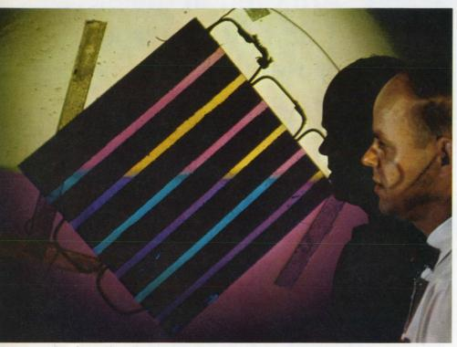
**Dr. Gene Haertling** looks at a projected view of a new transparent ceramic. Varying the voltages between electrodes (dark bands) changes the bire-fringence. This causes polarized white light shining through the material to be converted into colored light.
