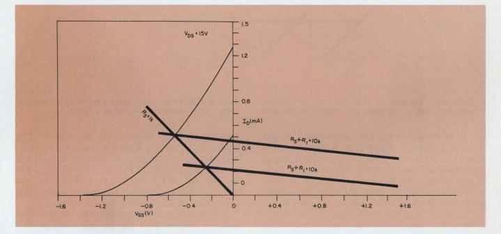
6. The bias load line is set by  $R_{\rm s}$  but the output load line is determined by  $R_{\rm s}+R_{\rm 1}$  when gate feedback is employed
