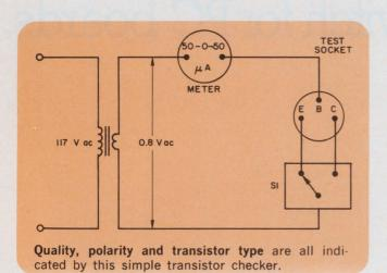
under test is considered defective; that is, it is either open or shorted. If the junction is good, the meter will immediately deflect to one side or the other of zero, depending on whether the device under test is an npn or a pnp.
