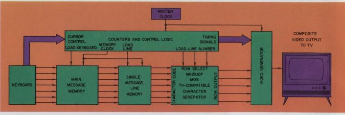
**3. Mostek technique** for connecting a standard keyboard to a TV set. An MOS 2240-bit, read-only memory func-
