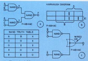
1. The wired-OR connections can eliminate gates in a DTL logic design. The three NAND gates (a), which perform the function f = AB + AC (b), for instance, can be replaced by two identical NAND gates with their outputs jumpered (c).
