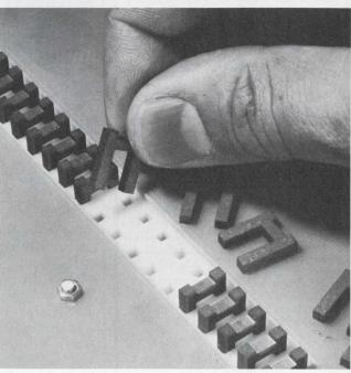
able U cores and I bars. The retainers for these components are plastic so that the retainers, instead of the components, are wrapped with the sense winding.
