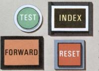
plays. Units available in 34" x 1" rectangular, 34" square, 54" round and 5% square designs. Bezels with or without barriers in black, gray, dark gray or white. Legends are positive or negative—either visible or hidden when "off." Switches are momentary or alternate action and low level to 125V at 5A, resistive.
