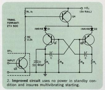
(about 100 pF) included to make the collector circuits of  $Q_1'$  and  $Q_2'$  dissimilar: this ensures that the multivibrator will not block. Conventional design consideration governs the choice of C,  $R_L$  and  $R_B$ . Power dissipation is zero in the standby state.
