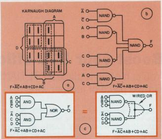
4. Significant savings in gate count result for some logic functions (a). In this case a simple NAND circuit requires five gates (b), but a simplified AND/NOR circuit uses three gates and a NAND/ wired-OR equivalent uses only two gates.
