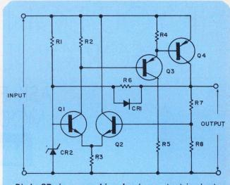
**Diode CR** $_1$  is reverse-biased unless output is shorted. Forward bias during short circuit protects power supply.
