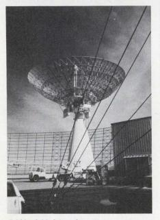
RAM vhf/uhf radar measures cross section of reentering payloads.
