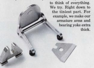
Thicker than years of testing and use say they have to be. Then, to make sure they don't cause wear problems, we insert a hardened shim between the hinge pin and the frame. The pin rides on the shim, instead of wearing into the heelpiece. (You can forget the bearing, it's permanently lubricated.)
