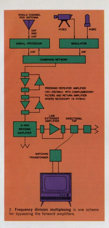
filter pair is reciprocal and therefore acts as a combiner as well as a splitter. The high-band port of each filter is connected to the forward amplifier. The low-band ports can be connected together—with a straight run of cable—as a lowfrequency bypass, or a reverse direction amplifier can be inserted. Since there is less loss at lower frequencies in the reverse direction, fewer amplifiers are needed.
