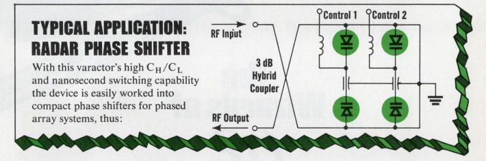
You can also use this binary varactor for RF Switching Digitally Controlled Oscillators and Filters Continuous Tuning Wideband VCO's and Filters Large Deviation FM Oscillators Negative Resistance Parametric Amplifiers Etc.
