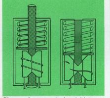
**Plunger in nonexplosive initiator** is released when wire is heated to the point where it breaks under tension.
