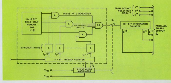
23. Low-speed Type III converter has a 1000-per-second conversion rate and  $\pm 0.05\%$  accuracy.
