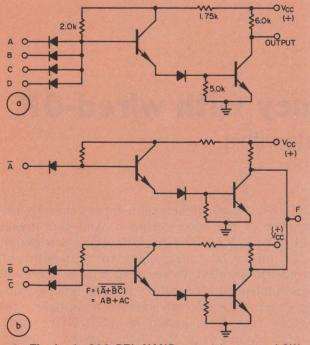
2. The basic 930 DTL NAND gate (a) gives a LOW output only if all inputs are HIGH. A simple connection of the output leads of two of these gates (b) results in an additional OR function; the combined outputs is LOW if either output is LOW.
