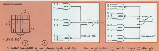
designer must be cautious. For some functions (a), the same number of gates is required after Boolean simplification (b), and for others (c) attempts at simplification result in an actual increase in the number of gates required (d). proper form
