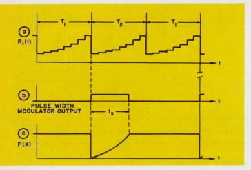
24. Simulated arc-tangent derivative (a) is switched to integrating counter by pulse-width modulator signal (b). Counter content (c) approximates arc-tangent function over period  $t_x$ .
