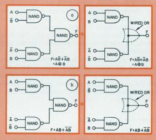
5. An exclusive-OR function at a one-gate saving (a), and a two-input coincidence detector, also at a one-gate saving (b), from NAND/wire-OR.
