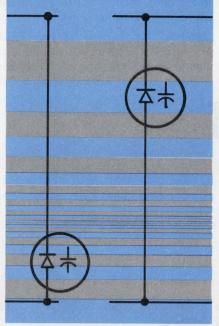
Designing a varactor-tuned oscillator for high-power operation is complicated by a consideration that doesn't have much importance in low-power circuits—loading of the oscillator circuit by the diode.
