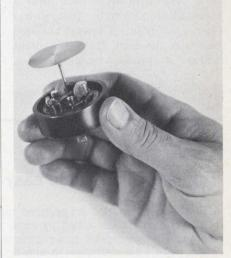
A disc-topped rod plus electronics make up the Voltage Probe Antenna
