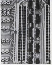
A new read-only core memory, which can have its program altered without being returned to its manufacturer, offers capacities to 20,480 bits at a cost of only  $2.5\phi$ per bit. Called the VROM, it has a mechanically interchangeable braid and diode board, thus permitting users to maintain a library of plug-in fixed-program tables.
