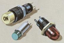
many thousands of Datalites and subminiature indicator lights available from Dialight. Variety of lens shapes, colors and finishes. Many different positive or negative legends. Incandescent 1.35-120V; neon—high brightness at 110-125V AC and standard brightness at 105-125V AC-DC. For clearance holes from  $\frac{9}{32}$ " to  $\frac{17}{32}$ ".
