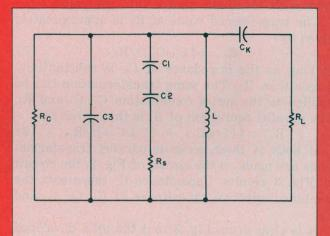
2. The effective series resistance,  $R_{\rm s}$ , of the diode should not be neglected when analyzing the loaded tank circuit.  $R_{\rm c}$  is the effective shunt resistance of the transistor,  $R_{\rm L}$  is the load and  $C_{\rm K}$  couples the load to the oscillator. Only rf components are shown.
