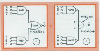
3. AND/NOR (a) and NAND/wired-OR (b) gates perform equivalent functions if connected in similar patterns. The designer performs Boolean calculations to minimize the gates in an AND/NOR system; then he replaces AND gates with NAND gates, NOR gates with the wired-OR connection.
