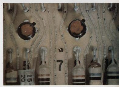
This printed-circuit board appeared clean after manufacturing. However, corrosion spots developed with time. They proved to be etching and plating solution residues that bled to the surface.
