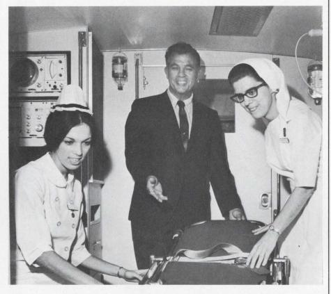
**Electronic monitoring equipment** is mounted inside the van within convenient view of personnel on either side of the stretcher.
