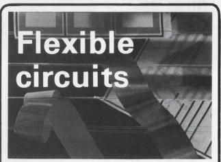
Kapton\* or Mylar\* flexible printed circuits are a specialty at Buckbee-Mears. We make them to standards of precision unsurpassed in the industry. We produce small wires to two mil apart on four mil centers, sizes up to five feet square. Tolerances held to ±.0002 inches on wires and space, shrinkage control guaranteed.
