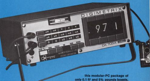
only 0.1 ft³ and 5¾ pounds boasts, along with much more, three-digit "Nixie" readout to 1200 with decimal point, automatic + and -, and an extra digit for accurate readings ±20% overrange, plus built-in galvanometer showing variation, amplitude, and range of measured parameter;
