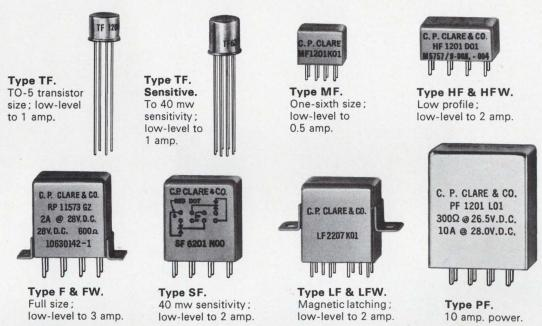
Industrial/Commercial Relays. A combination of economy and rugged construction to meet industrial/commercial requirements. Industrial/commercial versions are rated for 30 G shock and 10 G vibration.
