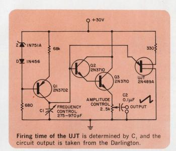
the UJT. At this point,  $C_1$  discharges through the UJT in one microsecond. Varying  $C_1$  adjusts the frequency of the sawtooth wave from 5 to 200 kHz. The charging capacitor is applied to the output terminals through a Darlington amplifier. The very high input impedance of the Darlington circuit does not load Q1, and hence will not affect the linearity.
