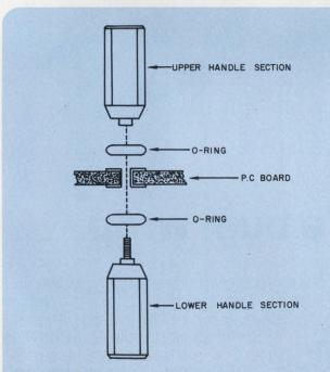
Simple PC board land-masking fixtures use O-rings to mask against the encapsulent (photo). Four such fixtures are used on this PC assembly during encapsulation.
