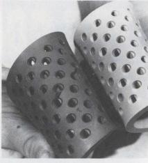
Mold life doubled. New RTV-630 silicone molds last twice as long as conventional silicones in molding epoxy parts for electronic modules. Tear strength of 100 lb/in (die B) makes "630" the toughest RTV yet...without sacrificing flexibility.
