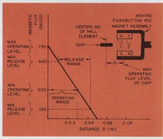
A U-shaped piece of iron with two polyvinyl magnets is the magnetic structure of the Honeywell solid-state switch. The chip is stationary, and the magnets move.
