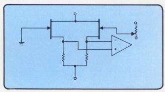
2. With potentiometer in one gate circuit the dual JFET cannot reduce common-mode errors due to high  $V_{\rm p}$ . A discrete JFET pair would also exhibit this difficulty.
