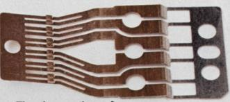
Then there are the contact springs. Ours are phosphorbronze. Others use nickel-silver. Our lab gave this stuff a thorough check, but found nickel-silver too prone to stress-corrosion. Atmospheric conditions which cause tarnish and ultimately stress corrosion have almost no effect on phosphor-bronze.
