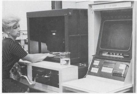
**IR temperature-sensing instrument**, developed at Autonetics to detect flaws in microcircuits, detects minute temperature differences on the surface of the human body and displays them on a CRT screen.
