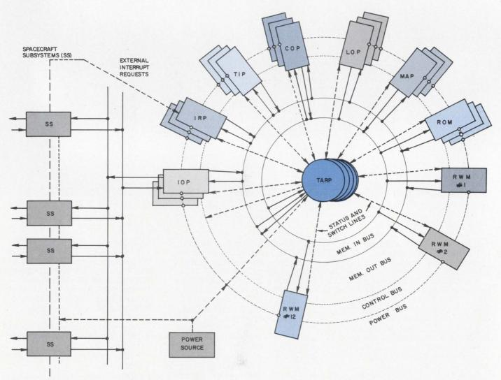
Self-testing and repairing computer (STAR) block diagram. The computer is essentially a replacement system. Test and repair processor (TARP) monitors status re-
