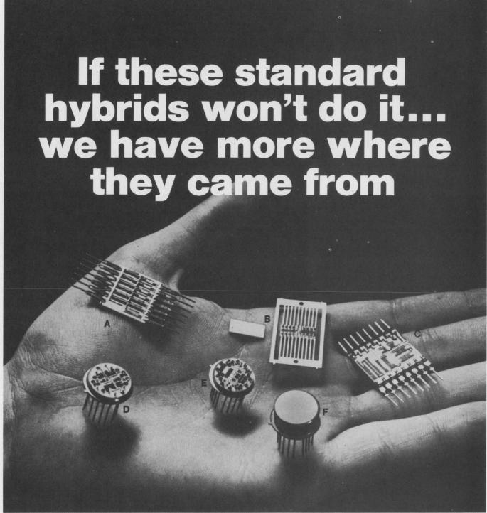
Standard hybrids featured in MEPCO "circuit of the month" program: A D/A binary voltage summing ladder; B ceramic sandwich resistor flatpack; C D/A binary current summing ladder; D DTL to MOS level shifter; E precision high speed ladder switch; F relay, lamp, core driver.
