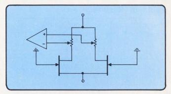
1. With potentiometers in source circuit this dual JFET requires touchy, time-consuming adjustment and the cost of the extra pot. If this circuit is used a pair of discrete JFETs, it would also show poor temperature tracking, and poor  $I_{\rm dss}$ ,  $V_{\rm p}$  and  $y_{\rm fs}$  tracking.
