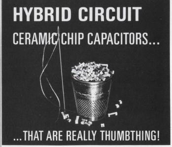
Put your finger on those so-and-so design problems with a selection of type K 1200's. Capacitance range is 10 pF to 2.5 Mfd. Dissipation factor is less than 2% @ 1 kHZ. Working voltages available, 25 thru 200 WVDC and more. Tempco is  $\pm 15\%$  max.  $-55^{\circ}$ C to 125°C. Our full line meets the applicable portions of MIL-C-11015 and MIL-C-39014.
