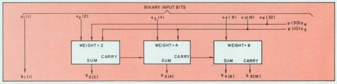
4. The reducing circuit cuts the binary output down to a maximum value of 29, and generates carry outputs
