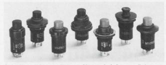
Cutler-Hammer's new military pushbuttons include seven distinct configurations, screw and solder-lug terminations, five double-break contact arrangements, and momentary-contact and push-pull types.
