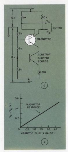
7. **The Magnistor is connected** in the circuit shown above. The outputs from the two collectors are then applied to a differential amplifier.
