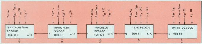
1. The binary-to-BCD decode circuit is defined in block form by the basic conversion equations. A logic circuit
