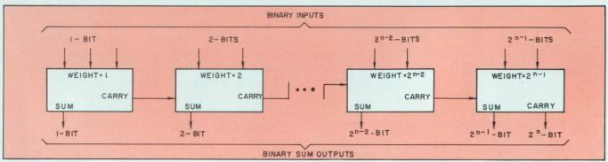
2. The standard binary n-bit adder is built from full-adder circuits. Although it offers a limited number of
