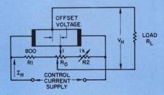
3. Hall connection misalignment is a principal problem. The circuit above compensates for the offset voltage.
