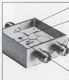
CIRCUIT FRAME ASSEMBLY—Consists of mounting enclosure, coax-to-microstrip transitions (launchers) and all mounting hardware. Accommodates Microwave Integrated Circuits (MIC's).
