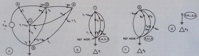
3. Generating the network graph is the first step in the analysis (a). The subgraphs for  $\Delta P_1$  (b),  $\Delta P_2$  (c) and  $\Delta P_3$  (d) are also shown. Note that subgraph  $\Delta P_3$  is only a single node. This has a value of unity.
