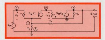
2. This equivalent circuit of the amplifier of Fig. 1 can be applied to other amplifiers with similar feedback and different biasing arrangements.
