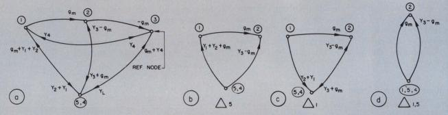
4. To evaluate the denominator, open-circuit all of the independent current sources and short-circuit all of the independent voltage sources. When this is done to the graph of Fig. 3a, the result is that shown in "a." The subgraphs  $\Delta_5$  (b),  $\Delta_1$  (c), and  $\Delta_{1.5}$  (d) are also shown.
