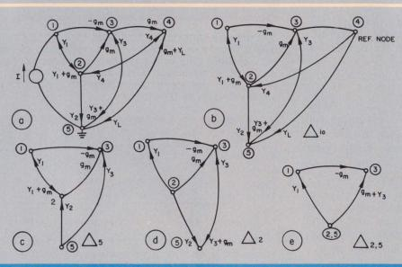
6. The input impedance is found by using the graph (a) to calculate the voltage at node 1. To evaluate  $\Delta_{\rm io}$ , the current source is open-circuited (b). The subgraphs  $\Delta_5$  (c),  $\Delta_2$  (d) and  $\Delta_{2,5}$  (e) are also shown.
