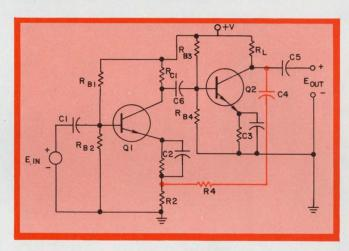
1. Extremely stable gain, high input impedance and low output impedance characterize this voltage-series feedback amplifier. It's called a voltage-series type because a portion of the output is fed back (via  $R_4$  and  $R_2$ ) in series with the input. When properly designed, the amplifier's gain is  $(R_2+R_4)/R_2$ .
