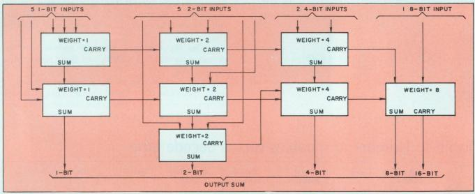
3. Adders are ganged by using the sum and carry outputs of all full adders as inputs to other adders or as
