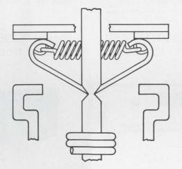
3. The contacts snap up into place and close the NO circuit. This positive snap action provides 120 grams of contact pressure and contact resistance below 10 milliohms-perfect for dry circuits.
