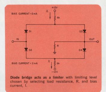
tortion below the limiting level will occur from dc to about 1 MHz. The limiting level is independent of temperature. The circuit has relatively low output and high input impedances.
