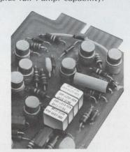
Need 2-amp. performance? The Model BR10 will operate dependably at 2 amps. (28 VDC), through 100,000 operations, in the temperature range —65 °C to +125 °C. Contact our Applications Engineering Group for further details.
