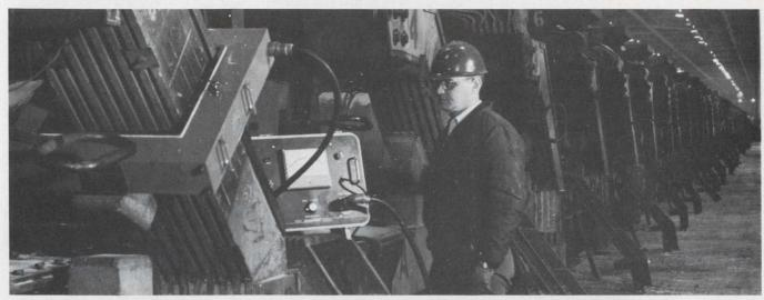
The venerable Hall-effect device is finding ever wider use in a variety of industrial and aerospace applications. Here, a Hall current-
