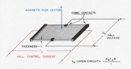
The Hall generator output is a voltage that is proportional to the product of magnetic field intensity and control current.
