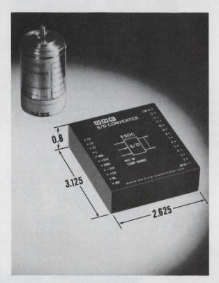
DDC has a new encapsulated module, only 6.6 cubic inches, which offers true 14-bit continuous conversion. The 8 ounce device, called the ESDC, has a specified accuracy of  $\pm 4$  minutes  $\pm 1$  LSB over the full operating temperature range. This spec takes into account all errors due to input rates to 360°/second, accelerations to 20°/sec², harmonic distortions to 10%, frequency variations to 10%, and amplitude variations to 10%. The 2.6" x 3.1" x 0.8" high module is designed for
