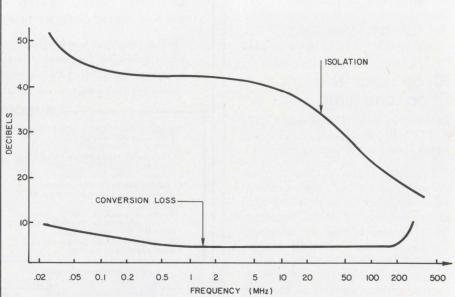
**Minimizing conversion loss and maximizing isolation**, a new transistor-sized double-balanced mixer spans the frequency band of 25 kHz to 500 MHz. Occupying but 0.05 cubic inches, this microminiature device holds conversion loss to 10 dB maximum and keeps isolation to 15 dB minimum.
