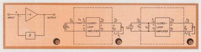
1. The general feedback amplifier (a) may be considered as a two-port network driven from a voltage source (b) or a current source (c). On this basis, the forward and feedback paths can easily be analyzed separately.
