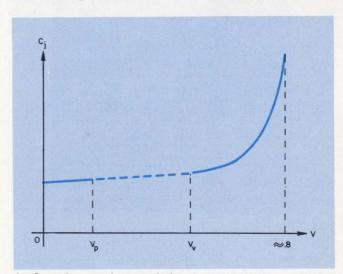
3. Capacitance characteristic of tunnel diode resembles that of an ordinary diode but is difficult to measure within the negative resistance region.
