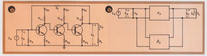
4. Typical shunt-shunt configuration (a) is best analyzed using y parameters (b). This selection of parameters is
