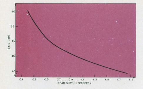
4. No freedom exists to specify the antenna gain once the coverage area is chosen. Here antenna gain is plotted against 3-dB beamwidth at a frequency of 4 GHz. The gain equation is given in Fig. 1, the formula for 3-dB beamwidth is  $\Theta = 7 \times 10^4$ /fD, where f is the frequency in MHz, D is the antenna diameter in feet, and  $\Theta$  is expressed in degrees. (Both formulas are from ITT's "Reference Data for Radio Engineers," fourth edition, p 753).
