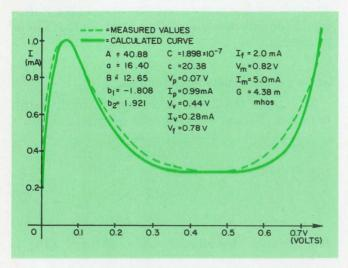
6. Static V-I characteristic for 1N2929 tunnel diode illustrates the closeness to fit that can be obtained by the curve-fitting method.
