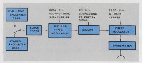
Block diagram of the 16,200-bit-per-second Mariner data-transmission system.
