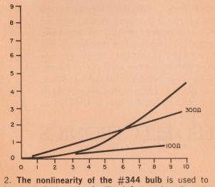
increase the negative feedback factor when the output increases. 100  $\Omega$  and 300  $\Omega$  lines are shown for reference.
