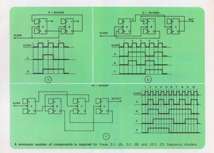
puts of J-K flip-flops. Minimum-hardware frequency dividers of this type for factors of 3, 5, and 10 are shown in the illustrations. These arrangements are suitable for either DTL or TTL J-K flip-flops.
