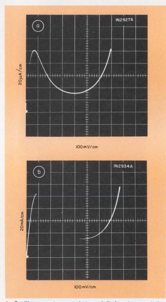
4. Oscilloscope traces of tunnel-diode characteristics facilitate measurement of peak, and valley points. The loss of detail in the negative resistance region of the 1N2934A makes measurement of  $V_{\rm g}$  difficult.
