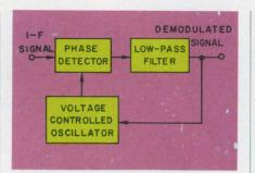
6. A phaselock loop can' serve as a threshold extension fm modulator. Since the VCO is made to follow the i-f, its control voltage is the demodulated output.
