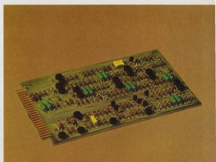
Typical printed circuit board used in the MDS 1101 Data-Recorder, showing the extensive use of Allen-Bradley hot-molded ¼ watt resistors.
