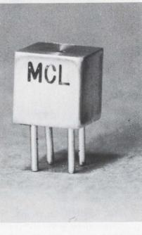
a new microminiature double-balanced mixer operates from 25 kHz to 500 MHz with a typical noise figure of less than 6 dB. This tiny device, model ASK-2, features a volume of only 0.05 cubic inches, occupying approximately the same board space as a TO-5 transistor package.
