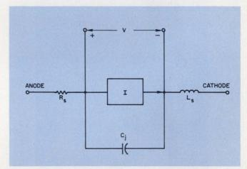
Topology of tunnel diode depicts the lumped parameters that must be evaluated.
