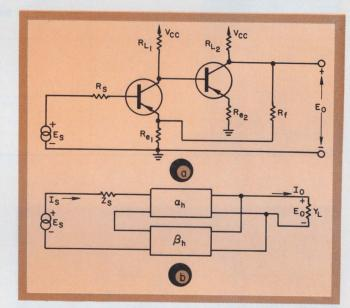
3. Typical shunt-series configuration (a) is best analyzed using g parameters (b) since I<sub>o</sub> is common to both the forward and reverse networks and Es is across both networks.
