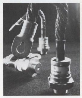
**Power plus.** New SCR has 450-A rating and PIV of 1200 V, p. 97.
