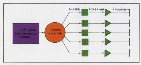
3. Phaser losses can be made unimportant through use of a separate power amplifier for each radiator. The amplifiers can be true amplifiers, or perhaps oscillators that are phase-locked to the input signal. In any event, this approach won't be practical until very lightweight reliable solid-state amplifiers are made available.
