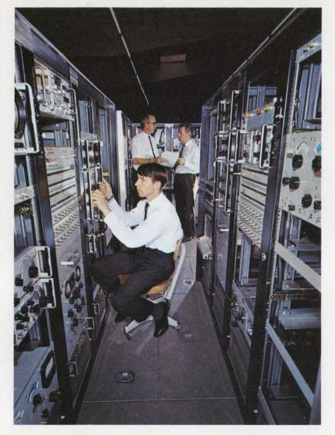
**Checking out a satellite isn't simple.** This mass of gear at Hughes Aircraft in El Segundo, Calif., is only part of the transportable systems test equipment needed to check out an Intelsat IV.
