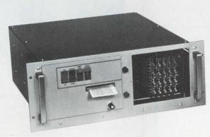
Printed circuit boards, with easily accessible switches permit unusual flexibility for Programmable Zero Suppress.
