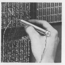
Probe lights up to check logic levels in a flash
