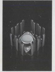
T03's, T066's, T015's and other case-mounted devices can be operated with many times more power when mounted in UP's. In still air, the staggered fingers dissipate by radiation and convection. In forced air, turbulence moves the air around each finger. Efficient in any direction. Outperforms extrusions dramatically.
