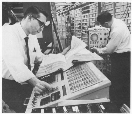
Master control center for New York Telephone Co.'s electronic switching system, one of five in the city. It handles 40,000 calls an hour and serves about 10,000 telephone customers.
