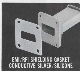
CONSIL  $\blacksquare$  Highly conductive, low volume resistivity; .001 ohm-cm³  $\blacksquare$  All pure silver-silicone rubber compound; 30 to 80 durometer  $\blacksquare$  Operating temp.  $-65^{\circ}$ F. to  $+450^{\circ}$ F  $\blacksquare$  Available in sheets, molded components, cut gaskets and connector gaskets  $\blacksquare$  Write for data #850, and FREE sample.
