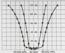
SPECIFICATION filter (A) 1 db Bandwidth 35 KHz Min. 6 db Bandwidth 45 KHz Min. 60 db Bandwidth 90 KHz Max. Ultimate Attenuation 80 db Impedance 50  $\Omega$  in & out Ripple 1 db Max. L.L.  $\leq$  4 db ENVIRONMENTAL: TR  $-55^{\circ}\mathrm{C}$  to  $105^{\circ}\mathrm{C}$  Vibration—Mil. Std. 202
