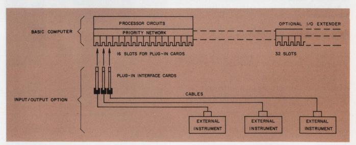
1. Computer interfaces with testers through a series of plug-in interface cards. Circuitry on the cards can be
