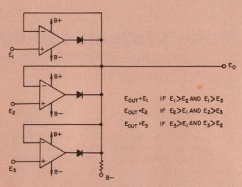
6. A trio of operational amplifiers passes the most positive signal. The effect of the diode drop is reduced by the loop gain of the amplifier. This is the P gate of Figs. 7 and 8.
