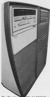
The Birtcher Model 8000 Component Test System automatically tests multiple lead components and circuits from simple IC's to over 200 lead logic cards, MSI, LSI units. Modular design allows flexible test applications providing a system that is never obsolete.
