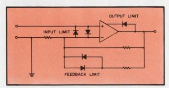
11. Latch-up is prevented by limiting the input or output voltage excursions with diodes or by increasing the feedback with diodes or zeners in the feedback line. Protection is needed because input transients are common.
