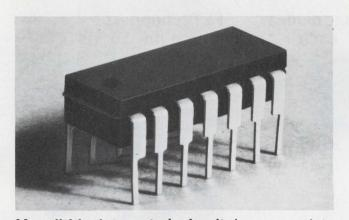
Monolithic integrated circuit is a complete a-m radio receiver on a single chip, p. 254.
