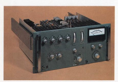
Combining the reliability of solid-state construction with the desirability of remote operation, a new L- and S-band signal generator can be programed for rf output frequency and level, as well as subcarrier frequency.
