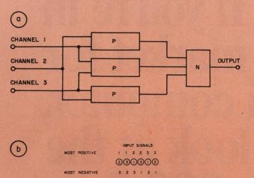
7. Three two-input P gates are combined with a three-input N gate (a). The 3! combinations are arranged in a truth table (b). The chosen signal, always the middle magnitude, is circled.
