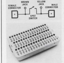
A Break-Out Box is designed to reduce hook-up and testing time. It offers a convenient method to measure or interrupt voltages, currents, and/or signals between any two pieces of equipment. A flip of a switch instantly opens or closes any circuit. Cumbersome shorting plugs are no longer necessary. It comes in a variety of connector configurations, is of rugged construction, low in cost, and available off-the-shelf.
