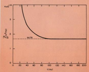
2. Resistors generate 1/f noise, so called because its power spectrum is roughly proportional to the reciprocal of frequency, in addition to the thermal noise component described by Johnson and Nyquist.
