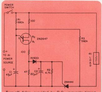
**Turn-off delay,** provided by R<sub>2</sub>C<sub>2</sub>, prevents timing circuit from commutating the SCR during short power interruptions.
