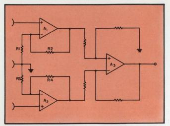
7. The compound differential circuit uses matched-gain, non-inverting preamplifiers before the common-mode rejection stage. Differences in gain between  $A_1$  and  $A_2$  lead to poor CMRR, of course, but the problems associated with the high, but variable, impedance of the biological source are avoided.
