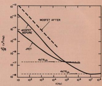
15. Noise voltages of field effect transistors, referred to the input, show that low-frequency excess noise predominates over a wide range, and that the junction FET has less low-frequency noise than the MOSFET. This is to be expected, since in the MOSFET, conduction occurs in the vicinity of surface states.
