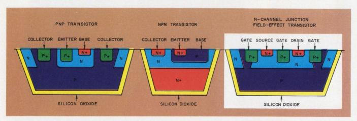
Achieving true interchannel isolation, a new monolithic 16-channel analog multiplexer forms near-ideal on-thechip analog switches by combining complementary bipolar transistors with n-channel junction FETs. This large-scale integrated circuit uses dielectric isolation to separate all structures, both horizontal and vertical.
