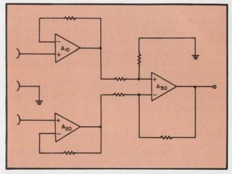
8. Voltage follower preamps improve the compound circuit because preamp gains are closely matched (close to unity), and the CMRR is limited only by the CMRR of the optimized differential stage A<sub>3</sub>.
