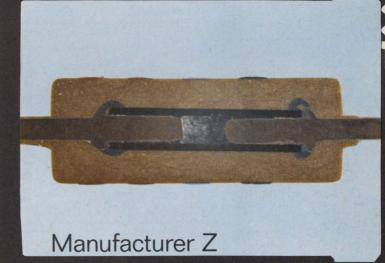
The above illustrations are from unretouched photomicrographs taken of four ½-watt fixed resistors. Compare the anchoring of the leads, the seal provided by the insulating jacket at the ends, the homogeneity of the resistance material, the sharp color code bands—and decide for yourself.
