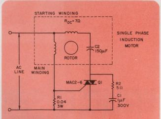
Triac allows current to flow in start winding until backs EMF reduces main winding current to near steady-state level.
