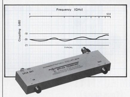
The Model DCM1-20 broadband 20 dB directional coupler covers the frequency range from 1,000 to 12,400 MHz. Its small size, light weight and excellent specifications make it useful for internal leveling, broadband power monitoring and reflectometer measurements. It is ideal for airborne systems which operate under severe environmental conditions.
