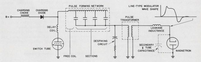
2. Risetime limitations make the conventional line-type pulse modulator unsuitable for the generation of very
