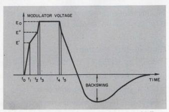
1. The critical period from  $t_1$  to  $t_2$  is the only interval over which there is a limitation on the RRV.
