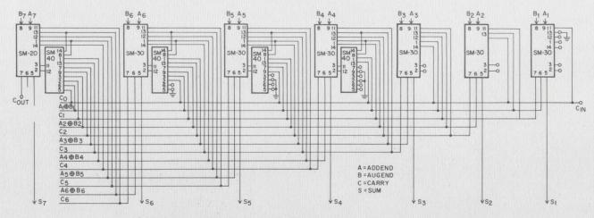
Fig. 2. Seven-bit section can be used to expand 8-bit unit shown in Fig. 1.
