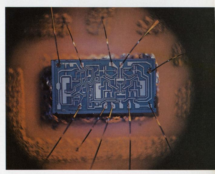
Monolithic integrated circuit chip containing three operational amplifiers will be used in a hybrid active
