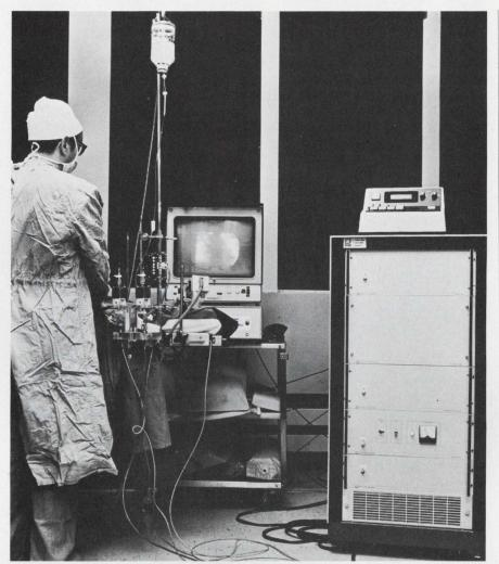
Video disc recording system (right), developed by Data Disc Corp., is connected to standard X-ray equipment at Stanford University Medical Center in Palo Alto, Calif. The X-ray motion pictures are recorded and played back at slow speed for the physician.
