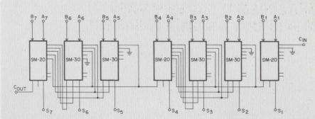
Fig. 4. Three-bit section can be used to expand 4-bit adder.
