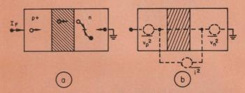
7. Current flow through a pn junction includes resistive flow of electrons and holes through the n and p regions, with associated resistance noise, and recombination in the depletion region, with associated shot noise (a). A simple model includes all of these noise sources (b).
