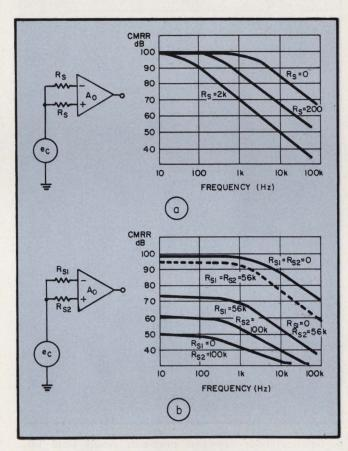
5. The CMRR of a 709 op amp is reduced, and the corner frequency is lowered, if the source impedance is increased (a). If the source impedances are unbalanced (b), the CMRR is decreased at all frequencies, and the corner frequency is further reduced.
