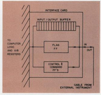
Typical interface card shown here contains storage and control circuitry.
