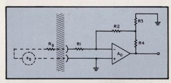
4. A further deterioration in CMRR results from this modification of the voltage divider feedback arrangement, although gain stability is improved due to increased input impedance. Typically,  $R_s=2~k\Omega$  to 150  $k\Omega,~R_1=1~M\Omega,~R_2=1~M\Omega,~R_3=100~\Omega,~R_4=10~k\Omega,~A_o=30,000,~and gain is 90 to 100.$
