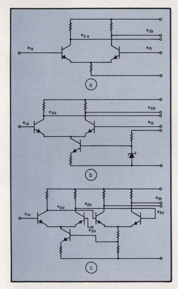
2. The differential pair is an essential part of every biological amplifier (a). For better common-mode rejection the common emitter resistor is replaced by a constant current source (b), which can be controlled by the common-mode output of a second differential stage (c).
