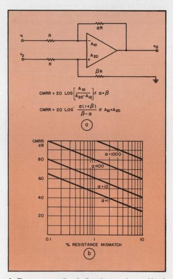
9. The common-mode rejection stage can be considered as an amplifier providing two uncoupled voltage gains to the signals applied to the two inputs. The CMRR is dependent on the matching of both the amplifier gains and the resistor ratios (a), and increases as the closed-loop gain,  $\alpha$ , is increased (b).
