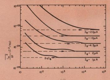
12. The noise current of a planar silicon transistor, referred to the input, closely follows Schottky noise at frequencies above a few kHz. At the lower frequencies, excess 1/f noise become significant.
