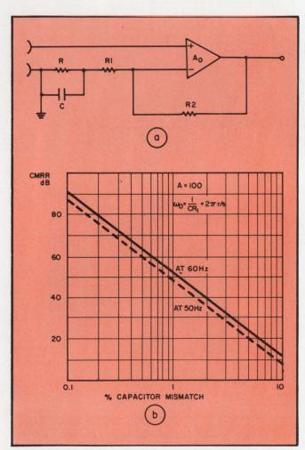
10. **Dc noise can be blocked** by a series RC circuit (a), but the capacitors must be carefully matched or they will degrade the CMRR (b). Such degradation is often the controlling factor in determining CMRR.
