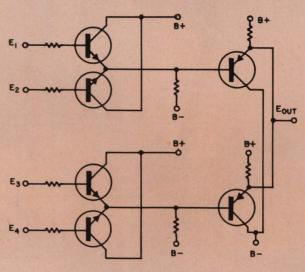
4. Transistor circuit compares four inputs and passes the second most positive.
