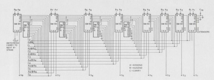
Fig. 1. Anticipated carry adder is up to 4.5 times faster than adder systems using ripple carry propagation.
