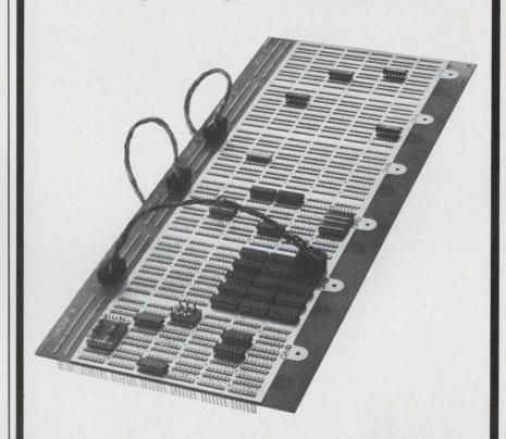
Simplifies design and production operations. Saves time and space. Direct mounting chassis eliminates need of logic cards — increases flexibility in prototyping, production and field service. A unique two dimensional approach to IC packaging with these outstanding features:
