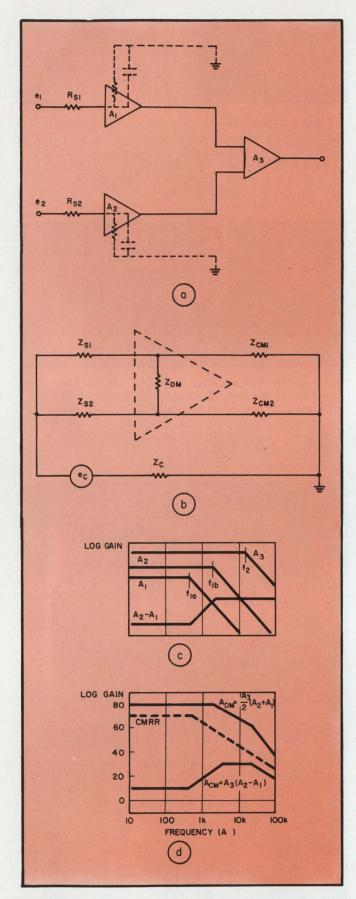
6. Common-mode rejection problems result from imbalances in the input stages of the op amp (a), which results in an imbalance of the equivalent bridge circuit (b). The difference in the input impedances of  $A_1$  and  $A_2$  results in gain curves as shown in (c). Subtraction of log gains  $A_{\rm DM}$  and  $A_{\rm CM}$  gives the CMRR (d).
