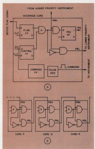
2. **Interrupt circuitry directs computer's** attention to the test instrument having the highest pre-established priority. When interrupt service is completed, other instruments may interrupt the computer.
