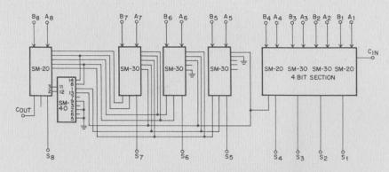
Fig. 5. Somewhat faster addition times can be obtained by using SM-40 expander to add 4-bit sections to basic 4-bit system.
