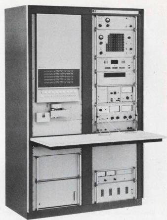
4. H-P Model 9500A Automatic Test System is used as an example of the application of the interface design ground rules described in the article.
