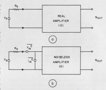
B. A circuit model of a noisy amplifier consists simply of a noiseless or ideal amplifier with noise sources  $\overline{v_{in}^2}$  and  $\overline{i_{in}^2}$  connected to its input. The noise sources represent the mean square values of the corresponding voltage and current fluctuations, and are chosen so that the resultant output noise power is equivalent to that of the real amplifier.
