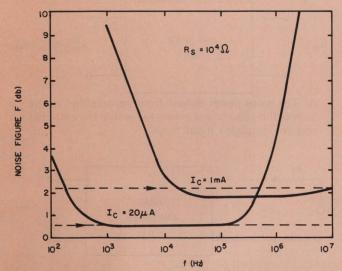
14. The measured noise figure of a planar silicon transistor corresponds to the noise figure calculated from the model only for mid-range frequencies. At low frequencies the 1/f excess noise predominates, and at high frequencies the decreased current gain of the transistor leads to an increase in the noise figure.
