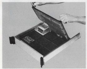
When you specify EECO 2D Hardware a computer converts your "Pin Logic List"\* into a wire plan and checks for errors and omissions before wiring begins. EECO plugs in the IC's, machine Wire-Wraps the backplanes and in days...your schematic is a drawer of working electronics with all necessary computer generated support documentation.
