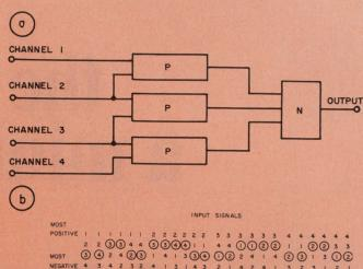
8. Using the same combination of gates as in Fig. 7, but with four inputs instead of three, one of the middle signals will pass (a). The circled number in the truth table (b) shows which one it is.
