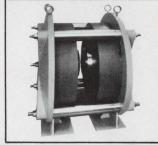
Moderately priced and specifically designed for high performance with flexibility and accessibility. Five models – 4, 4V (4 inch diameter), 7, 7V (7 inch diameter) and 10 (10 inch diameter). Magnet pole cap surfaces are precision ground and polished to optical tolerances to achieve optimum magnetic uniformity. 4V and 7V models are variable gap models with continuously adjustable spans. All magnets are capable of providing a stepped variable gap by means of precision ground spacer blocks.
