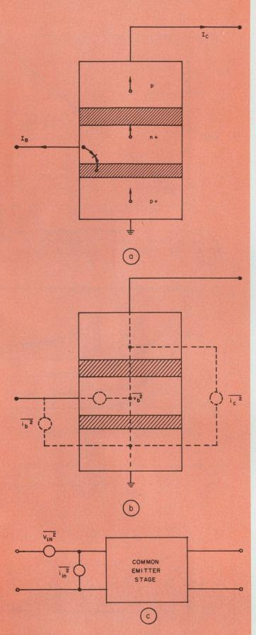
10. The noise generated in a transistor, in the commonemitter mode, is due to shot noise in the collector current and resistance noise and shot noise in the base current (a). A circuit model includes these effects by using the standard noise generators (b) and can be modified to refer all noise to the amplifier input (c).
