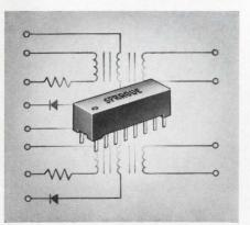
A single module may contain up to four identical circuits. They're particularly useful in memory systems where a similar repetitive pattern exists.
