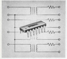
You get pulse transformers and resistors (diodes and capacitors) (can also be included) in a circuit tailored to your specifications.
