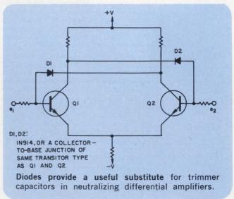
This technique is also suitable for use in linear IC amplifiers, many of which use a differential amplifier in their front end.
