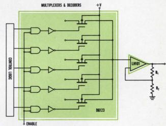
Only one TO-86 package is required to accomplish the above switching functions. Packages include switch drivers that accept standard DTL, RTL, or TTL logic signals.
