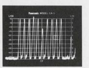
Subcarrier level changes Often a subcarrier level changes with a resulting communications malfunction. This display on the CRT shows that one subcarrier's level is down 12 dB. Another is over the predetermined acceptable level.
