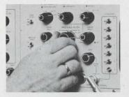
2. A selector knob sets the frequency scale in one of five settings from 15 Hz/division to 1.4 kHz/division. Interlocked circuit functions in the analyzer automatically optimize the display for any setting of the frequency scale.
