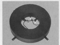
Dual section potted delay line. Outer race accounts for 980 nanoseconds; an inner nest exhibits 61.1 nanoseconds of delay. 50 ohm coaxial cable .215" diameter. Weight is 25 pounds for the 16" diameter, 3" high package.
