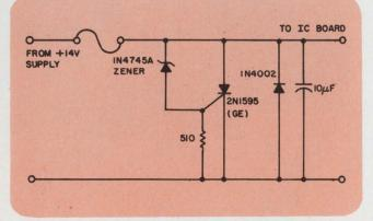
Protection against overvoltage and polarity reversals is provided by this inexpensive circuit. gate voltage of 0.8 V. The 5 per cent 1N4745A zener diode breaks over at a maximum of 16.8 V, so that the SCR turns on at an input voltage of 17.6 V or less, and does so in less than one microsecond. This is compatible with the +18-V limit of the particular ICs being protected.
