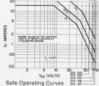
energy reliability that's needed for very tough switching jobs—resistive or inductive. The 28-volt shunt regulator above, for example, is amply handled by the DTS-103 ( $V_{CEX}$  of 80 volts). For complete data on this circuit, ask for our application note No. 42.
