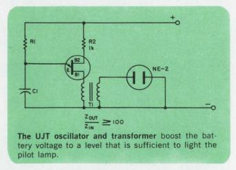
supply voltage is in the 6 to 40 volt range. For very low voltage operation, a 2N2840 should be used, which will operate with voltages as low as 1.5 V. The values of  $R_1$  and  $C_1$  will determine the frequency of oscillation.
