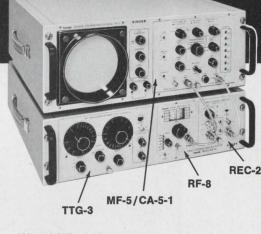
Model MF-5/CA-5-1 Spectrum Analyzer display section features high resolution/low distortion and 70 dB dynamic range.
