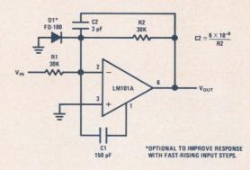
FIGURE 2. Feedforward Frequency Compensation
