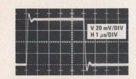
FIGURE 4. Small Signal Transient Response with Feedforward Compensation
