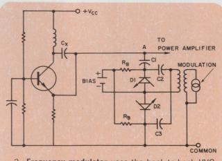
2. Frequency modulator uses the back-to-back VVC configuration to control a modified Colpitts oscillator.
