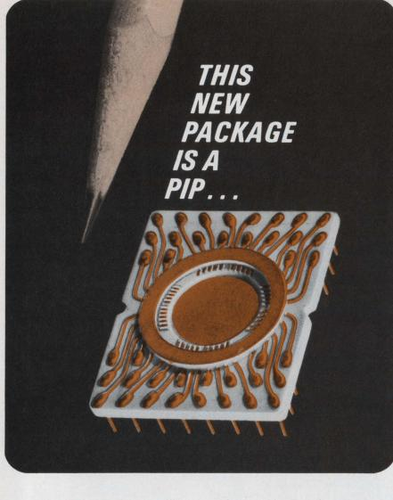
It's a 40-pin Plug-in-Package (PIP) from the Cermetron Division of National Beryllia—30% lighter, and with 8 to 10 times the thermal conductivity of similar packages using other materials, because it is made from BERLOX—Beryllium Oxide.
