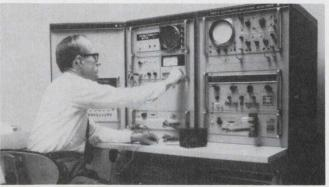
(illustration Intradyne-owned Computer-Controlled Network Analyzer (HP-8540)
