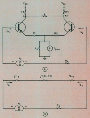
4. Differential amplifier with floating input (A) has the equivalent of (B). It can be handled with the equations of Table 1, using the appropriate D.
