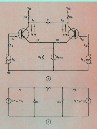
2. Differential amplifier with single-ended voltage sources (A) has the equivalent circuit of (B).
