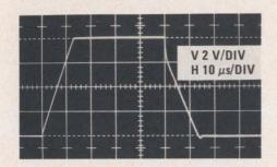
FIGURE 6. Large Signal Transient Response with Standard Compensation
