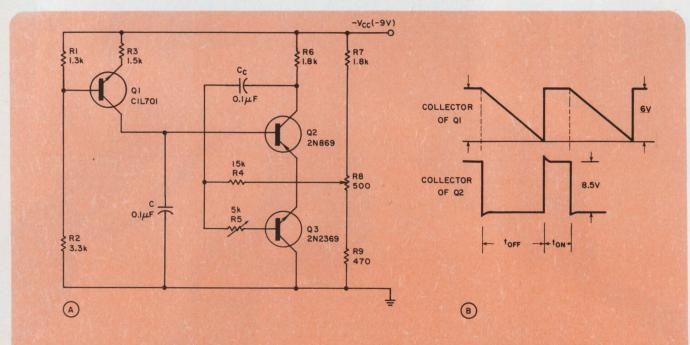
**Voltage ramp having excellent linearity,** is developed at the collector of Q1 as a result of capacitor C being charged from a constant-current source.
