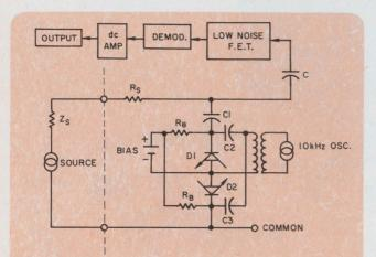
1. Solid-state "vibrating capacitor" electrometer uses two reverse biased, back-to-back voltage variable capacitors.
