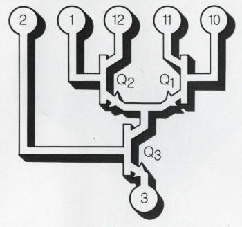
Here's another of RCA's growing family of "building block" IC's—usable as high-speed sense amplifiers, low noise IF and RF amplifiers, balanced mixers, wideband amplifiers, oscillators, and many more.
