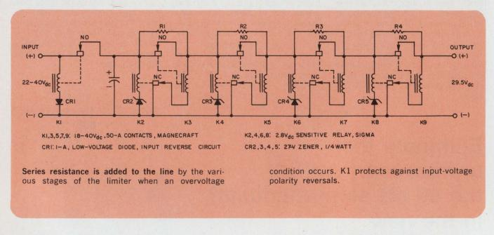
applied to systems having other power requirements by changing zeners, power relays, and resistors accordingly. Howard Cohen, Project Manager, Decitron Electronics Corp., Brooklyn, N.Y.
