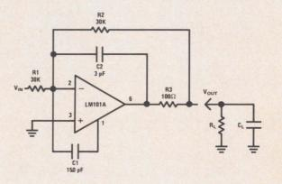
FIGURE 7. Capacitive Load Isolation
