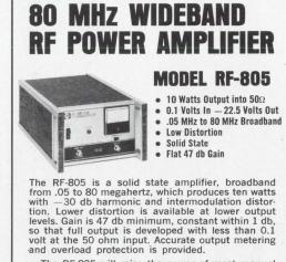
The RF-805 will raise the power of most manual and swept tuned signal generators and thus extend the usefulness and versatility of available signal generators. Receiver testing, wattmeter calibration, antenna testing, RFI testing, attenuator measurements, and filter and component testing will be aided with the use of this equipment.
