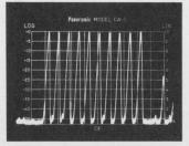
3. The high resolution of the Singer Model SSB-50-1 provides this clear display of the multiplexed channel. The amplitude of each subcarrier is shown as a function of frequency. The display demonstrates complete operational readiness at a glance.
