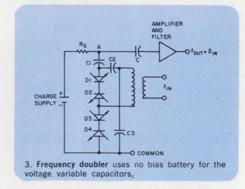
It should be noted that the efficiency of all these circuits is extremely high.
