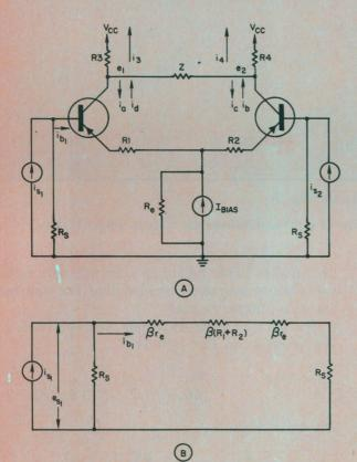
3. Differential amplifier with single-ended current sources (A) has the equivalent circuit of (B) when  $i_{s2} = 0$ .
