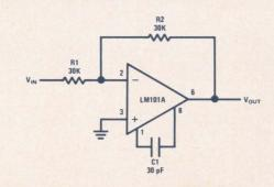
FIGURE 1. Standard Frequency Compensation
