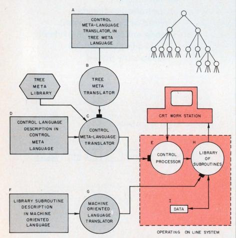
2. A hierarchy of languages help give the on-line graphical interaction system its flexibility. The tree structure used for organizing information for quick retrieval (upper right) is a basic principle upon which the system is designed.
