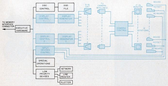
1. **On-line computing system** used at SRI includes 5-inch precision CRTs whose presentations are picked up by a high resolution TV camera and then transmitted to one
