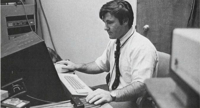
**Spellbound by a graphic console,** a Stanford Research Institute designer churns data into a computer by means of a "mouse" (right hand) and five "piano keys." This permits text to be written and modified without his eyes leaving the screen. Details on p. 25
