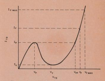
1. The negative-resistance characteristic of the tunnel diode is the heart of the threshold sensor. The circuit changes state when the input current to the diode exceeds the peak current  $I_{\rm p}$ .
