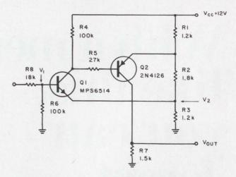
1. **Complementary circuit provides** Schmitt-trigger type operation with a zero output-voltage offset at a savings of one transistor over the conventional three-transistor approach.
