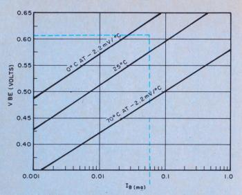
4. The base-emitter characteristic of the transistor used must be drawn for the temperature extremes at which the circuit must operate. These curves are used in the iterative design procedure to ensure that the transistor remains off when the input current is below the threshold.
