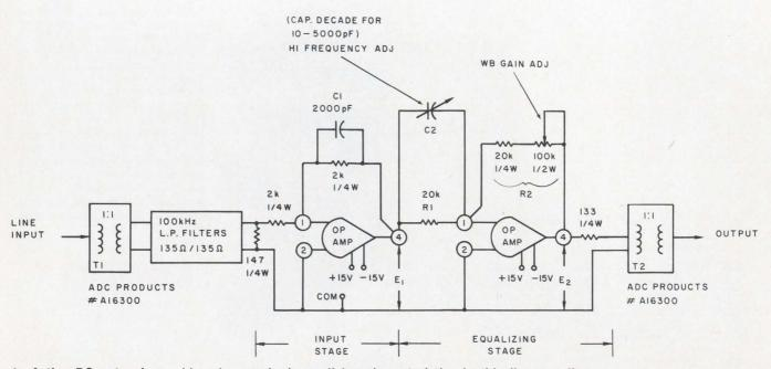
1. Active RC network provides the required equalizing characteristics in this line equalizer.
