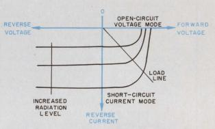
4. **Photodiode operation** can take place in either the third- or fourth-quadrant of the current-voltage characteristic.
