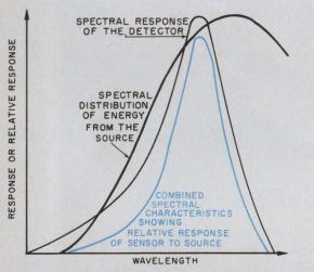
3. Combined characteristic shows the coincidence between spectral response of a detector and the spectral distribution of the source.
