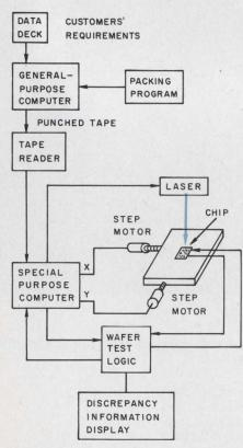
1. Automatic encoder-tester can encode and functionally test a 1024-bit array in 5 minutes. logic "1," and disconnected diodes as logic "0."
