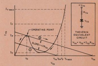
3. An equivalent voltage source and series resistor feed current to the tunnel diode. This combination yields load lines as shown, with slope depending on the series resistance and position depending on the input current  $I_{\rm IN}$ . The operating point moves up with the load line as  $I_{\rm IN}$  is increased until it reaches  $I_{\rm P}$ , then it jumps to the second positive resistance region. The output voltage  $V_{\rm OUT}$  drops suddenly as the circuit changes state.
