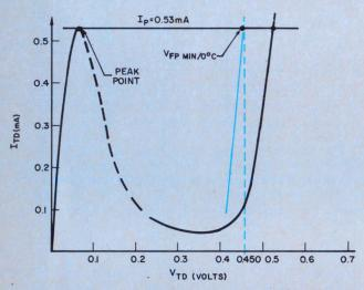
5. The lowest  $V_{\rm FP}$  expected over the operating temperature range of the sensor is plotted on the diode curve. This voltage, added to the voltage drop across the resistor R<sub>D</sub>, must be sufficient to turn on the transistor.
