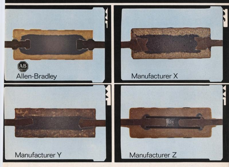
The above illustrations are from unretouched photomicrographs taken of four  $\frac{1}{2}$ -watt fixed resistors. Compare the anchoring of the leads, the seal provided by the insulating jacket at the ends, the homogeneity of the resistance material, the sharp color code bands—and decide for yourself.
