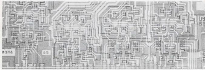
**MSI 4-bit counters** perform synchronous counting at speeds greater than 15 MHz.
