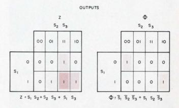
4. Karnaugh maps are used to simplify the circuitry and to relate the toggle signals to the flip-flop states and the inputs. The state of each flip-flop is given by the corresponding S number. Thus,  $S_2$  gives the state of FF2.
