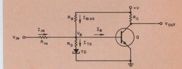
2. The threshold sensor uses a tunnel-diode transistor combination to provide output drive capability. The current through the diode is a measure of the voltage  $V_{\rm IN}$ . When  $V_{\rm IN}$  rises enough to cause  $I_{\rm P}$  to flow through the diode, the output voltage  $V_{\rm OUT}$  suddenly drops to the "low" state.
