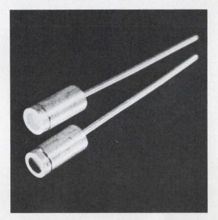
The light-activated silicon controlled rectifier is exactly analogous to the normal SCR, except that light provides the gate triggering. The gate-cathode junction acts as a photodiode to generate the triggering current. Optimizing the light-sensitive properties of the SCR, however, causes it to be more sensitive to heat. This problem limits the device to a restricted range of operating temperature.
