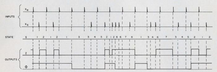
1. A train of reference pulses,  $X_{\rm R}$ , and a typical received signal,  $X_{\rm s}$ , which are to be phase locked, are shown. The system states are identified on the third line. The
