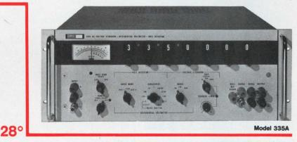
Ordinary room temperatures are just dandy for Fluke calibrators. For instance, our Models 332B and 335A are specified to an accuracy of 20 ppm at 23° C. And, in typical room environments, accuracy is degraded by only 10 ppm.
