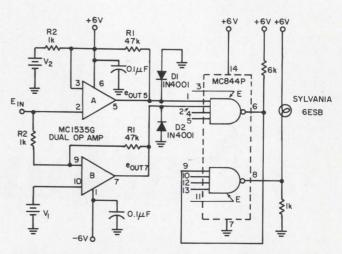
2. When circuit senses out-of-range condition, the pilot lamp becomes lighted.
