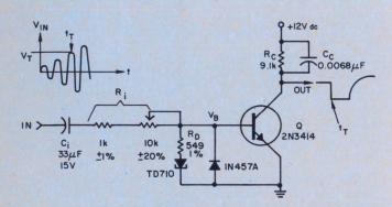
6. An ac coupled threshold detector senses the peak values of a 10 kHz sine wave, if they exceed a preset level. The diode connected from base to emitter discharges the coupling capacitor during the negative half-cycles of the input waveform.
