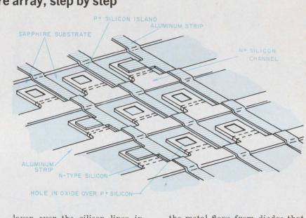
layer over the silicon lines insulates the two conductors at the crossovers in the matrix. Encoding is done by removing the metal flaps from diodes that are to represent logic "0." The remaining metal-covered diodes represent logic "1."
