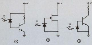
5. Short-circuit current mode of photodiode operation provides a simple linear light-intensity transducer.
