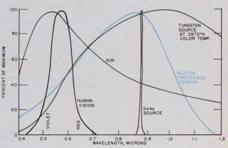
2. Spectral characteristics form the basis for matching a photodetector to a light source. Some common characteristics are shown here.
