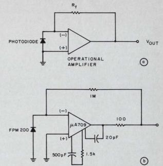
8. **Basic light-sensing system** (a) provides an output voltage that is linearly related to the input light intensity. An actual circuit of this type is shown in (b).
