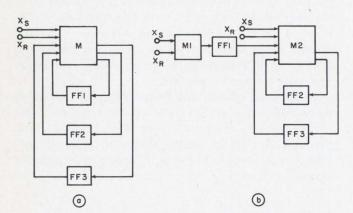
3. Decomposition can simplify a design. Before decomposition (a) three flip-flops had to be considered in designing logic network M. After decomposing the system into two subsystems (b), by having flip-flop FF1 differentiate between state groups, the logic is reduced to two simpler networks.
