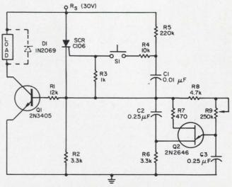
The output pulse duration is controlled by resistor  $R_9$ , which determines the charging rate of  $C_3$ .
