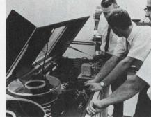
Plated disc memory with multiple read/write heads
