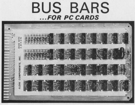
A laminated bus bar with distributed capacitance on a printed circuit card for power and ground distribution, eliminating the need for a multilayer card.
