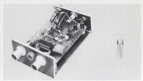
Discrete circuit write amplifier at left was shrunk to hybrid version at right, in TO-5 case.
