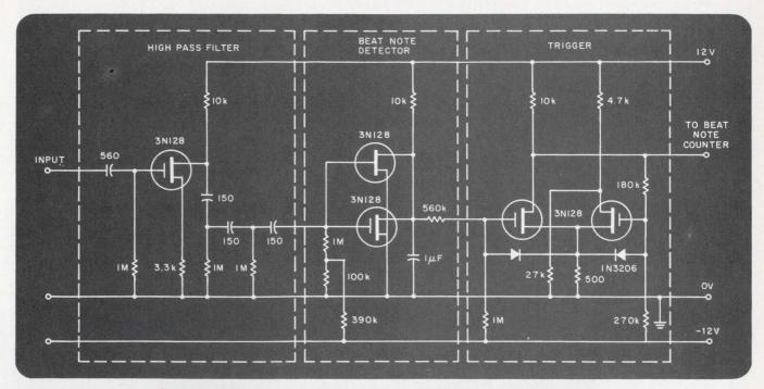
5. The high pass filter, beat note detector, and trigger detect "lock-in" and generate beat-note pulses.
