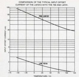
An order of magnitude improvement. The LM 101A has every advantage of the LM 101, but with 20 nA offset current and 100 nA bias current guaranteed over a  $-55^{\circ}$  to  $125^{\circ}$ C temperature range.
