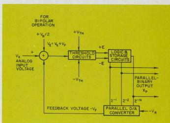
2. Parallel-feedback a/d converters use feedback between output and input to control the conversion process. The feedback is provided by a parallel d/a converter.
