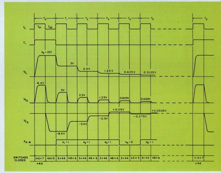
16. Waveforms of the charge-equalizing converter show that digital output  $X_{\mathrm{S-M}}$  is a ONE when voltage
