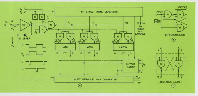
5. The successive-approximation a/d converter sets each output storage circuit to either a logical ONE or ZERO in accordance with input  $V_{\rm x}$  and feedback voltage  $V_{\rm f}$ . The
