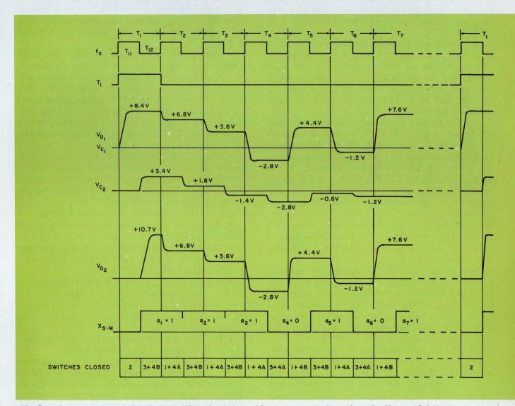
10. Sample waveforms of the dual-amplifier circulation a/d converter are shown here for  $V_{\rm X} = +8.4$  V.
