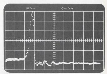
2. A train of very short pulses, rich in harmonics, provides frequency markers which are spaced at intervals equal to the repetition frequency of the pulse train.
