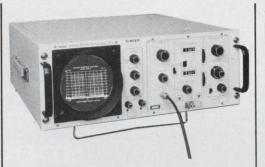
A **UR-3** module (100 Hz to 700 KHz) is ideal for applications in telemetry systems. This module is shown here scanning all 21 constant bandwidth IRIG telemetry channels.
