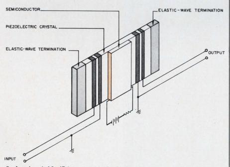
2. A gain of 12 dB/cm was obtained with this phonon amplifier using a lead-zirconate-titanate piezoelectric crystal and n-type silicon as the semiconductor. The elastic-wave terminations prevent reflections by absorbing the acoustic waves that hit them.
