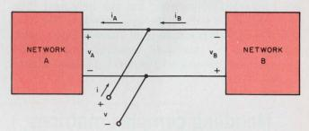
1. Forced equality is imposed on all voltages in a parallel interconnection. The current, i, of the new port is the algebraic sum of the currents of the original ports.
