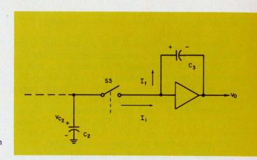
13. Adding of charges can be accomplished with an operational amplifier and two capacitors.
