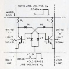
3. A photosensitive flip-flop must be more sensitive than one that is written into electrically, because the amount of light available is limited. Two extra diodes are added and are connected to a hold/erase line. This arrangement allows complete discharge of both transistor bases.
