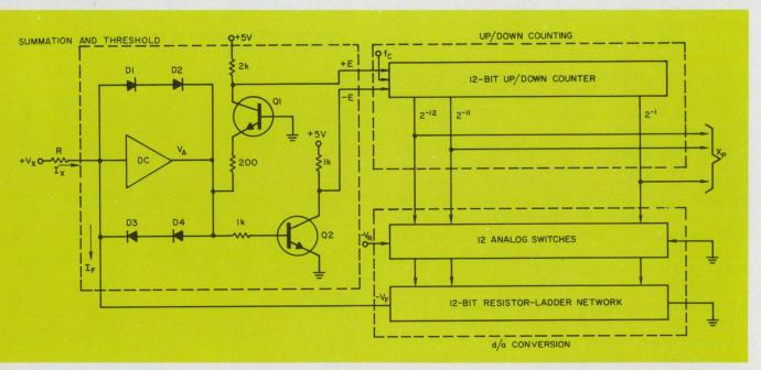
3. The servo a/d converter uses an up-down counter to generate the digital output signal. The counter is driven
