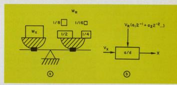
1. The mechanical process of weighing (a) is analogous to analog-to-digital conversion (b).
