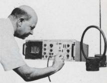
The **VR-4** module (1 KHz to 27.5 MHz) can be used to survey the entire communication frequency spectrum. For this and other applications, Singer provides a full range of accessories, including both antennas shown in this picture.
