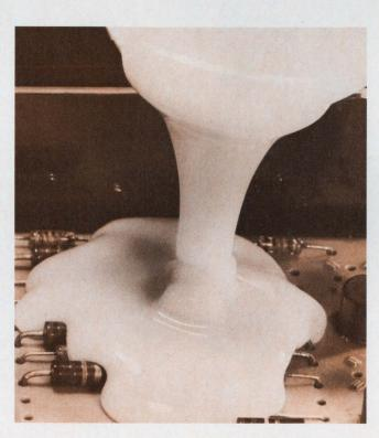
New premixed, ready-to-use white Sylgard silicone encapsulating resin flows freely around components and provides virtually unlimited working time at room temperature... cures in one hour at 135 C and in two hours at 100 C... no post cure required... no reversion... low water absorption... self-extinguishing.
