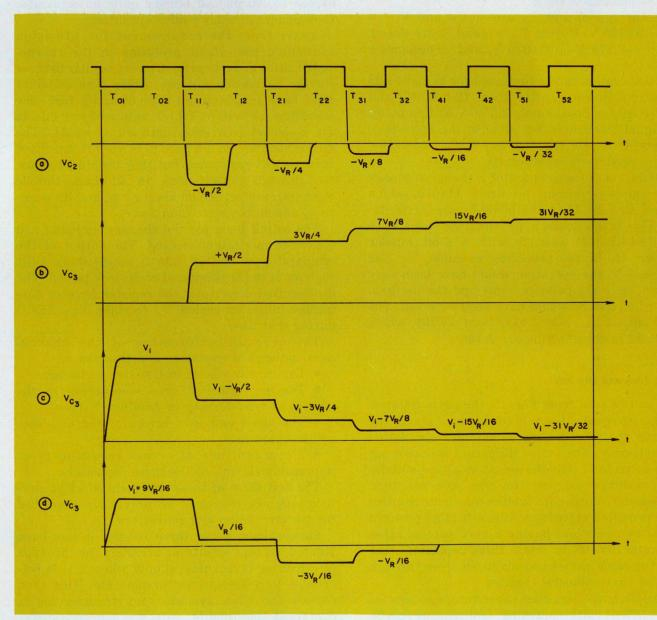
14. Waveforms show how the addition of charges by the dc operational amplifier and two capacitors of Fig. 13
