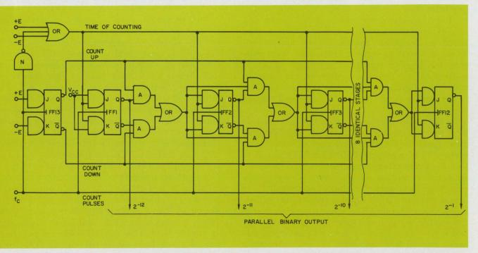
4. Serial-carry counter is enabled when either error signal, + E or - E, is LOW. When both error signals are
