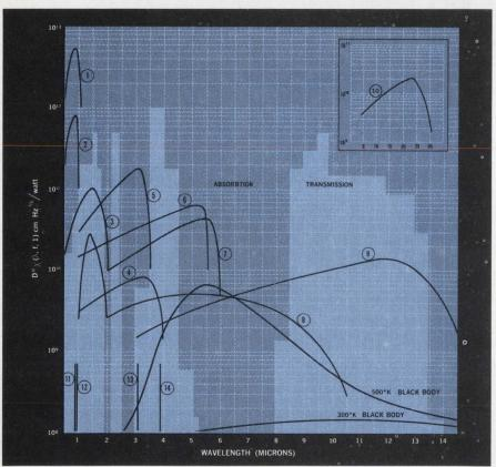
Ge (Au) (PC), 12° GaAs EMITTER 300°K InAs (PV), 300°K Si (PV). GaAs (PV). 300°K InAs (PV). 196°K 9 Ge (Hg) (PC). 30°K 13° InAs EMITTER 77°K 10 Ge (Cu) (PC), 4°K 14° InAs EMITTER 300°K InSb (PV) Ge (PV). 300°K InSb (PC). 77°K 11° GaAs LASER
