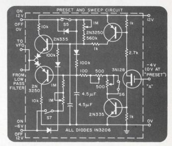
7. The sweep circuit "pulls" the VCO frequency upward or downward, depending on the position of the switches, until the beat note counter and logic apply ground to input A.
