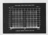
When two channels drop away, their absence shows up instantly on the spectrum analyzer's CRT display. The analyzer is also used for checking signal to noise ratio, the amplitude taper of a telemetry system, or distortion. Besides scanning all the channels, it can provide an expanded display of any one of them.
