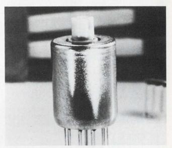
IC-compatible rotary switch packs ten positions in 5/16-in. diameter. Page 104
