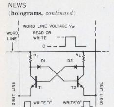
2. A charge-storage flip-flop results from the addition of two diodes to a conventional flip-flop. The diodes retard the discharge of the base region of the ON transistor, giving the flip-flop a short-term memory.
