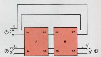
3. The most general interconnection of two networks has both series and parallel connections. The two 4-port networks shown here are the same ones shown in Fig. 2, and the same notation applies.
