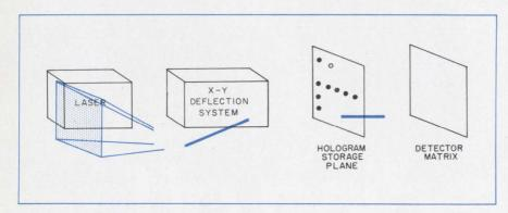
1. A proposed hologram-reading array uses modified charge-storage flip-flops for optical data read-in. Information stored in the hologram in binary form is reconstructed in an array of light spots in a readout plane. Each spot occupies one of two positions and thus corresponds to a binary bit. The array of light sensitive flip-flops at the readout plane is set or reset according to the positions of the light spots.
