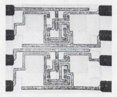
Light-sensitive flip-flops are the basic cells of the hologram-reading array. The base regions are made quite large (4 by 4 mils) to increase the amount of photocharge accumulated and thus the sensitivity.
