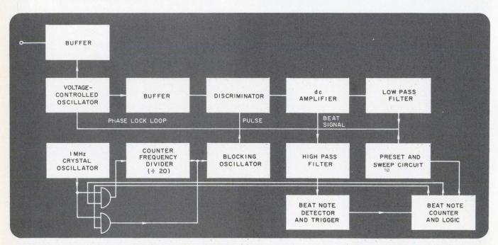
1. This frequency synthesizer eliminates high-frequency counters and avoids the associated high current drain. Only one divide-by-N counter is used, at a comparatively
