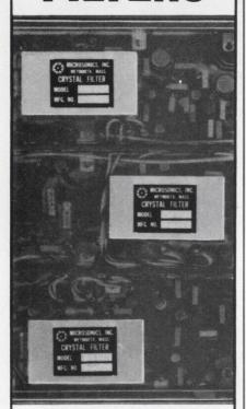
Microsonics, Inc. has designed and developed phase tracking crystal filters, in which the phase between filters will track within close tolerances, over wide temperature ranges, without temperature control. Any one of the standard multi-pole filters such as Butterworth, Tchebycheff, Bessel, etc. may be obtained with phase tracking requirements. In the event of tight tracking requirements, the filters are produced in matched sets according to the customer's requirements.
