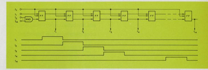
6. Ring counter is a simple way to implement the 14-stage timing generator needed in the successive-approxi-
