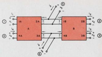
2. Cascaded networks have ports connected in parallel; the new ports thus formed are not considered ports of the network. Thus, currents at these ports must be constained to be zero.
