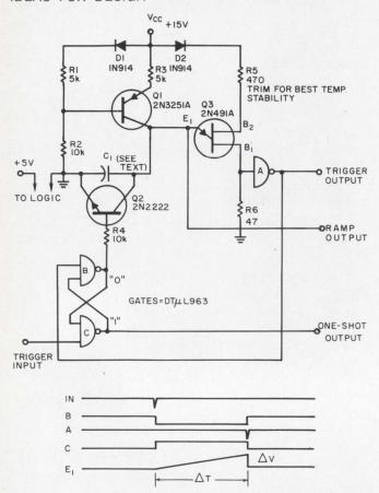
A latch enables the generation of a single-shot pulse, ramp and delayed trigger.
