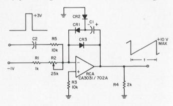
Ramp generator has a fast fall time and is fairly linear. All diodes can be any germanium types. The value of C is selected to provide the desired period.
