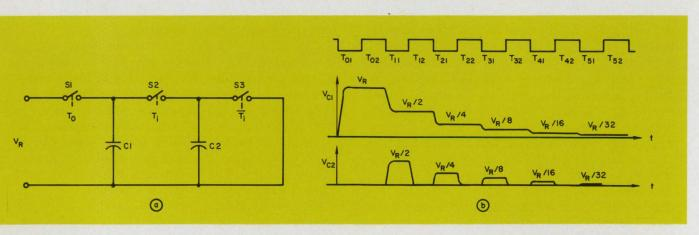
12. Equalizing charge between two capacitors provides a method of generating the binary fractions  $V_{\rm R}/2$ ,  $V_{\rm R}/4$ ,
