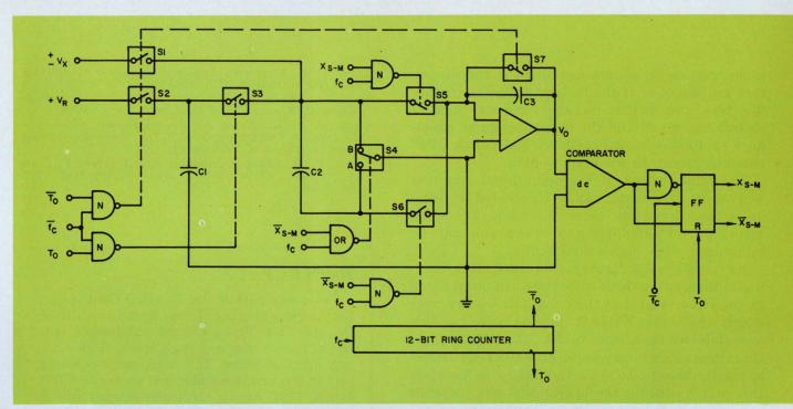
5. The charge-equalizing a/d converter uses two capacitors, C<sub>1</sub> and C<sub>2</sub> to generate the binary fractions.
