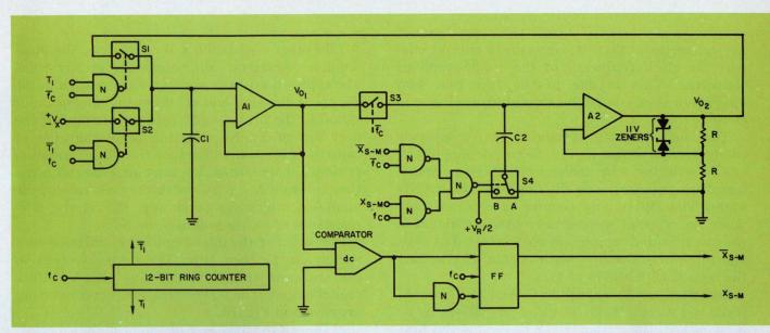
9. Two sample-hold circuits are used in the dual-amplifier circulation a/d converter. SH1 has unity gain. SH2
