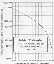
Insulation resistance of STABELEX Capacitors can reach 10,000,000 megohm-microfarads or more at room temperature or above under certain operating conditions. This feature, plus their low temperature coefficient of capacity, low power factor and extreme stability, makes STABELEX Capacitors the logical choice for instrumentation and other advanced circuitry.
