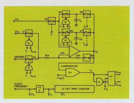
7. The single-amplifier circulation a/d converter employs two capacitors,  $C_{\rm A}$  and  $C_{\rm B}$ , alternately as storage devices. When  $C_{\rm A}$  is charged,  $C_{\rm B}$  holds, and vice versa.
