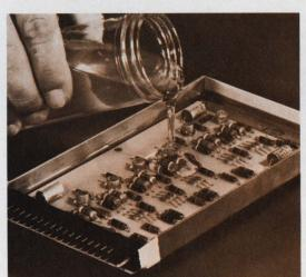
Shock and vibration are two of the operational environments that take heavy toll of delicate electronic gear. Improved protection is available with a new shock absorbent Dow Corning solventless silicone encapsulating resin which absorbs these forces with very little internal reaction.
