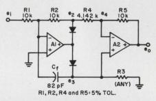
2. Degenerate form of ideal rectifier uses only four precision resistors.
