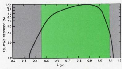
The response of the photodiode is 5 ns from 0.45 to 1.1 microns, or from the near ultraviolet to the near infrared.
