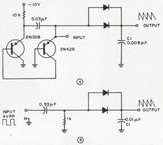
**Sawtooth** is obtained when a sine, square, or triangular waveform of 4-V pk-pk is applied to the input (a). For square waves the circuit reduces to (b). Two diodes are used to lower output resistance to increase rise time.
