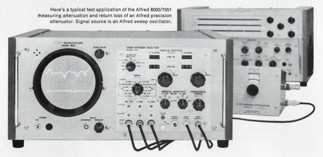
Now, with one totally new instrument, measure gain, loss, absolute or relative power levels, VSWR, and impedance magnitude (reflection coefficient). The new Alfred 8000/7051 system speeds and simplifies rf and microwave measurements.
