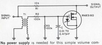
No power supply is needed for this simple volume compressor circuit.
