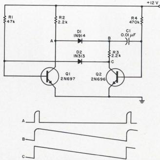
A linear sawtooth is obtained from this simple circuit. With the values shown the period is about 2.5 ms. Waveshapes existing at various points are shown below the schematic.
