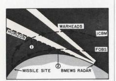
The low-flying FOBS travels a long way before it is detected by the lineof-sight Ballistic Missile Early Warning System (BMEWS). ICBMs, for which BMEWS was designed, fly much higher and disturb the radar's lower, fan-shaped beam soon after leaving the pad.
