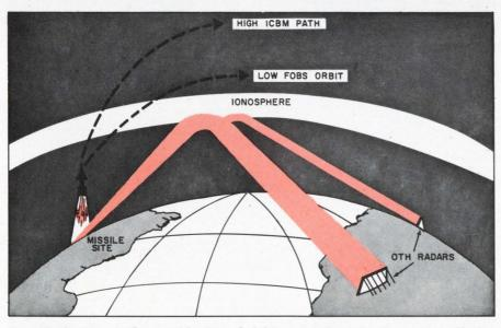
**Over-the-horizon radar** avoids line-of-sight restrictions by bouncing off the ionosphere to detect launchings of ICBMs and FOBSs alike at the site. A signal that bounces off the horizon only once can reach a target as much as 2000 miles away. Those that zigzag up and down twice or more reach much farther.
