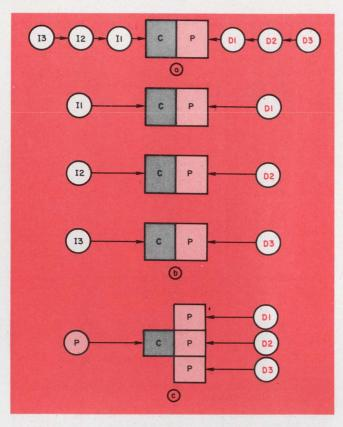
1. **Development of parallelism** began with the aim of improving the throughput of the pipeline computer (a). Simply paralled identical processors (b) executing the same program could have common control logic (c).
