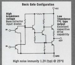
Device dissipation (typ) 2.3mW per Gate —7mW per Flip-Flop. Full military operating temperature range— -55°C to +125°C Flip-Flop clock frequencies (typ) 3MHz. Single power supply +3.8V to +6.3V; 4V optimum. NAND gates pincompatible with popular 930 DT Lcircuits.
