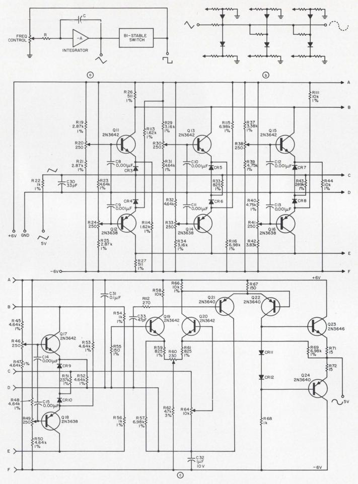
Sine waves obtained from (c) are derived from the basic triangle- and square-wave generator (a) after clipping in
