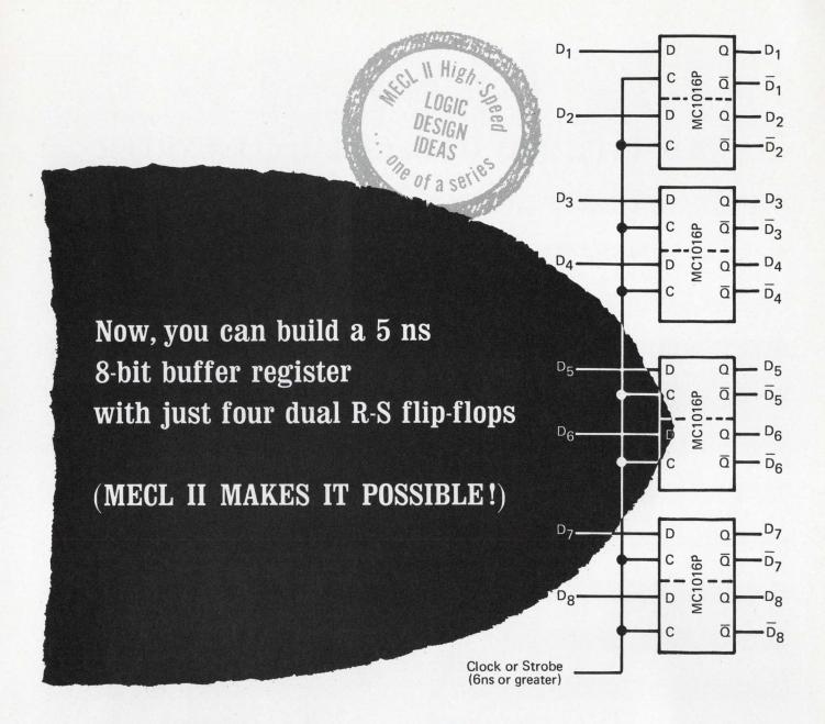
Yes, there's a new, simplified, less-expensive way to build a highly-versatile, widely-used 8-Bit Buffer Register. Simply use four MC1016P integrated circuits from Motorola's MECL II
