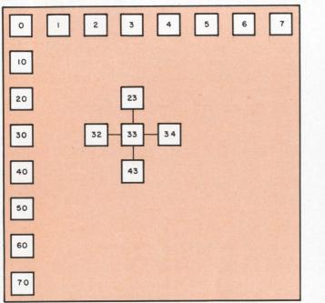
3. **Direct parallel word transfers** between processing units are only allowed between nearest neighbors. The transfers are maintained for both separate and joined quadrants. Note the octal numbering system.
