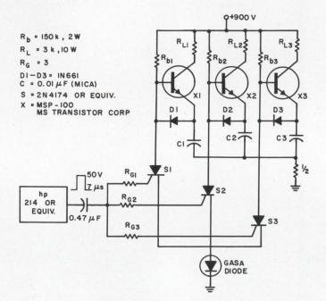
**300-A**, **80-ns pulses** needed to operate a GaAs laser are delivered by this three-parallel-stage circuit at 10 kHz.
