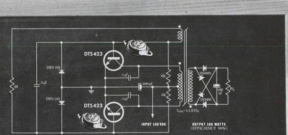
Application of Delco high voltage silicon power transistors: the DC to DC Converter.
