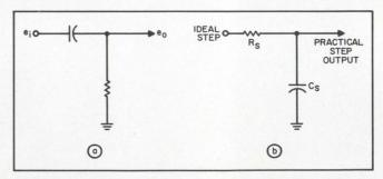
1. Passive RC differentiator (a) passes leading edge of step input but discriminates against a dc level. Equivalent circuit of stray resistance and capacitance (b) is really a lag network. The time constant is difficult to measure — it is easier to think of it as the time it takes the practical step function to reach 63.2% of its maximum value.
