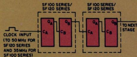
Fig. 6—High-speed ripple counter can be clocked at up to 50 MHz.
