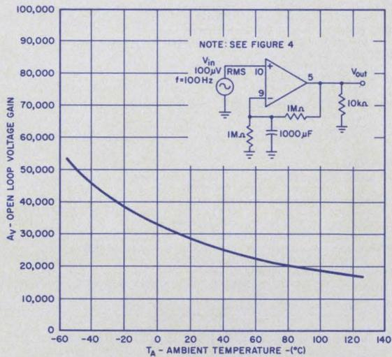
OPEN LOOP VOLTAGE GAIN VS AMBIENT TEMPERATURE
