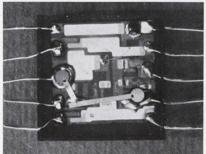
6. In the schematic for a single stage, S1, S2, and S3 are shorts that can be opened to adjust input impedance (above). The stage is made on glass (below).
