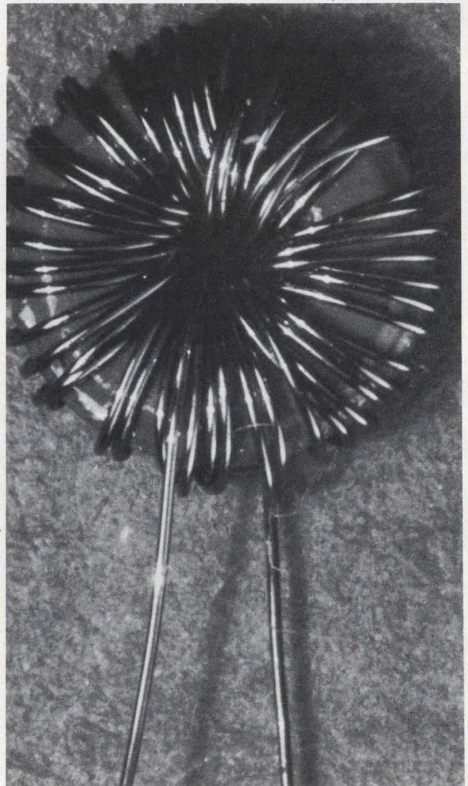
This miniature inductor is used to tune the circuits to the proper center frequency.
