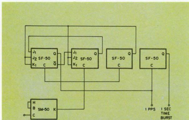
Fig. 1—Simple, accurate 1-Hertz generator using SUHL ICs.
