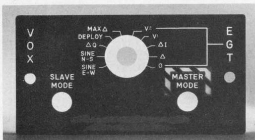
For visibility and legibility without eye strain, the edge lighted instrument panel is unsurpassed, especially under adverse ambient light conditions.
