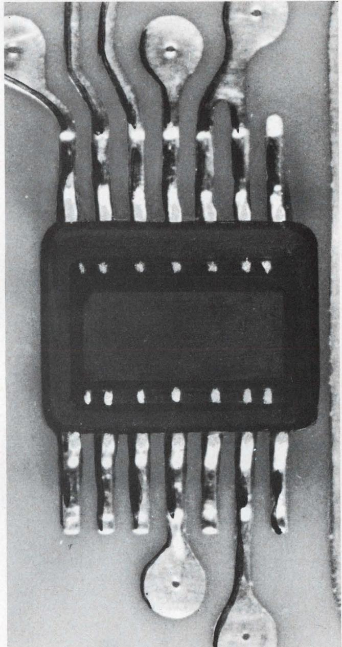
Prealloyed solder-and-flux creams improve quality of microelectronic soldering. Page 90
