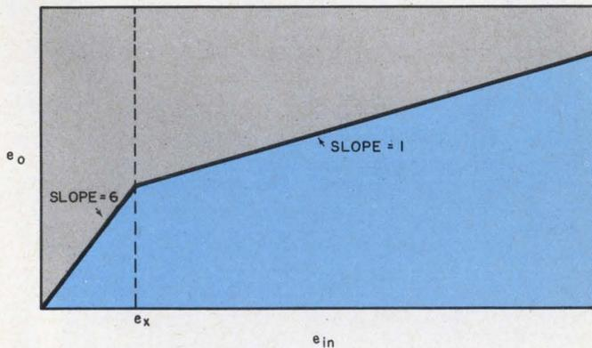
4. Duo-gain characteristic shows small-signal gain = 6 ( $e_{in} < e_x$ ) and large-signal gain = 1 ( $e_{in} > e_x$ ).  $e_x$  is the voltage across  $R_x$ .
