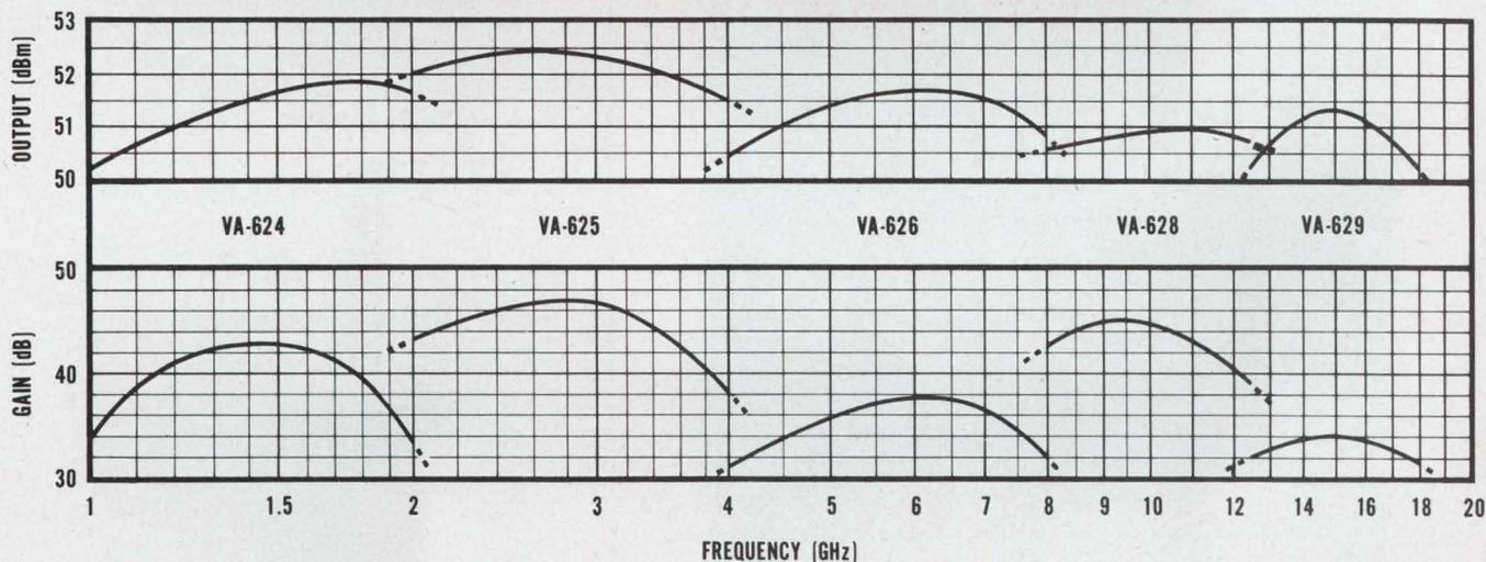
Varian's  $\geq 50$  dBm CW TWT's offer unmatched performance over the 1 to 18 GHz frequency range. These tubes can be supplied with air or conduction cooling and are conservatively rated at 100 watts, but can be supplied to deliver over 200 watts of r-f output power. (Similar TWT's are available at the  $\geq 20$  watt level).
