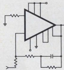
For example, Radiation's RA-239 Broadband Amplifier is used in the lag-lead DC servo preamplifier illustrated. Feedback components are selected to optimize overall preamplifier parameters... without regard to the active element in this configuration.
