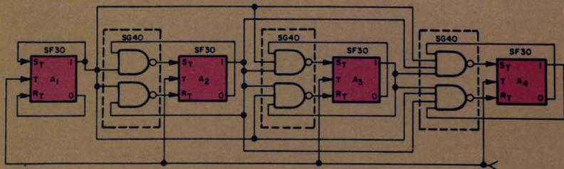
Fig. 3—Synchronous binary counter with SRT flip-flops.
