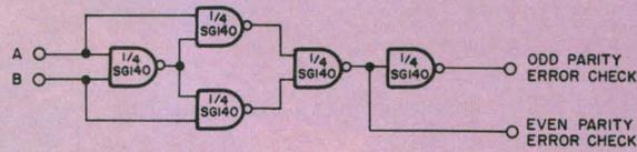
Fig. 2—ODD/EVEN parity checking for two bits.
