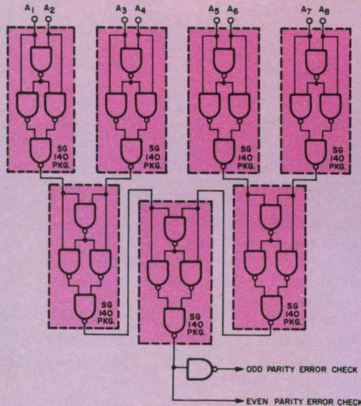
Fig. 3—Parity checking for 8-bit binary word which includes the parity bit.
