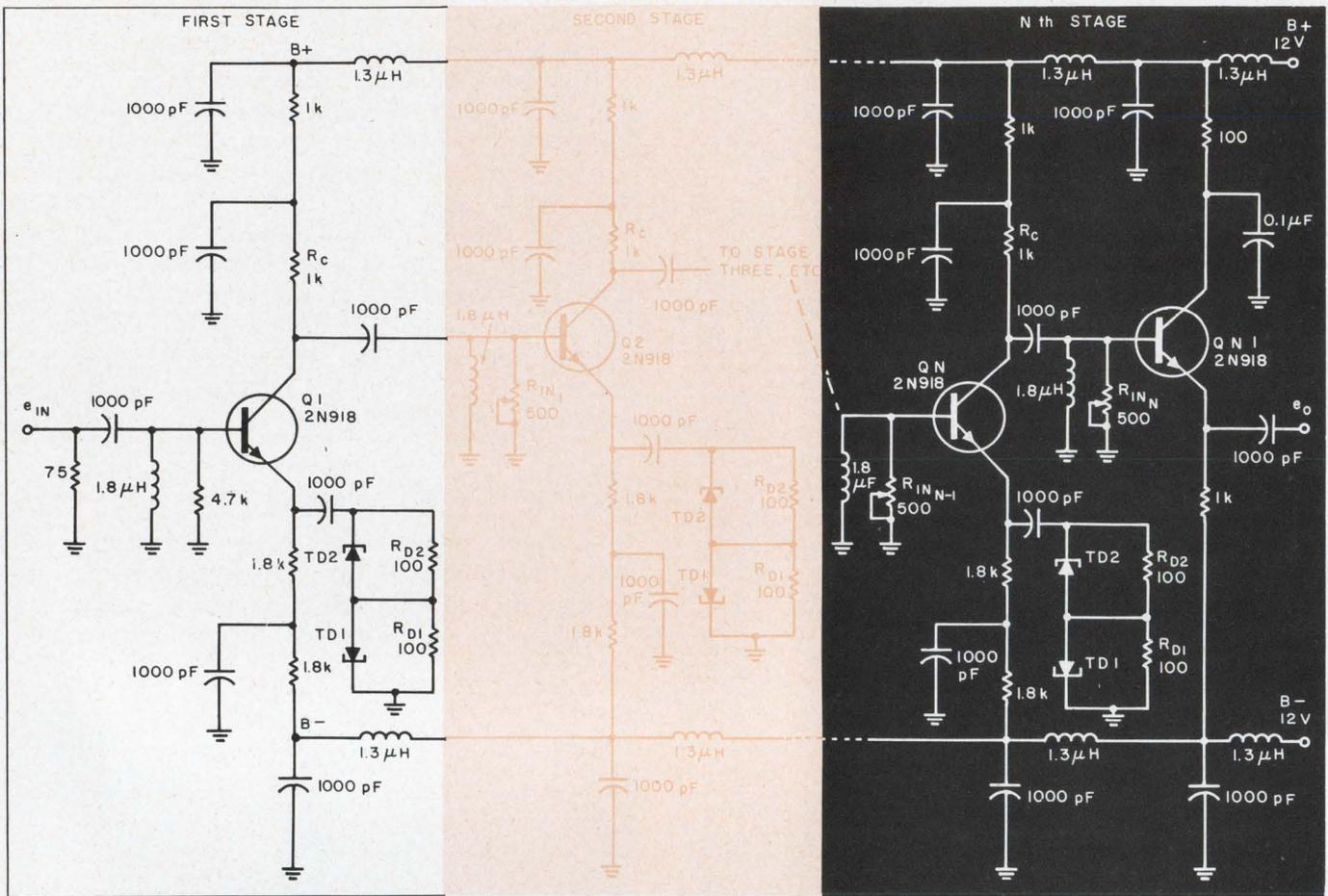
7. Complete schematic shows input stage, output stage and N<sup>th</sup> stage. All capacitor values are in pF. Transistors
