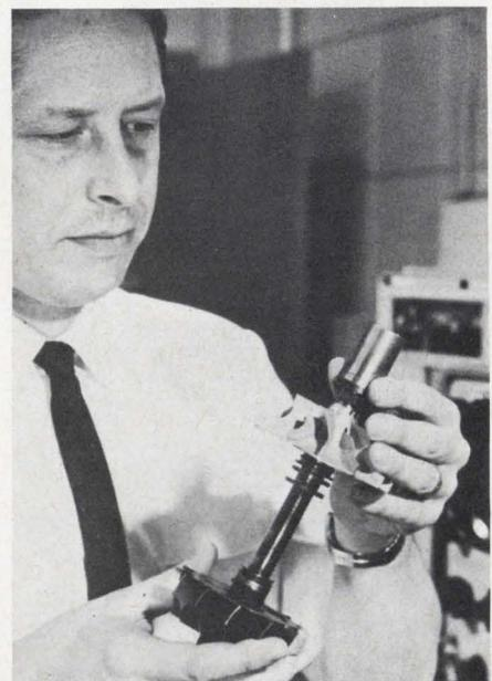
Tiny FM transmitter mounted on a turbocharger impeller is able to relay strain gauge signals when the shaft is rotating at 100,000 rpm.
