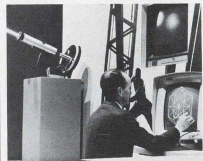
An infrared light beam carries data between an IBM System/360 computer in the Canadian Government pavilion at Expo 67 and a receiving unit and graphic display terminal (above) in the Man the Producer pavilion half a mile away. The path of the beam has been simulated by photographic retouching.
