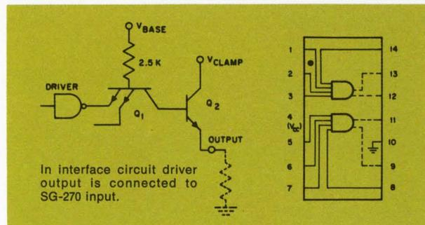
in the Figure. Here, the driving gate (or gates) is connected to the input of an SG-270 dual 4-input OR expander.
