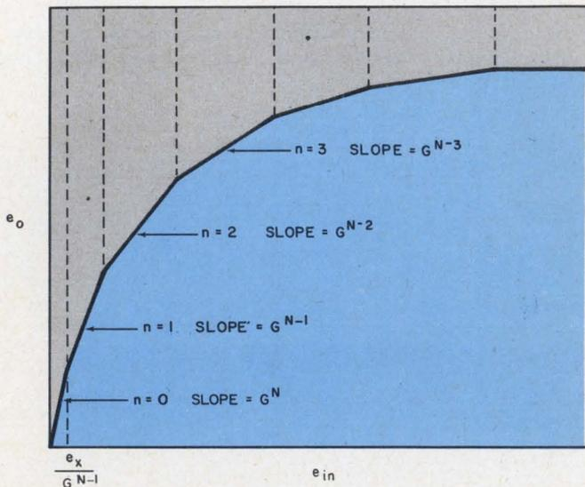
5. Cascading many stages yields an amplifier with a linear response for small signals and a logarithmic response for large signals.
