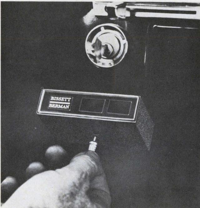
**Tiny electrochemical timing cells** are the heart of this auto maintenance computer. Page 122
