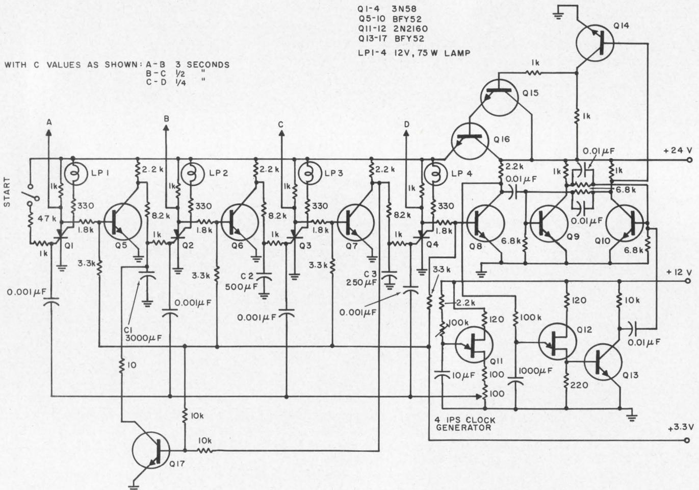
Time delay between events can be varied in this programmed sequence switch. Input to the switch may be
