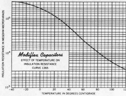
The new Modiflex Capacitors utilize a synthetic film and a liquid plastic dielectric to produce a capacitor with highly desirable characteristics.
