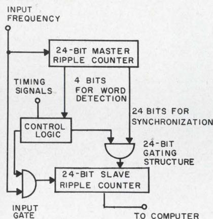
Two 24-bit ripple counters are used, one a master, the other a slave. Both counters count the input frequency, but in addition, the slave counter may either be synchronized with the master counter, or disconnected from the input frequency by the control logic.
