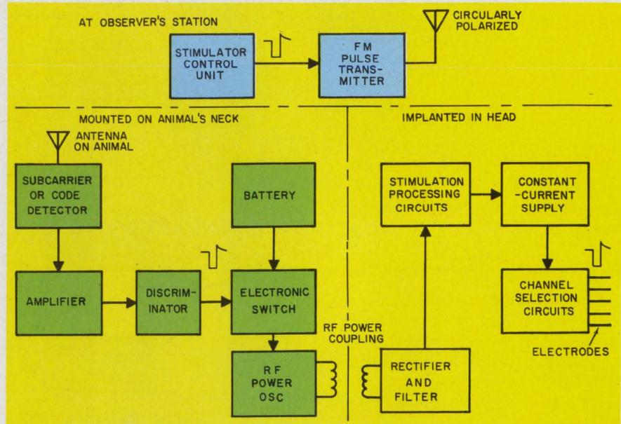
2. **Microminiaturized implantable stimulator** would draw power from electronics pack mounted on animal without using leads that pierce the scalp. Integrated circuits and biological power source might permit implantation of receiver and antenna as well.
