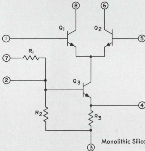
Monolithic Silicon Integrated Circuit, CA3028
