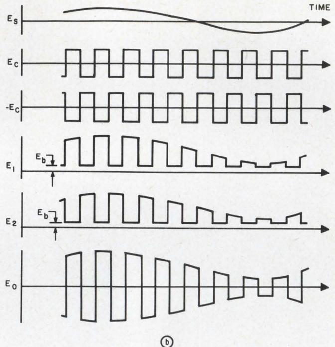
Amplitude modulated output, *E<sub>o</sub>*, is obtained with the simple circuit (a). All waveforms on common time base are shown in (b).
