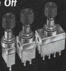
Exceptionally high current. Positive snap-action with fast make and break contacts. SPDT, DPDT & 4PDT, useable as either a Normally Open or Normally Closed switch. Silver contacts and terminals.
