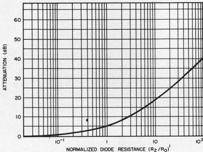
2. **Continuously variable attenuation** is achieved by changing the diode's resistance. Here the resistance is normalized with respect to the system's impedance,  $R_0$ . It is assumed that both diodes in Fig. 1 have the same resistances; which vary from 0.5 to 5000 ohms. The range of the attenuator is greater than 40 dB, and its insertion loss is less than 0.1 dB.
