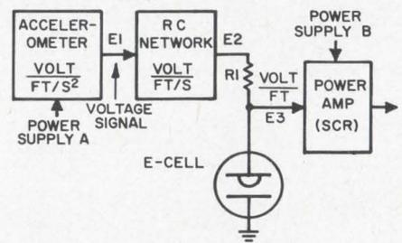
3. **Double-integration function** is performed as E-cell provides a signal source which indicates the distance from the voltage output of an accelerometer. Uses are in airborne cargo drops or ordnance.
