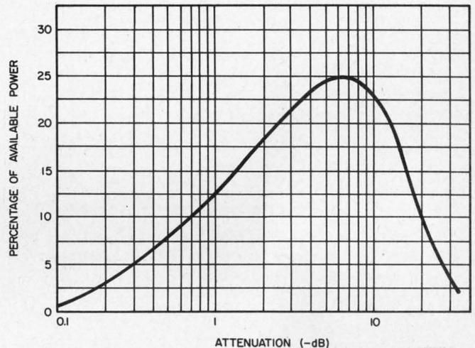
3. **Dissipation in the diodes reaches its peak** at the 6-dB attenuation level. The absorbed power is expressed as a percentage of the total input power. Each diode must therefore be rated to dissipate one-fourth of the controllable power. However, if  $R_1 R_2 = R_0^2$ , then even a larger percentage of the input can be dissipated in a diode. Diodes can dissipate 1 to 5 watts with good heat sinks.
